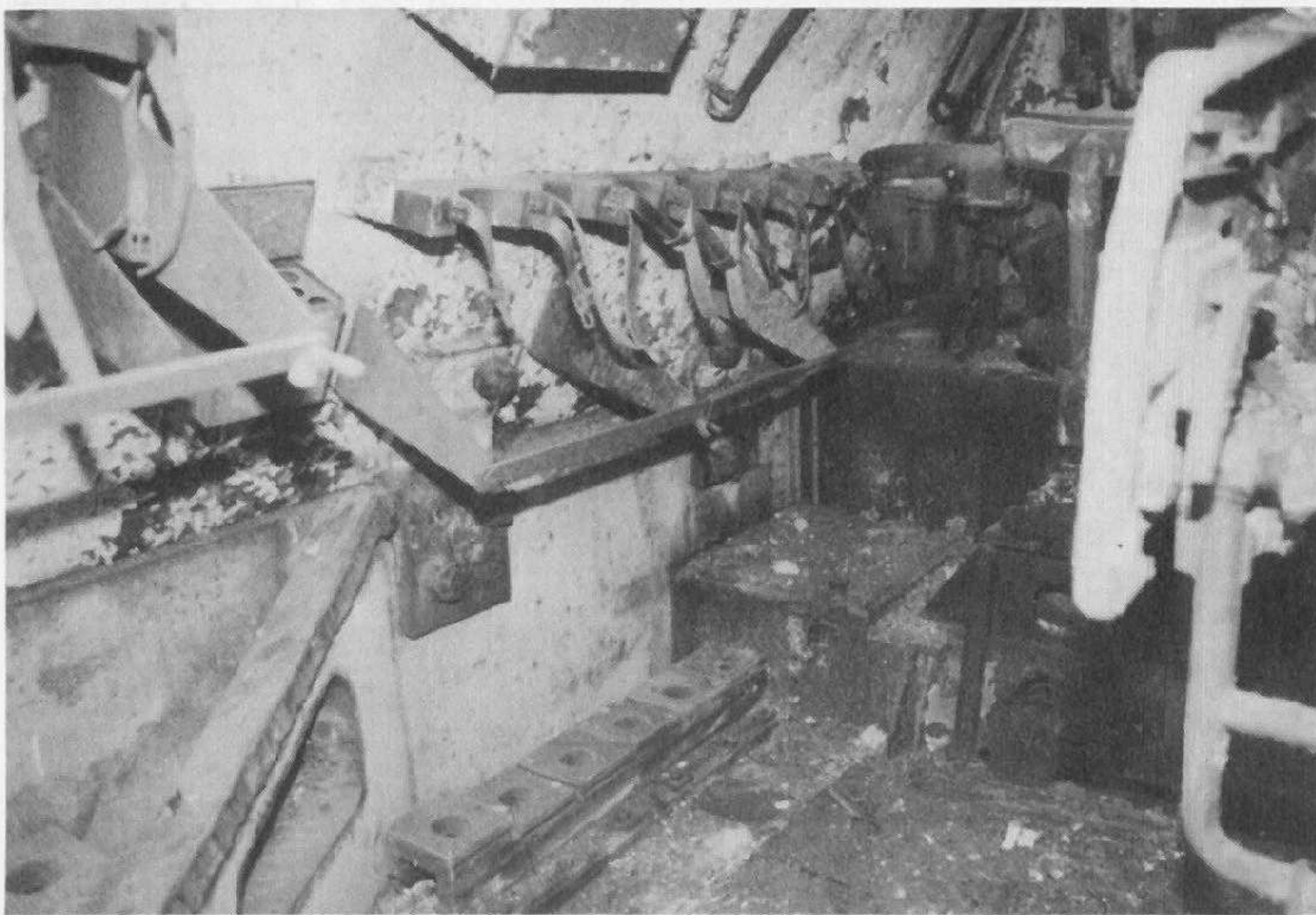
The ammunition in the Elephant was stowed nose down, with the projectile resting in a hole cut in a wooden block. A frame mounted on the wall had leather straps that secured the other end of the round. The differences in the two colors of the interior is very obvious here.
