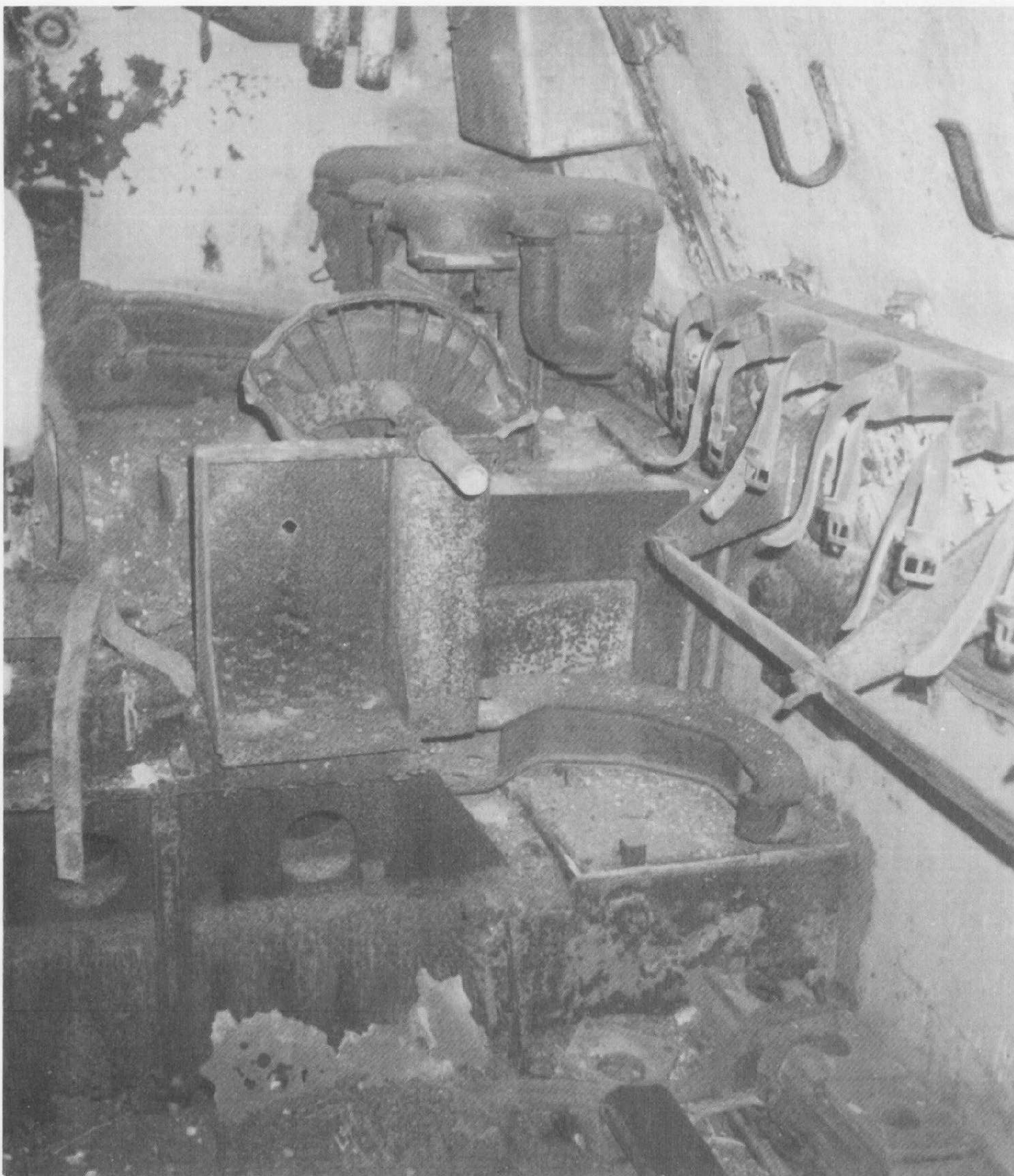
An overall look at the fighting compartment to the right side of the main gun. The commander's seat is folded forward. Except for the floor, the inside of the vehicle is in better condition than might be expected. Of interest is the color of the interior. The walls of the fighting compartment were painted a shade of white while the walls of the hull (seen in the lower right of this photo) appear to be a green/gray color.
