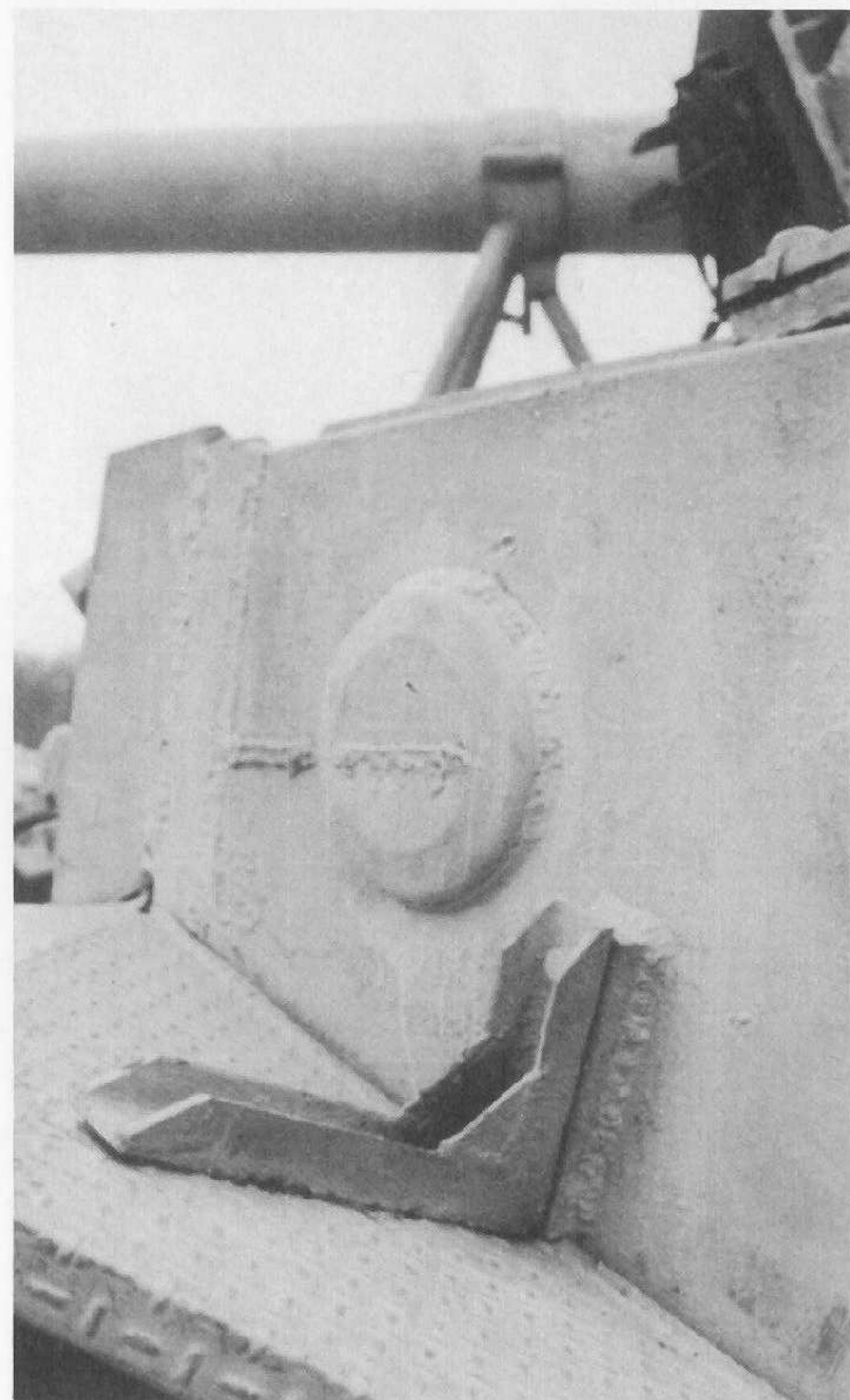
The angled plate off of the frontal armor on each side had a round view plate with a view slit in the center. The front fender support and the thickness of the frontal add-on plate are shown here as well.
