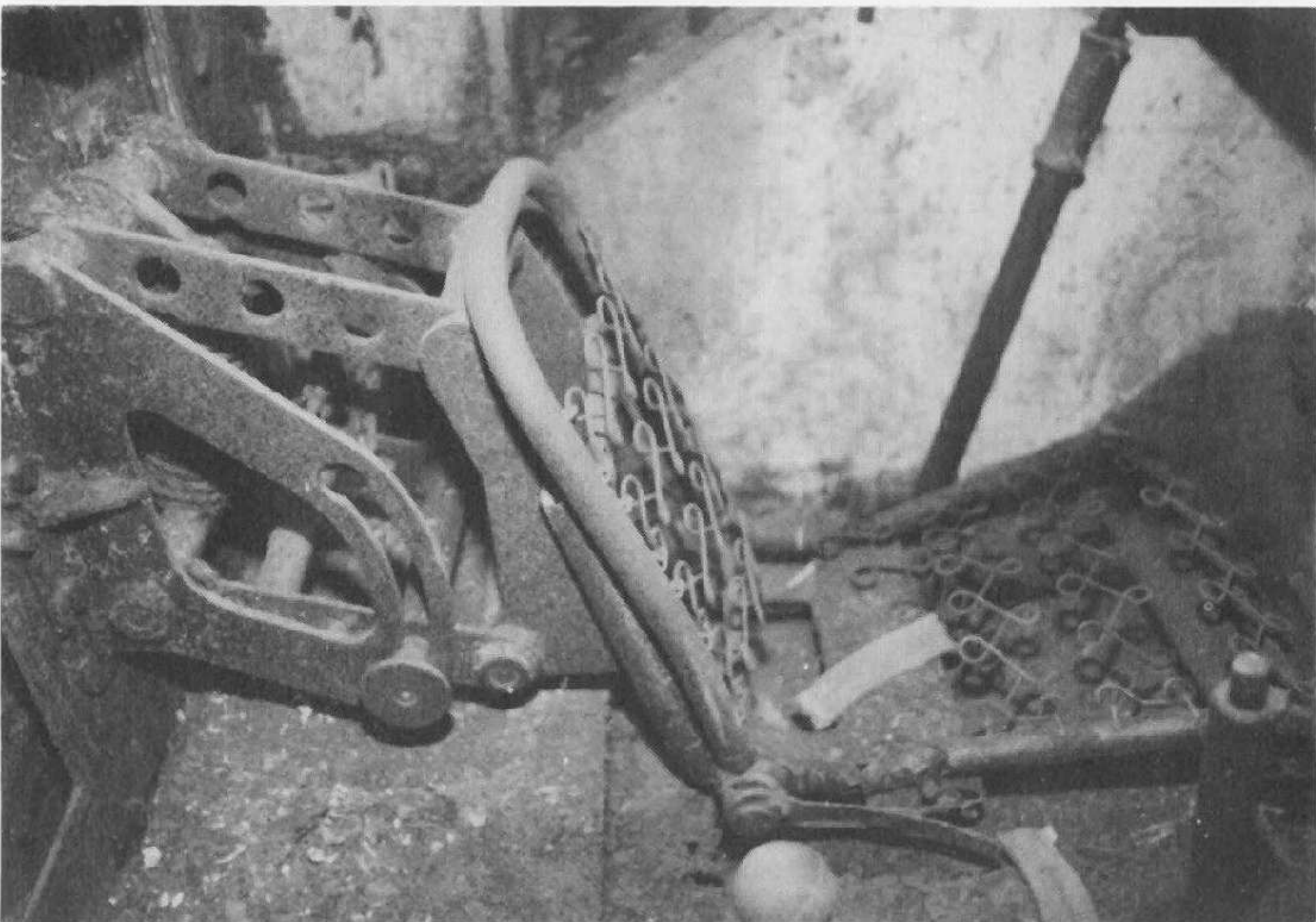
A close look at the operating mechanisms for raising and lowering the crew seat. Although the bow machine gunner's seat is missing I would assume that they would be similar.
