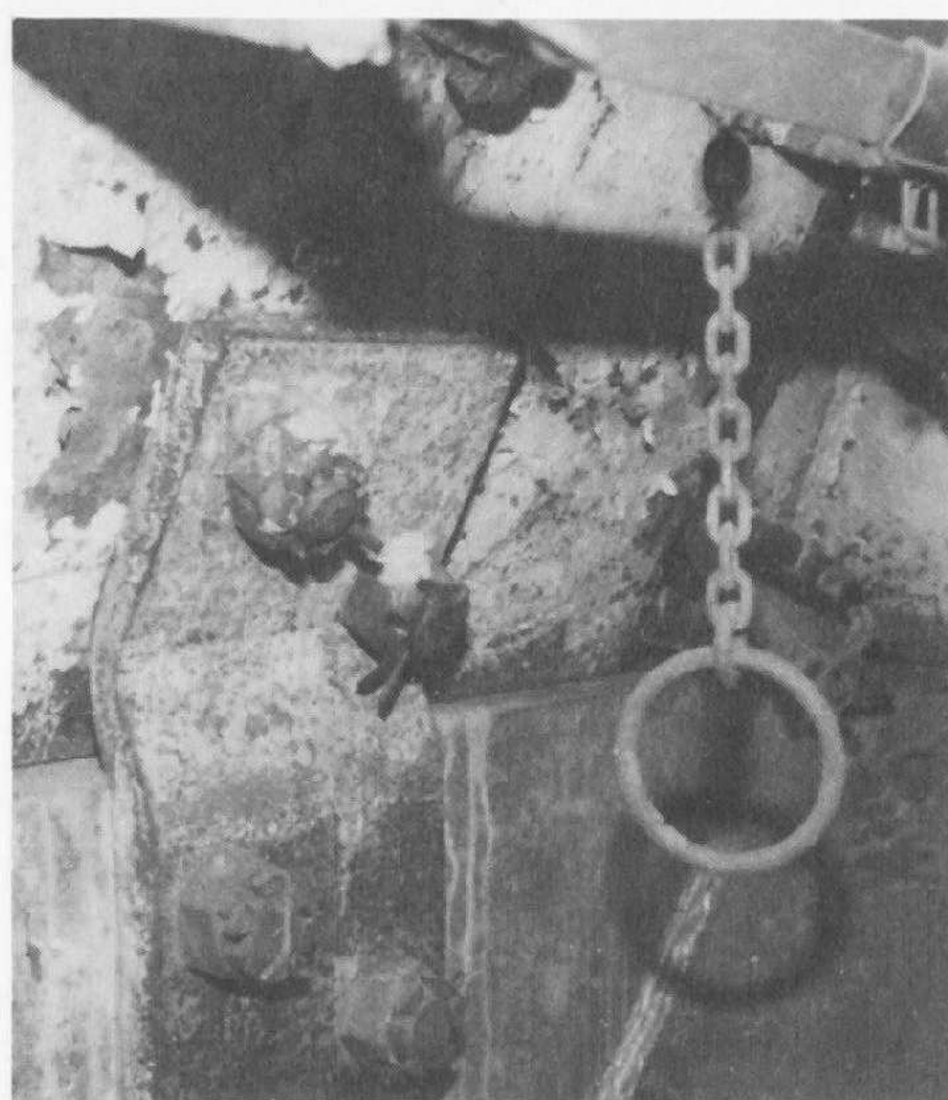
The connecting plate and backside of the conical bolts that hold the fighting compartment to the hull. Each bolt is also secured with a cotter pin.
