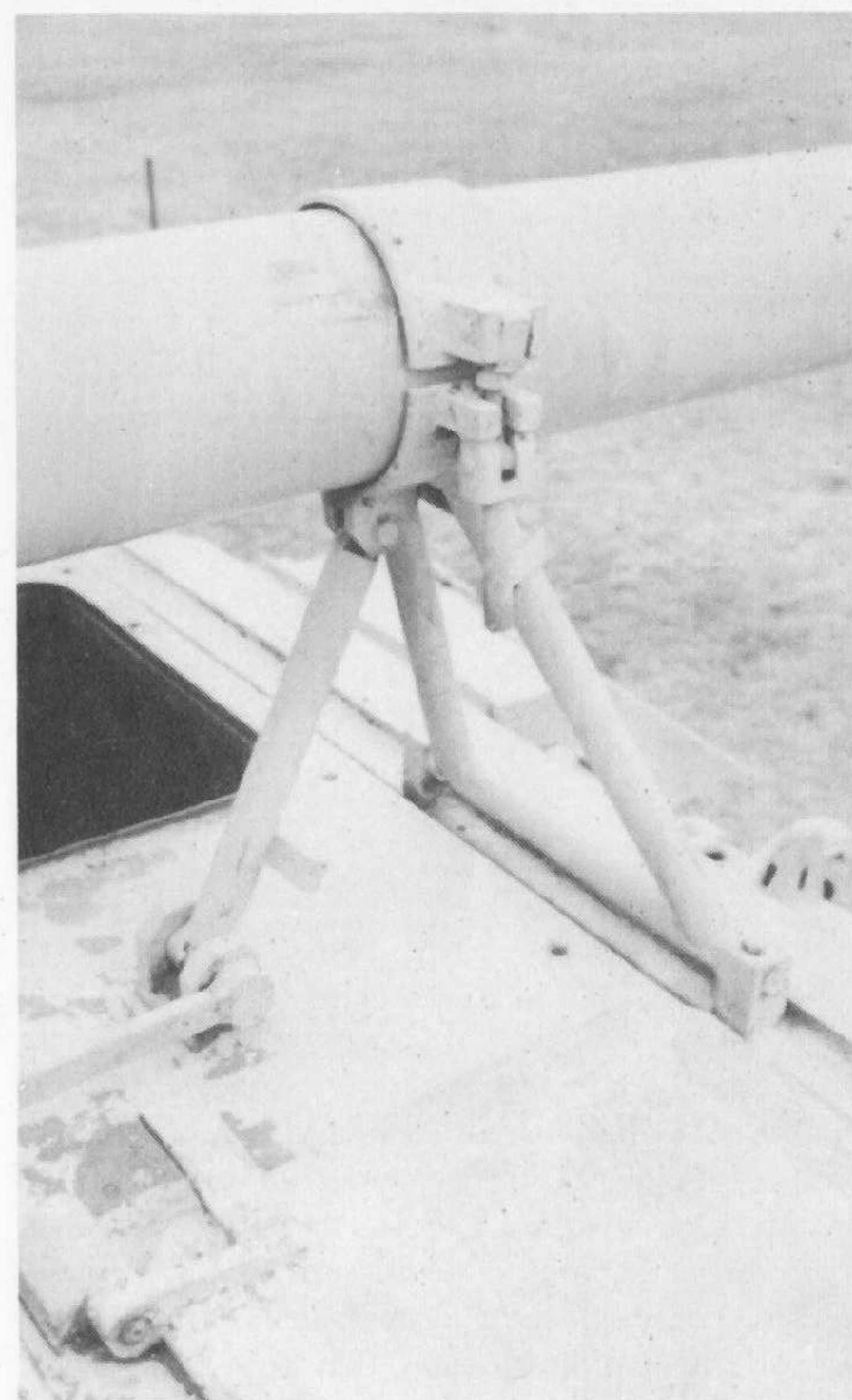
The gun travel lock. There is a nut in the gap between to the two halves that is tighten or loosen as the case may be.
