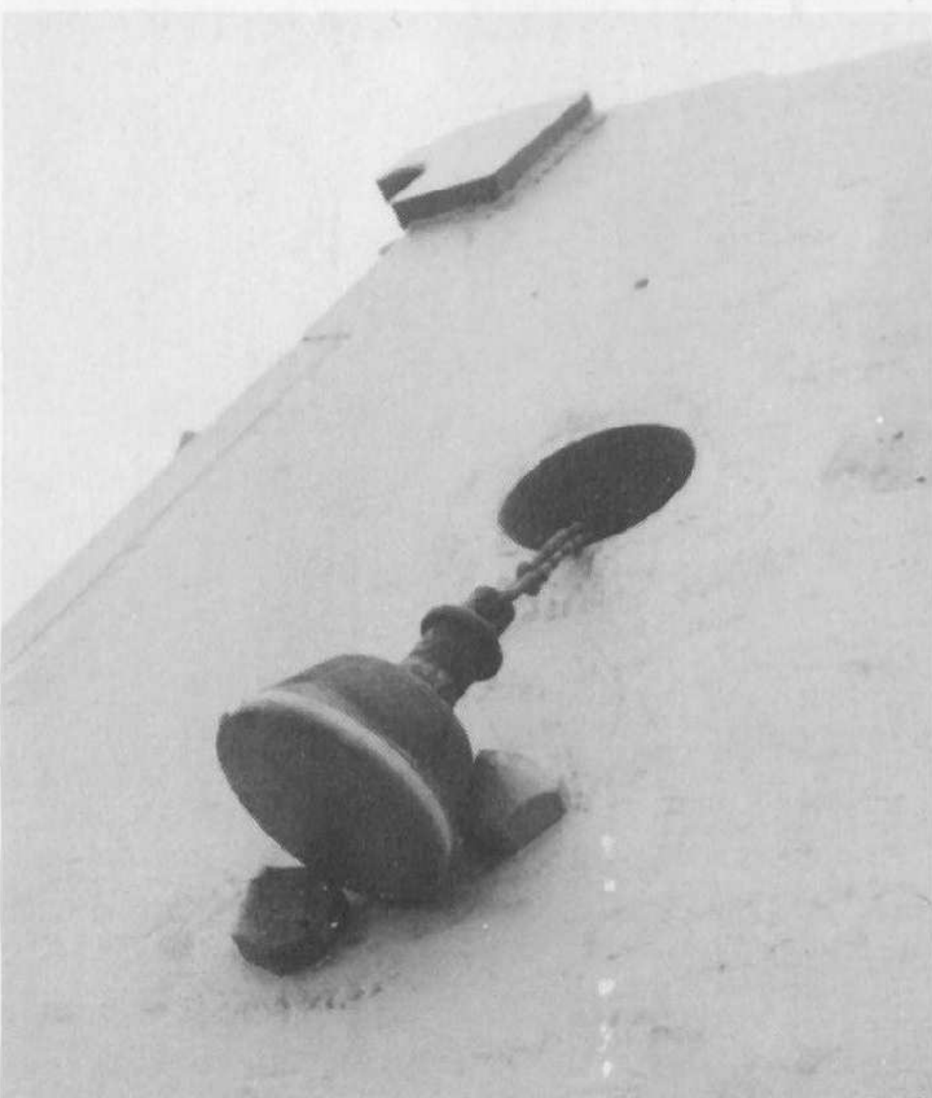
The right side pistol port has been punched out and allowed to hang at the full extension of the retrieval chain. Note the cone-shape to the pistol and the corresponding shape in the hull plate. This photo also clearly shows the rough cut to the interlocking plates. After testing in the US and years of being stored outside, little is left of the zimmerit that covered the Elephant at the time of its capture.
