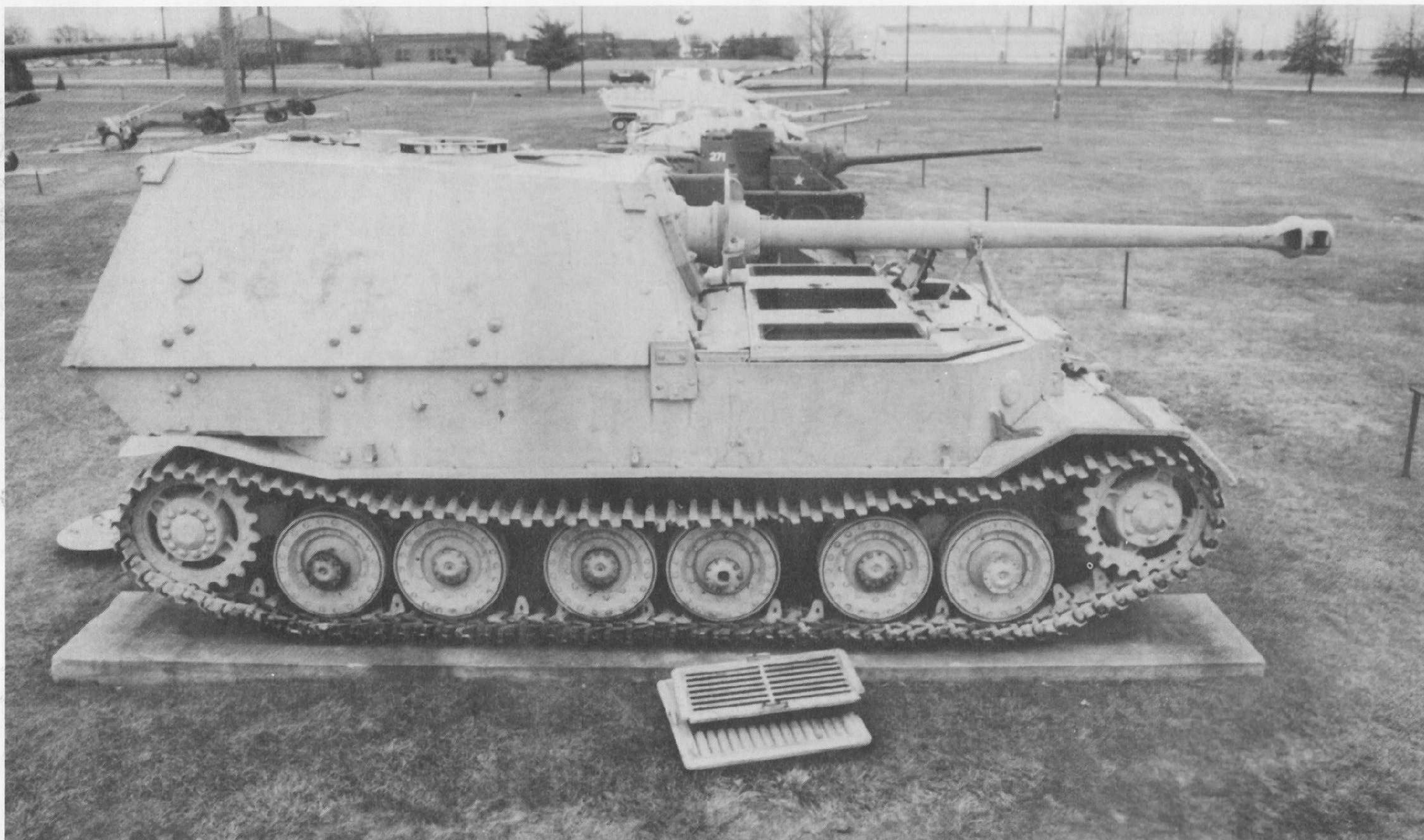
As in the photo above, the radiator air intake grill has been removed. On the ground underneath is the main engine access panel. These grillworks are enormously heavy and once felt can lend new appreciation to the difficulties of working on these vehicles, especially if you factor in combat and inclement weather.
