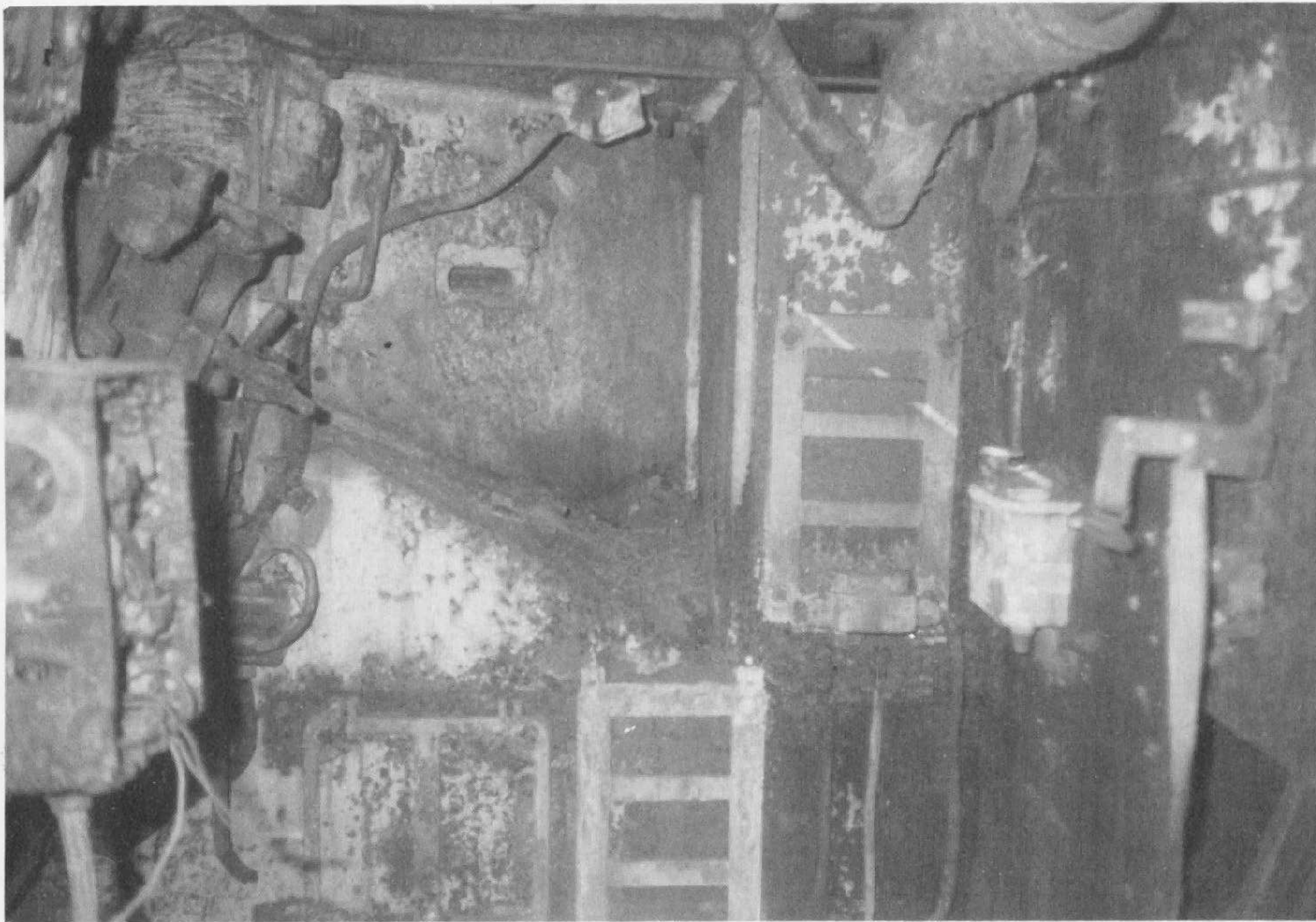
From the driver's position looking across at the bow machine gunner's area. Of note is the large spring and hatch arm in the upper right, the side vision slit near the center and the radio racks. You can also see the radio lead cable snaking up to the roof along the side wall.
