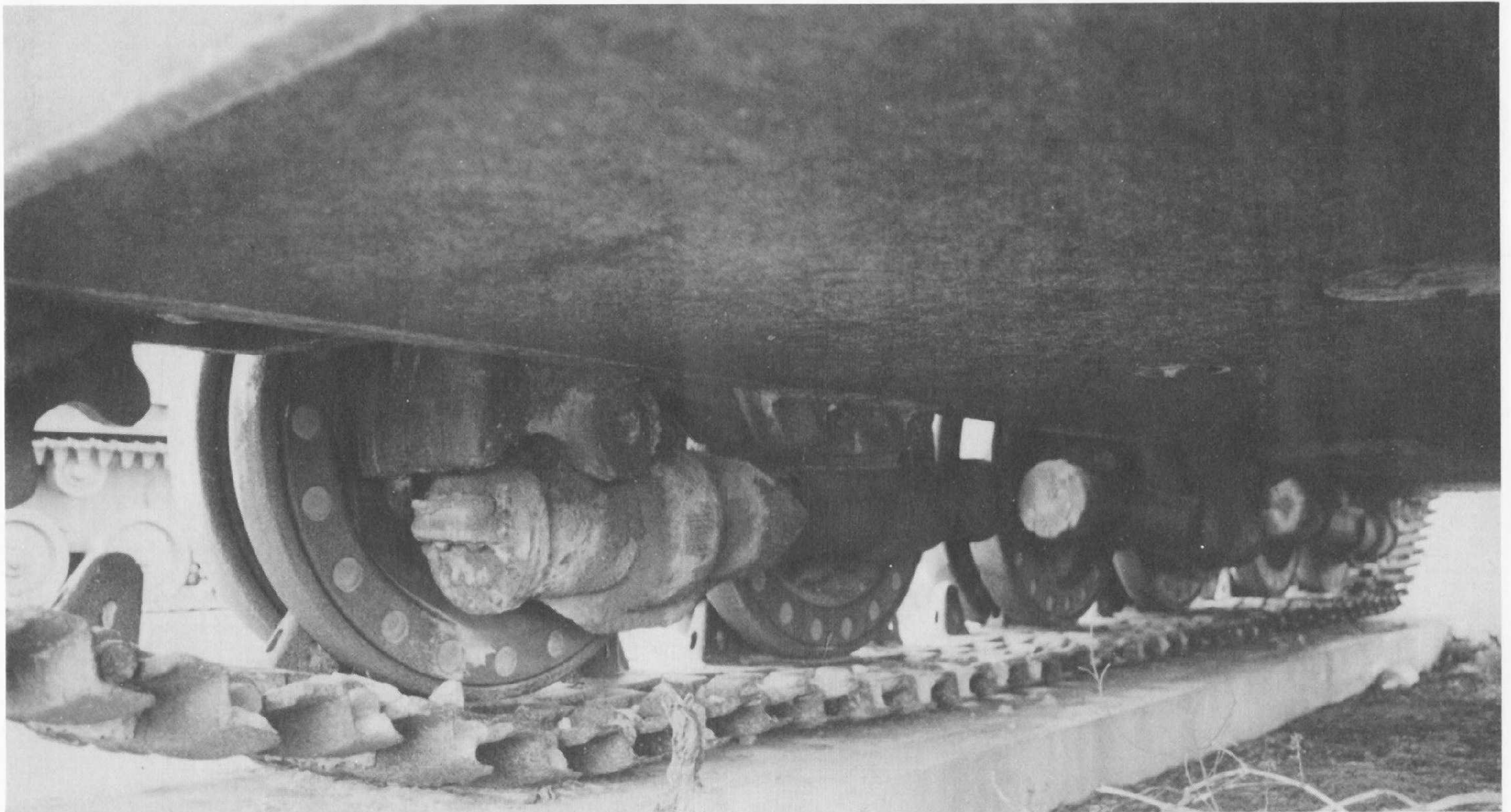
All six bogie assemblies are similar in principle, however, the rear assemblies on both sides are reversed. This can be seen in the photo. Despite their similarities, the assemblies are not interchangeable. For example a rear assembly cannot be mounted in either the center or forward positions, nor can an assembly be interchanged with its corresponding assembly on the opposite side.
