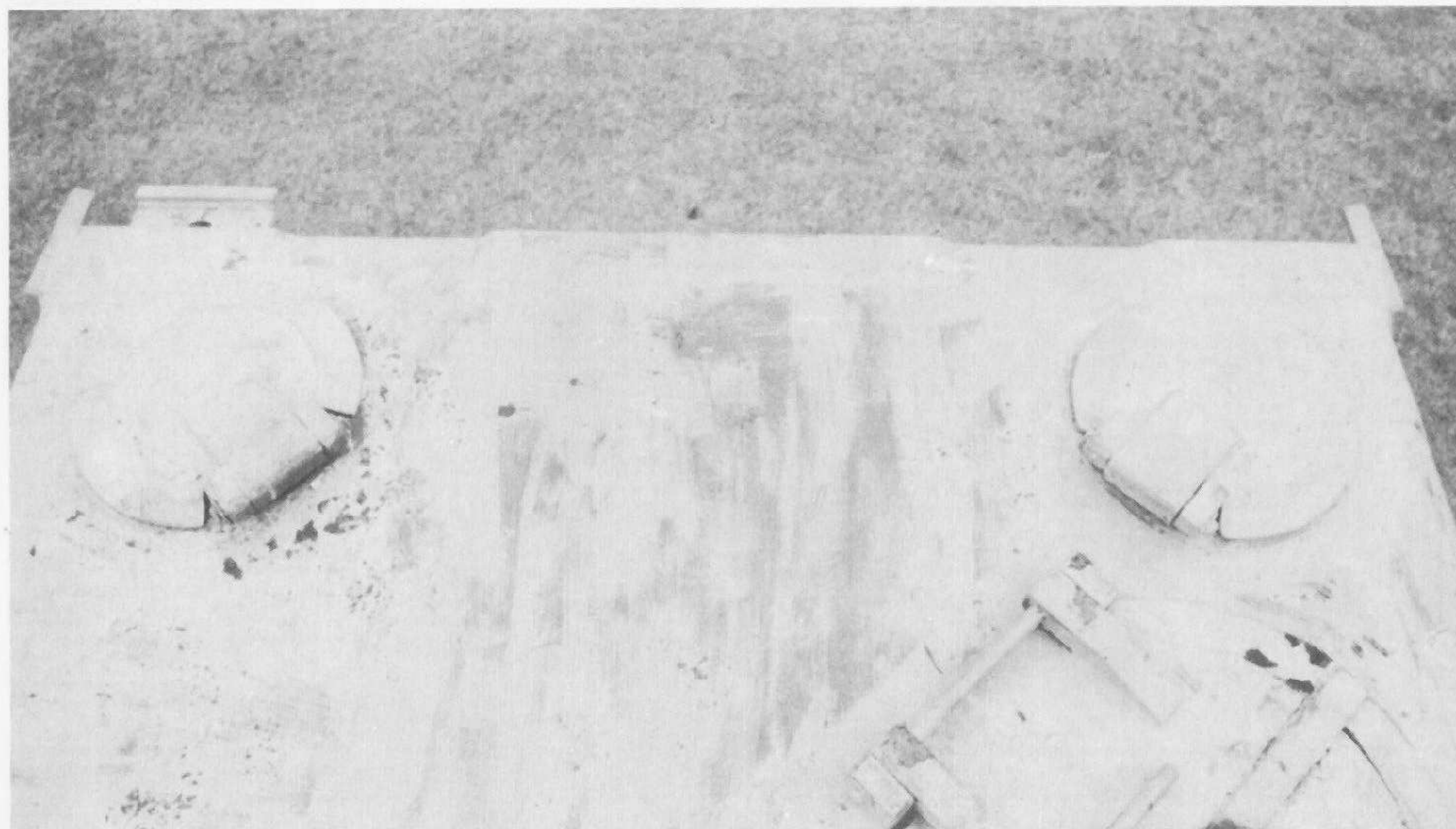
Small periscope ports for the loader's use, both identical and located in the back corners on top of the fighting compartment.
