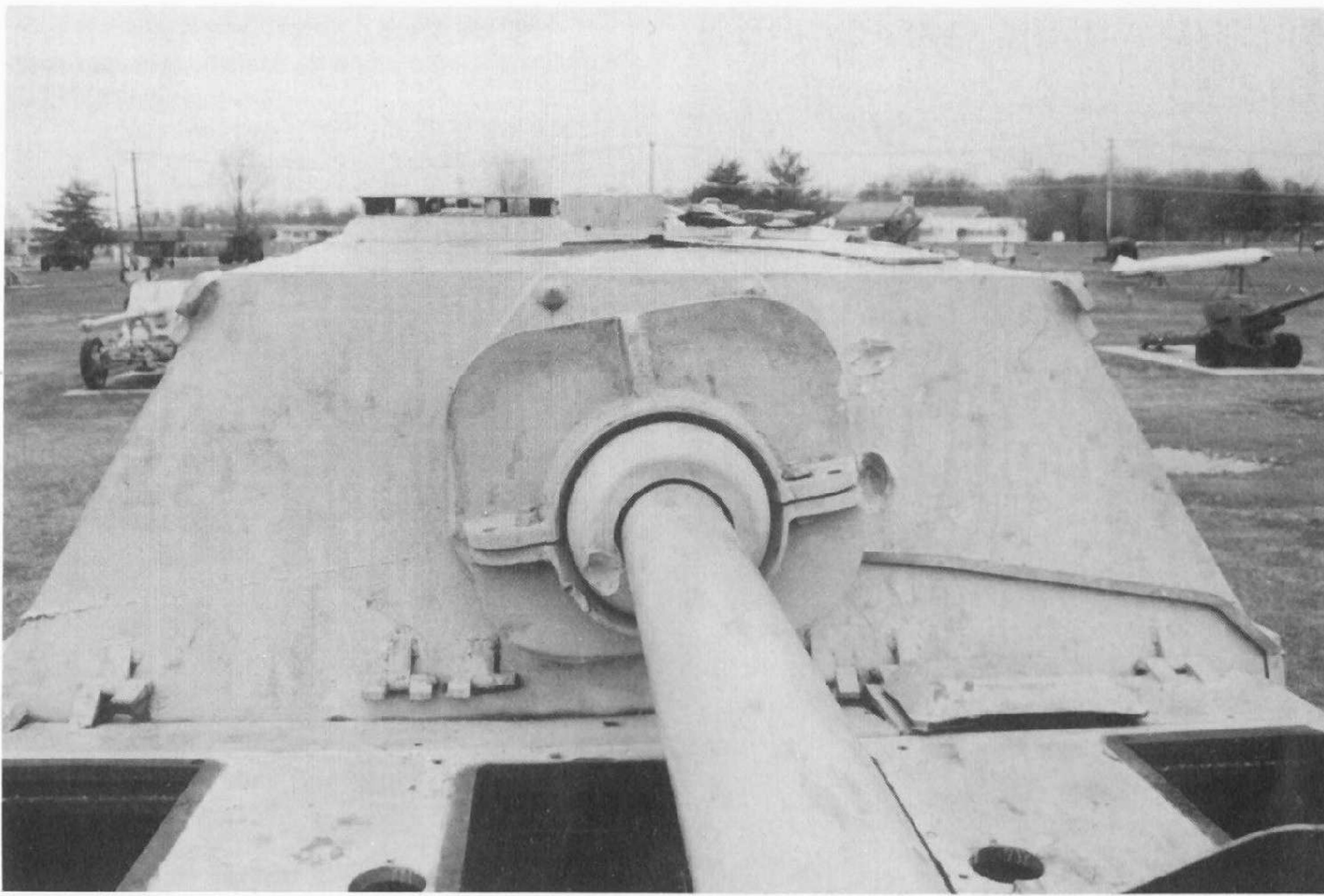
Aberdeen's Elephant came in with a small amount of shell damage, including the frontal shell shots that can be seen on the add-on collar (which is flat on the backside) and the front plate: Perhaps less noticeable at first is the missing rain guard missing from the right side (left in the photo) and the broken welds on the brackets that hold the back plate of the engine deck to the front armor slope. In this photo all but the two brackets on the right are broken. The result has been that the rear engine deck plate has settled down at an angle and rests below where it should be. The plate should be welded to the four brackets that are shown on the front plate, this in turn would bring the plate up level with the rest of the deck.
