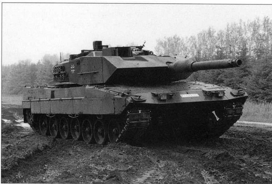
The component trial vehicle, KVT, was taken from the fifth batch (MaK) and used for the improvement programme. The KVT was later converted to the instrument trial vehicle, IVT, seen here in 1991. (Krauss-Maffei-Werkfoto)
