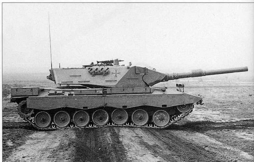
Seen here is Prototype 14 with one of the seven prototype turrets, presumably turret 17, equipped with the Rheinmetall 120 mm smooth bore main gun, during tests at Kampftruppenschule 2 (German Armour School) in Münster in 1974. (FMZ/Panzertruppenschule)
