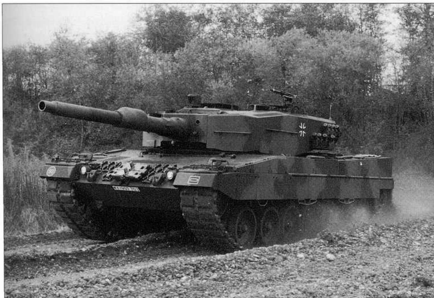
The eighth batch introduced new rear sections for the side skirts and slightly reshaped mounts for the smoke mortars. The collimator of the muzzle reference system is not yet fitted. (Krauss-Maffei-Werkfoto)
