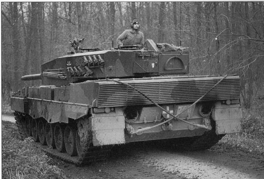
This view of a Leopard 2 A4 (second batch) of PzBtl. 23 in 1987 shows the old-style engine grilles still in use. (Uwe Schnellbacher)
