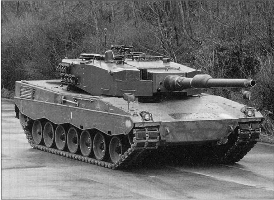
The Leopard 2 AV PT 19 underwent comparative trials against the XM1 prototypes of Chrysler and General Motors in the USA. Its armament was changed from the 105 mm to the Rheinmetall 120 mm smooth bore gun while still in the USA after these tests. The Leopard 2 AV is seen here after its return to Germany. (Krauss-Maffei-Werkfoto)
