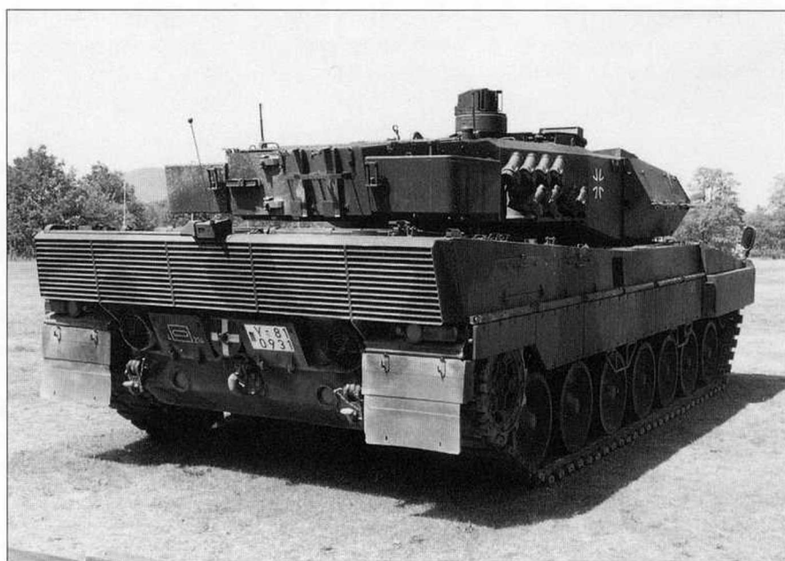
This view of the same PzBtl. 214 tank shows the racks on the turret rear for chocks and spare end connectors. The driver's rear-view camera can be seen above the coolant air outlet grille, in an armoured box. An attached sighting device allows the commander to judge the vehicle's rear end when manoeuvring. (Michael Jerchel)
