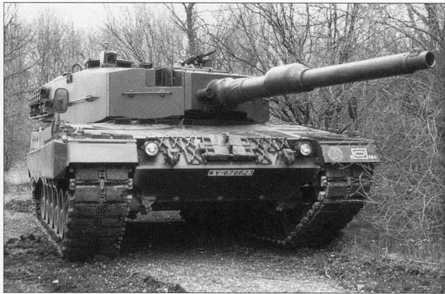
Three pre-series vehicles and two pre-series turrets were delivered in 1978 to the German Armour School in Münster. Shown here is the third pre-series chassis with the second pre-series turret and fake tactical markings. (Krauss-Maffei-Werkfoto)
