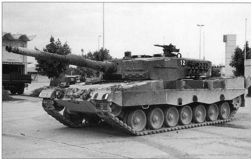
A licence-produced Swiss Panzer 87, with the new side skirt forward sections, standing ready during an exercise at the Swiss Armour School in Thun in 1993. Note also the extra grousers on the left turret front. (Andreas Kirchhoff)
