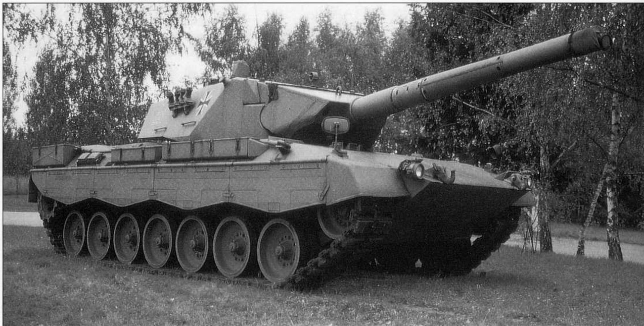
The early prototypes of the Leopard 2 resembled at first glance the Leopard 1 A4. The one shown here is equipped with the Rheinmetall 105 mm smooth bore main gun. (Michael Jerchel)
