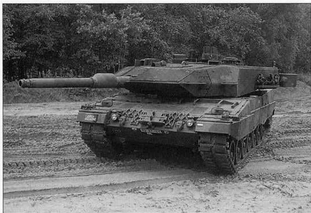
A Leopard 2 A5 NL of 42nd Tank Bataljon, the first unit so equipped, which received its first improved Leopard 2 in May 1997. The Dutch-built smoke mortars are clearly seen on the turret side. (Michael Jerchel)
