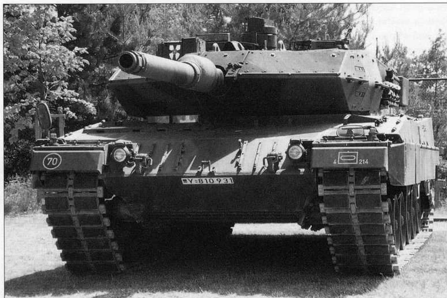
This Krauss-Maffei built Leopard 2 A5 (seventh batch) was converted by MaK in 1996 and serves with PzBtl. 214 in Augustdorf. (Sabine Rotter)
