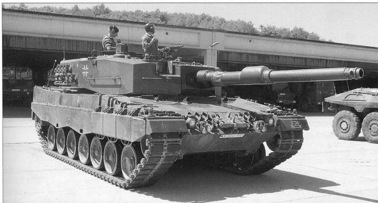
The divisional reconnaissance battalions were also equipped with the Leopard 2 A4. This fifth-batch vehicle of PzAufklBtl. 2 shows the collimator at the right side of the barrel's end, fitted in 1994. (Michael Jerchel)
