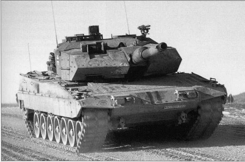
The TVM max. was a converted eighth-batch vehicle and was also known as TVM I. It was later used for comparative trials in Sweden. (Krauss-Maffei-Werkfoto)
