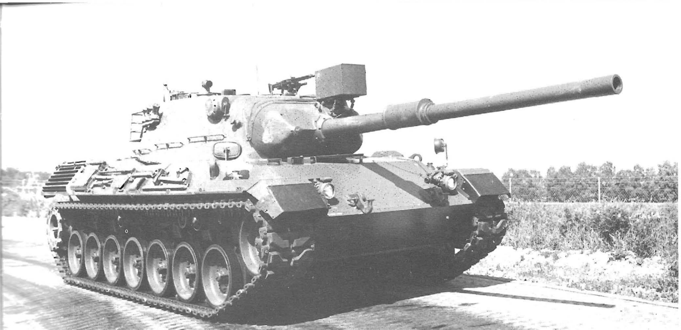
Three views of the Leopard 1A1. Note the eccentric fume extractor on the 105mm gun and the lack of a thermal sleeve for the barrel. Krauss Maffei
