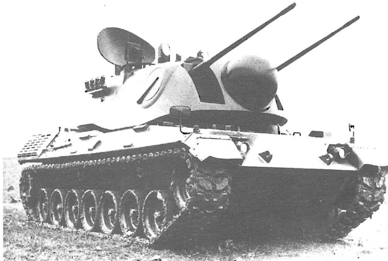
Left: Prototype of the Matador twin 30mm anti-aircraft gun system on the Leopard 1 chassis; this was dropped in favour of the twin 35mm system. Rheinmetall
