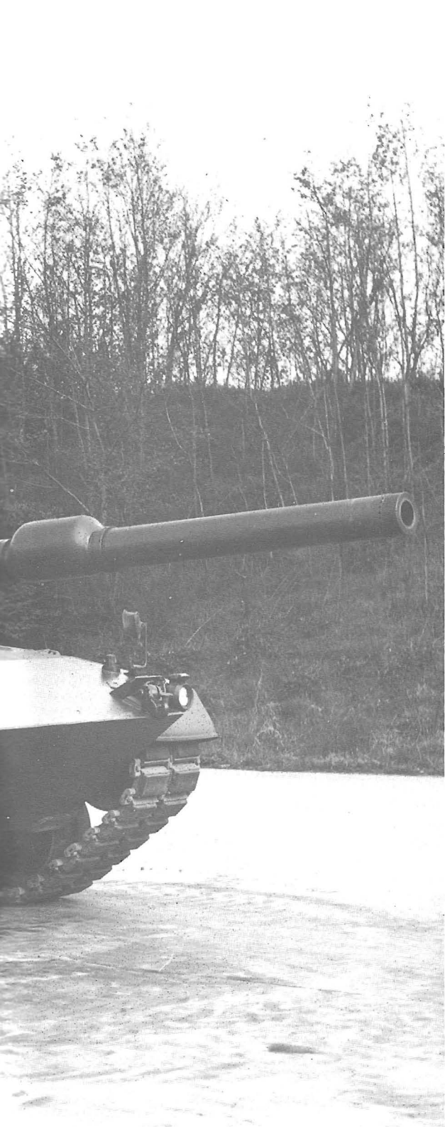
Left: Early Leopard 2 prototype armed with 120mm main gun and Rh202 20mm cannon at commander's station. Krauss Maffei
