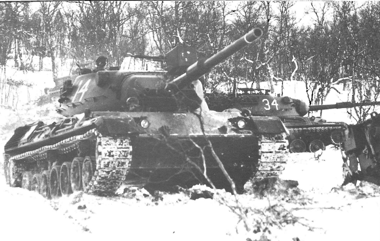
Above left: Leopard 1 of the Belgian Army. Note the commander's FN machine gun in place of the German MG3. The Belgians took 334 Leopard MBTs, a number of which were fitted with the SABCA fire control system. Belgian Army
