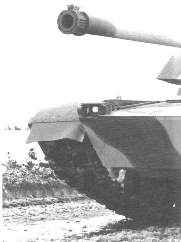
Right: The American Army's next MBT is the XM1 Abrams still under development. Their first MBT not based on the M26 evolutionary chain, the XM1 is armed with a 105mm main gun, has Chobham armour and should prove equal to any MBT of the next generation. Chrysler
