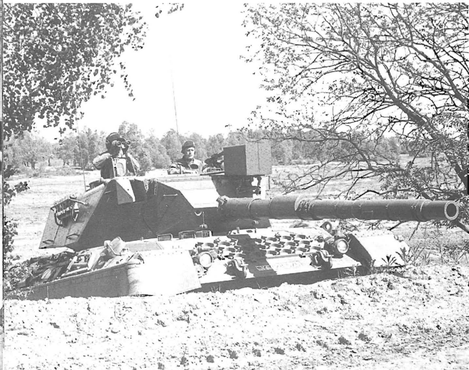
Left: Leopard 1A4 with searchlight attached. Note commander's panoramic telescope, part of the integrated fire control system on this version of Leopard.
