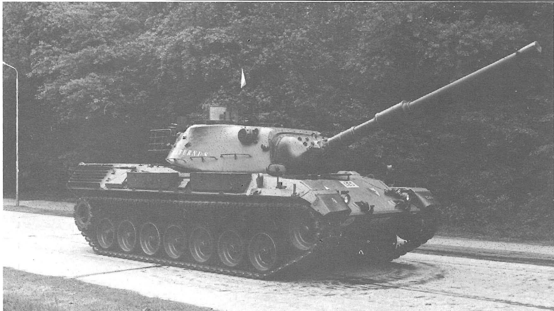
Left: In 1967-68 the Dutch Army tested the Leopard 1 and Chieftain. They eventually ordered 453 Leopards which were delivered 1969-71. This vehicle shows the Dutch stowage box modification on hull sides but has not yet been fitted with smoke dischargers, of which the Dutch have their own variety. Dutch Army
