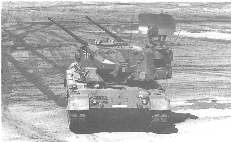
Left: Gepard – 420 are in German Army service. Note surveillance radar erected – when retracted it swings back and down to lie horizontally over the engine decks. BdV
