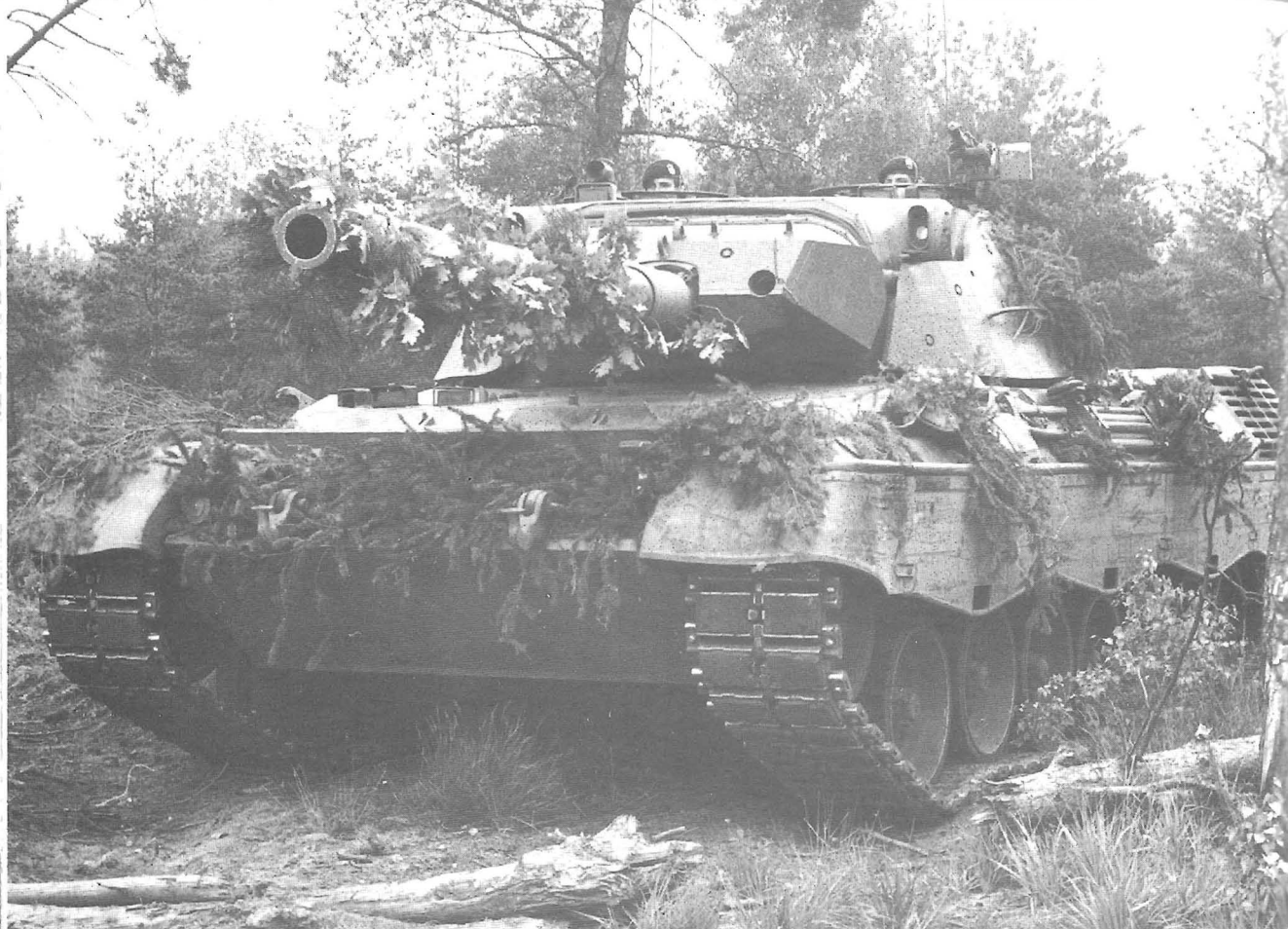
Above and right: Two views of the Leopard 1A1A1 – the updated and uparmoured version of the Leopard 1 and 1A1 – showing clearly the additional mantlet armour and the side and rear turret armour which covers the stowage baskets. Both vehicles have thermal sleeves on their 105mm main guns and early exhaust louvres. Wegmann
