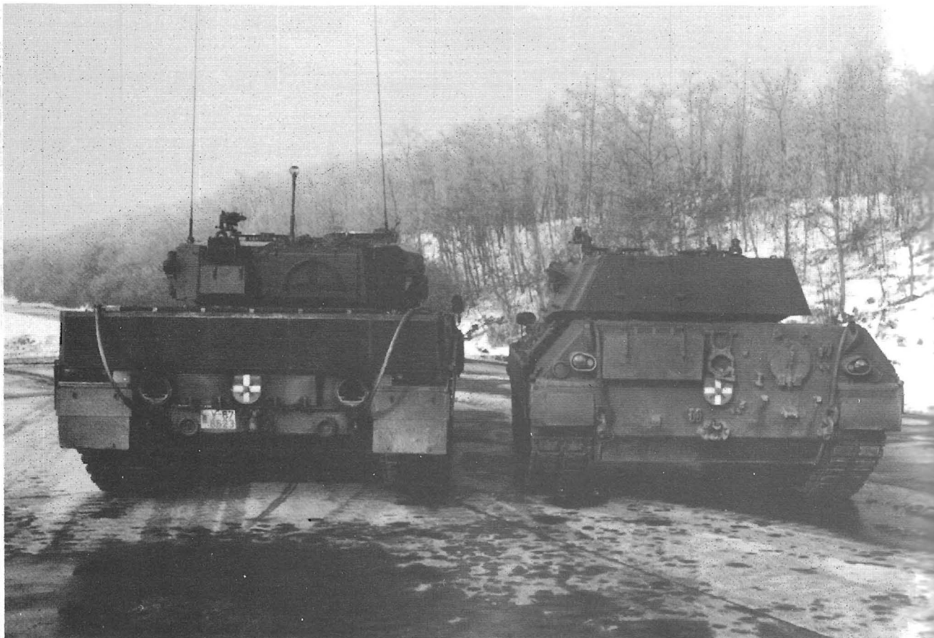
Above: Rear view showing differences between the Leopard 2 (left) and Leopard 1A3. Krauss Maffei
