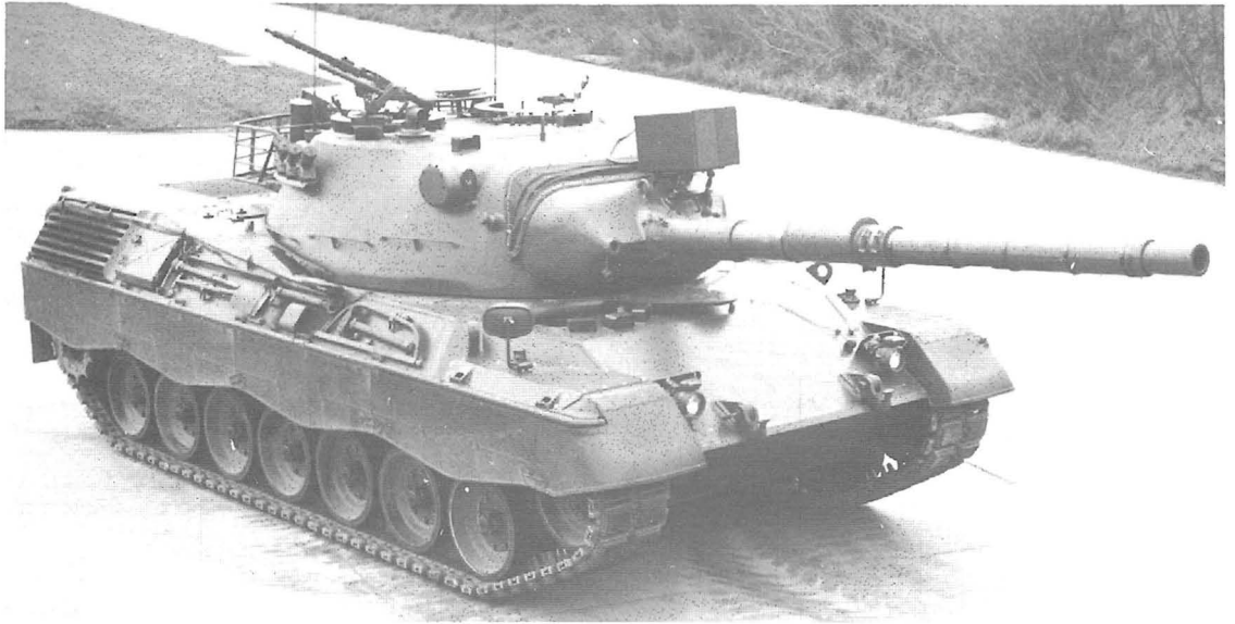
This page and above right: Four views of the Leopard 1A2. All these vehicles have thermal sleeves on their 105mm main guns and rubber side skirts. The vehicle in photograph at left has a wading attachment over the commander's position. Note the differences between the Leopard 1A2's cast turret and the welded turret of the Leopard 1A3 (below right). All Krauss Maffei
