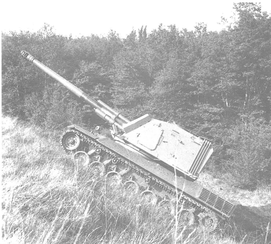
Above and left: A private venture between Krauss Maffei and GIAT of France involved the marrying of a Leopard chassis with a French 155mm GCT turret. (A specification for this project can be found on p110.) Krauss Maffei
