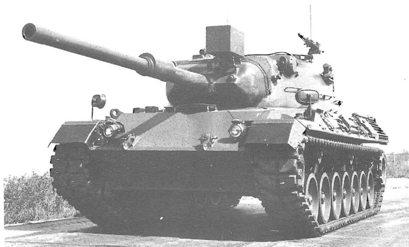
Three views of the Leopard 1A1. Note the eccentric fume extractor on the 105mm gun and the lack of a thermal sleeve for the barrel. Krauss Maffei
