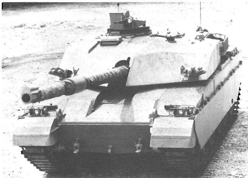
Left: Shir 2 with Chobham armour and 120mm main gun. The Shir will not see service with the British Army although it is the direct link between Chieftain and Challenger, the British next generation MBT.
