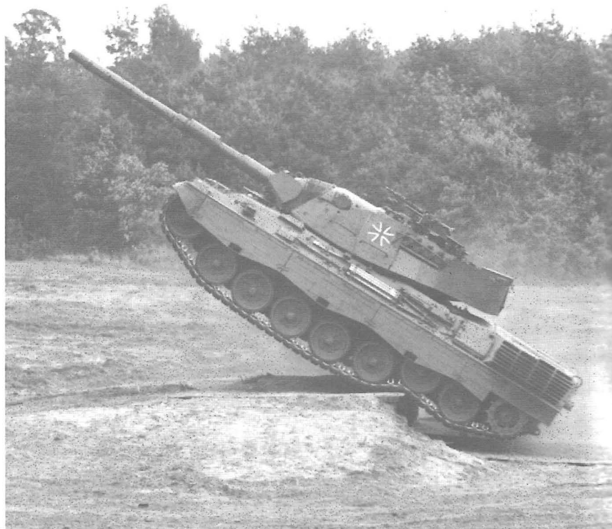
Above and right: Two views of the Leopard 1A1A1 – the updated and uparmoured version of the Leopard 1 and 1A1 – showing clearly the additional mantlet armour and the side and rear turret armour which covers the stowage baskets. Both vehicles have thermal sleeves on their 105mm main guns and early exhaust louvres. Wegmann
