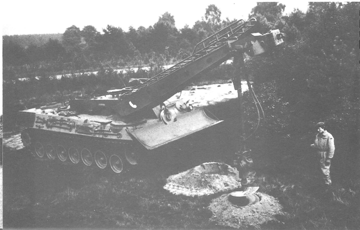
Below right: Leopard Pioneerpanzer using its dozer blade. Krupp MaK
