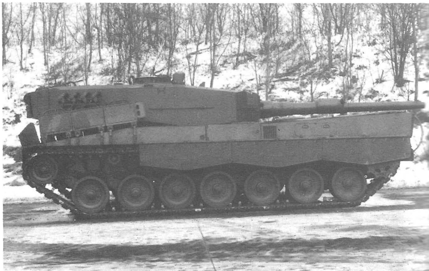
Right: Leopard 2 with turret to rear and front skirt plates raised. Krauss Maffei
