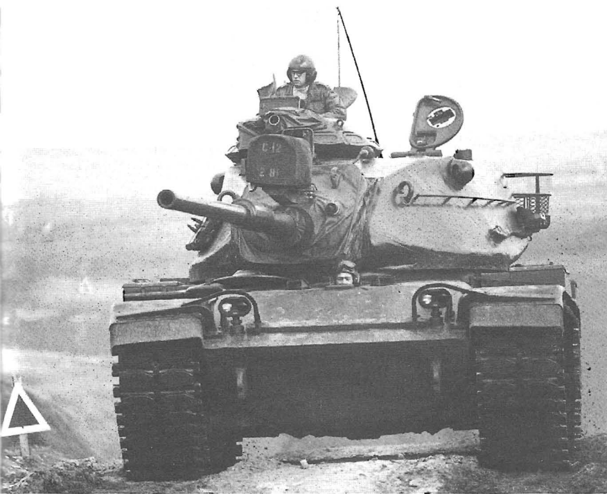
M60A1 – the current American MBT – evolved from a 1944 design, the M26 Pershing, via the M46, M47 and M48. While it has all the conventional modern 'add-on' aids – laser rangefinder, stabilisation, electronic fire control system – it is nevertheless an improvement of an old design, sound rather than spectacular. It is armed with the British 105mm main gun. The photograph shows an M60A1 in Germany. US Army
