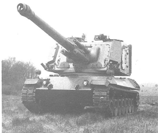
Above and left: A private venture between Krauss Maffei and GIAT of France involved the marrying of a Leopard chassis with a French 155mm GCT turret. (A specification for this project can be found on p110.) Krauss Maffei
