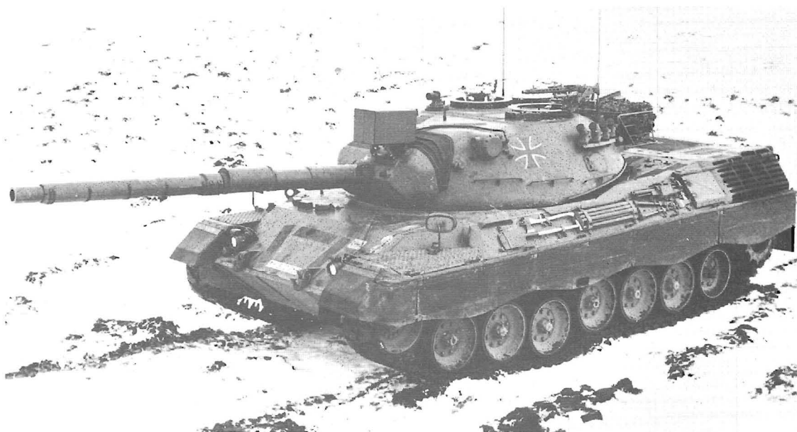
Below: Leopard 1A2 – note the thermal sleeve on 105mm main gun and side skirts. RAC Centre
