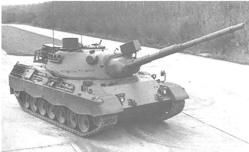
This page and above right: Four views of the Leopard 1A2. All these vehicles have thermal sleeves on their 105mm main guns and rubber side skirts. The vehicle in photograph at left has a wading attachment over the commander's position. Note the differences between the Leopard 1A2's cast turret and the welded turret of the Leopard 1A3 (below right). All Krauss Maffei
