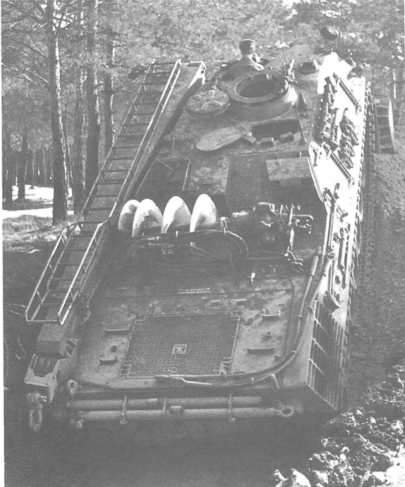
Left: AEV showing clearly the stowage of the auger in place of the spare powerpack which can be carried by the ARV. Krauss Maffei
