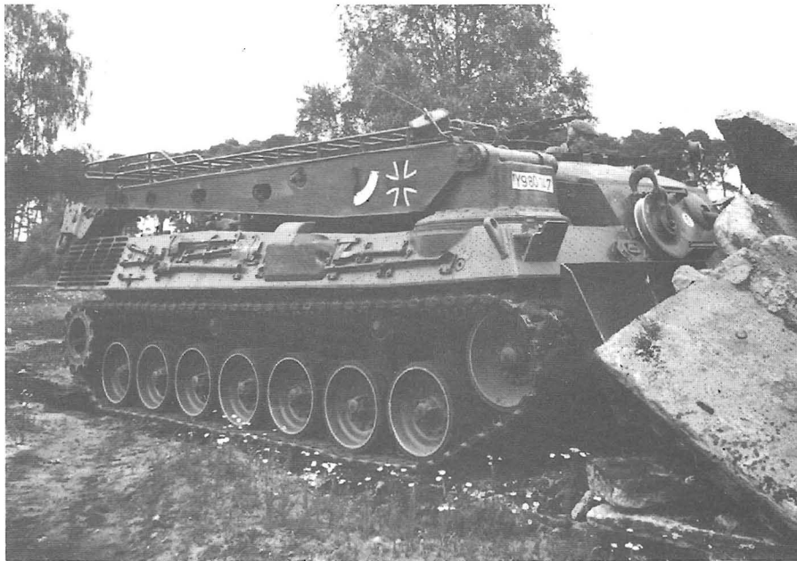
Right: Pioneerpanzer (AEV) using its bulldozer. Note driver's position and hull side detail differences from the Bergepanzer (ARV) – the ladder on the jib-boom (although this is occasionally removed), auger just visible behind the boom on the rear decks and the modified cover on the middle of the hull. Krupp MaK
