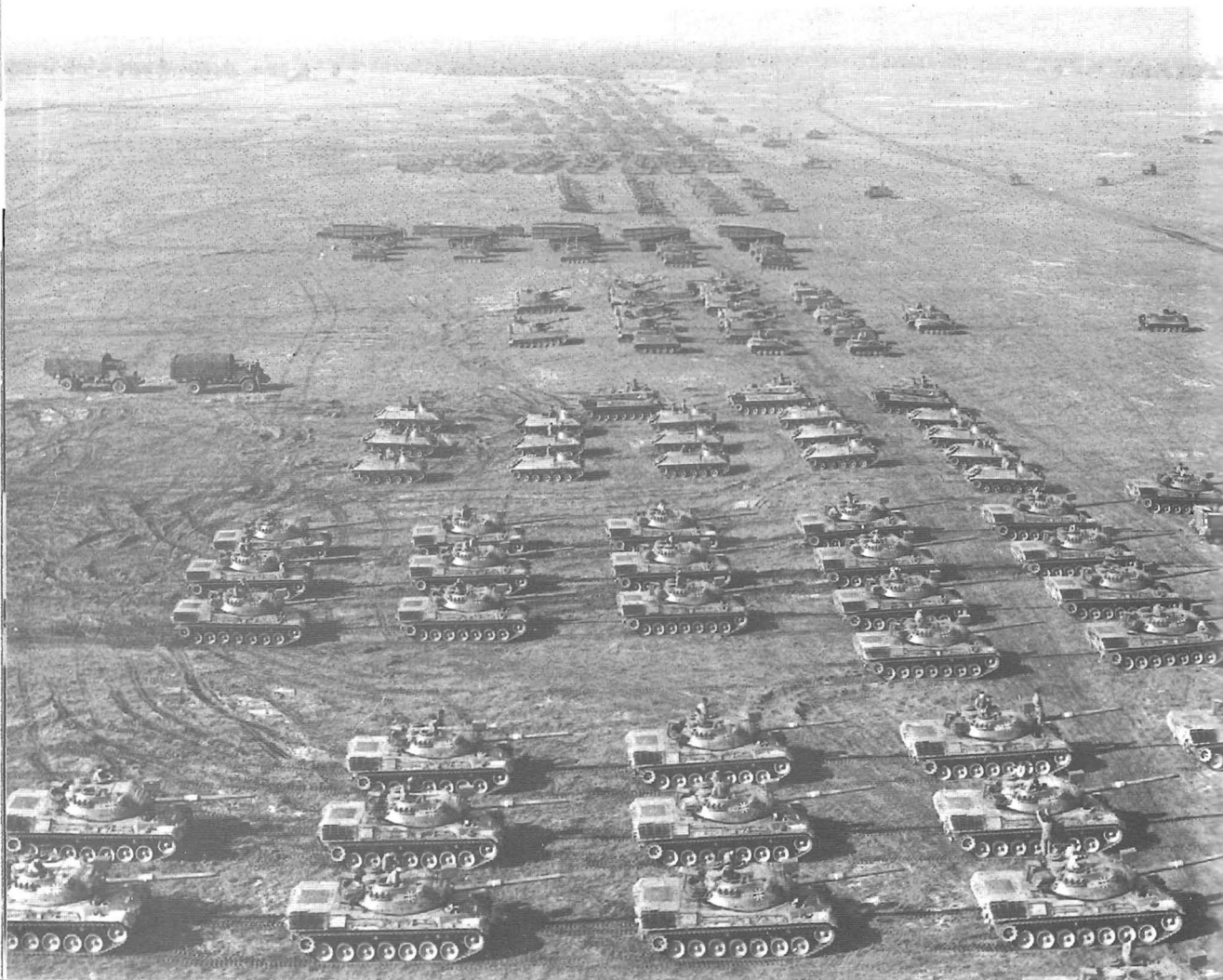
Below: End of Exercise 'Fore Front' in 1971. Nearest to the camera are early production Leopard 1s (note verticals on exhaust louvres) with later versions in middle distance. Also on parade are SPZ 12-3 APCs, Leopard ARVs, M113s, M109s, M48 AVLBs, while in the far distance are Chieftains.
