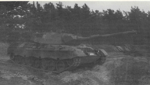
LEOPARD 1 A5 Battle Tank, the newest, enhanced fighting-value version of the LEOPARD 1 for the German army. These vehicles are externally recognizable by the box-shaped periscope exit of the main aiming telescope with heat-sensitive observation device on the turret roof and the panoramic aiming telescope extending out above it. (Kraus-Maffei)
