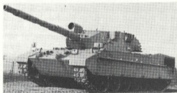
Export tank of the Italian armament industry, OF 40 Mark 2 of the OTO Melara firm. Eighteen OF 40 Mark 1 tanks were built for Dubai and revised to Mark 2 status (fire-control computer), another eighteen Mark 2 tanks were delivered new from the factory. (Soldat und Technik)
