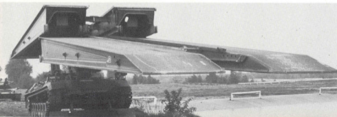
To extend the potential use of the BIBER for surmounting wider obstacles, a quick bridge on supports (SAS) was developed.
