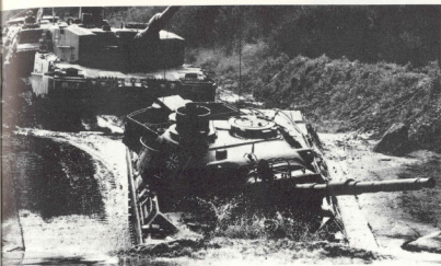
Fighting vehicles crossing a water obstacle. Front: LEOPARD 1 A1A2 with adapted additional armor and deep-fording shaft on the commander's cupola; in the middle, LEOPARD 2 A1; behind it the amphibious FUCHS Transport Tank. (Soldat und Technik)
