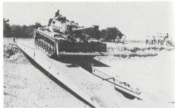
An M48 A2 battle tank with plow blade, formerly in army use, crossed a bridge laid by a BIBER.
