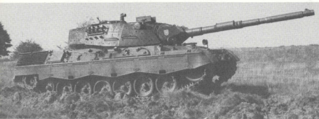
LEOPARD 1 A5, still during testing; the superfluous observation bulges of the three-dimensional range finder have not yet been removed. From this perspective the higher-mounted panoramic periscope can be seen clearly. (Soldat und Technik).
