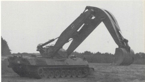
Above: One forerunner of the Engineer Tank 2, made by the MaK firm, with cantilever-arm excavator. Under the concept of "Armored Engineer Machine" (GPM), a universal vehicle to handle the whole scope of engineering tasks on land and in the water under the protection of armor and ABC fire was to be developed.
