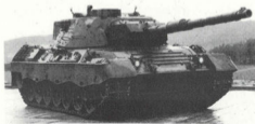
LEOPARD 1 A5 in its final form, without the observation bulges of the formerly used three-dimensional range finder; the field-adjusting system is mounted on the muzzle of the gun. (Soldat und Technik)
