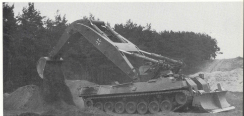
Above: One forerunner of the Engineer Tank 2, made by the MaK firm, with cantilever-arm excavator. Under the concept of "Armored Engineer Machine" (GPM), a universal vehicle to handle the whole scope of engineering tasks on land and in the water under the protection of armor and ABC fire was to be developed.
