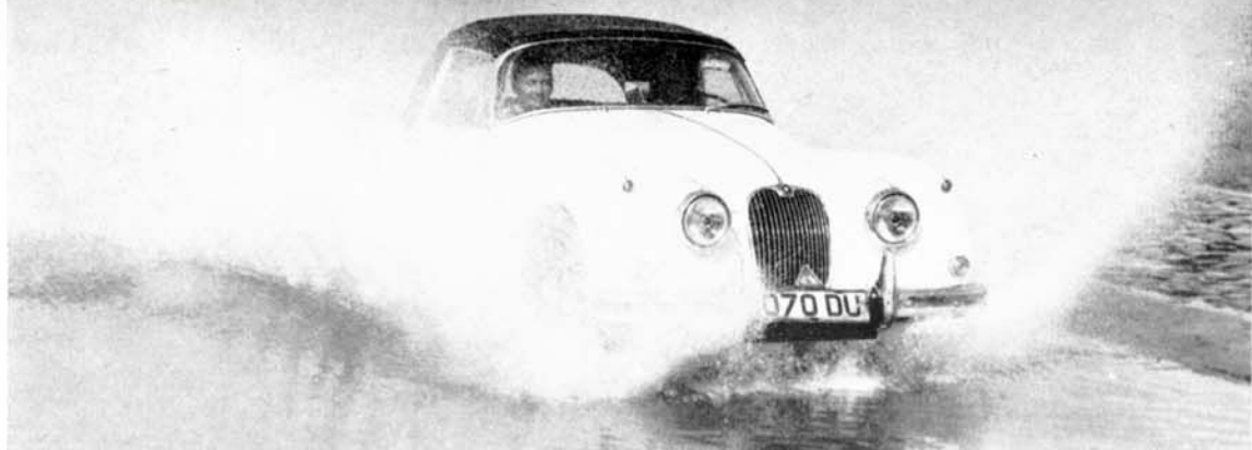
Testing . . . the XK 150 drophead coupé at the Motor Industries Research Association's Nuneaton proving ground during tests of the Dunlop disc brakes introduced on production Jaguars in 1957.
