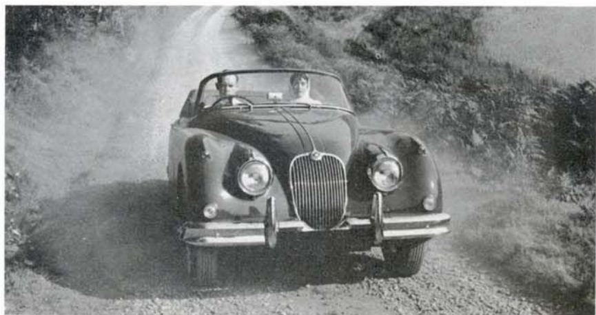
Touring . . . note the XK 150's return to a 'slatted' type grille, as opposed to the XK 140's one-piece grille.
