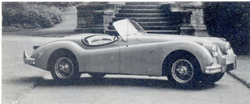
XK 140 in roadster form. On all XKs the rear wheel spat was omitted when wire wheels were fitted. Note the protective bumpers and the one-piece grille.
