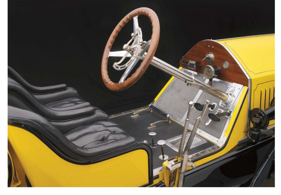
The Bearcat's minimal bodywork, including a simple hood and trim fenders, kept its weight relatively low. It had no doors, no windshield (a monocle windscreen could be fitted to the steering wheel column), no cowl, and no top. A stiff clutch and an intimidating hand-crank starter helped give the Bearcat a reputation as a "real man's" car.
