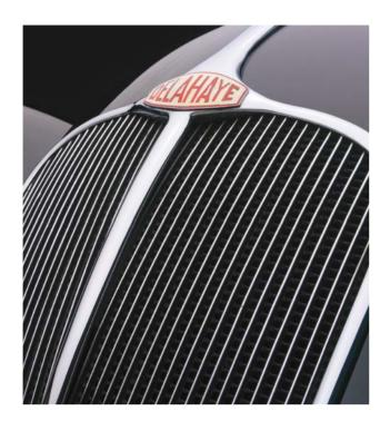
boomerang-shaped curves. The radiator grille is divided by a strip of chrome that runs back to the hood, where it splits into three strips—the two side strips continue along the length of the body, sweeping down the doors and rising dramatically over the rear fenders; the central strip runs straight back along the hood top to the triangular cowl.
