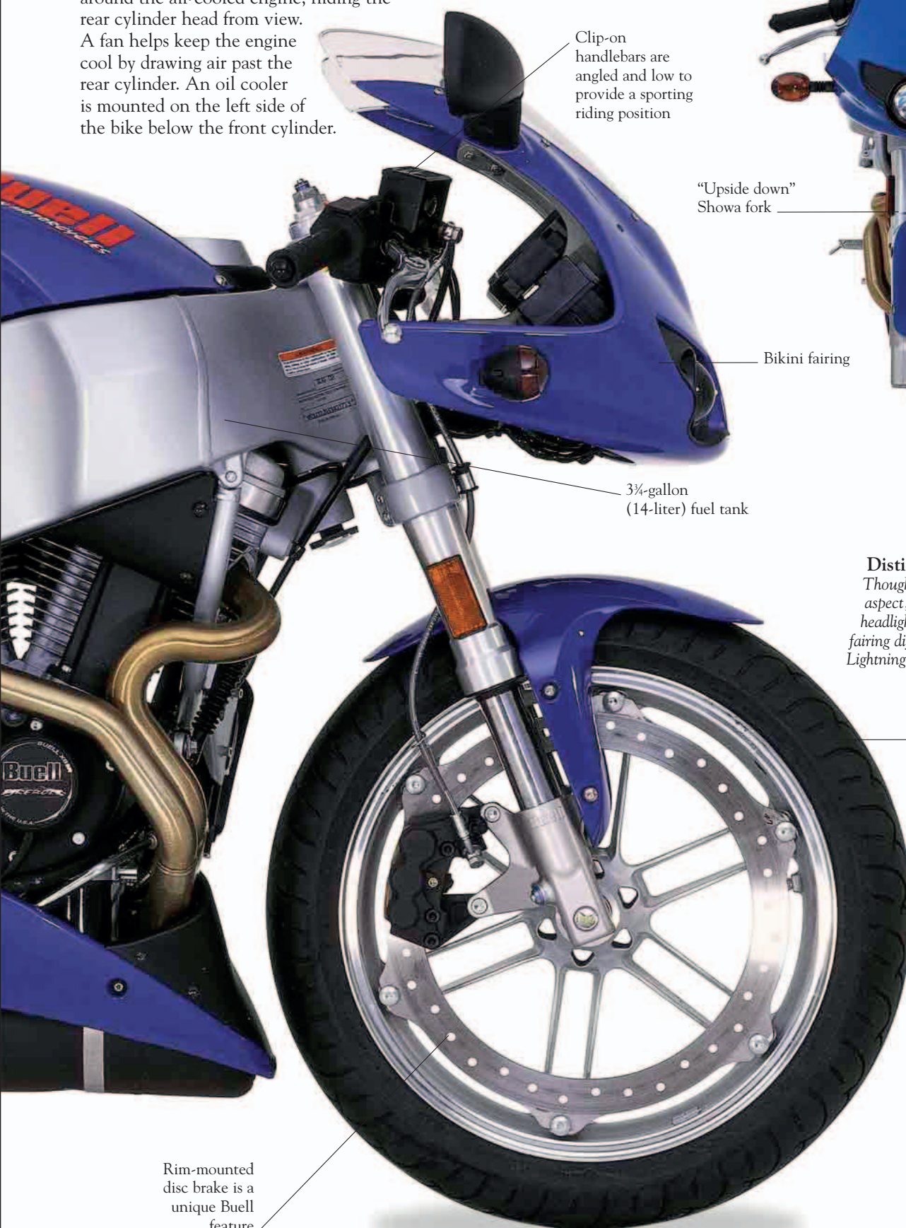
Dunlop tires developed for the bike are a special lightweight construction
