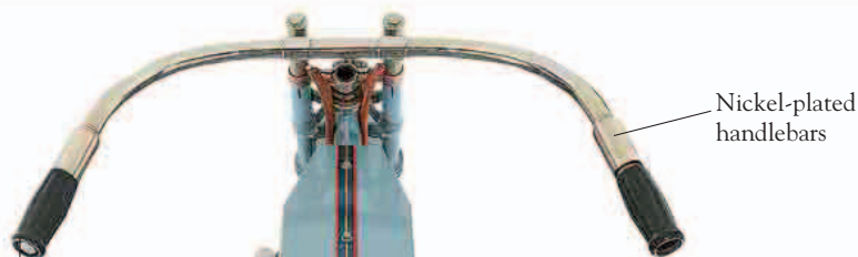
Twist-grip for the ignition advance retard mechanism
