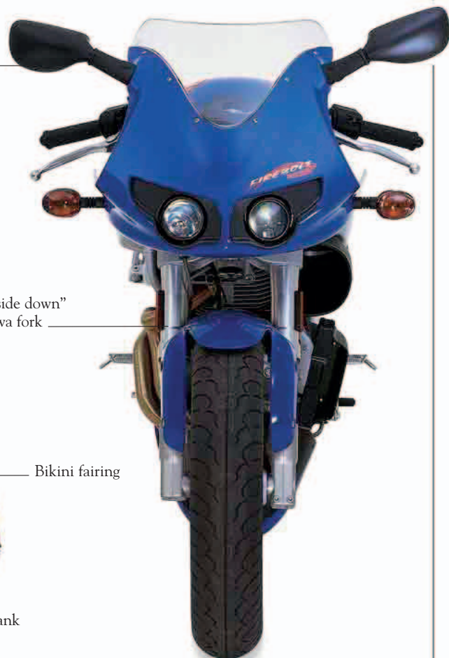
Clip-on handlebars are angled and low to provide a sporting riding position
