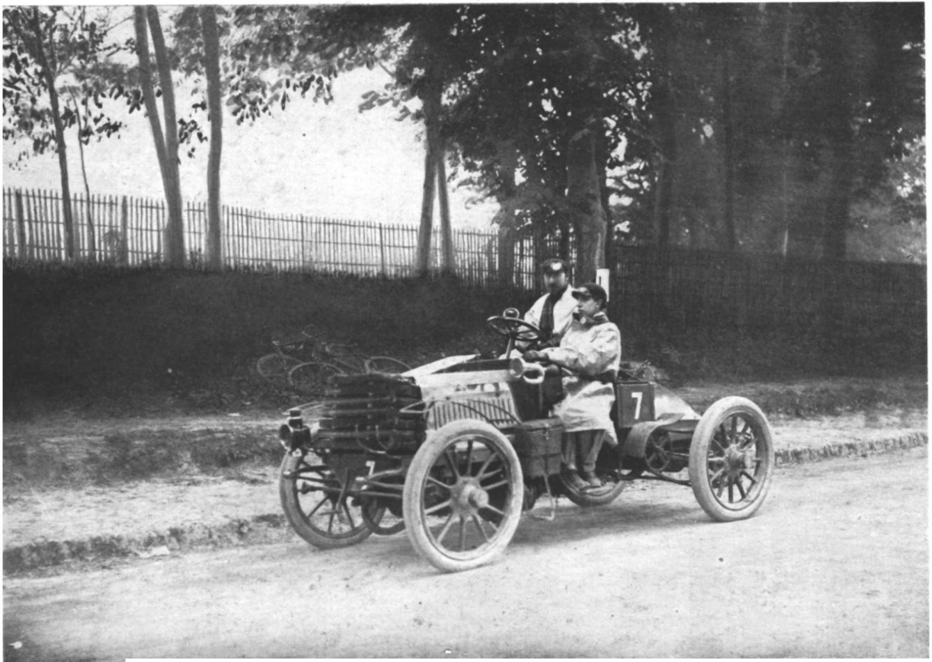
EARLY WINNER-This photograph shows Girardot on his 7.4-litre 40 h.p. Panhard in the 1901 Gordon Bennett race which he won at an average speed of 37 m.p.h. for 372.6 miles.
