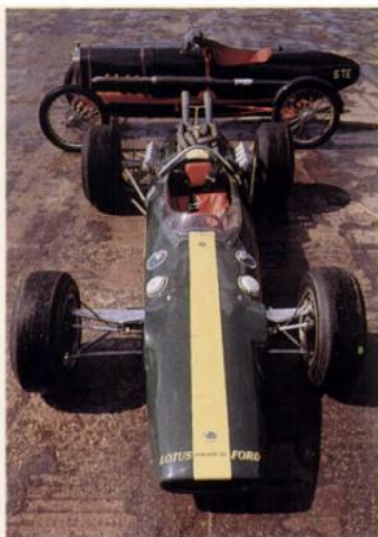
Indy Lotus with offset suspension and veteran Ford racer. Car at rear is 1917 Indianapolis-style Model T racer.
