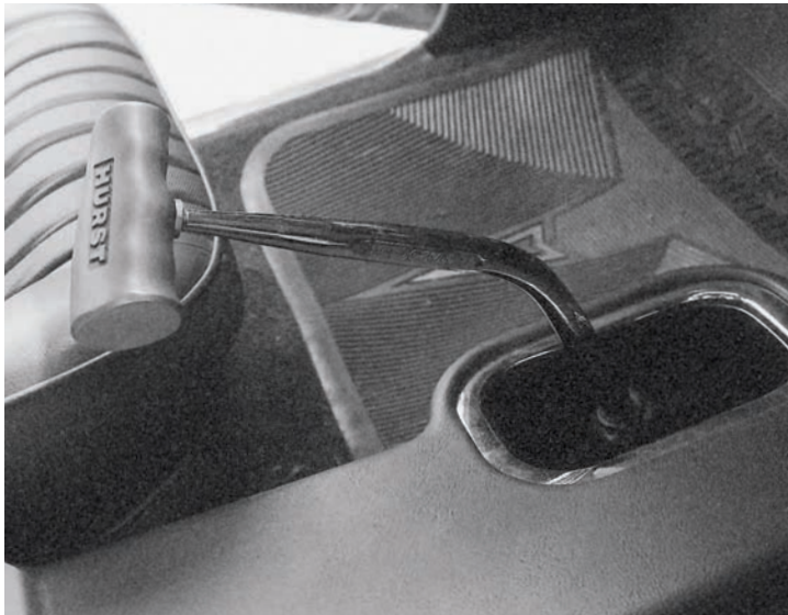
The Hurst shifter made rowing through the giant gears in the transmission a much easier task.
