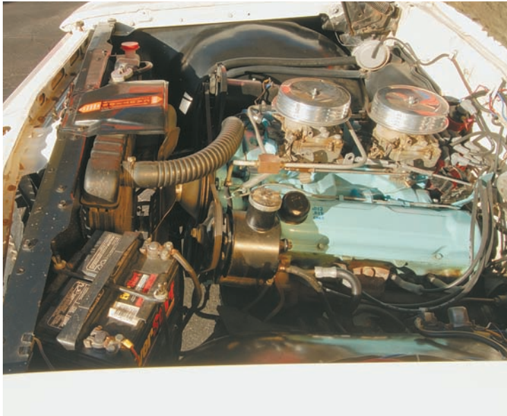
Wangers' race cars used a pair of four-barrel carburetors in place of the three two-barrel setup on the street cars.
