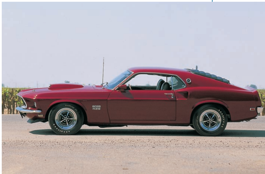
The Boss 429 was really just a vessel in which to homologate the new 429 NASCAR racing engine.
