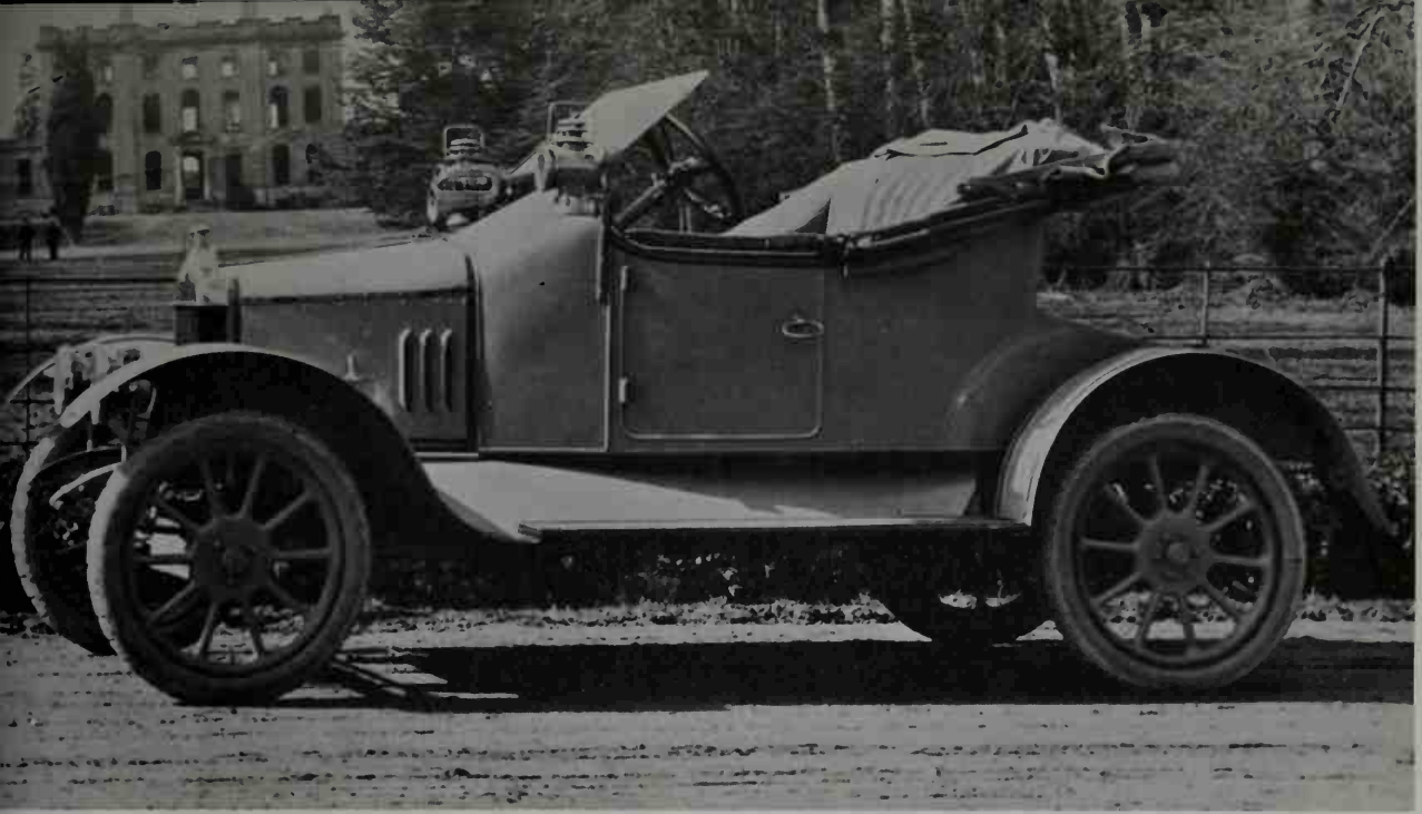
The 4-cylinder (62 x 90 mm.), 9.5-HP "Rhyl" of 1913 was the first light car out of Standard. This 1.1-litre model had worm gear final drive, 90-inch
