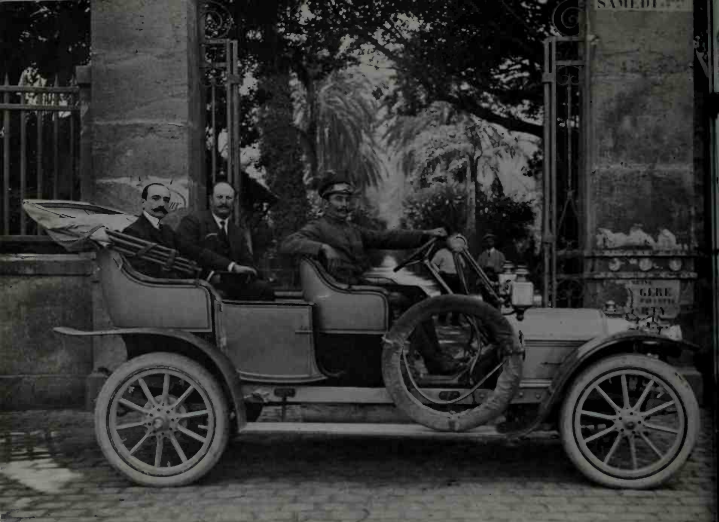
1907 FN Type 2,000 "Super de Luxe" double phaeton used a 4-cylinder engine and shaft drive. An automatic carburetor dispensed with the hand
