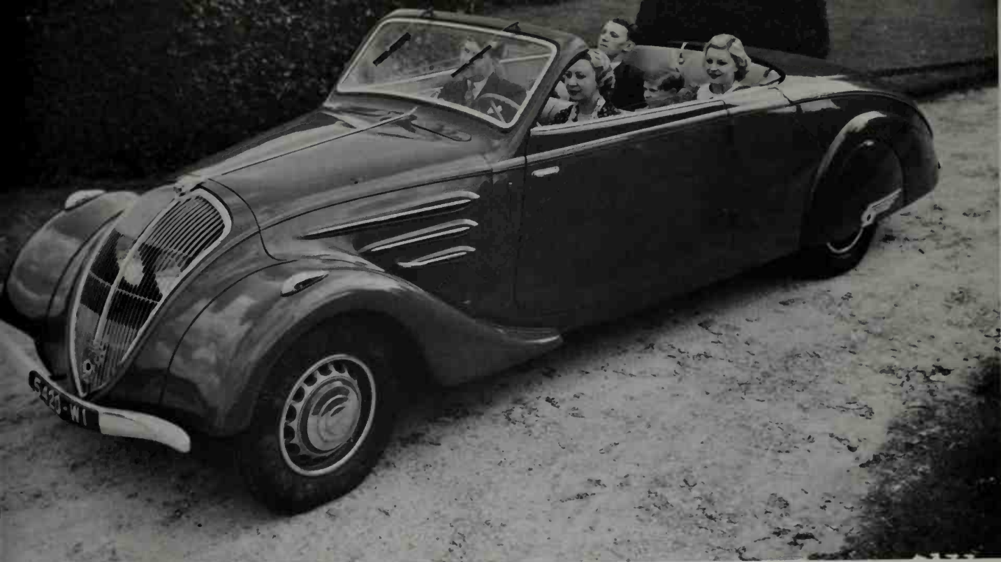
Open six-passenger coachwork on the 1938 Peugeot 402 with 4-cylinder, 2,142-cc. engine. (S.A. des Automobiles Peugeot)
