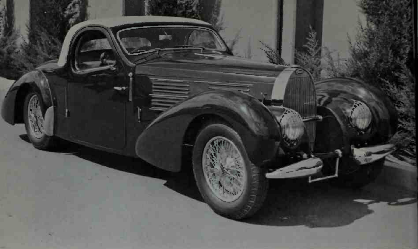
A Bugatti 57C coupé with coachwork by Gangloff of about 1939. The engine was a 3,257 cc. 8-cylinder, dual-ignition unit developing 135 BHP un-
