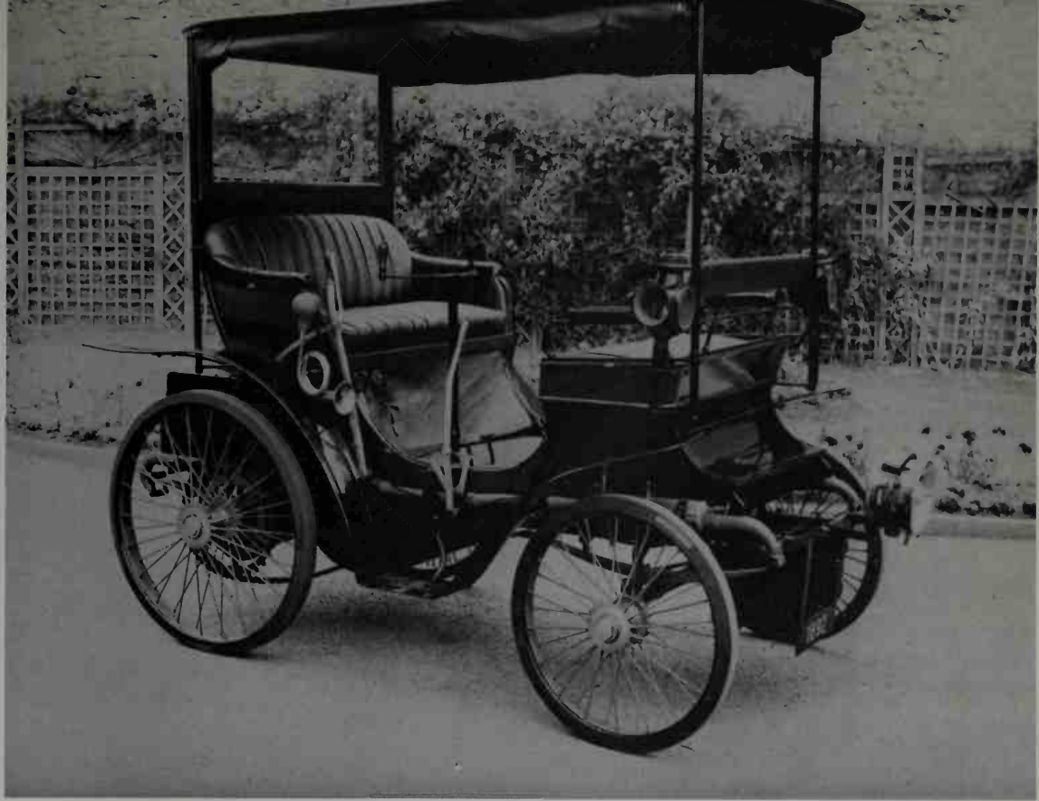
The 1892 Peugeot "vis-à-vis avec dais" (canopy) had a 1,645 cc. engine and could seat four to five
