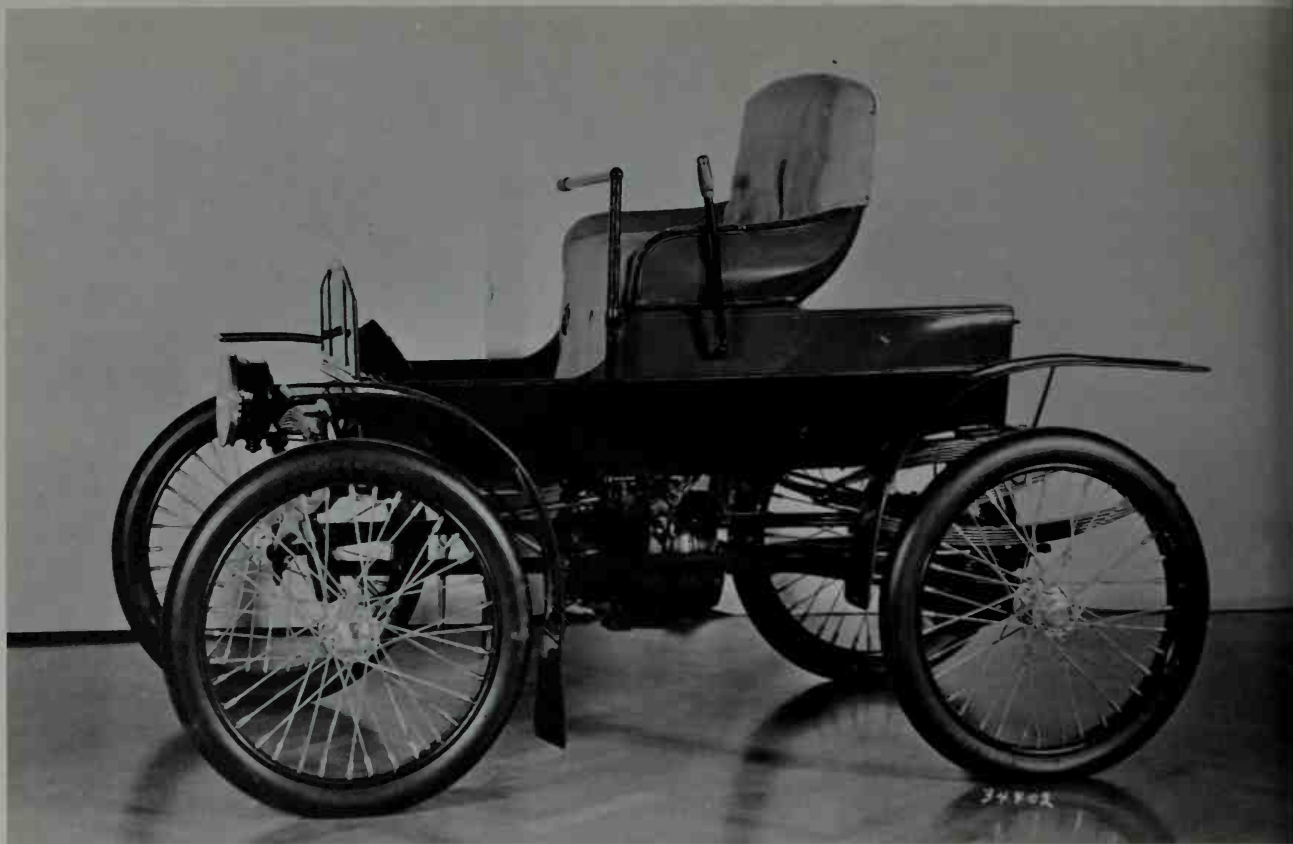
The two-seater Baker electric car of 1902 had a wheelbase of just 63 inches and, unusual for its time regardless of motive power, featured a shaft
