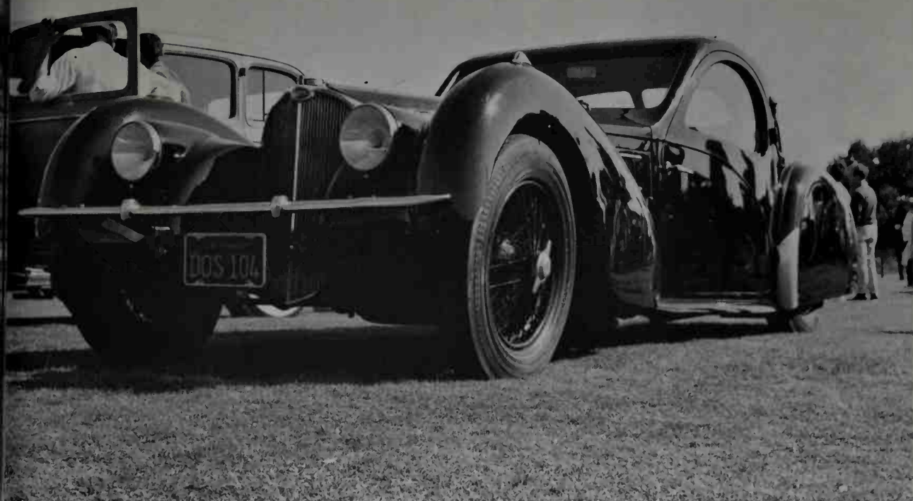
The Type 57S Bugatti is distinguished, externally, from the 57C by pointed radiator grille; produced during 1936–38. ( Joseph H. Wherry )
