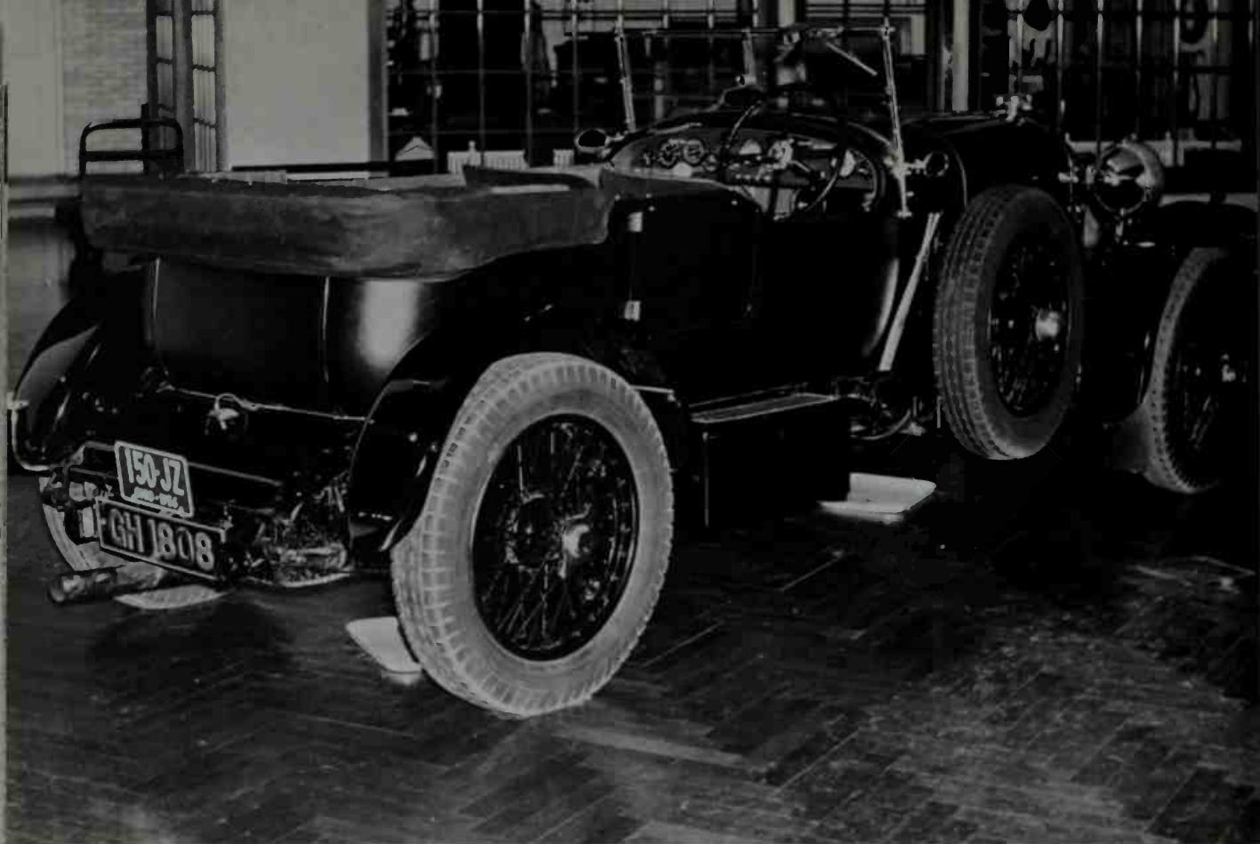
Weymann leather-covered coachwork on a 4.5-litre Bentley of 1930 in a period scene during a
