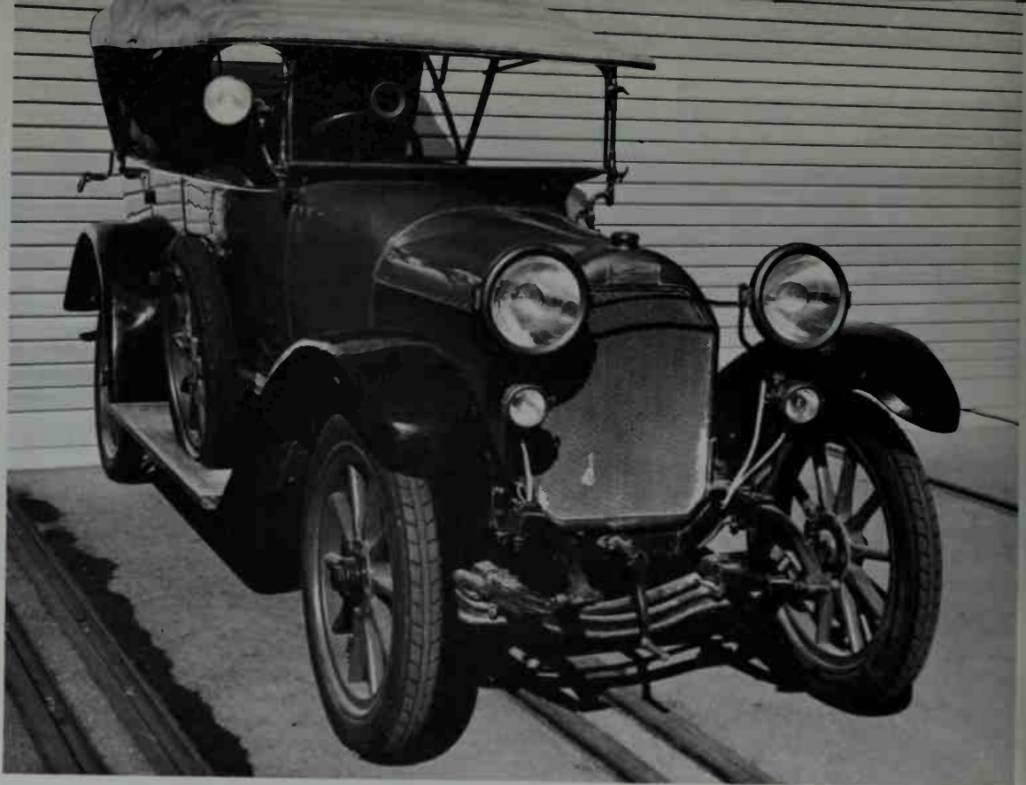
The 1914 Martini 6-seater tourer was popular as a military staff car; was also extensively exported. The 4-cylinder engine with bore and stroke of 85 x
