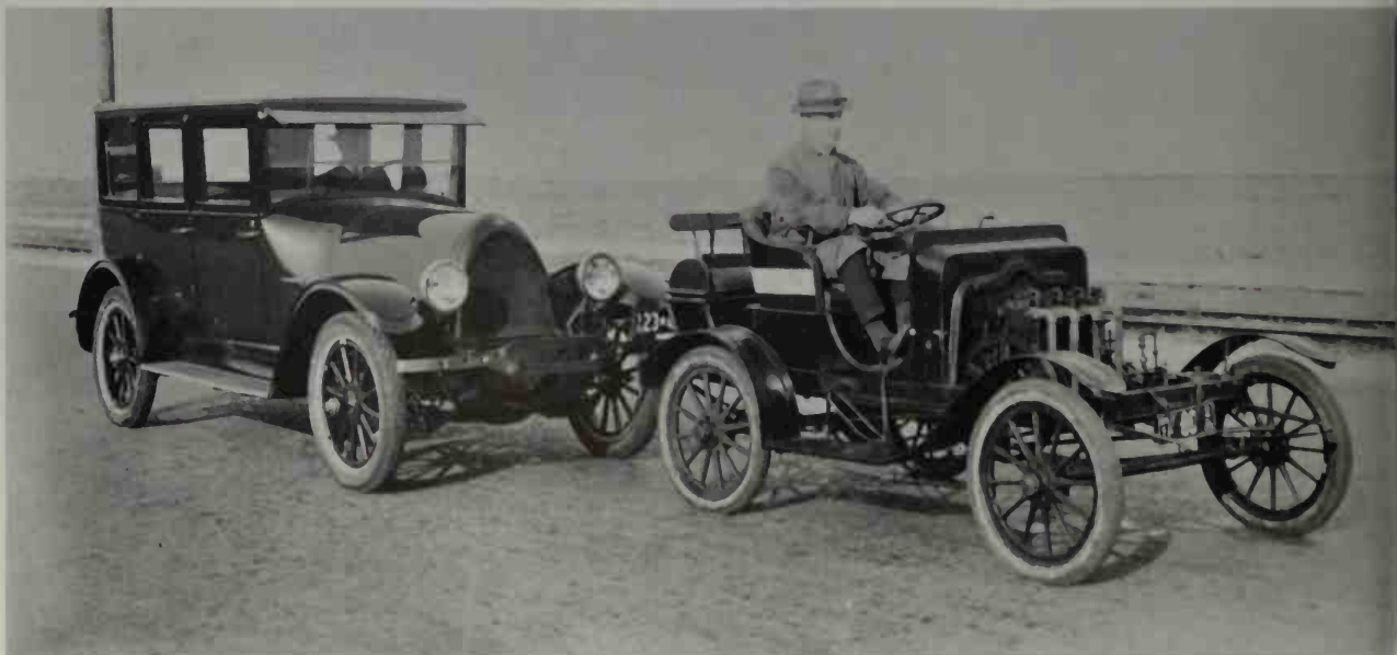
Bare chassis of pre-war, 20-HP Franklin discloses the full-elliptic springs, nearly vertical steering column and transversely mounted, 4-cylinder, 1.2-
