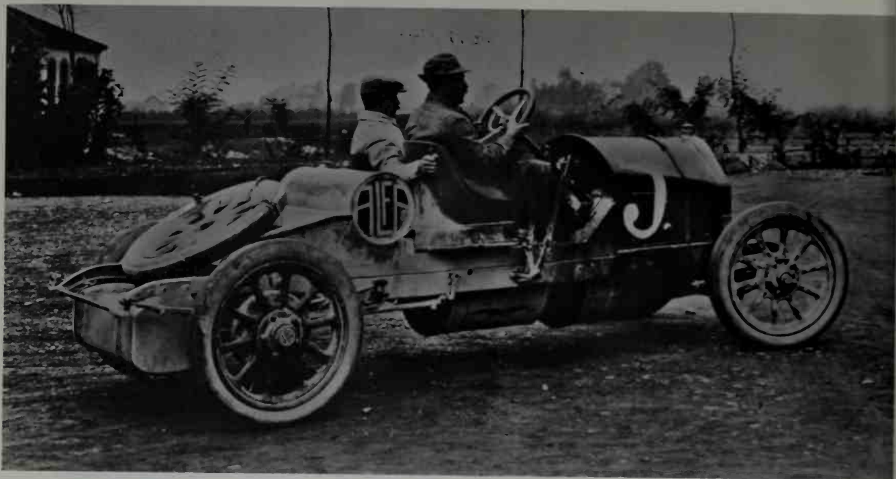
The first all-Italian car from the ex-Darracq works in Portello was the A.L.F.A. 24 HP of 1910. Power was by a side valve, 4,084 cc., mono-bloc
