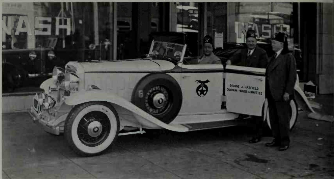
The dual-ignition, straight-8 Nash phaeton of 1932; comfort on 130-inch wheelbase for parades
