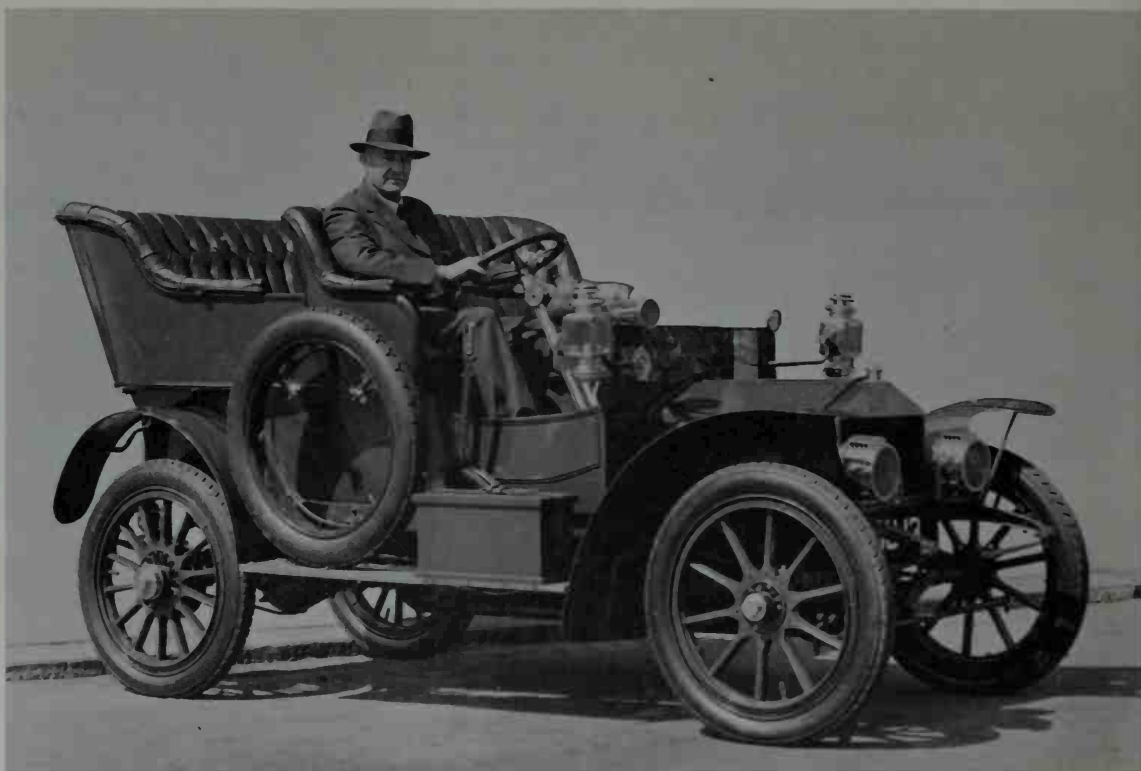
The 1905 Rolls-Royce 10-HP, 2-cylinder model, instantly a success due to unexcelled craftsmanship. Royce pioneered full pressure lubrication in
