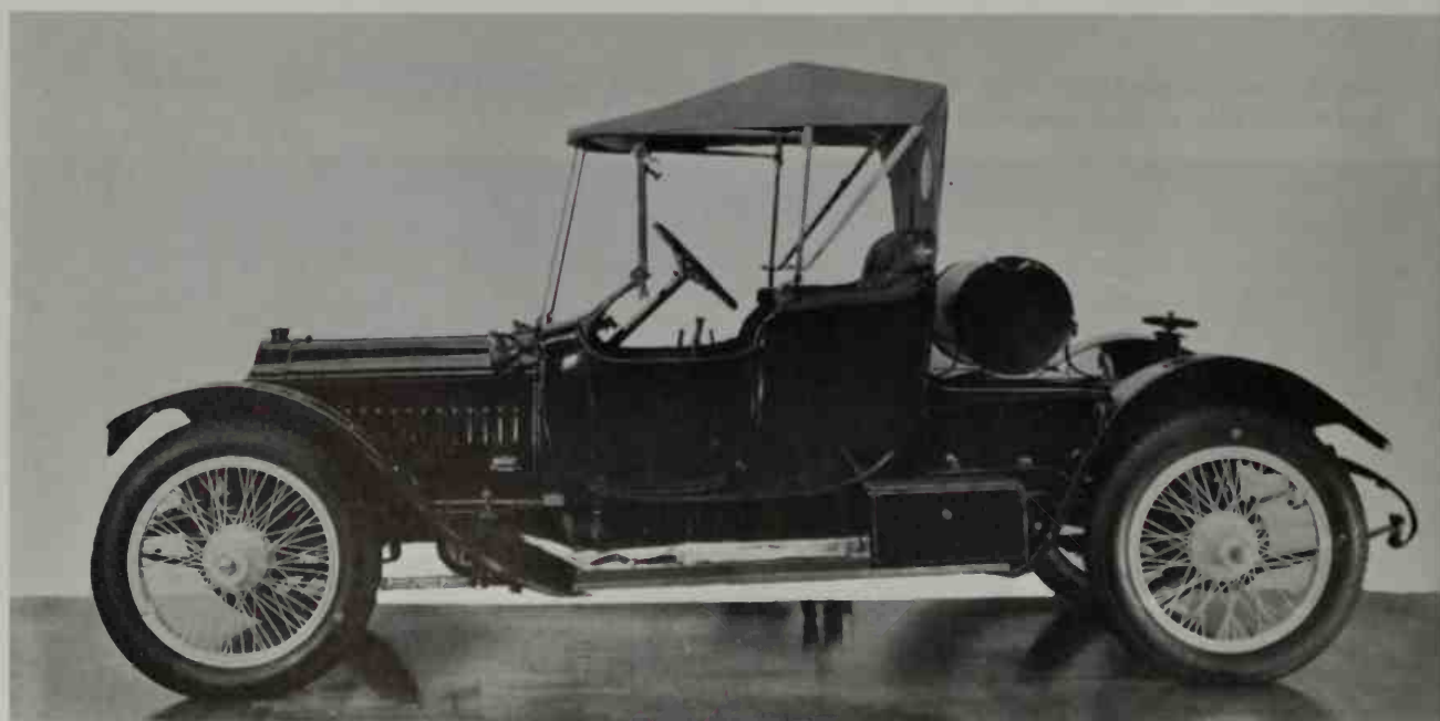
1911 De Dion-Bouton roadster was imposing on a 129-inch wheelbase. A large V-8 engine developed 26 CV. ( Henry Ford Museum )
