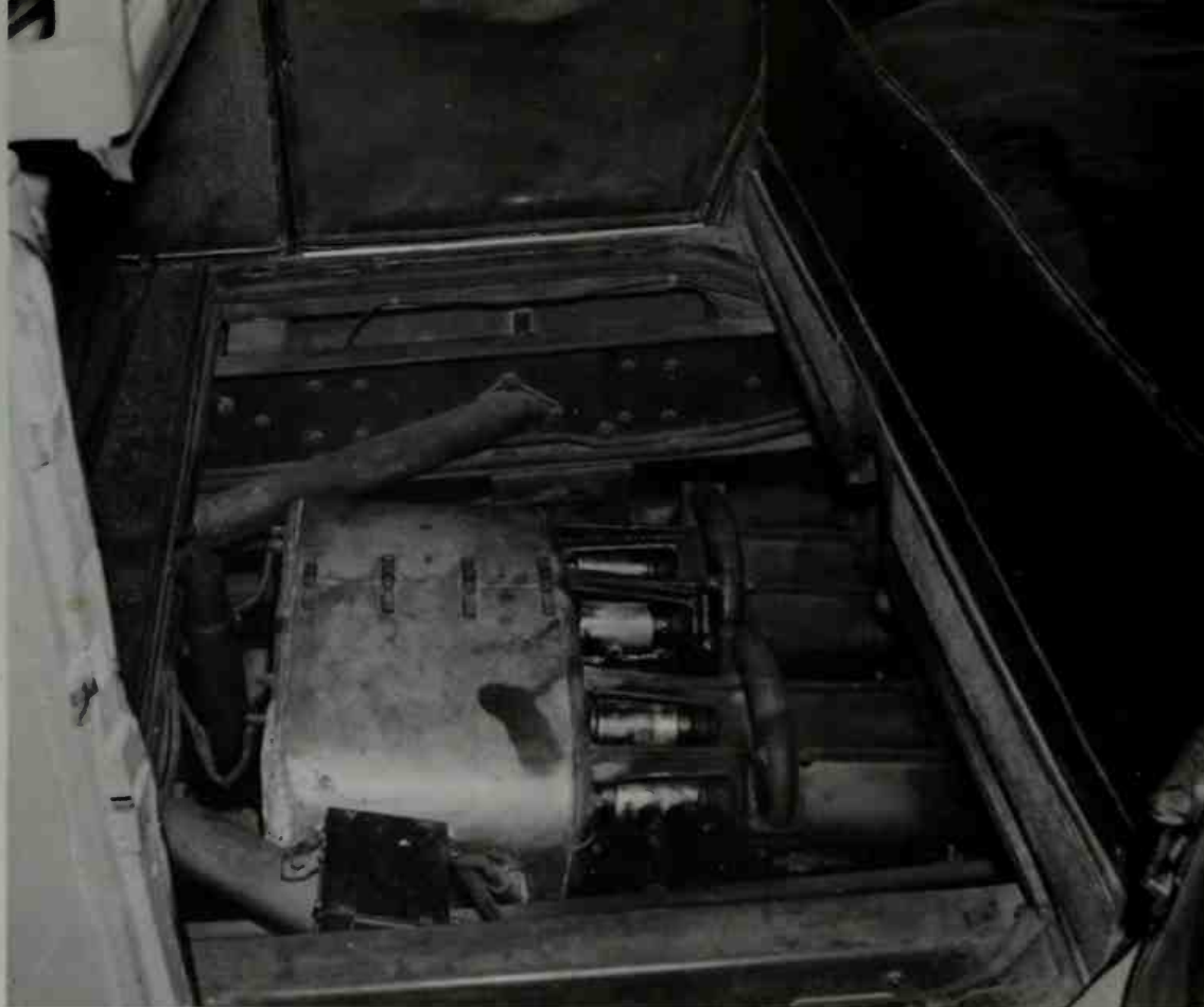
The engines of the Doble Steamers occupied the space between the longitudinal frame members beneath the floor of the rear passenger compart-
