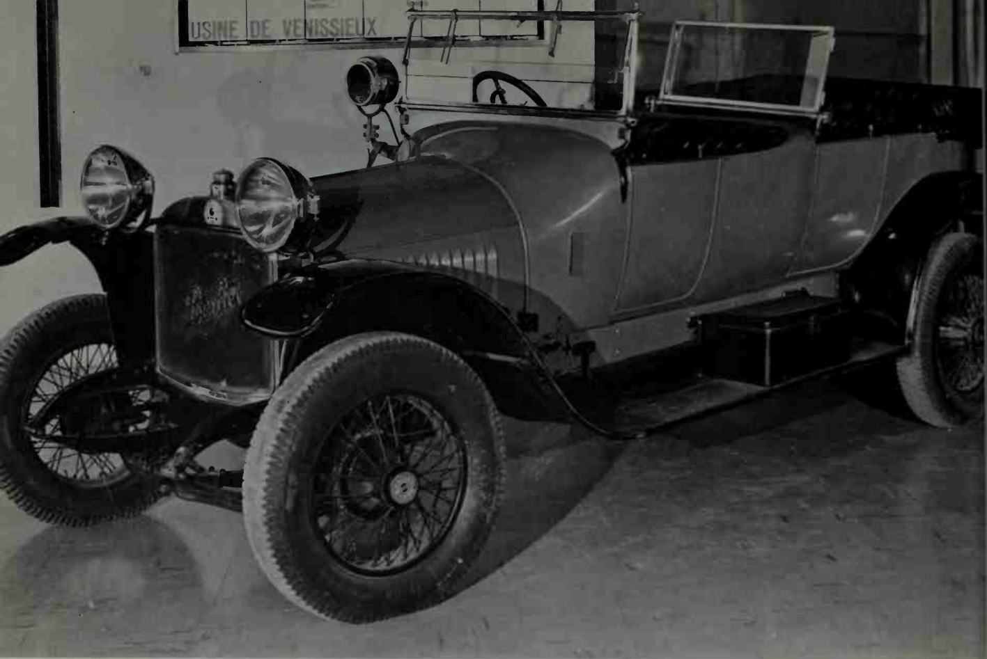
French elegance—the 4-cylinder, 4-litre Berliet dual-cowl torpedo on 126-inch wheelbase. Note
