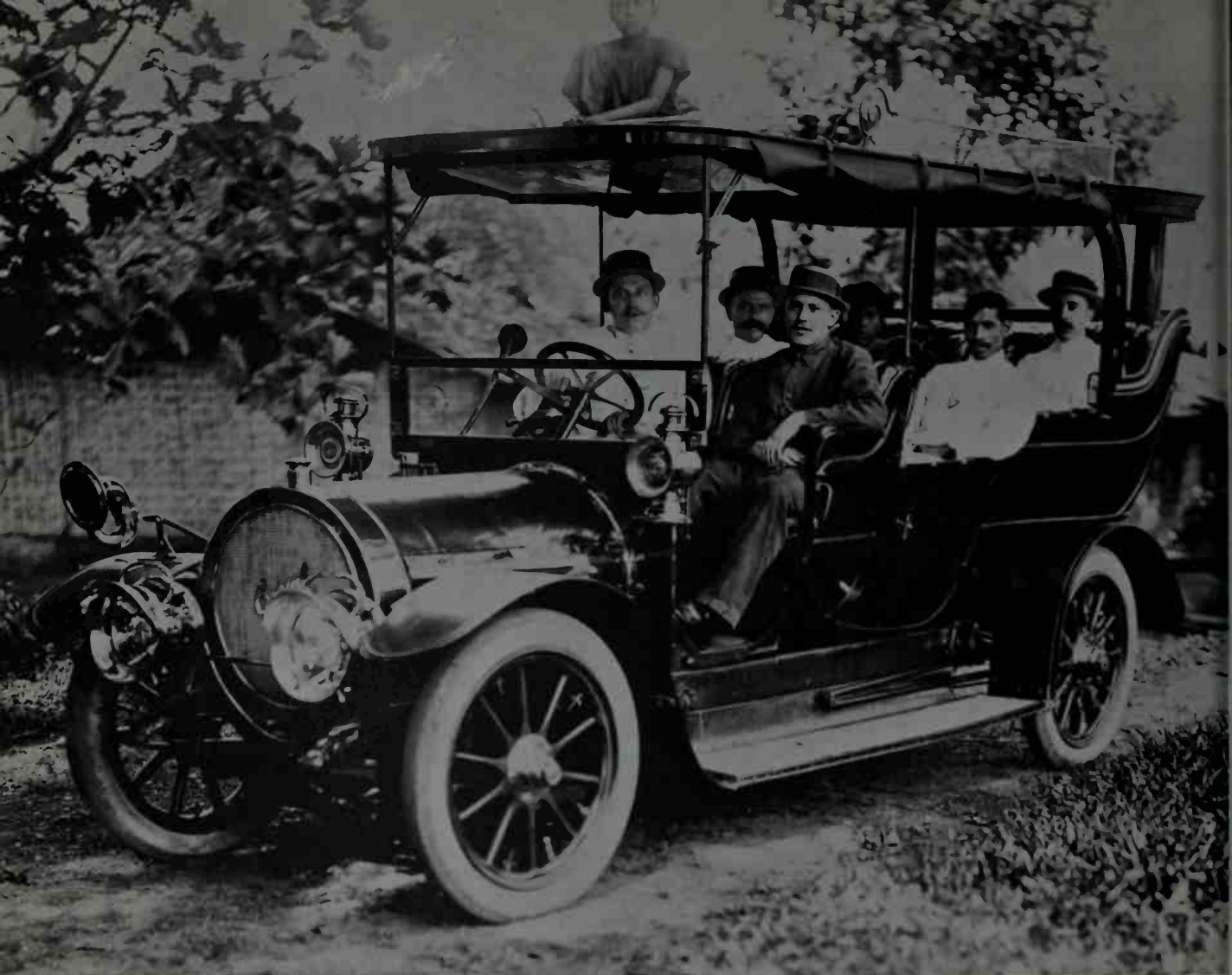
A large car, the 1908 Eysinck had a 6-cylinder engine. The bracket on the steering column located the rubber horn bulb at the driver's right
