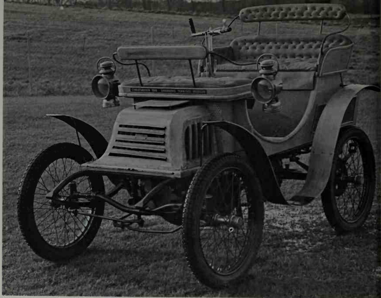
H. C. Christiansen built his first car in 1899. The chassis is of tubular construction. ( Danmarks Tekniske Museum )
