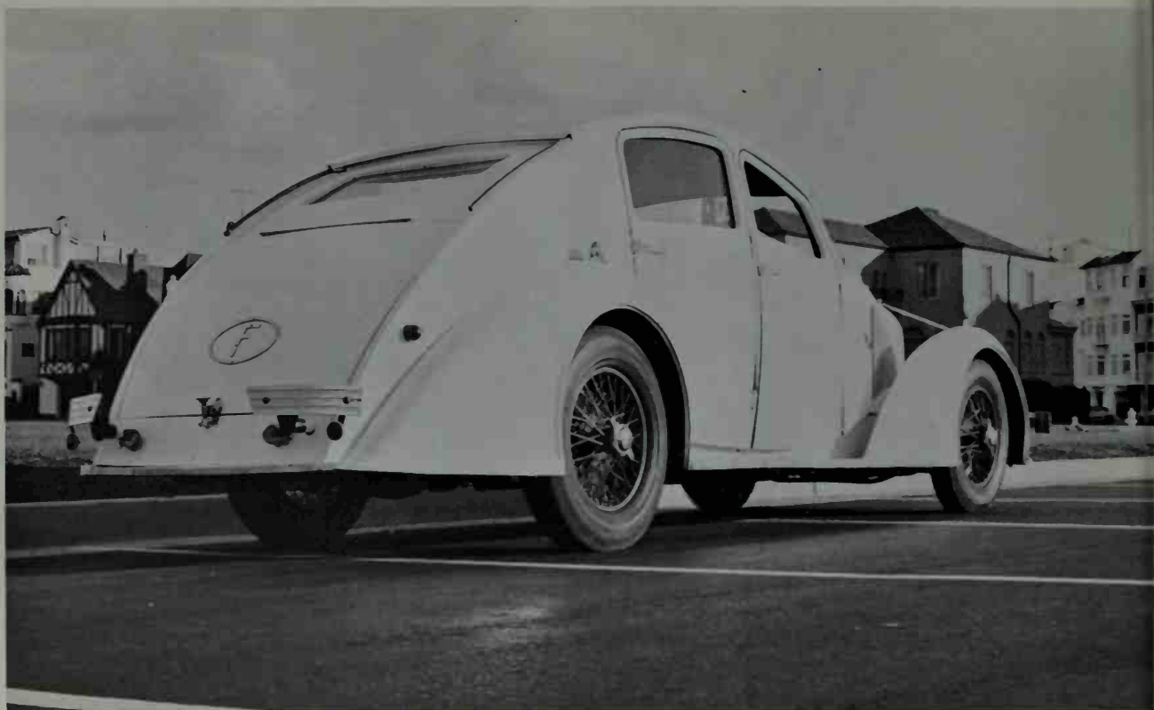
Roof slid back on rails along edges; doors were hung on piano hinges. The 1934 Voisin "Aero Sport." (Joseph H. Wherry)
