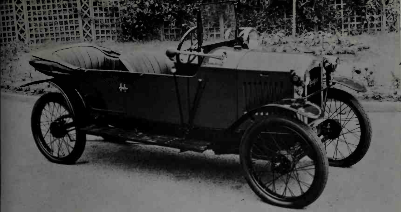
The diminutive 1921-23 Peugeot "Quadriette" Type 161 had 91-inch wheelbase. Driver and passenger sat in tandem. L-head, four 50 x 85-mm.
