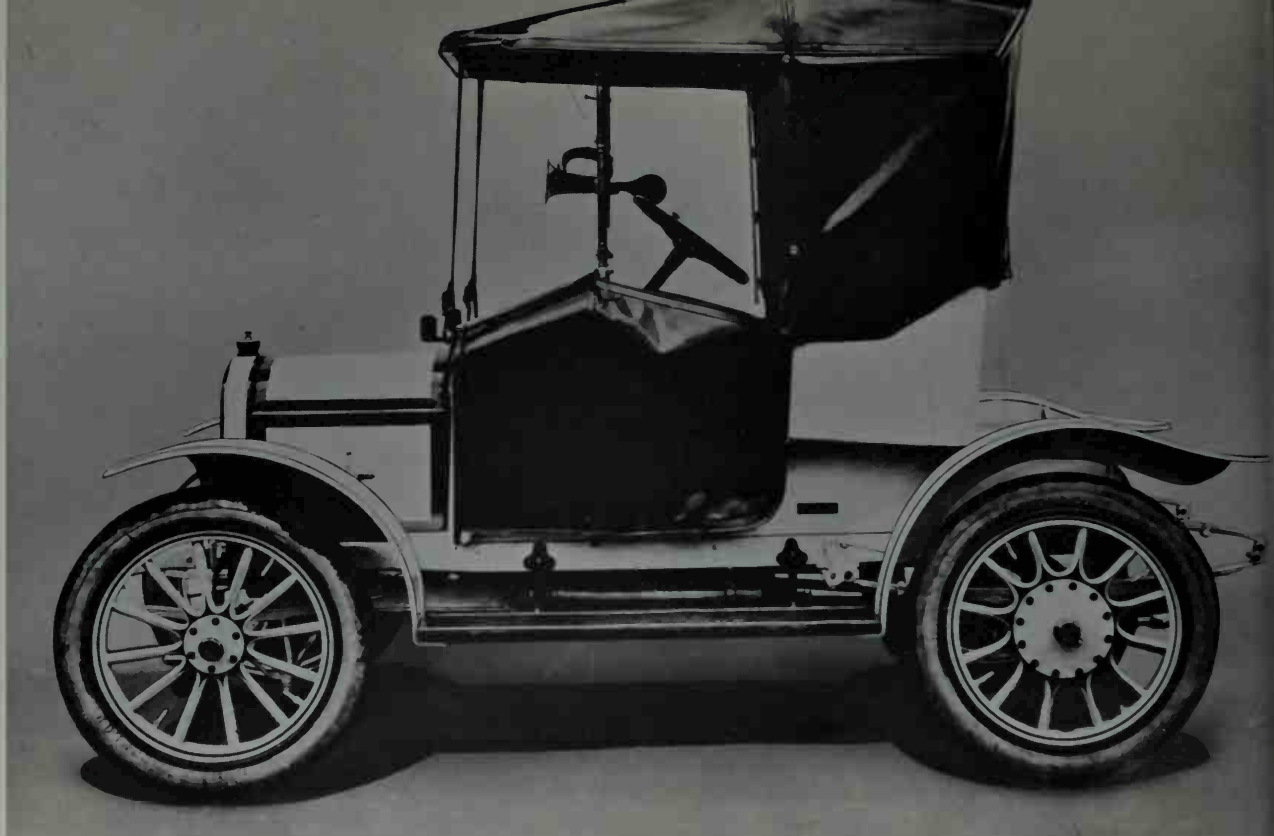
The 1909 single-cylinder, 7-HP Austin, one of the marque's first production models and the original
