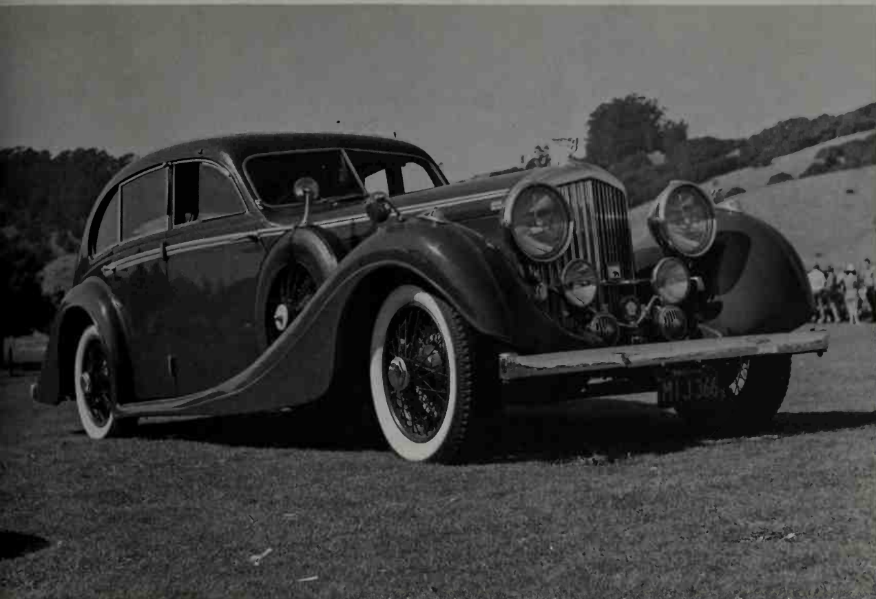
4.25-litre, 6-cylinder (89 x 114 mm.) Bentley of 1937 with aluminum coachwork by Gurney Nutting. Note the filled seams between body and
