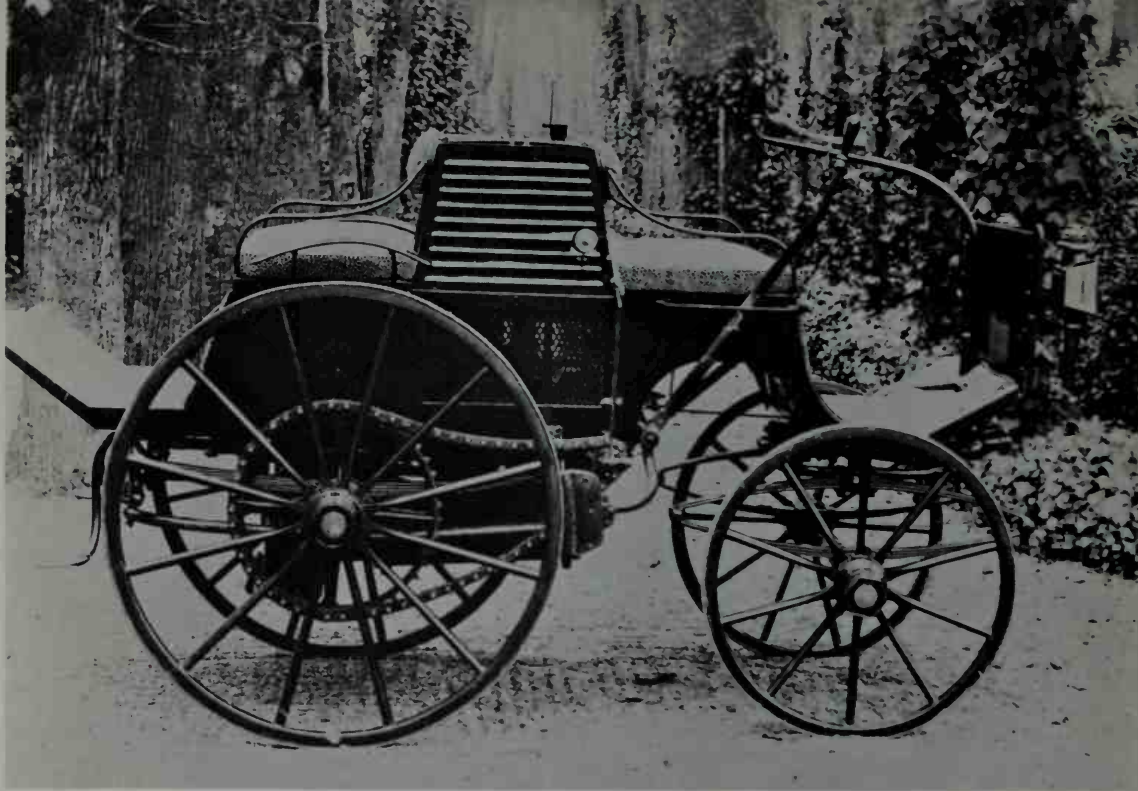
The first Panhard car of 1889-90 had a rear-mounted, vertical, 2-cylinder, 2-horsepower engine;
