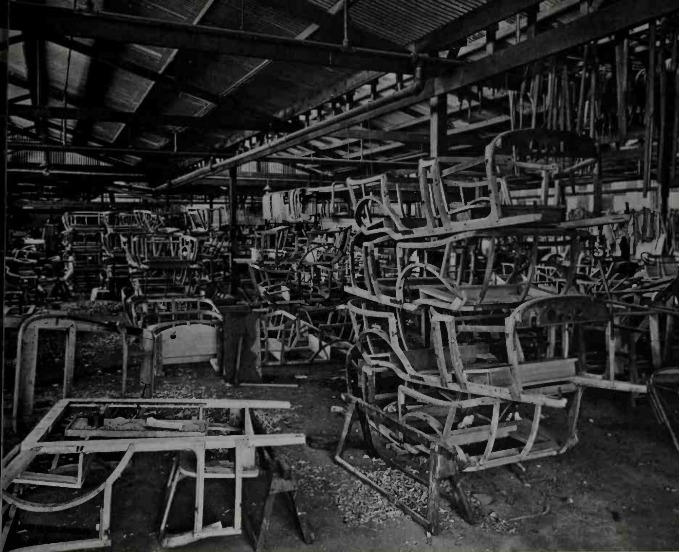
Hardwood frames for automobile bodies in the Holden coachworks in 1918. ( Wheels Magazine )
