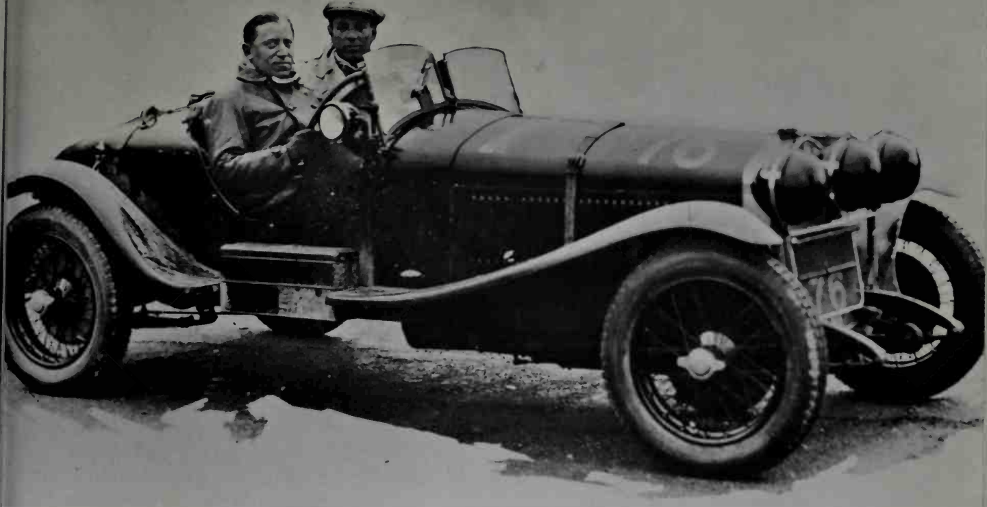
Pirola and Guidotti in the Alfa Romeo 6C 1,500 SS in which they won their class in the 1929 Mille Miglia. The 6-cylinder, 1,487-cc., supercharged
