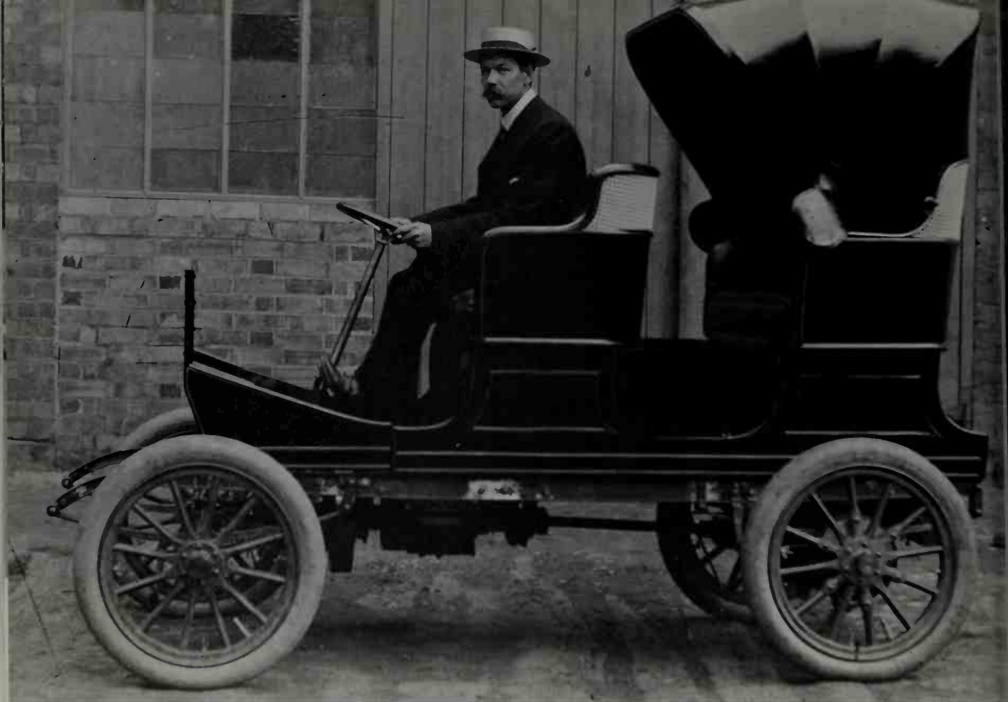
The first Standard car was this 6-HP, shaft-driven, 1.4-litre, single-cylinder (127 x 76.2 mm.) wicker-
