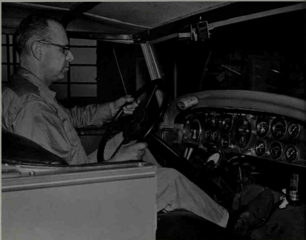
Bernard Becker studies the full facia of instruments in the 1930-31 Doble. In addition to the usual performance gauges, steam cars had pres-
