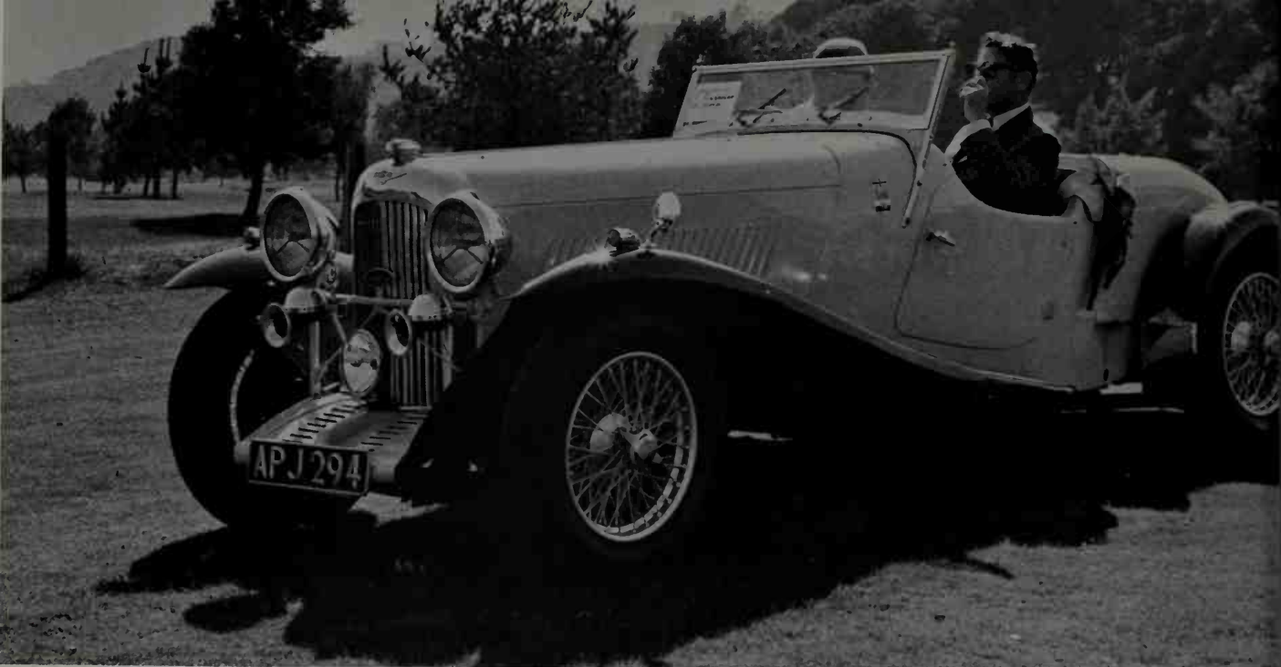
The 2,931 cc., 6-cylinder (72 x 120 mm.) Lagonda 16/80 sports two-seater of 1933 owned by G. Vaughn. The 6-cylinder engines were made by
