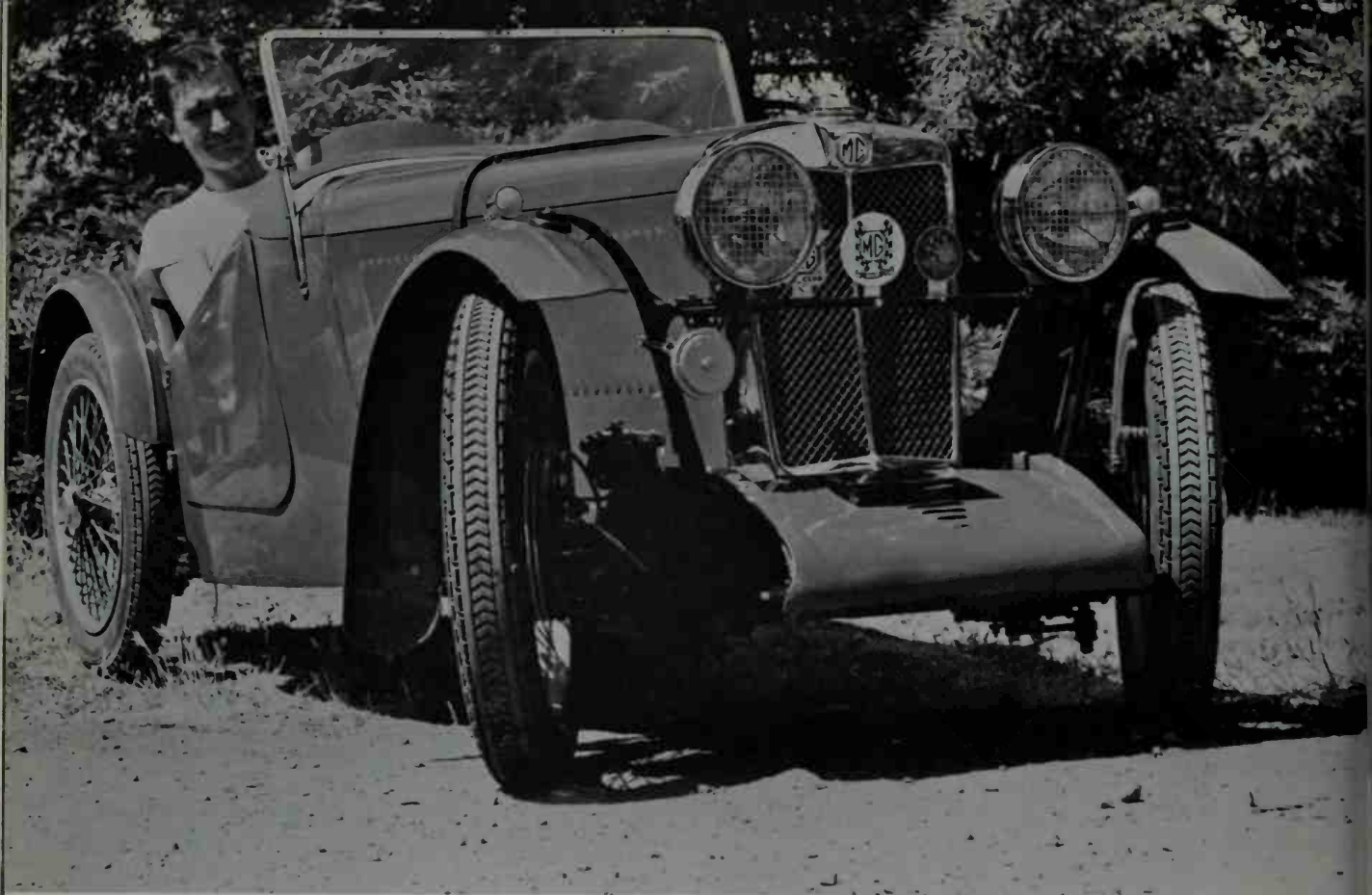
The single overhead-camshaft J2 "Midget" M.G. had 4-cylinder, 847-cc., 36-BHP engine; was light,
