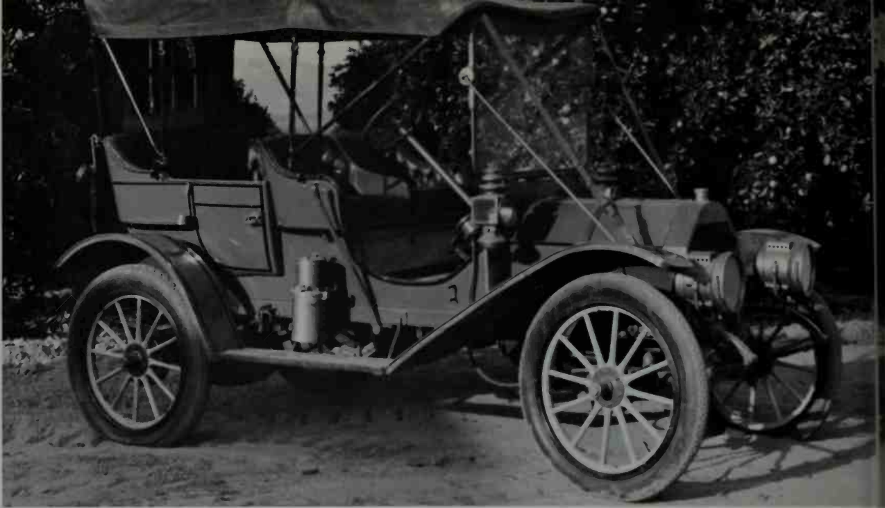
The 1909 Cartercar (1907-16) had a friction drive which gave an infinite number of gear ratios. The foot brake pedal functioned as a parking brake when depressed, as shown here, and moved to the right where it locked in place by a ratchet device; the speedometer mounted outboard of the body on the armored cable was an added item in a later year. This car is in the Lindley Bothwell collection. (Photo by Author)
