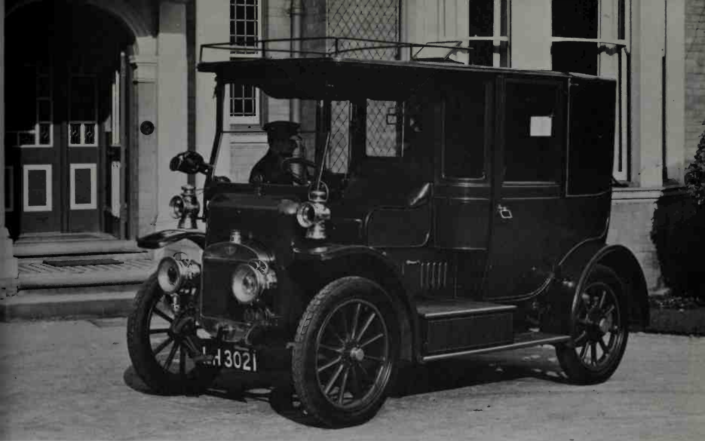
The popular Austin "Town Carriage" of 1911, technically a landaulet. Driver sat over the engine. ( British Motor Corp. Ltd. )
