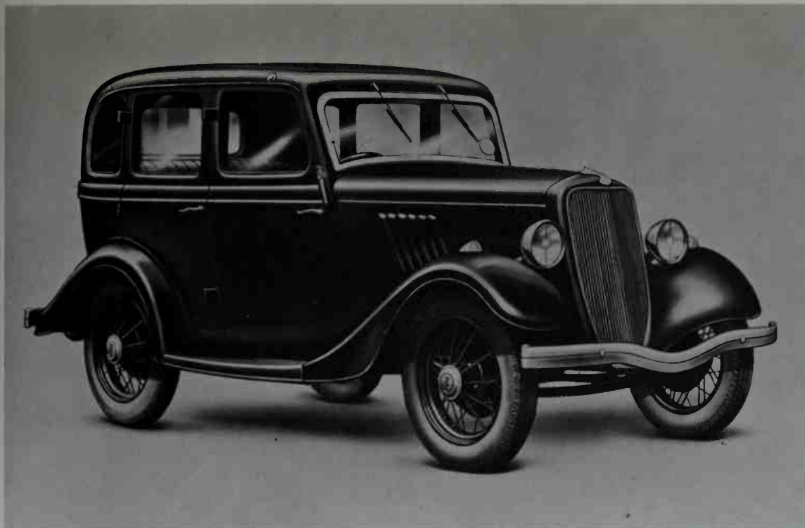
The 1935 Ford "Ten" with L-head 1,172 cc., 4-cylinder engine looked like a miniature Ameri-
