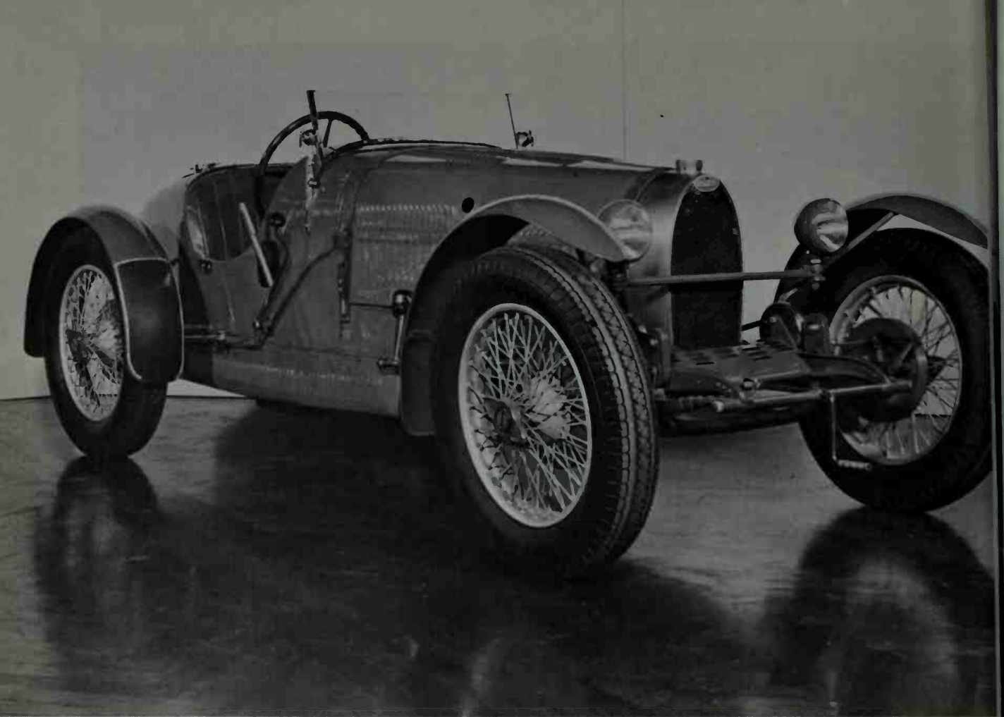
Bugatti type 35T with supercharged 2,270 cc. engines were the nemesis of opponents on the grand prix circuits. ( Henry Ford Museum )
