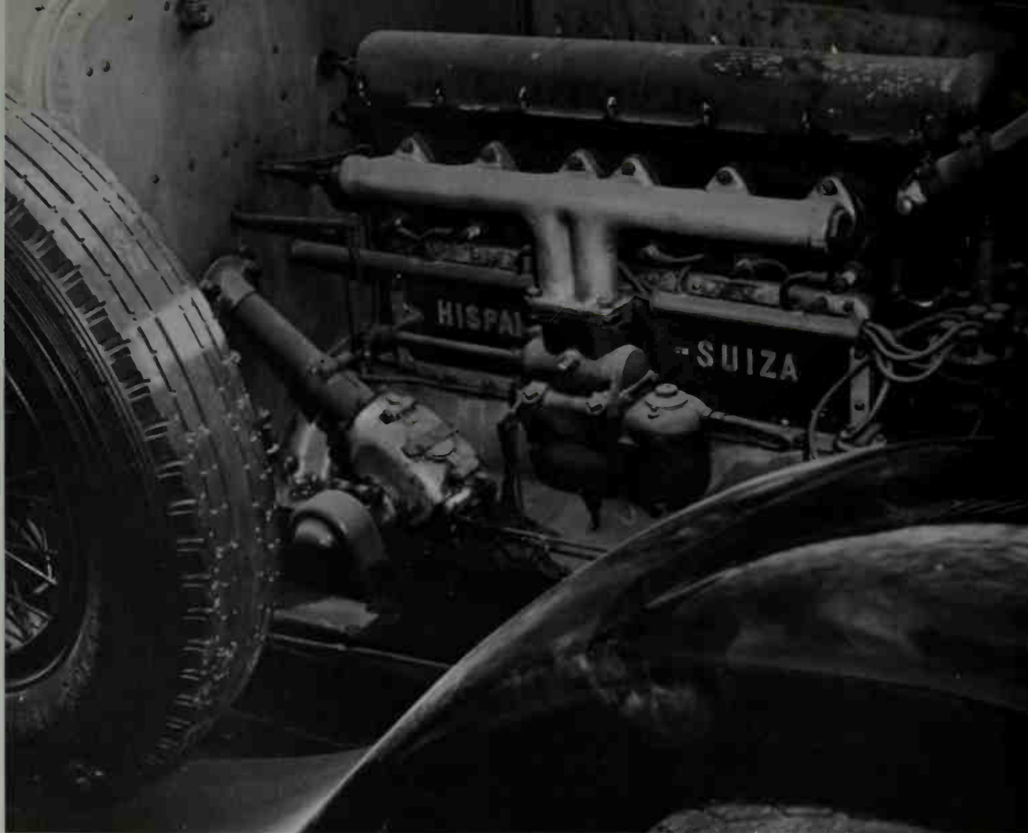
The 6.5-litre, 6-cylinder, single-ignition, overhead-camshaft engine in the 1922 Hispano-Suiza
