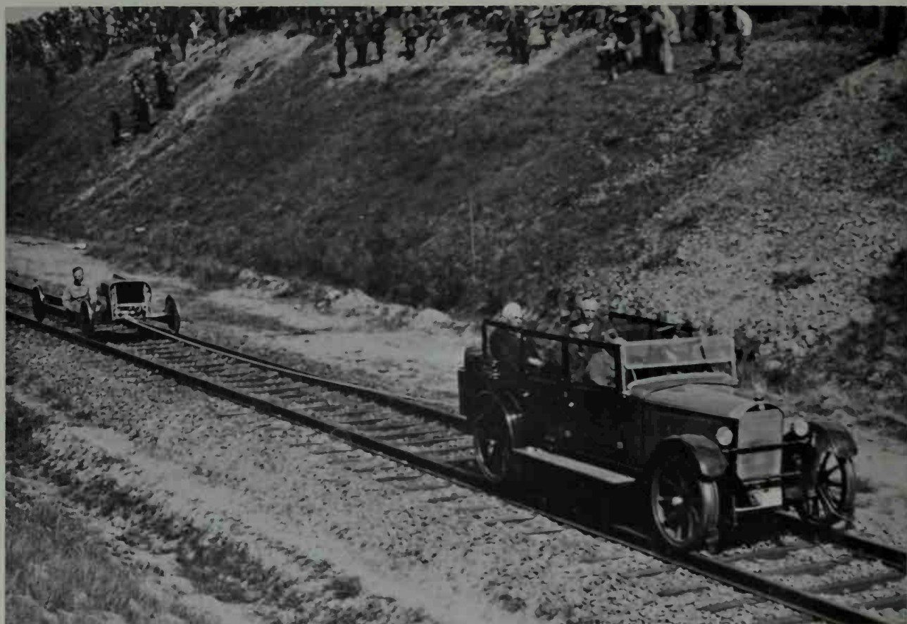
Tests of Opel-Raketwagen "Rak 3" involved large tow car and rails. (Adam Opel AG)
