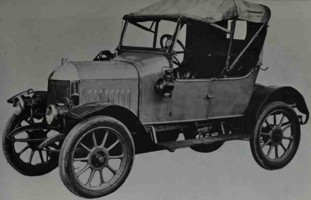
Ancestor of the M. G. and the first production Morris was the 1913 "Oxford," a 90-inch-wheelbase, 10-HP, 4-cylinder (60 x 90 mm.), 1,018 cc.
