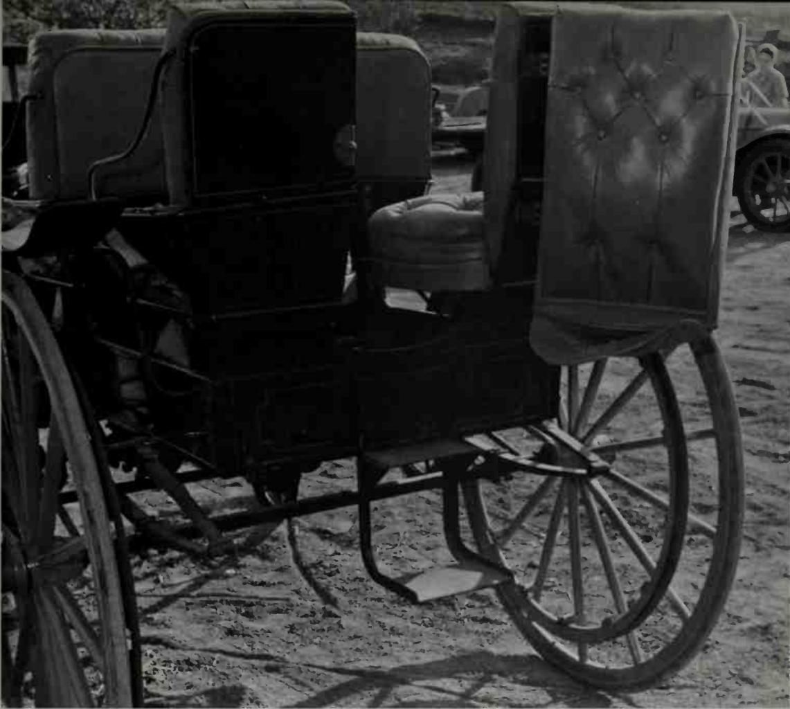
This 1902 Holsman Auto Buggy belongs to the Lindley Bothwell collection and is the four-seater model; rear passengers entered through a tonneau
