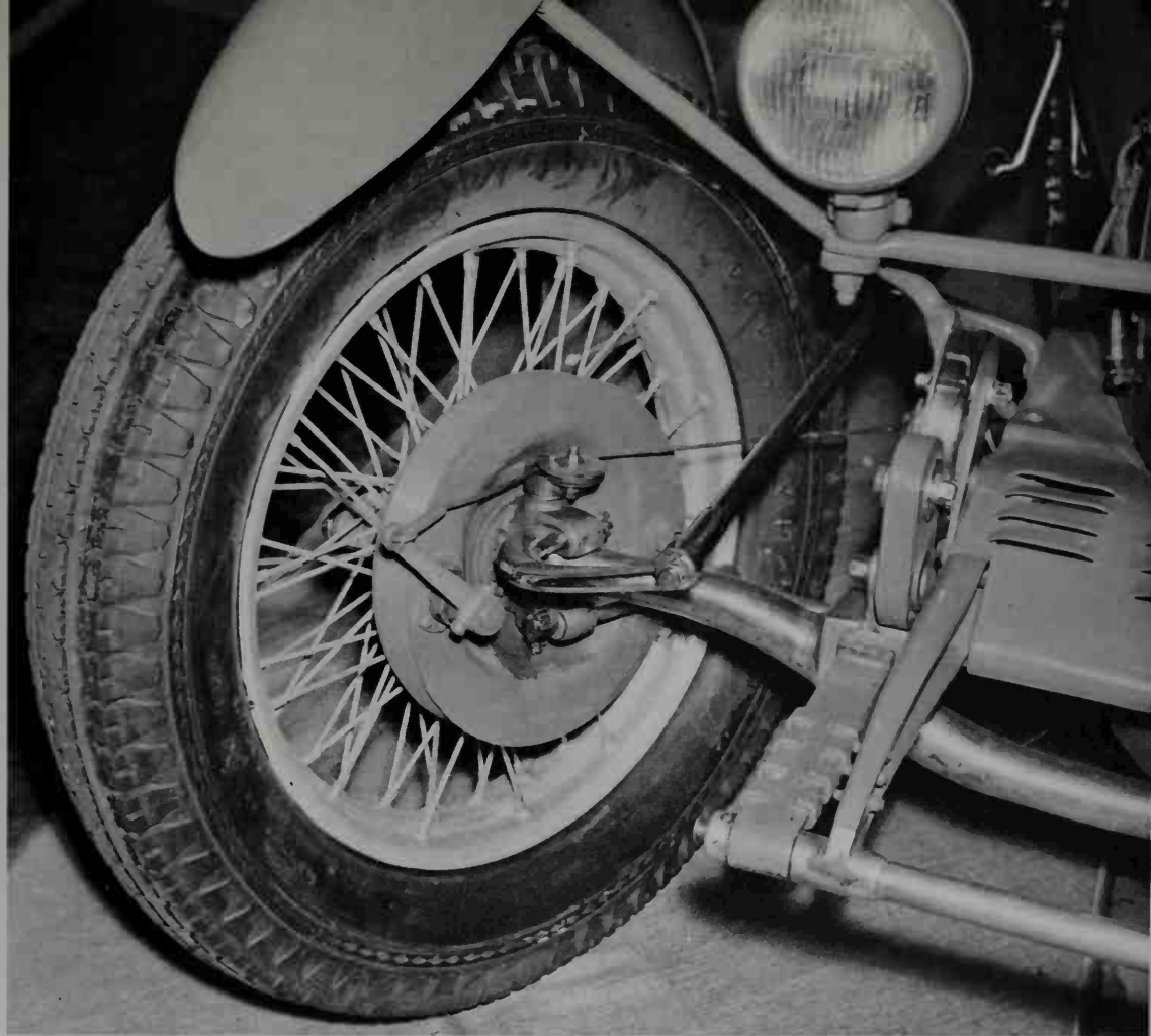
Converted for road use, this Bugatti 35T has wire wheels. Note finned brake drum, spring through
