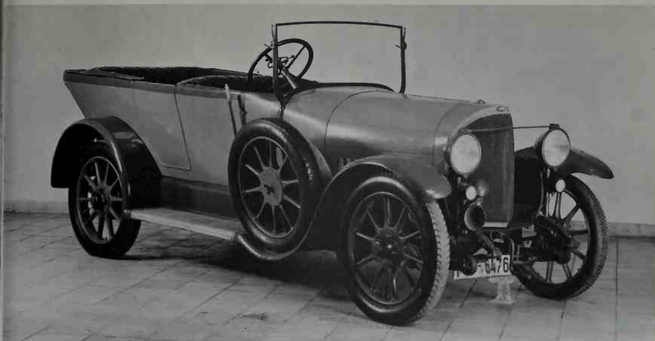
Tulip body and pointed radiator shell on 8/25-HP, 4-cylinder 1920 Opel shows influence of pre-
