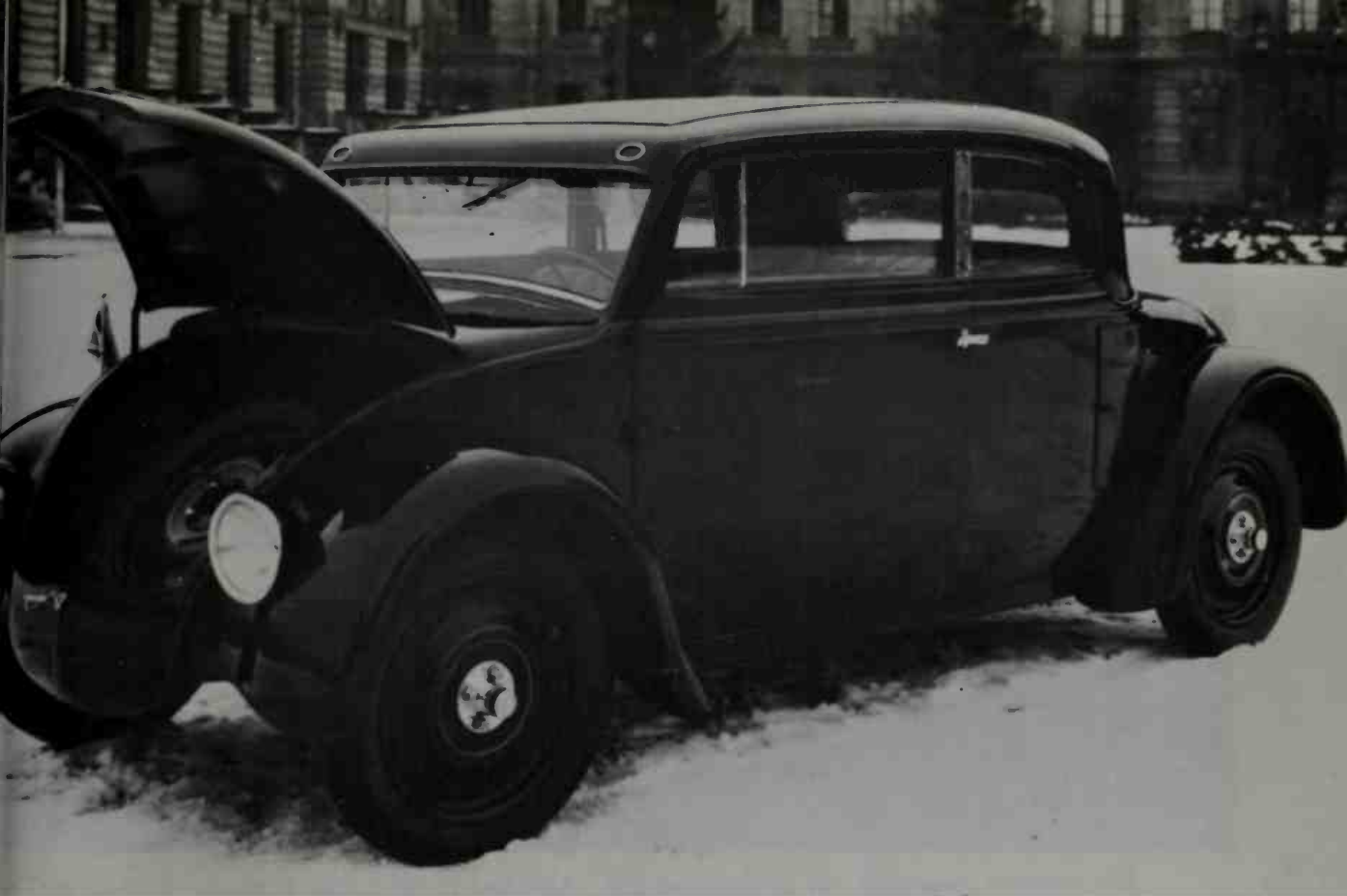
The experimental Skoda Type 932 of 1934 had its 4-cylinder engine in the rear. Note the spare
