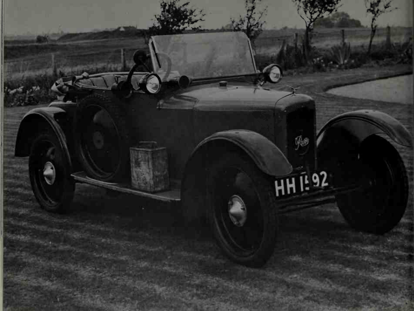
The immensely popular 2-cylinder (85 x 88 mm.), air-cooled Rover of 1922; wheelbase 88 inches. (Leyland Motors Ltd.)
