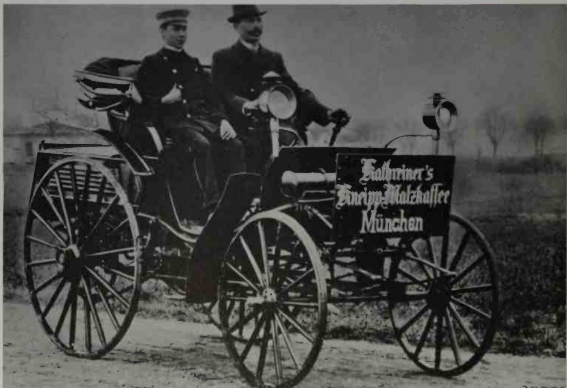
The Benz "Victoria" of 1893-94 had a rear-mounted, air-cooled, single-cylinder engine devel-
