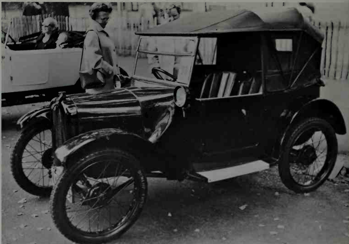
The 4-cylinder (56 x 76 mm., 749 cc. displacement) Austin "Seven" of 1923 brought motoring within the means of the masses; continued with
