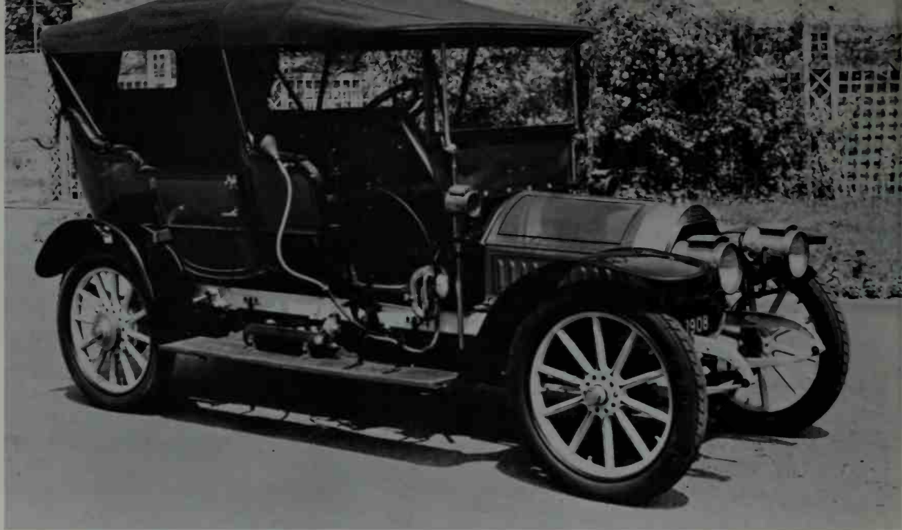
The Lion-Peugeot of 1908 had a 4-cylinder, 2,211-cc. 16 CV engine coupled to a 4-speed gearbox. (S.A. des Automobiles Peugeot)
