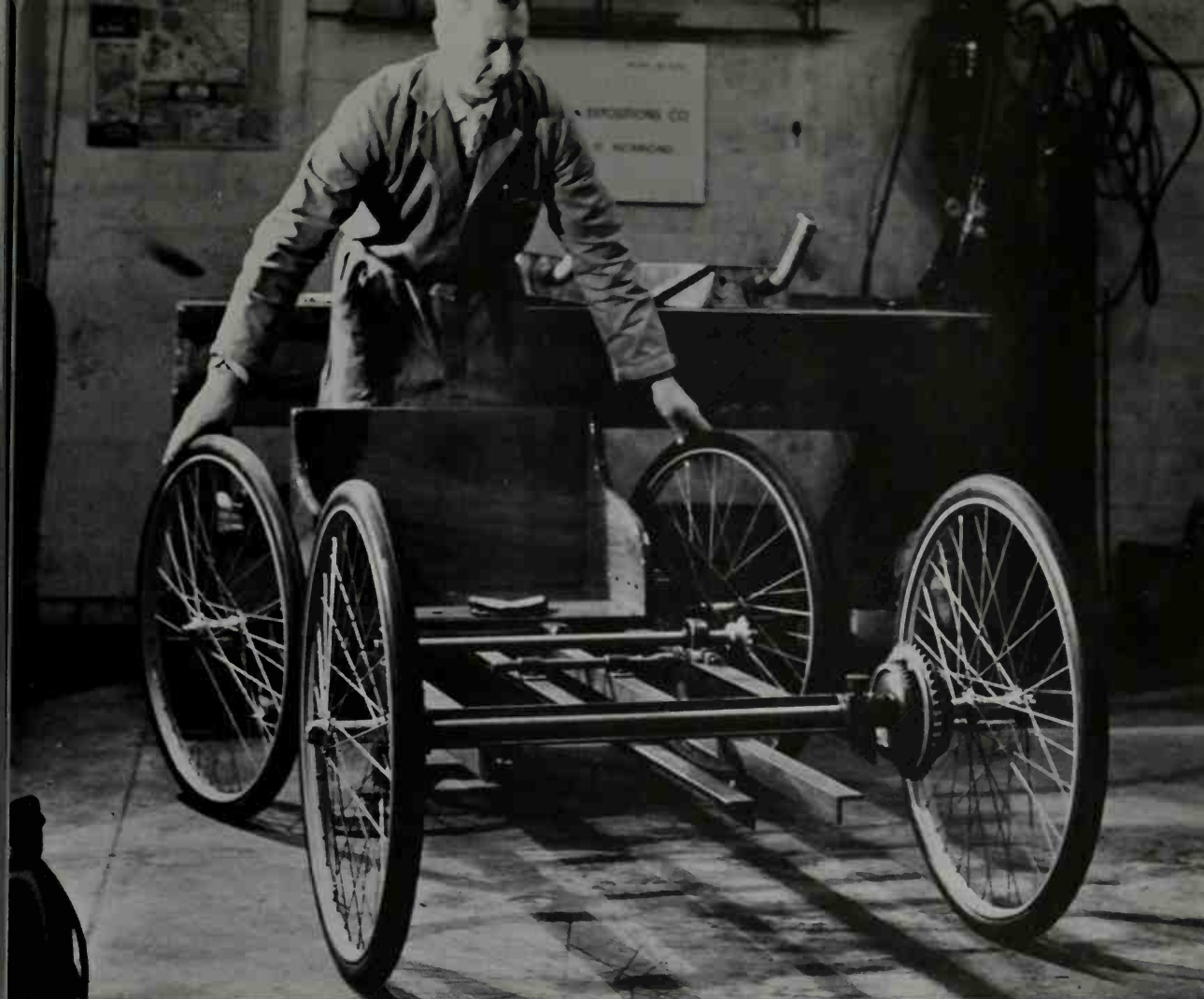
Mr. Tom Myers, engineer of Melbourne, Australia, shown in his workshop where he built a replica of a four-wheel, light motor vehicle of the cyclecar
