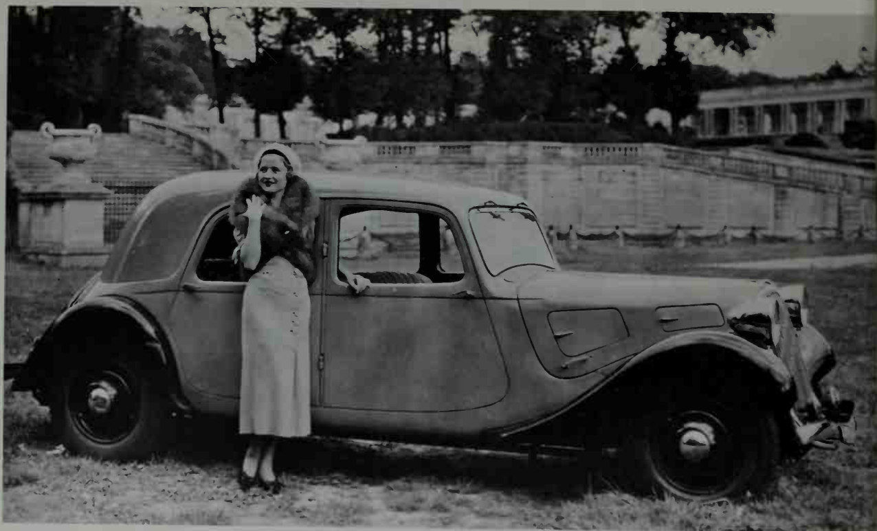
Citroën's famous "traction avant"—front-wheel-drive—cars were introduced in 1934. The "Light Eleven" model. ( Société Citroën )
