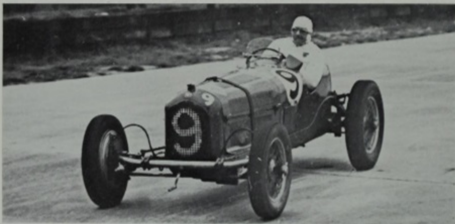
Frank Ashby's car at the Dunlop Jubilee meeting at Brooklands in 1939, showing the narrow bodywork he fitted and the Dubonnet fit with Ashby's own Lockheed brake conversion. (Louis Klemantaski)
