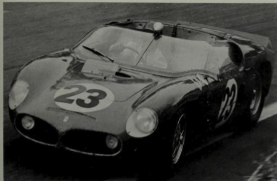
Richie Ginther in the 1961 Le Mans 246 SP one of the first of the 2.4-litre rear-engined V-sixes. This was the first car to use a rear spoiler (Geoffrey Goddard)
