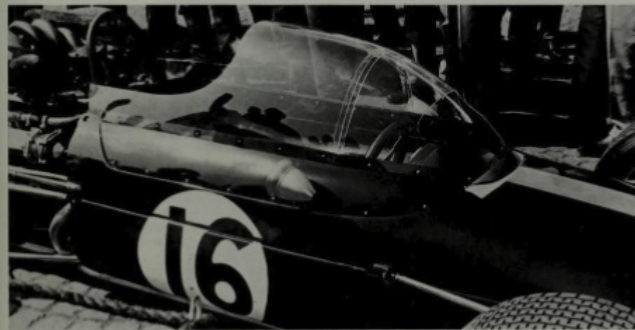
Horses for courses: for Monza Brabham tried this bubble canopy and also a gearbox cover in an attempt to reduce the BT24's drag. He suffered parallax problems with the canopy and ran standard bodywork in the race
