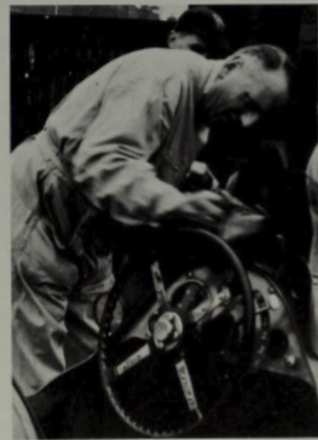
This picture of Etancelin cleaning his aero screen shows the selector on the steering column for the Wilson four-speed pre-selector gearbox, also "Phi-Phi's" supplementary cowling each side of the screen. He finished second to Ferraris in both the European and Czech GPs of 1949.
