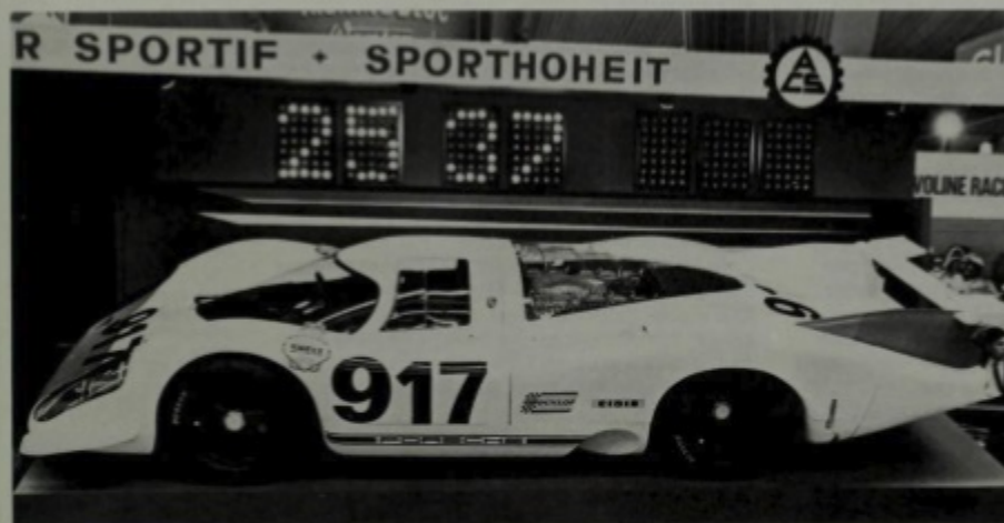
The first 917 to be built was the talk of the 1969 Geneva Motor Show. It was exhibited with its bolt-on long tail, and was listed at 140,000 DM (about £14,500 at the time). The very conservative figures of 520 hp and 200 mph were claimed. (Geoffrey Goddard)
