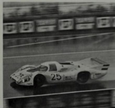
1970—No 25, driven by Elford-Attwood, was much more stable, despite its fixed rear wing and absence of front spoilers. The concave nose and unswept tail are notable features. (Geoffrey Goddard)
