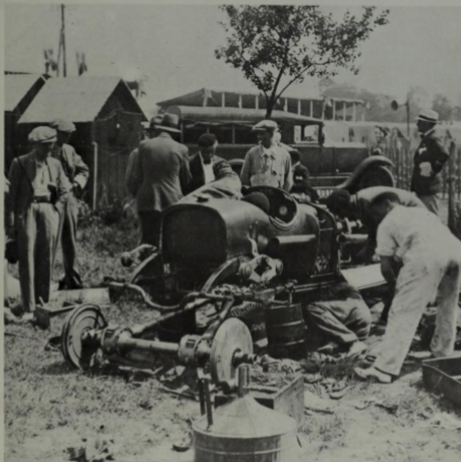
Mechanics changing Lehoux's gearbox between a heat and the final at Dieppe in 1934, showing the higher cockpit side of the later cars and also the unique dual drive transmission
