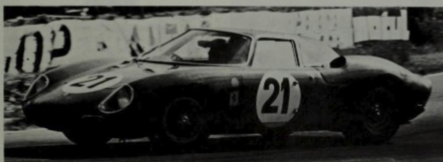
Externally the 365 P delivered to selected private entrants was identical with the 330 P2 works cars, but they had a larger (4.4-litre) engine with two instead of four camshafts. Graham Hill taking stock of the Maranello Concessionaires' car at the start of the 1965 Nürburgring 1000 Kilometres (Michael Cooper)
