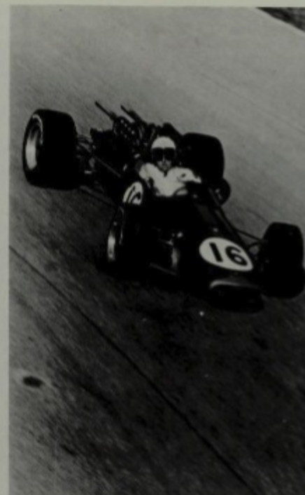
Not this time: Brabham lost the '67 Italian GP to Surtees' Honda on the last corner, and finished a close second. Here the oil-covered BT24 hurtles into the Parabola, showing its tail fins and air deflectors ahead of the front suspension. These created a low pressure area in the suspension "bays" which extracted hot air from the radiator
