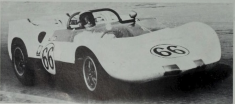
Mosport, 1964: a new nose and accompanying tail treatment make a more homogeneous racing car. Cooper wheels have replaced the earlier Lotus variety. (Pete Lyons)
