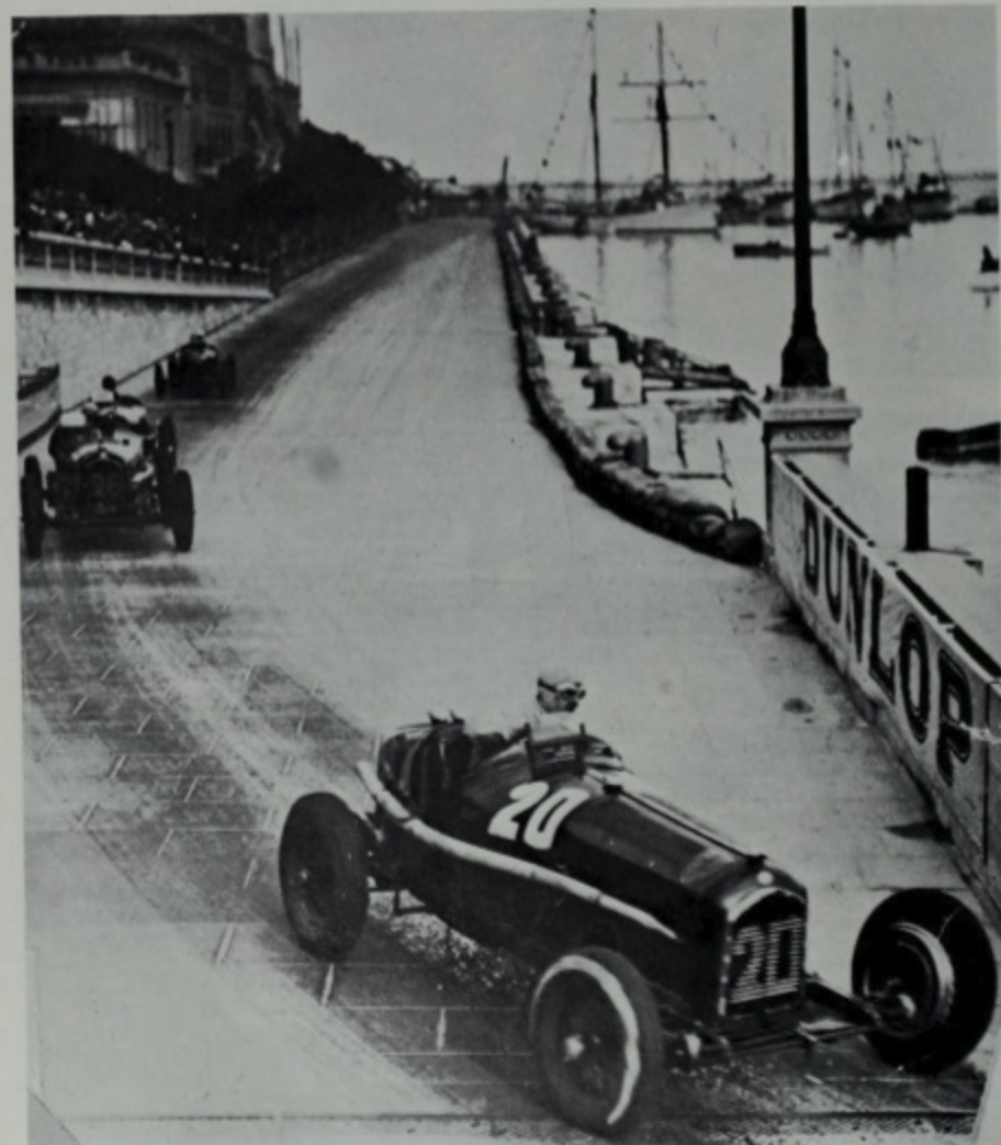
Guy Moll winning the Monaco GP in a 2.9-litre car in 1934. These 1934 Monaco cars were interim models having the wider cockpit but still retaining the low sides, whilst the apertures for the superchargers were still to be seen on the nearside
