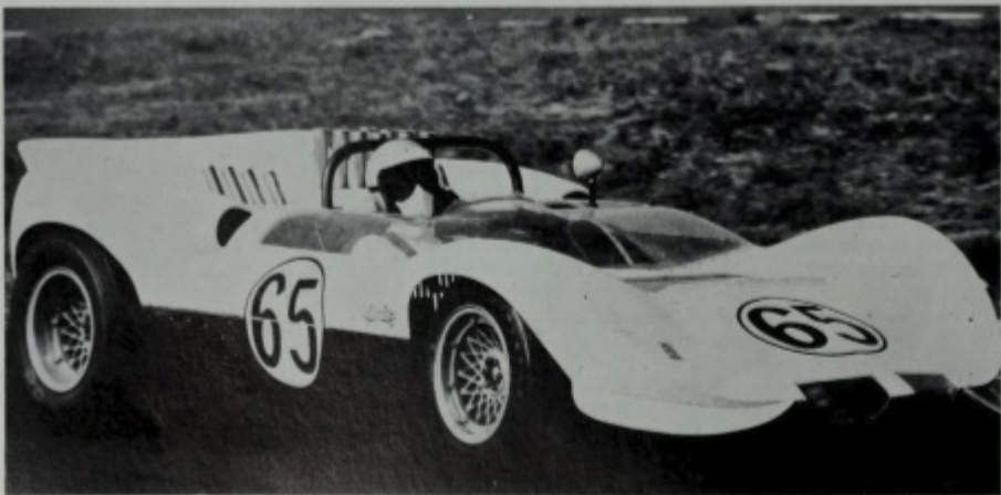
Moustaches and down-force: the car nears the end of its roofless development. By now it has its own wheels but the restless experiments with exhaust pipes continue. (Pete Lyons)
