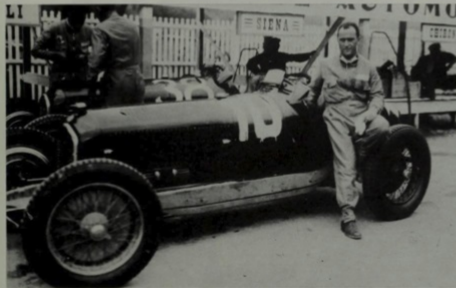
Luigi Fagioli at San Sebastian in 1933. The apertures in the bonnet side for the superchargers were a feature of the narrow-bodied 2.6-litre cars, but the very small rear brake drums used at San Sebastian were uncommon
