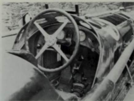
The cockpit of Brian Lewis's 2.6-litre Mannin Moar car, with the twin rev counters prominent on the dashboard
