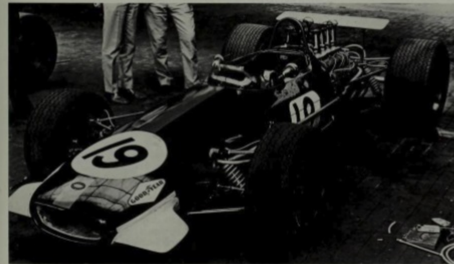
The new quad-cam Repco 860 V-8-powered BT26 for 1968 was beautifully made but had a string of problems which tended to be aggravated by the 12,000-mile gulf between racing shop and engine works. The spaceframe chassis used alloy sheet stressed skinning in place of tubular triangulation
