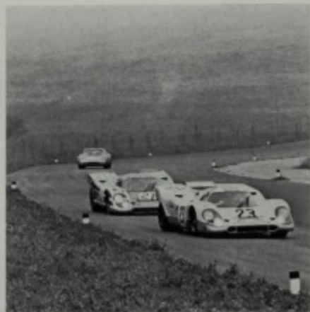
Two of a kind at Zeltweg, 1970. No 23 has the additional small rear aerofoil, first used on the John Wyer cars at Le Mans. The other car, fresh from its victory at Le Mans, has the standard 1970 short-tail, which was replaced in 1971 by the lower, finned tail. (Geoffrey Goddard)
