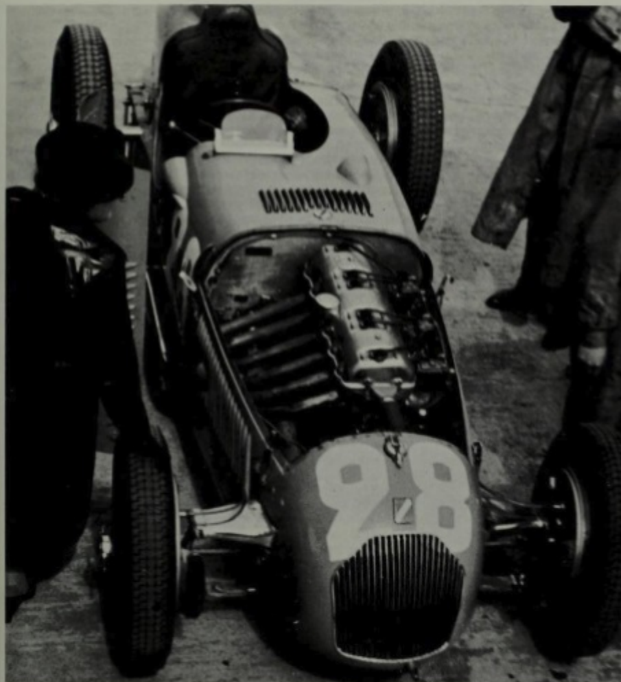
Lago forebear 2: the 4.5-litre offset GP car of 1939, showing cockpit set to the right, and the engine and transmission to the left.
