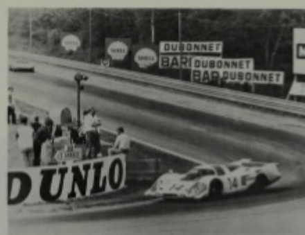
Three vintages of long-tail cars at Le Mans: 1969—No 14 of Stommelen-Ahrens cornering at Mulsanne. Note the asymmetric positions of the mobile tail flaps as the car rolls. (Geoffrey Goddard)
