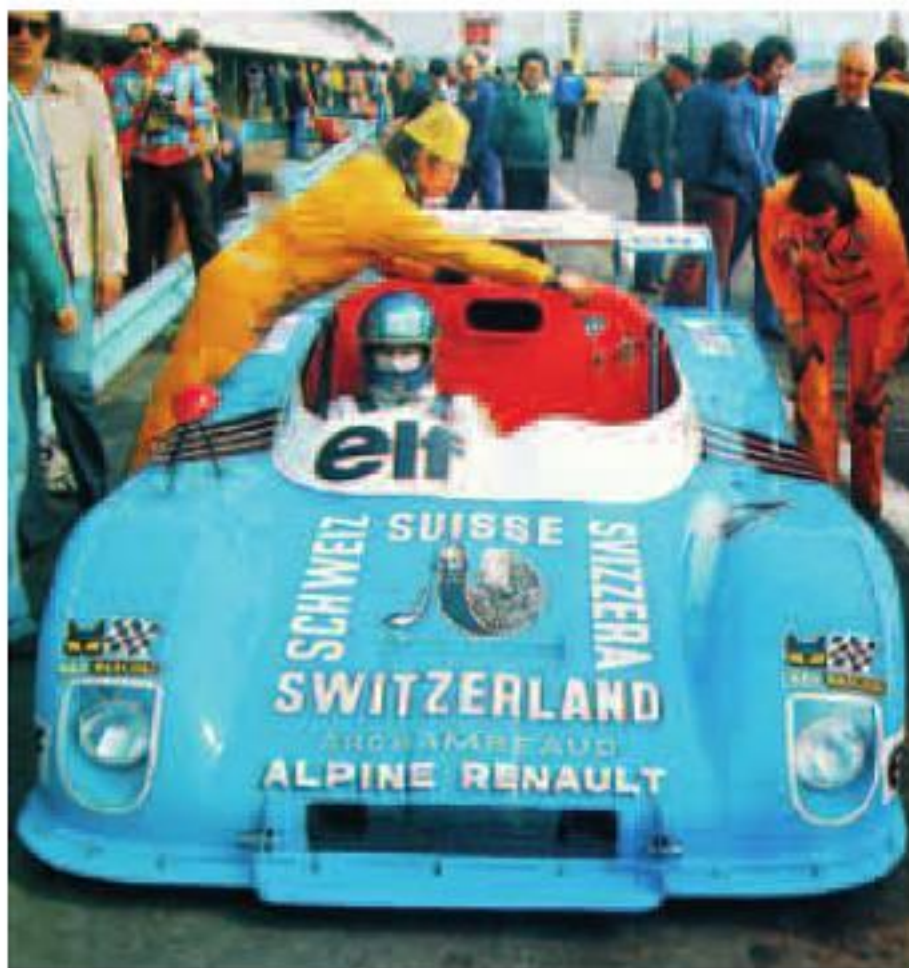
Adjustable splitter and flap for radiator air inlet on the Larrousse car. (Photo CD)
