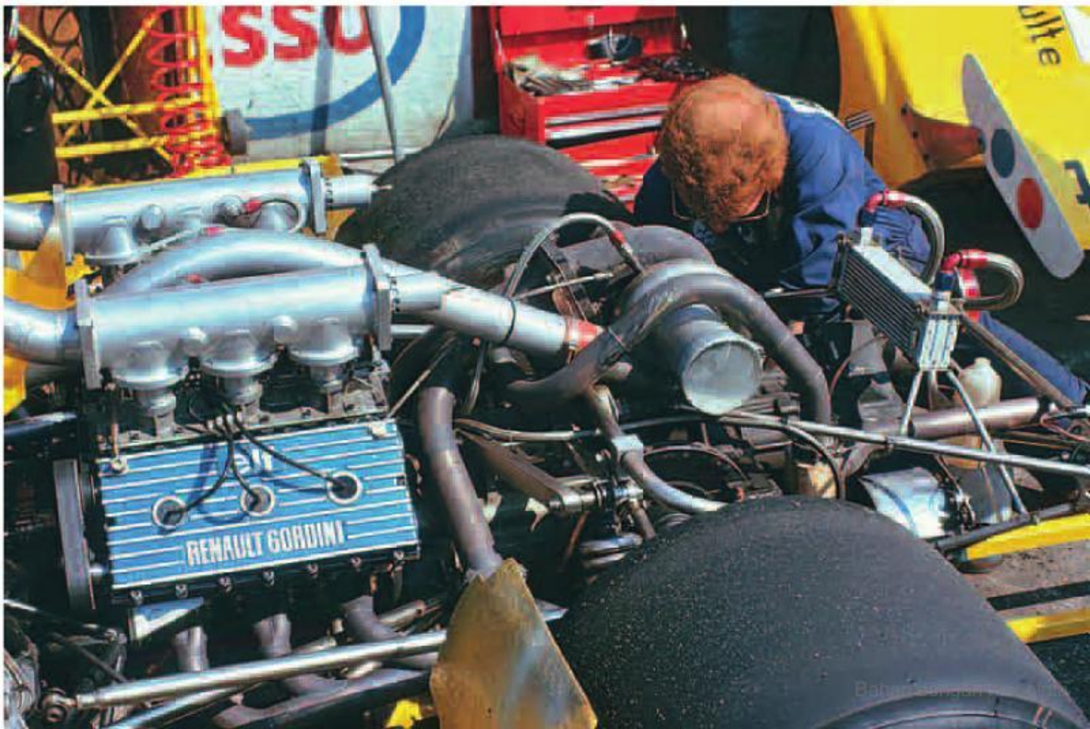
Single turbo mounted above the gearbox. (Photo AB)
