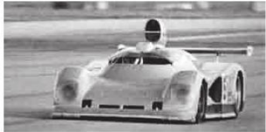
A443 – early secret test (no decals), with brush skirt and bubble. (Photo FXD)
