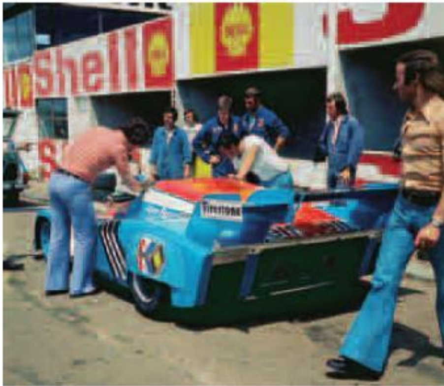
Covered rear wheels, one of many experiments. (©R)
