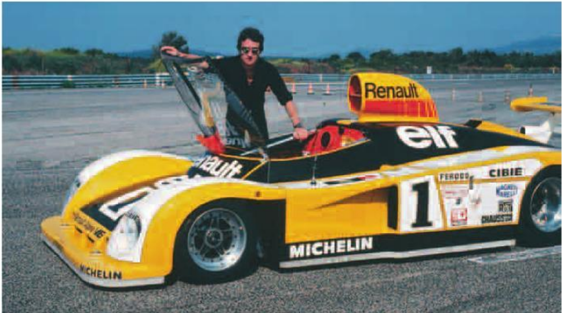
Depailler demonstrates the bubble; also visible are the brush skirts around the front and sides. (©R)
