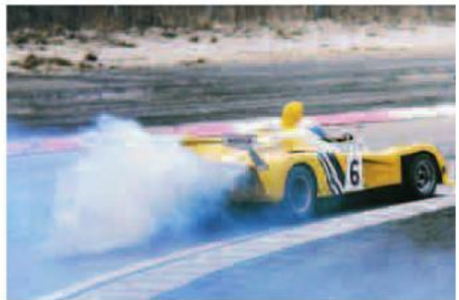
Head gasket failure. (Photo GL)
