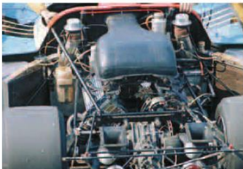
Earlier air intake point (the black unit on top of the engine) under the rear bodywork. (©R)
