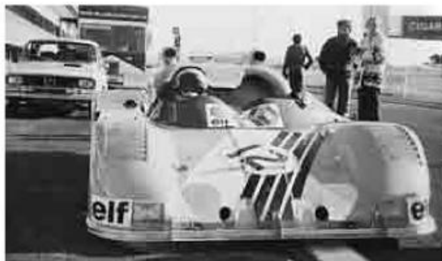
Note the air intakes on the engine cover. (Photo GL)
