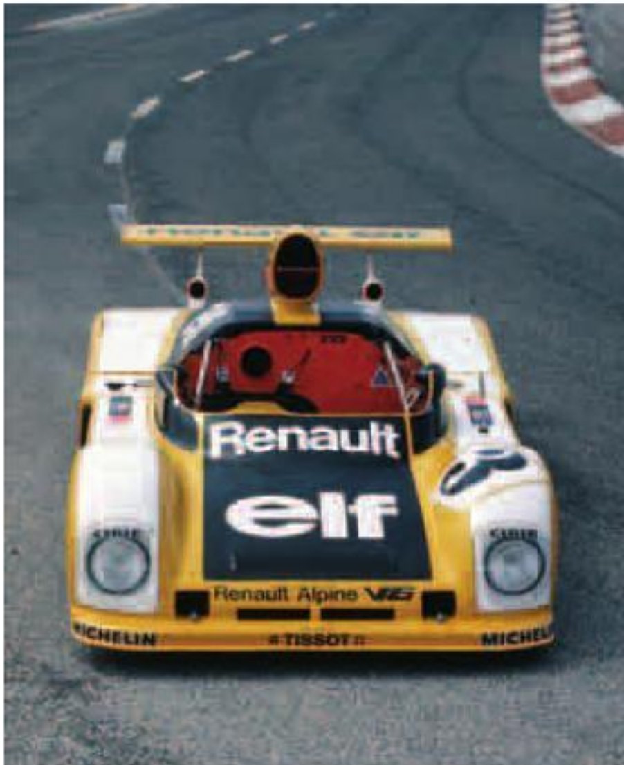
Note the air intake nacelles in the rear wing supports. (©R)
