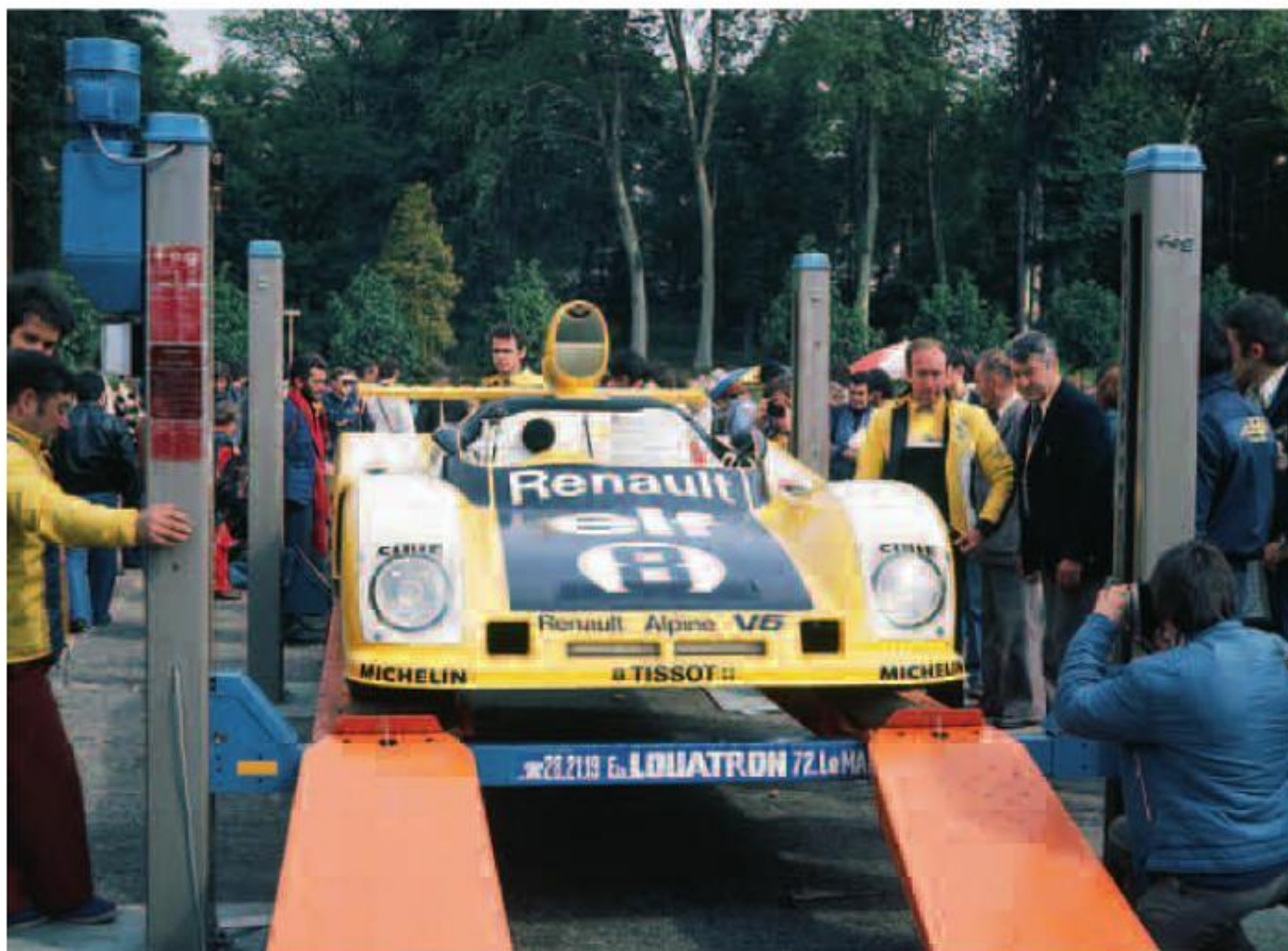
The four-post ramp for underneath checks. (©R)
