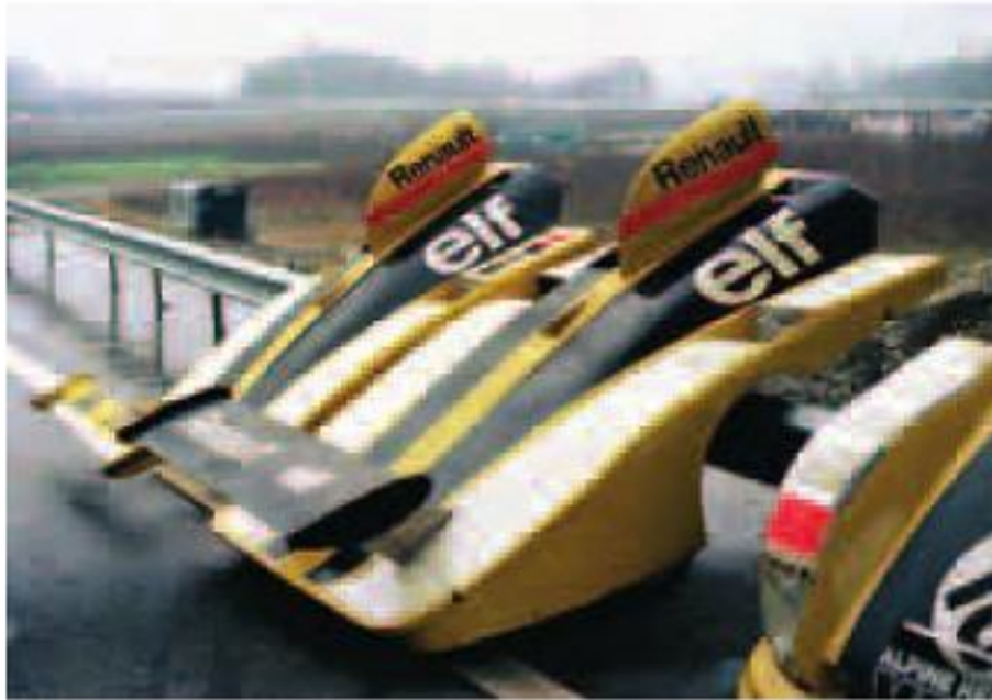
Different body panels without central strut. (Photo JC)
