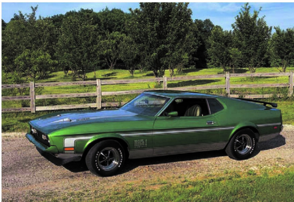
Ford's last big-block 429 Mustang appeared in 1971. From there, the top performance model was still the Mach 1, with the hottest engine option being the 351 Cleveland small-block. This '72 Mach 1 is fitted with a Cleveland V-8, as well as the optional ram-air hood.
