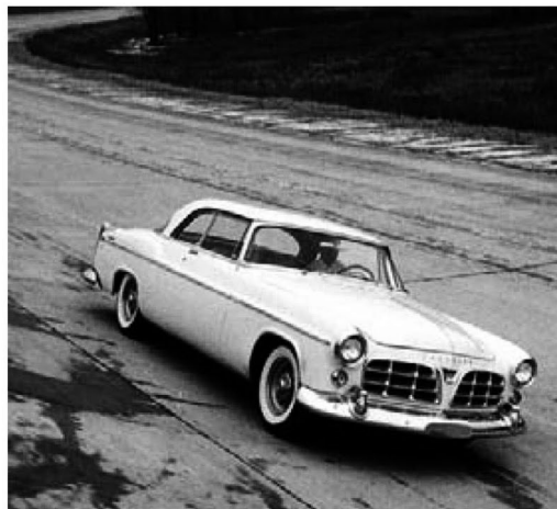
Still others believe this machine was the first true musclecar. In 1955, Chrysler combined luxury and prestige with its hot 331 hemi V-8, creating the C-300, a car named for its industry-leading horsepower figure, 300 of course. Although obviously much bigger and heavier, this beautiful brute could still run right along with Chevrolet’s sporty Corvette. Chrysler Historical Archives
