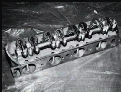
Above left: The 302 Tunnel-Port got its name from cylinder heads with pushrod tubes that ran through the intake ports. Ford Motor Company Photo
