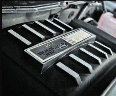
A plate at the rear of the intake manifold displays the Boss 302's VIN, with its unique "U" engine code as the eighth digit, along with the car's sequential vehicle number. John Moore/Location Imaging, courtesy Ford Racing
