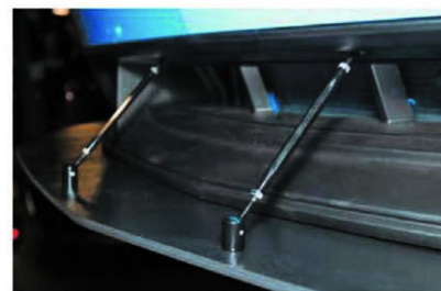
A pair of stanchions supports the Laguna Seca front splitter. To accommodate customer installation, a bracket is supplied behind the bumper cover, along with plugged holes in the cover for the stanchions to pass through. John Moore/Location Imaging, courtesy Ford Racing
