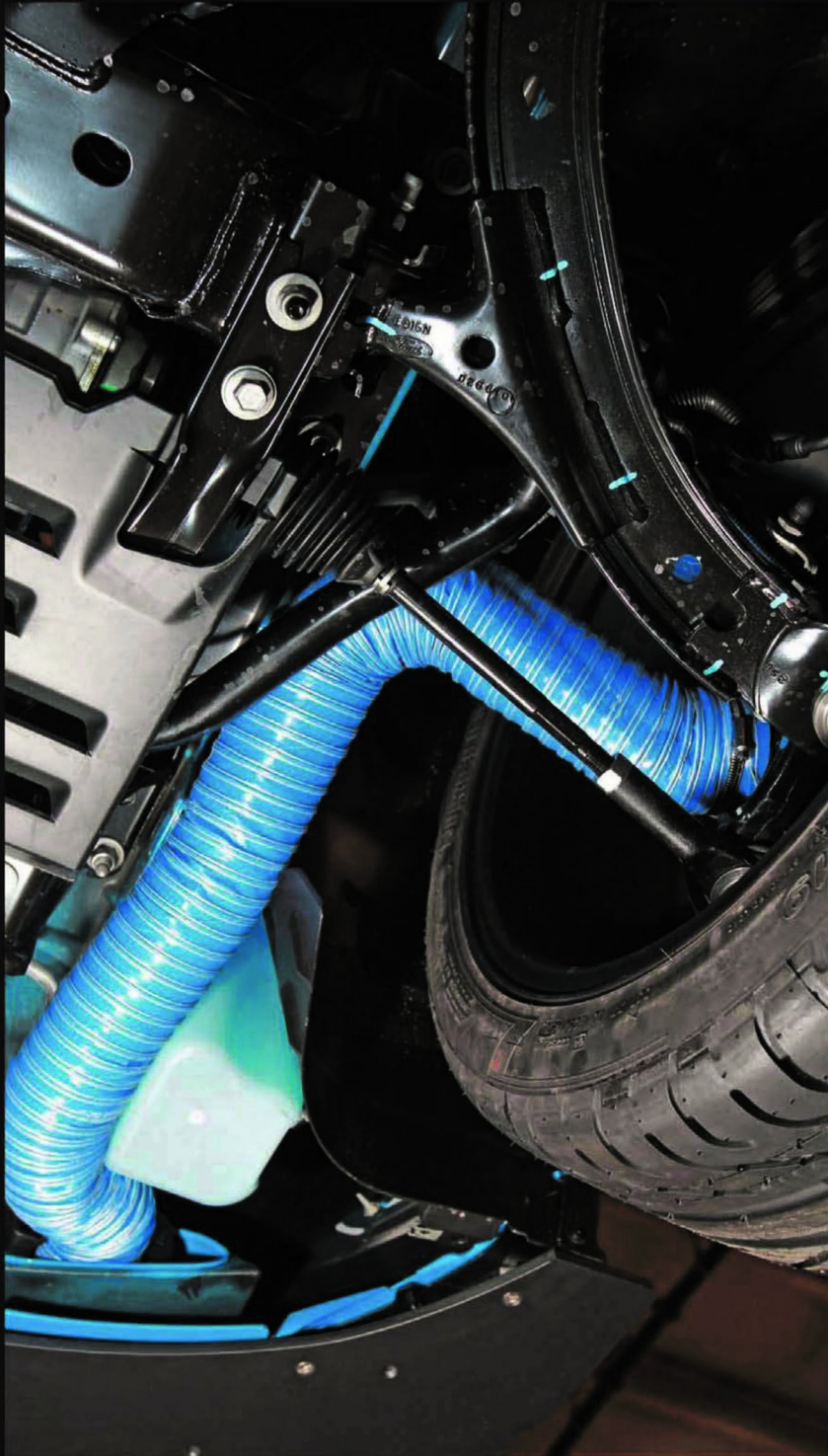
Functional Ford Racing brake ducts keep the Laguna Seca's front rotors cool under competition conditions. Supplied with the car for installation by the dealer, the ducts draw air from the openings at each corner of the lower front fascia. John Moore/Location Imaging, courtesy Ford Racing
