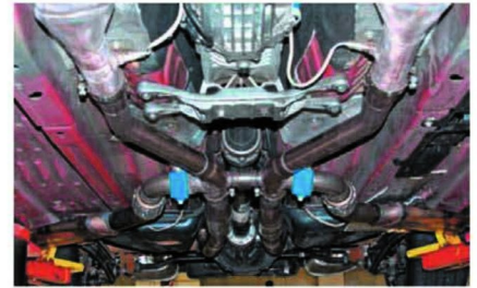
The quad exhaust system became a unique sound package for the Boss 302. Sidepipes split off from the main exhaust system to envelop the driver in exhaust tone. On this prototype, you can see the valve fixtures in blue. At this point, before orifice plates were designed, they had manual set-screw adjustment. Shawn Carney/Ford Motor Company Photo
