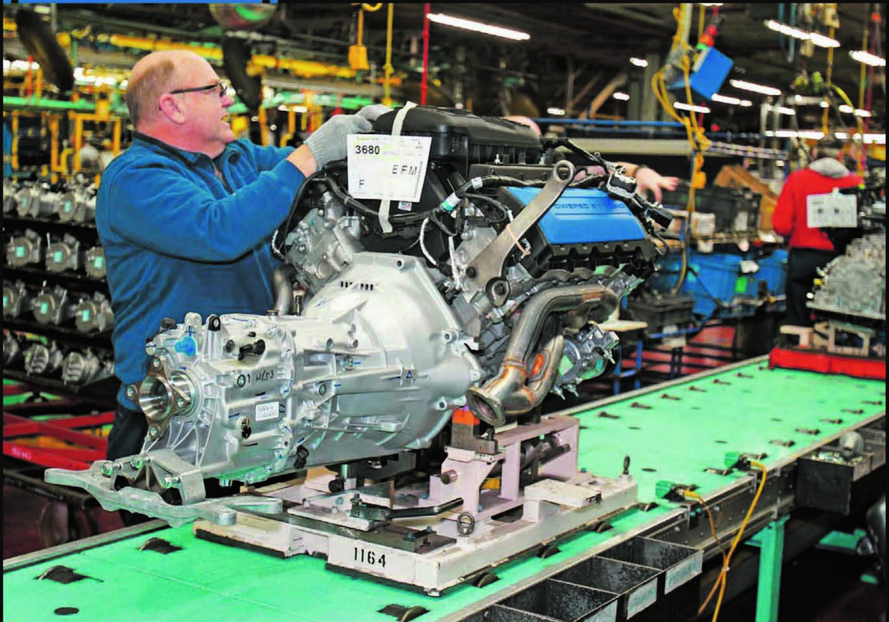
After the installation of a special race-inspired clutch, the six-speed manual transmission is mated to the Boss 302 as it makes its way to the vehicle assembly line. John Moore/Location Imaging, courtesy Ford Racing
