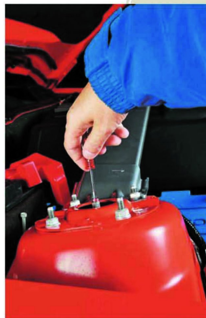
With manually adjustable struts and shocks, driver interaction is needed to change the setting from 1 (soft) to 5 for all-out track driving. John Moore/Location Imaging, courtesy Ford Racing
