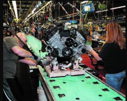
Boss 302 engines are built at Ford's Essex Engine Plant in Windsor, Ontario, Canada, then shipped across the river to Mustang's AAI assembly plant, where they receive their blue cam covers and other final dress before installation in the U-code Boss 302s. John Moore/Location Imaging, courtesy Ford Racing
