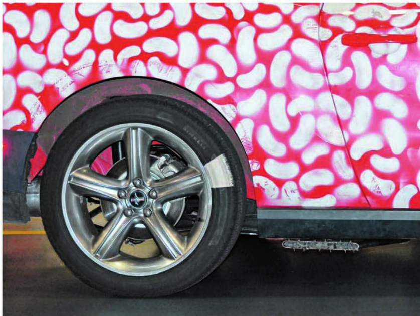
An early demo of the quad exhaust system used NASCAR-type sidepipes with steel wool stuffed inside for noise control. Note the "cow print" camouflage on this red Mustang, which was eventually equipped with a Boss 302 engine for NVH development work. Shawn Carney/Ford Motor Company Photo
