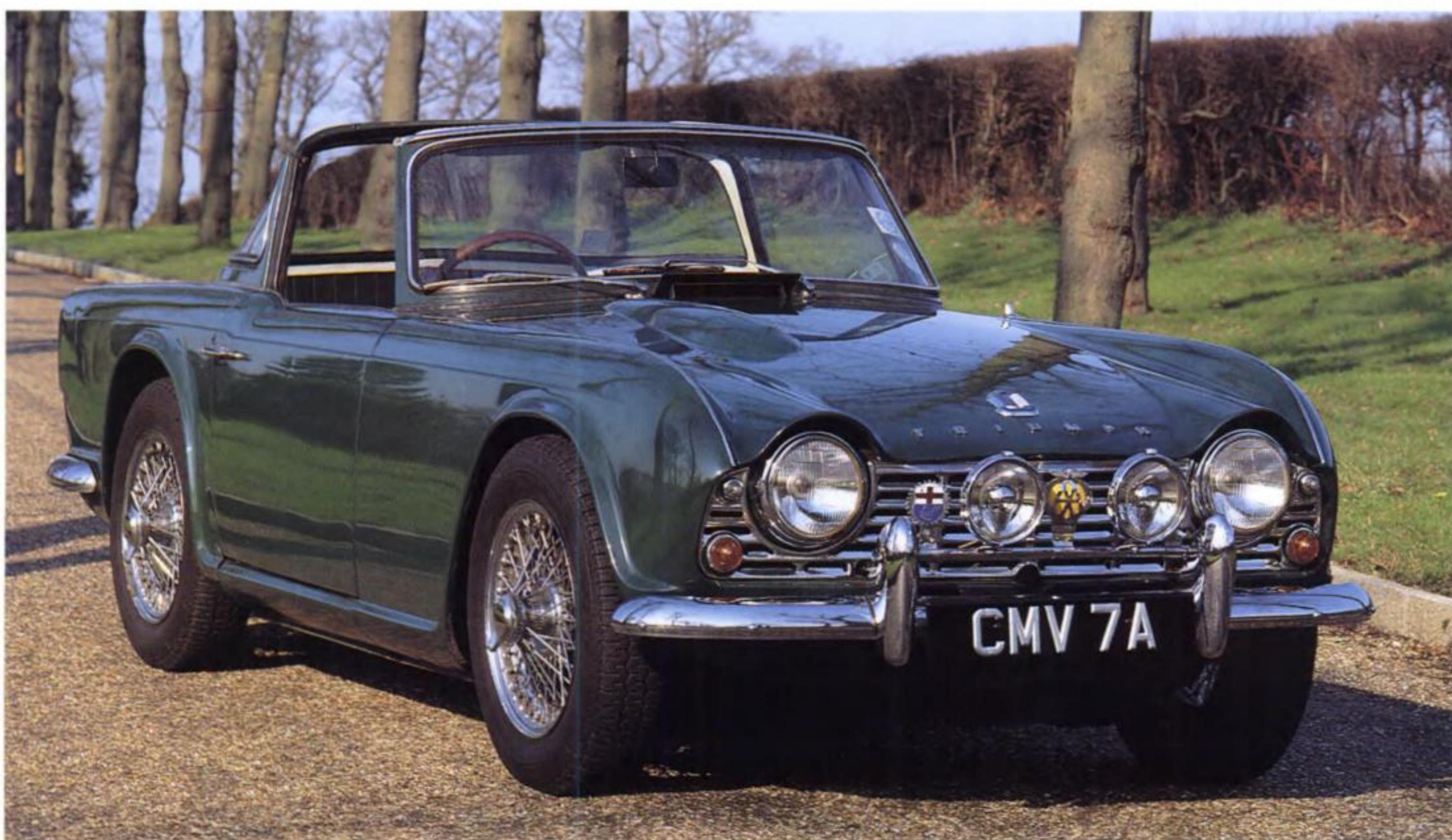
The Triumph TRs were robust and honest sports cars, which steadily became more refined. This TR4 has a modified TR3 chassis carrying a body designed by Michelotti. It was the first TR to have wind-up
