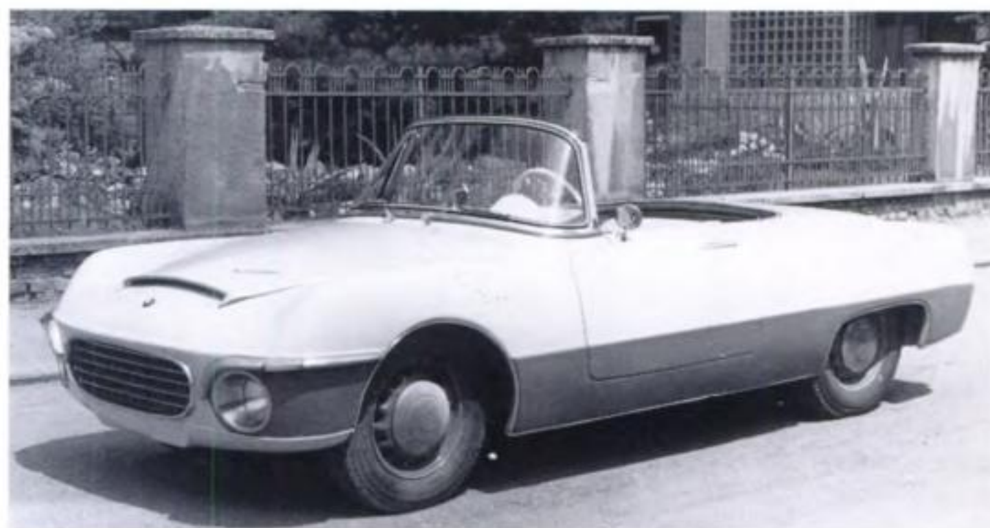
One of two 1100cc Skoda 440s fitted with fibreglass bodies (by Karosa) in 1956 for national rallies
