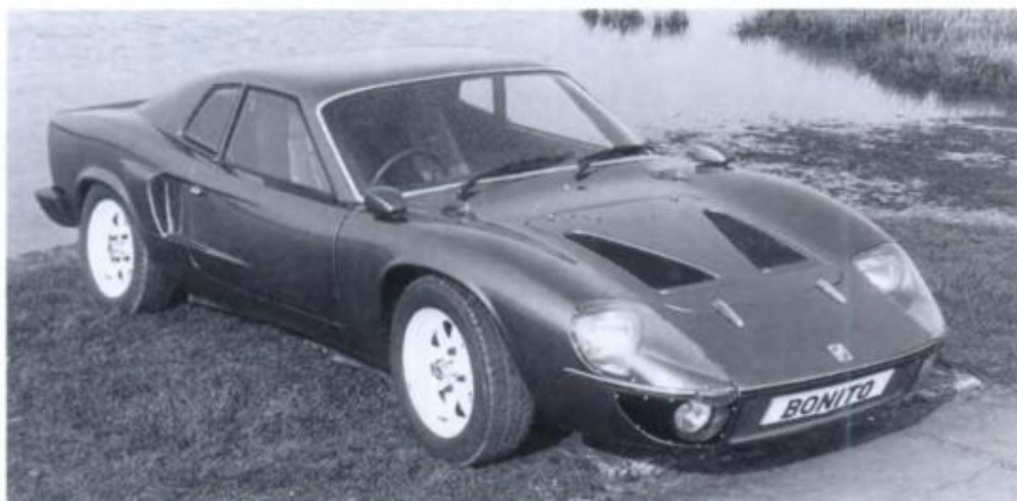
ACM Bonito was based on VW chassis
