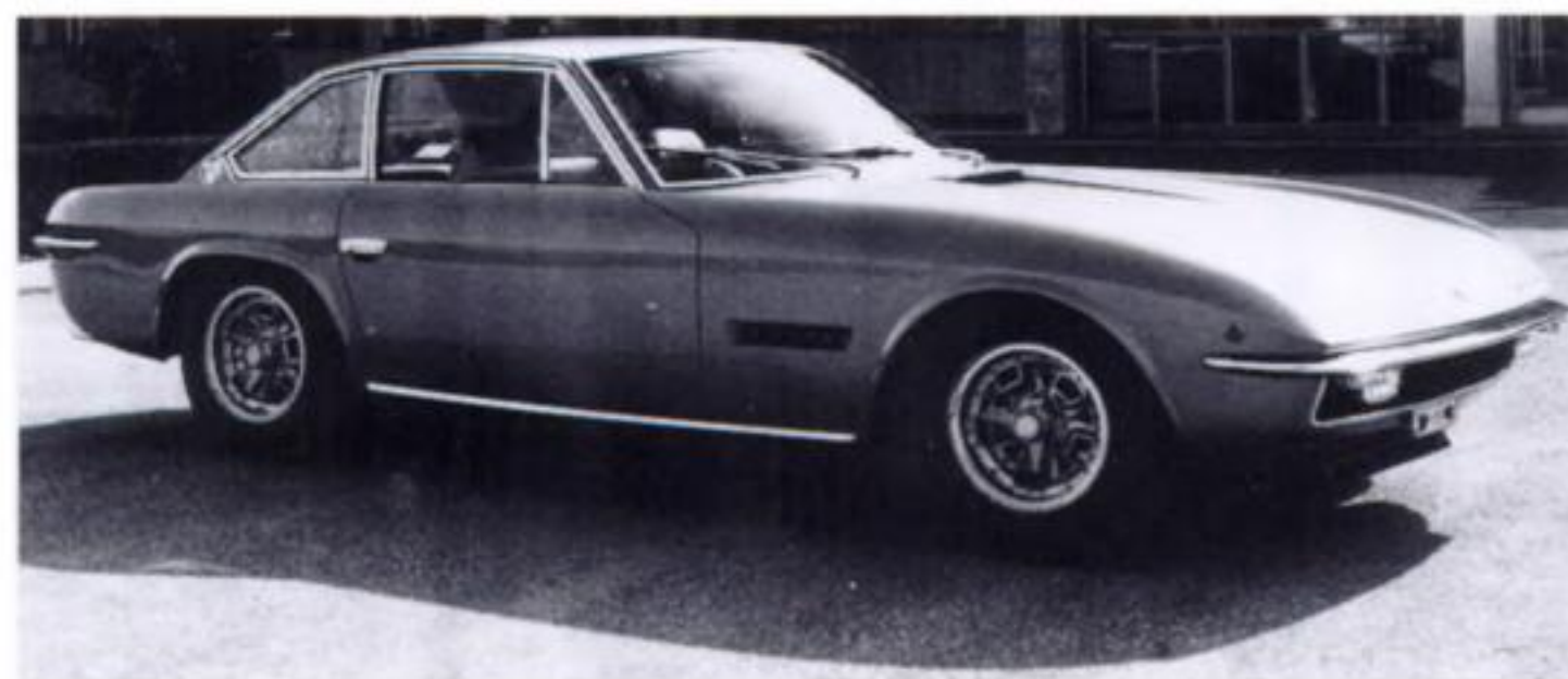
Islero had retractable headlights
