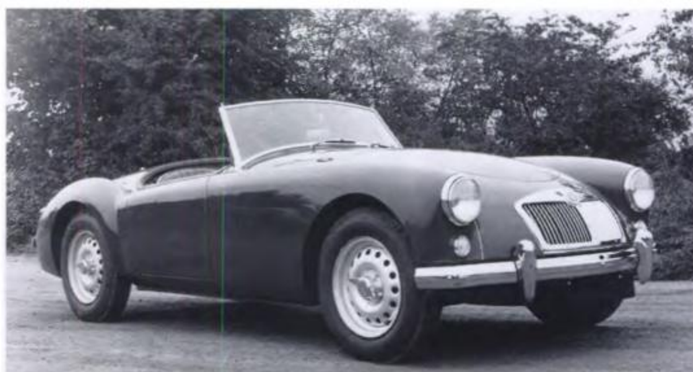
MGA Twin Cam had centre-lock wheels
