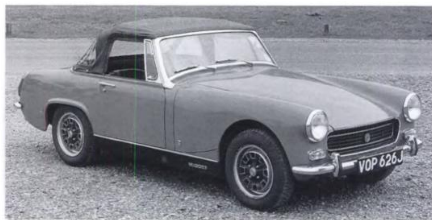
1971 Midget MkIV (above) had squared rear wheel arches. From 1972 they were rounded (below)
