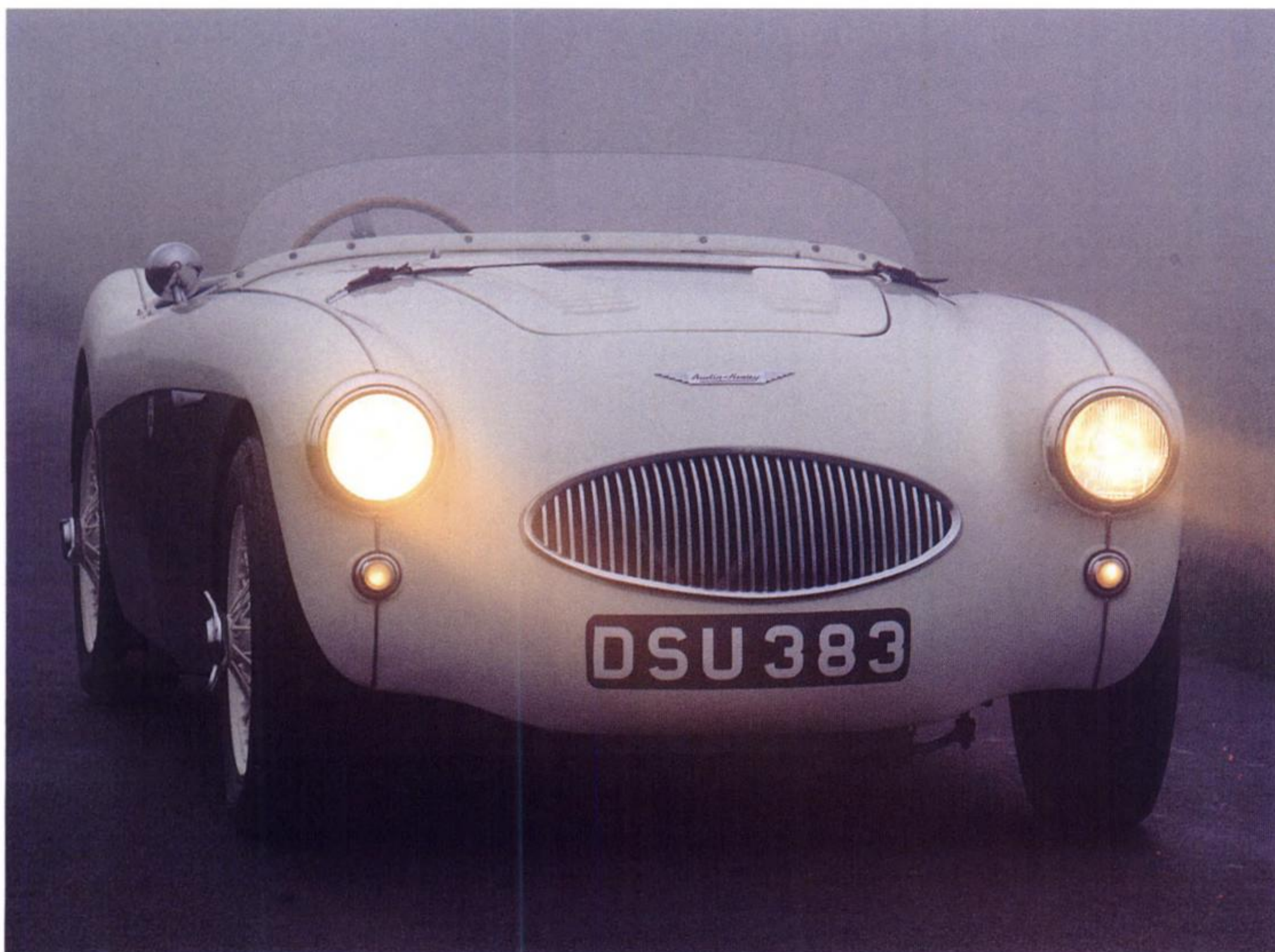
Low Perspex screen and lack of embellishments such as bumpers hint at the competitions intentions for the Austin-Healey 100S. The bonnet strap is almost anachronistic, a large fuel filler cap behind the cockpit was in character, as were the bonnet louvres and the omission of hood and side screens
