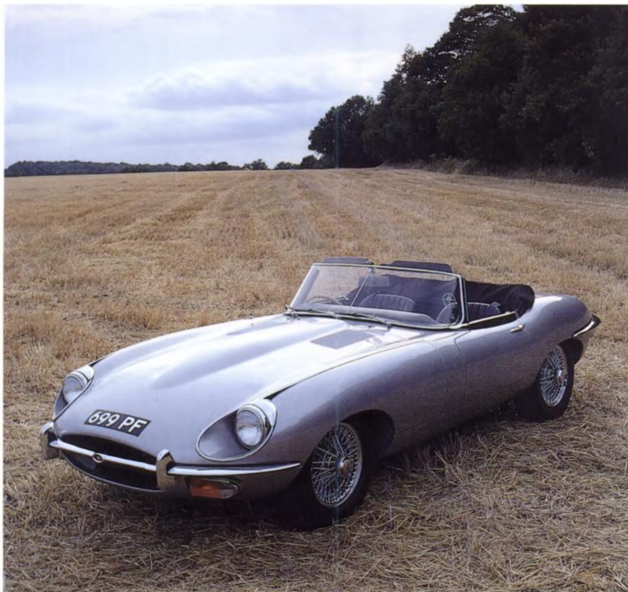
Jaguar's E-type, on the other hand, was in the forefront of a new sports car generation. This is a Series 2 roadster with the classic twin-ohc straight six in 4.2-litre form
