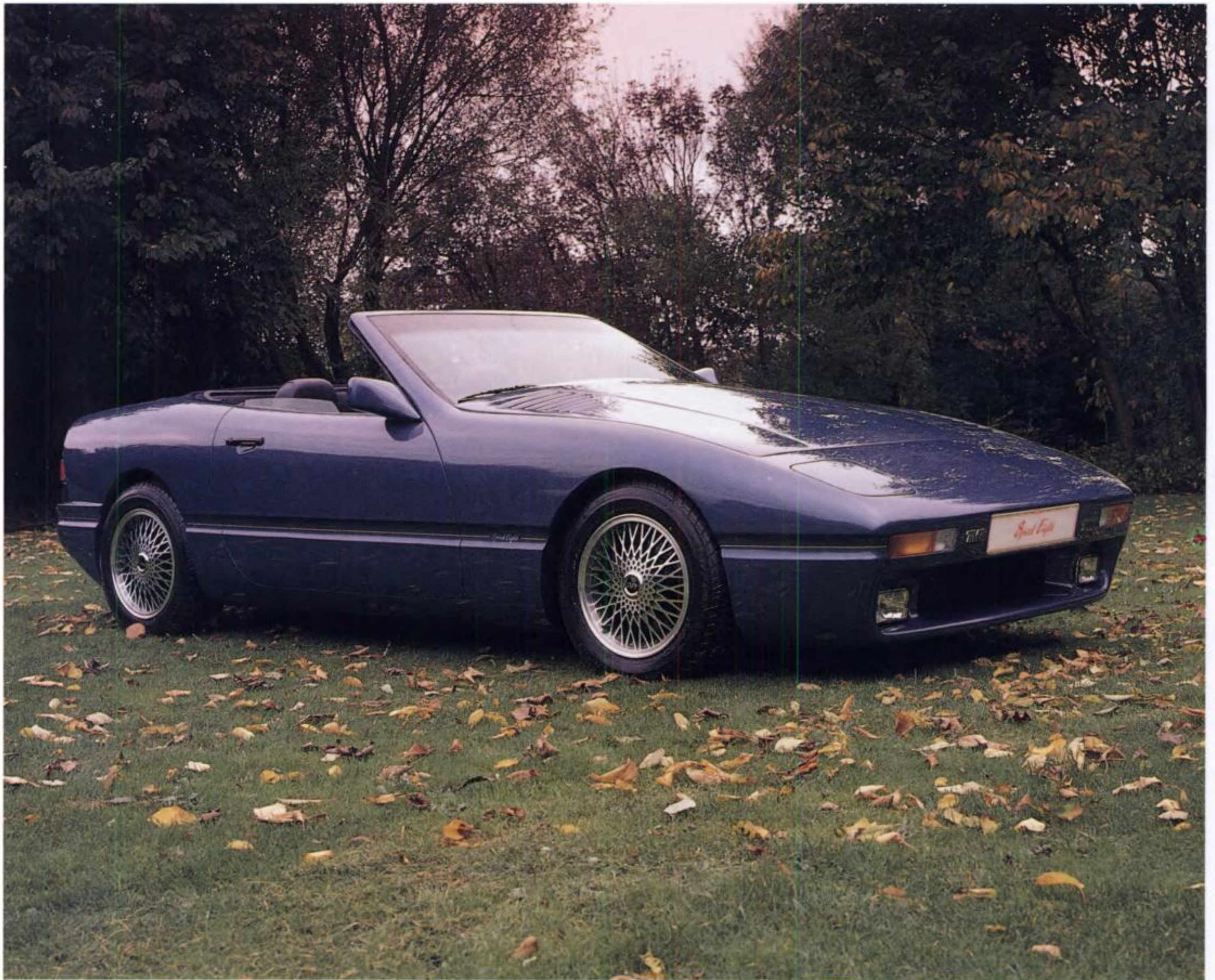
TVR has built cars in an old tradition for more than forty years. Generally the pattern has been two-seaters with front-mounted engines and backbone space frames that do tend to restrict cockpit space. This is a Speed Eight from 1989
