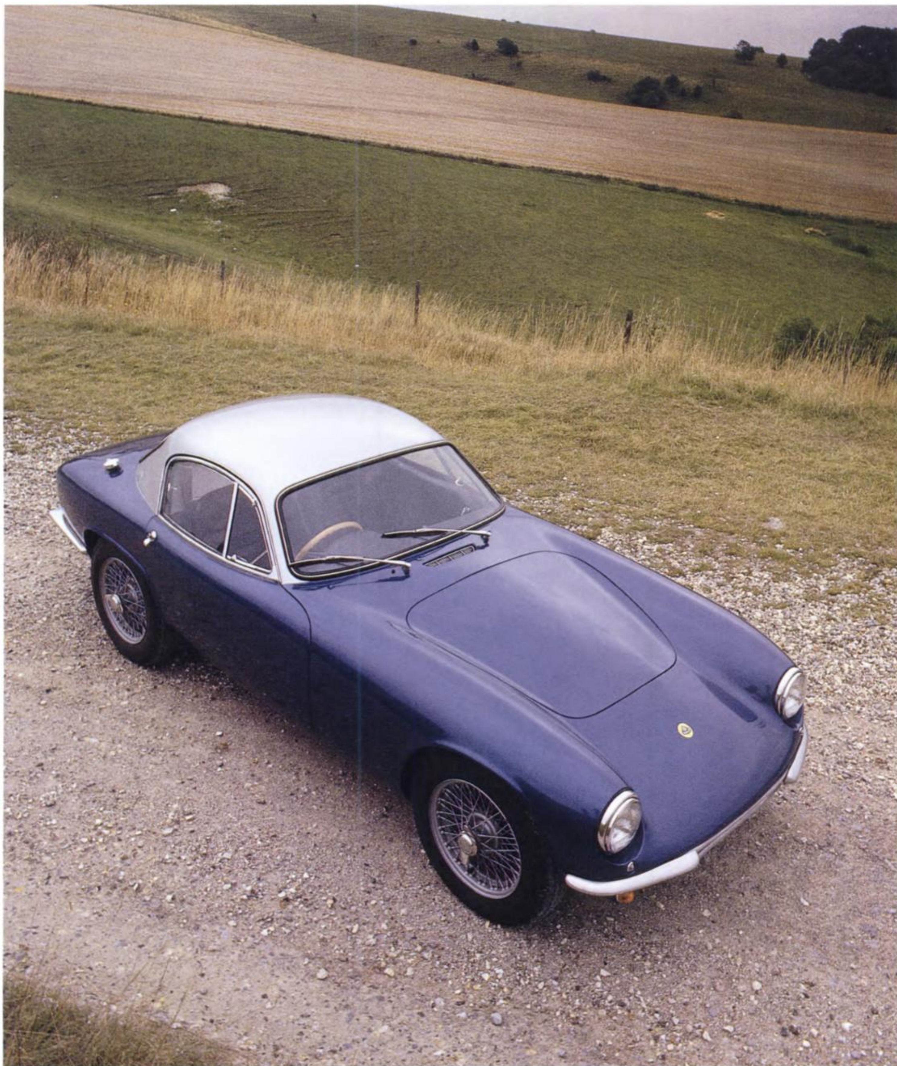
The Lotus Elite of 1957-63 had a drag coefficient of 0.29 to confirm visual impressions of aerodynamic efficiency. That figure was seldom matched 30 years later
