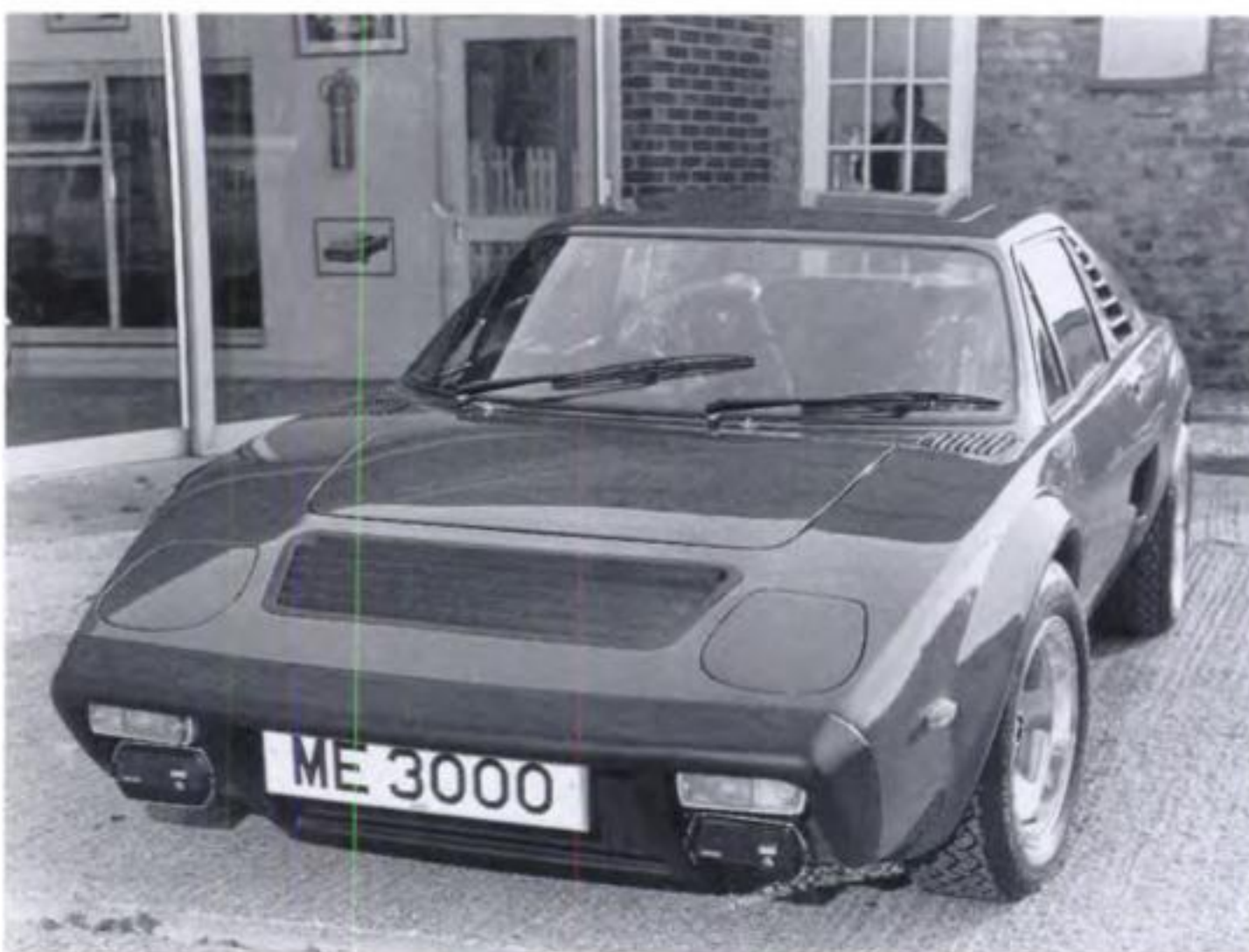
AC 3000 ME had Ford V6 mid-mounted engine
