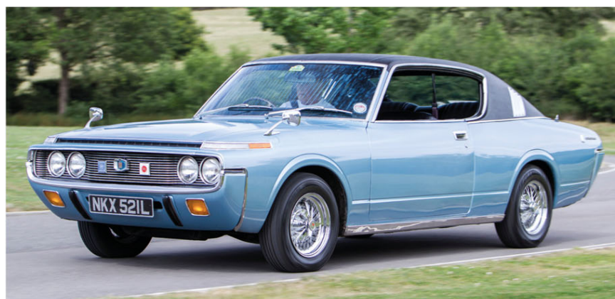
Toyota Crown Hardtop Coupe, 1971 Designed for the 1970s, the Crown followed US styling trends; the power unit was a 2.6-litre straight six.
