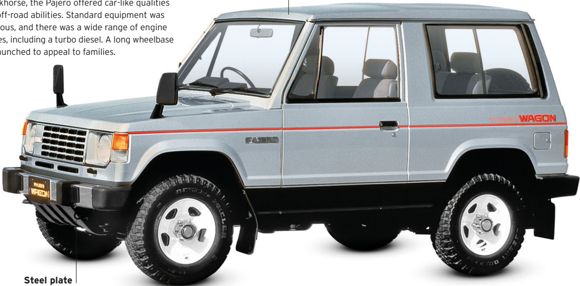
Steel plate protects engine and gearbox
