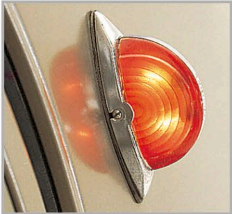
Simple signalling Indicators were added to the rear pillars in the 1950s. An ingenious innovation, they could be seen from the front and the rear in this position, which meant that only two were needed. Simplicity was key to the design of the 2CV.
