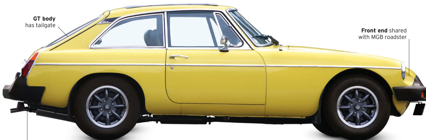
Impact-resistant polyurethane bumpers introduced in 1974
