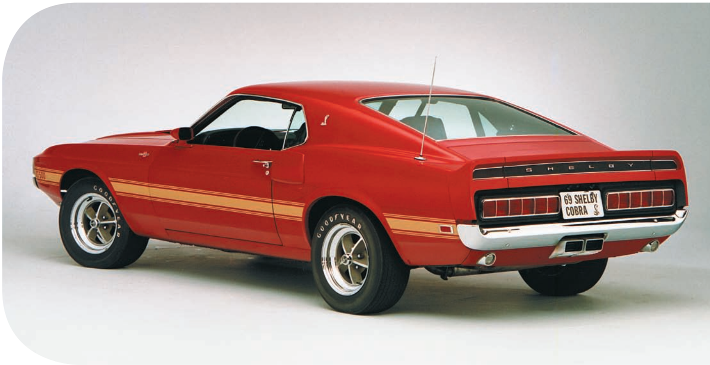
A fiberglass deck lid, rear panel, and quarter panel caps gave the 1969 Shelby its own look, along with Thunderbird taillights and a center-mounted exhaust port. Ford Motor Company
