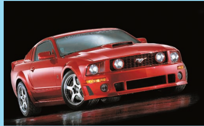
Roush Performance favored the muscle car look for its twist on the S197. The top-of-the-line Stage 3 added a ROUSHcharger supercharger to the new three-valve 4.6-liter for 415 horsepower. Roush Performance
