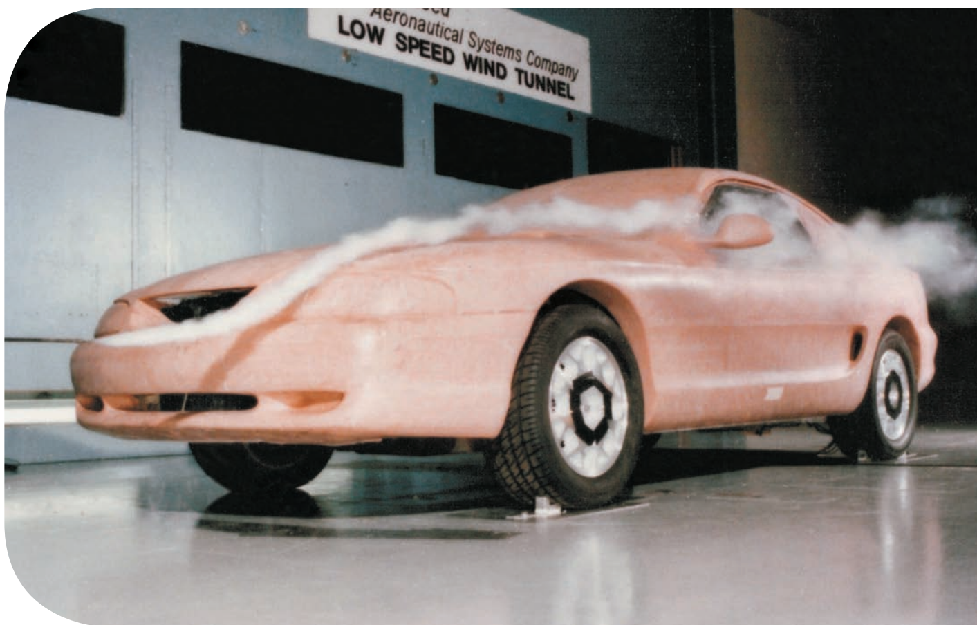
A 3/4-scale version of the SN-95 was used at Lockheed's wind tunnel to fine-tune the final body shape for optimum aerodynamics. Ford Motor Company
