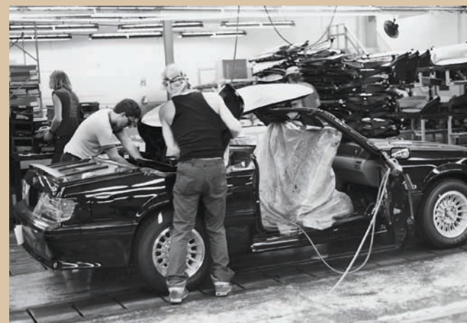
Convertibles topped hardtop sales from 1990 to 1993, but they didn't roll off the Dearborn assembly line with their ragtops. Ford sent hardtop Mustangs without roofs to Cars and Concepts near Brighton, Michigan, for installation of the convertible tops. C&C also handled the T-top conversions. Source Interlink Media
