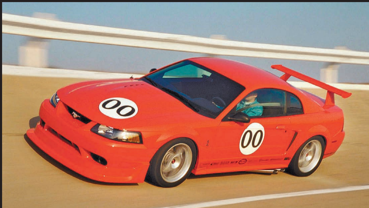
With a 5.4-liter V-8 and a wild rear wing, SVT's 2000 Cobra R was a "boy racer" that immediately set a new standard for a production Mustang. Ford Motor Company
