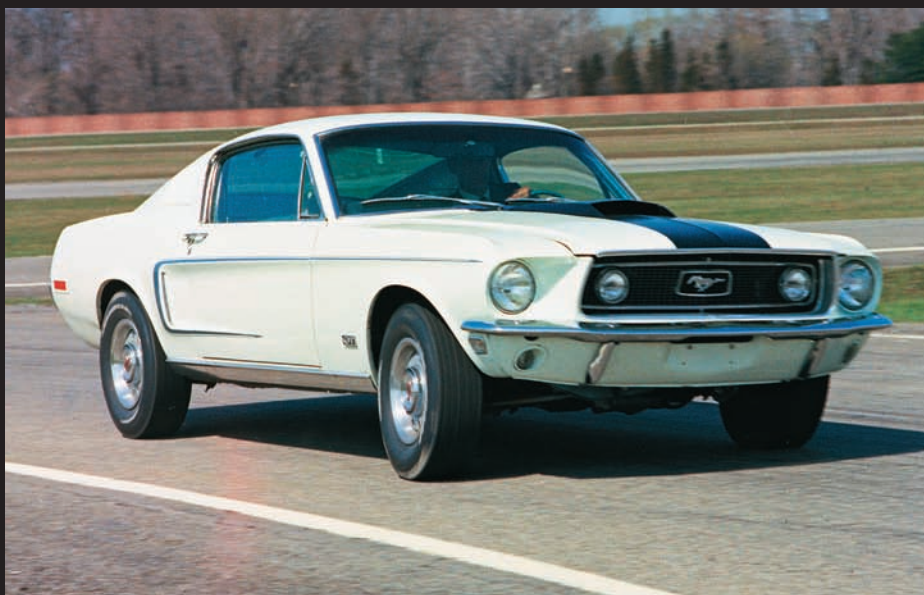
Rated at 335 horsepower, the 428 Cobra Jet utilized many of Tasca Ford's KR-8 modifications. For the first time, the hood scoop was functional thanks to a special air cleaner with a vacuum-operated flap that allowed cooler outside air into the carburetor under full throttle. Ford Motor Company
