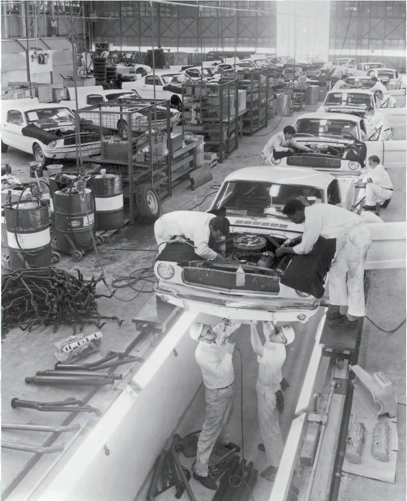
In early 1965, Shelby American moved into a pair of hangars adjacent to the Los Angeles airport where Mustangs rolled along an assembly line with an underground pit so they could be converted into GT350s. Shelby American
