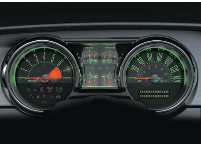
Another new technology was more aesthetic than functional. With the optional MyColor instrument cluster, drivers could personalize their instrument cluster background to any one of 125 colors. Ford Motor Company
