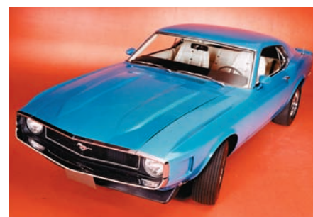
At Ford, the Quarter Horse concept was known as the composite Mustang because it used parts and pieces from several car lines. The formula was simple: take a Mustang SportsRoof and mix in a Cougar instrument panel, hood and front fenders from the Shelby, and Boss 429 engine. Ford Motor Company
