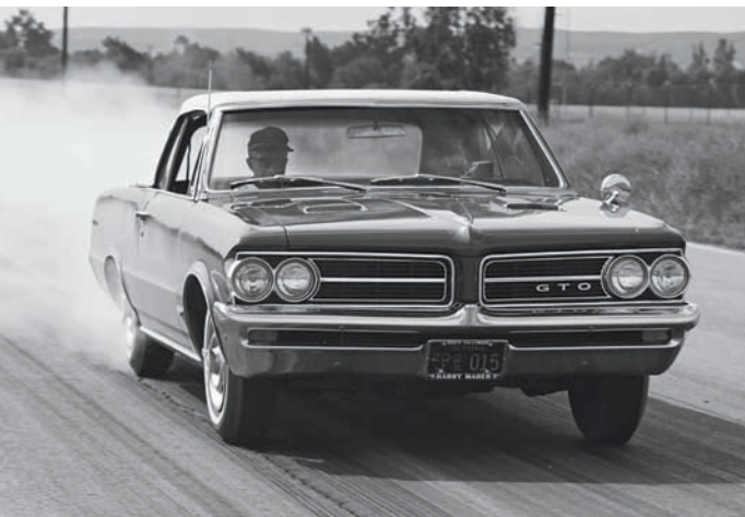
Pontiac triggered the muscle car market with its GTO option for the 1964 Tempest, powered by a 389 V-8 with available Tri-Power induction. Identified as a compact or intermediate car with a big V-8 engine, the muscle car would power the American performance car industry for the next seven years. Source Interlink Media
