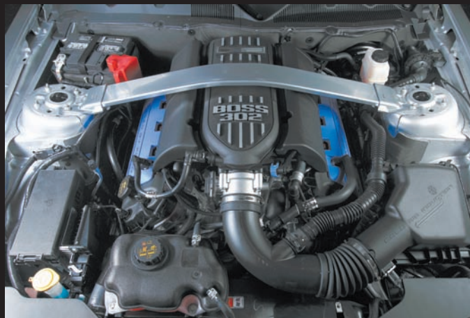
A short-runner-in-a-box intake manifold was the key to the Boss 302’s high-revving 444 horsepower. Ford Motor Company
