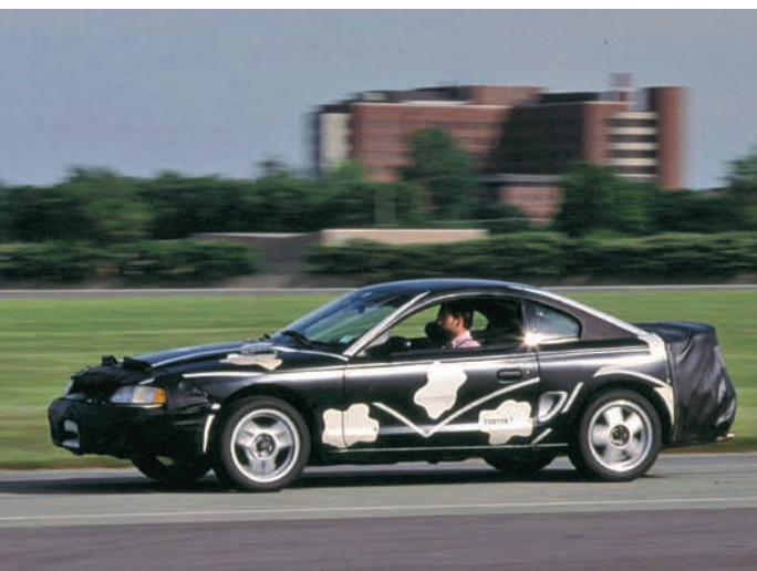
The SN-95 Mustang was subjected to extensive testing to meet the goals for ride and handling. This disguised mule was named Cooter after the mechanic in the TV show Dukes of Hazzard . Ron Sessions
