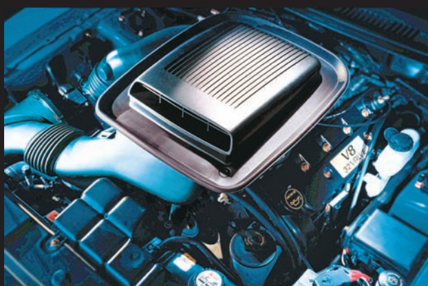
The 2003 Mach 1's most distinctive feature was its Shaker hood scoop, a functional Ram-Air unit that recalled the Cobra Jet Mach 1s from 1969 to 1970. Ford Motor Company
