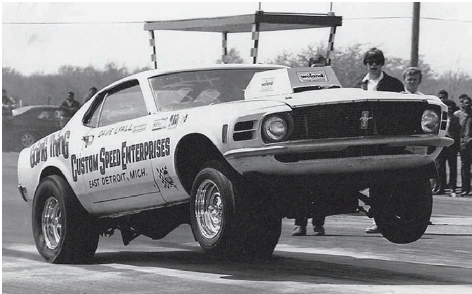
In response to altered-wheelbase Chryslers, Ford Drag Council leader Dick Brannan asked Holman-Moody to build a Mustang with a longer wheelbase and set-back engine. It is often recognized as the first Funny Car. Source Interlink Media
