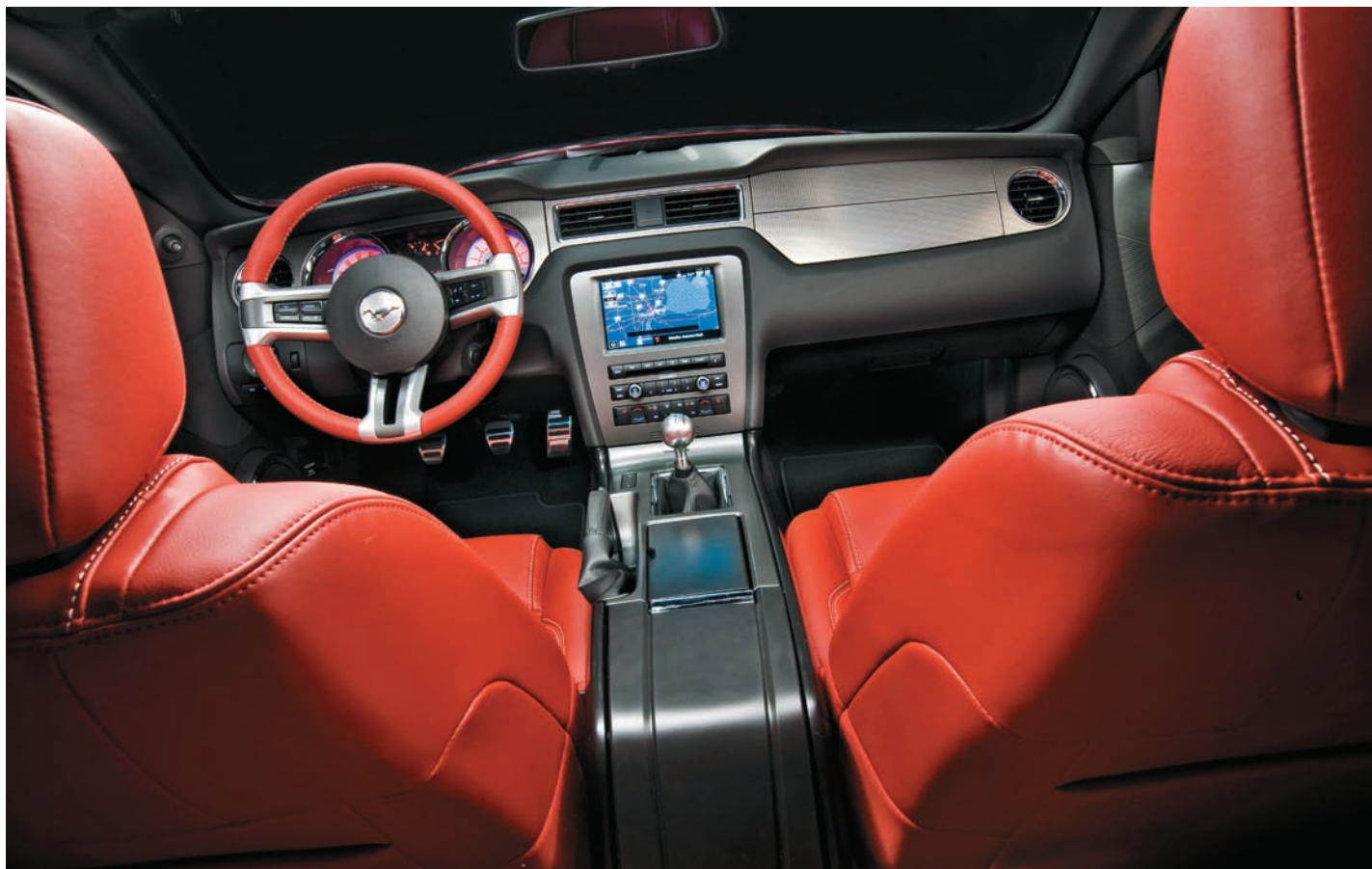
The 2010 Mustang interior was updated with new materials, genuine aluminum panels, and a one-piece instrument panel that flowed into a center stack for Ford's SYNC communications and entertainment system. Ford Motor Company
