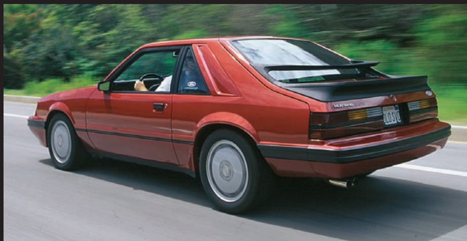
Aerodynamics played a large role in the SVO's performance and appearance, including the Mustang's first and only dual-plane rear spoiler. Ford Motor Company
