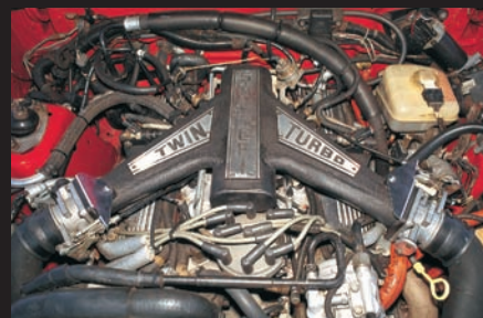
To power his 25th Anniversary Mustang, Roush replaced the 5.0-liter with a 351 and bolted on a pair of turbochargers from the Thunderbird turbo coupe. Source Interlink Media
