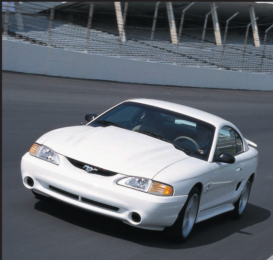
Like the earlier 1993 model, the 1995 Cobra R was built for the racetrack. With a 351 engine, a taller cowl-induction fiberglass hood was part of the package. Source Interlink Media
