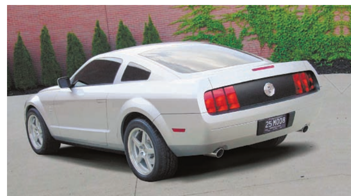
The S197 design evolved into a roofline with side windows in the C-pillar, similar to the 1966 Shelby, and a rear panel with triple-lens taillights and a faux cap to evoke the center-mounted fuel filler used from 1965 to 1973. Ford Motor Company
