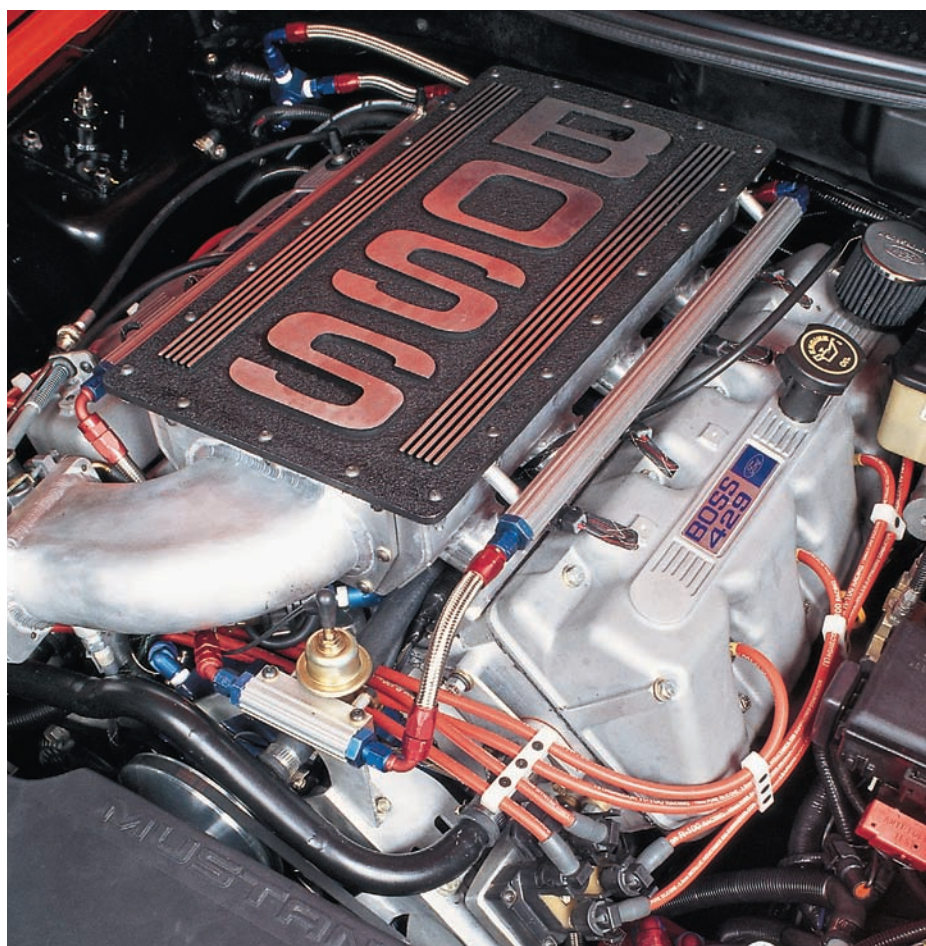
Roush Racing built the 604-cubic-inch Boss 429 engine for the Boss SN-95 Mustang. Tom Wilson
