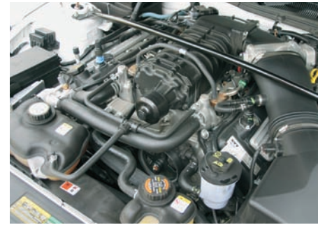
SVT's Shelby GT500 was powered by a 32-valve 5.4-liter V-8, the largest displacement for a regular production Mustang engine since 1973. Supercharging boosted output to 500 horsepower. Donald Farr
