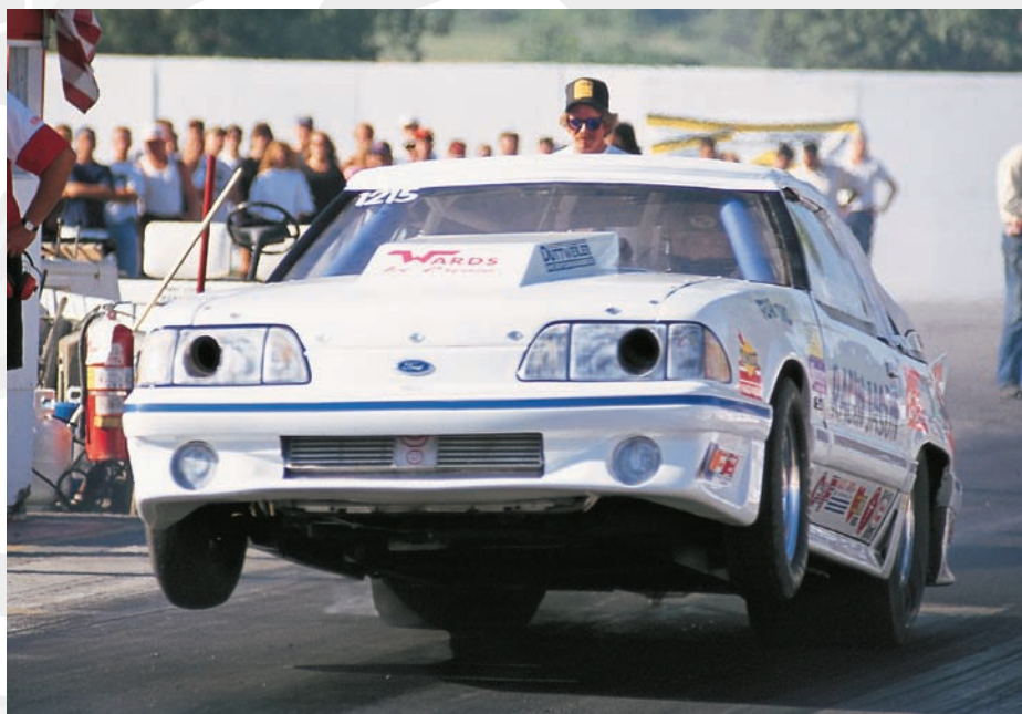
By the mid-1990s, drag racing 5.0-liter Mustangs had progressed from modified street cars to all-out race cars. In 1996, "Racin' Jason" Betwarda campaigned the "World's Fastest 5.0" with hired gun Mike Ragusa behind the wheel and a twin-turbocharged Duttweiler performance engine under the hood. The convertible routinely ran high seven-second ETs at 185 miles per hour. Donald Farr
