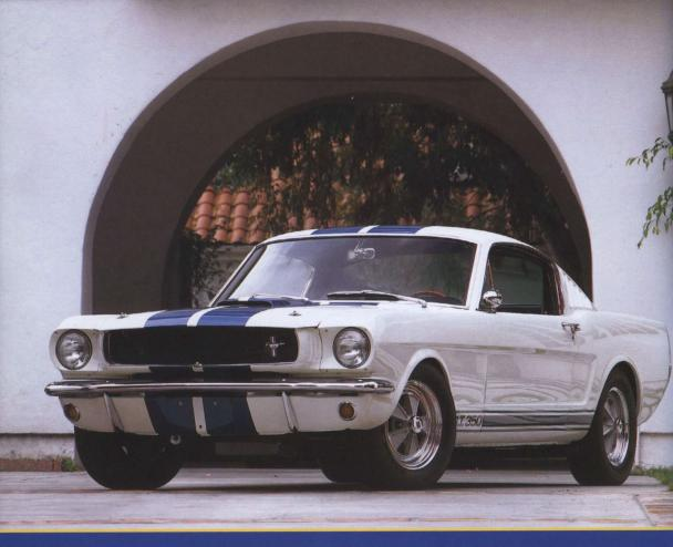
At Ford's request, Carroll Shelby of Cobra sports-car fame created a high-performance Mustang fastback. Called GT-350, it deleted the rear seat to save weight and included a 306-hp V-8.
