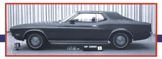
A near-flat rear roofline marked '71 SportsRoof fastbacks (above left). Hardtops got a swoopy "tunnelback" treatment with inset rear window.
