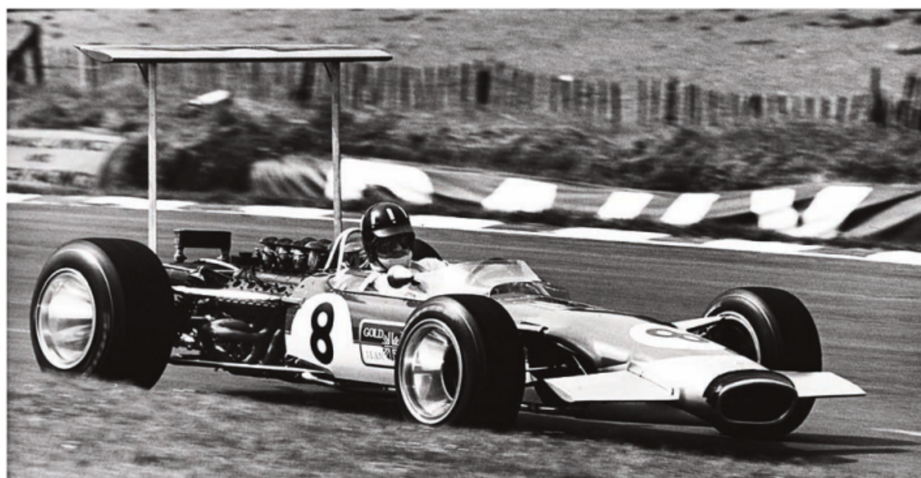
Graham Hill behind the wheel of Lotus 49B, chassis number R6, in one of its many iterations: nose fins and a tall aerofoil mounted to the rear suspension. Classic Team Lotus
