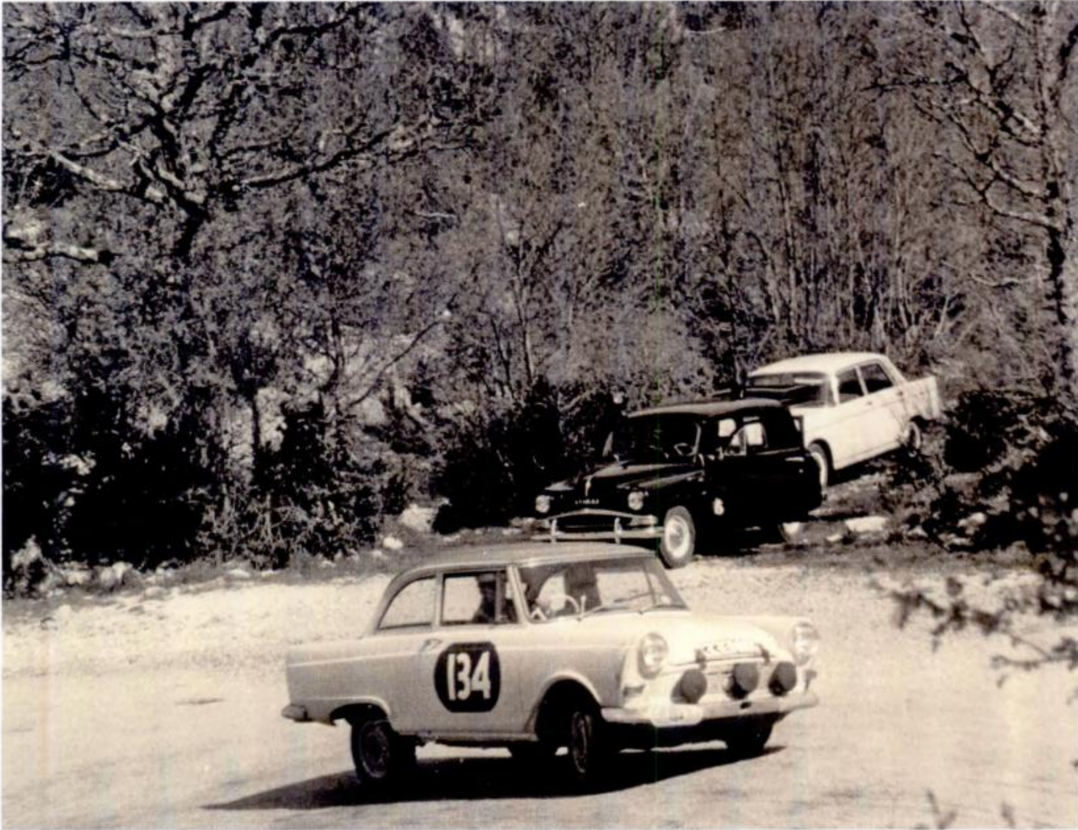
Left: DKW, Tulip rally, 1967 In total contrast, here is my first rally car, the little 750cc three-cylinder two-stroke front-wheel-drive DKW, climbing the Mont Ventoux at my first international rally as a driver. Vic Elford collection
