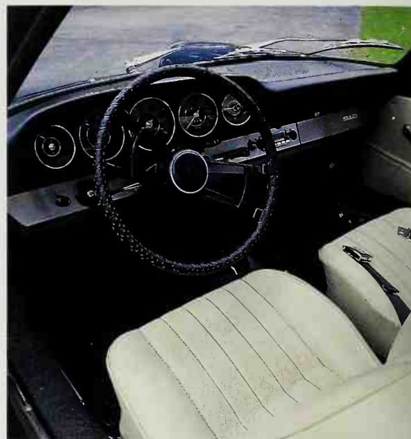
At a glance, it was tough to tell a four-cylinder 912 from the costlier, more potent six-cylinder 911—which, of course, was the whole point. Five-dial 911 gauge set (above) and lack of side-marker lights identifies this U.S. version as a '67 model.
