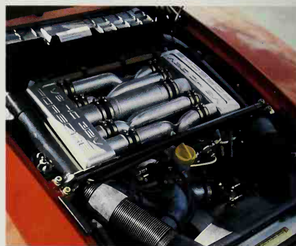
Opposite top: Smoother tail, "detached" rear spoiler identify the latest 928S 4. Other photos: The 1985-model 928S introduced an enlarged 5.0-liter V-8 with 32 valves.
