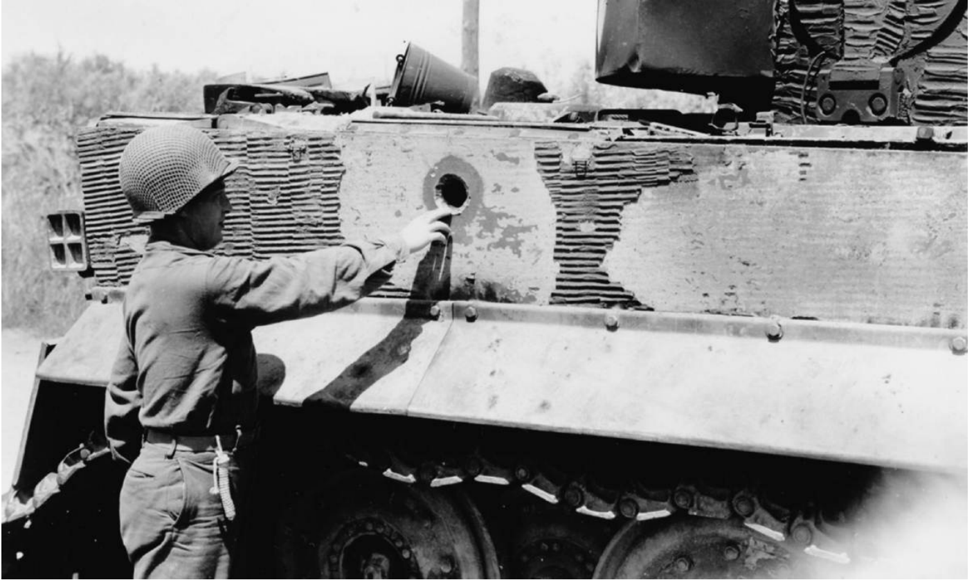
A Tiger from the 508th Heavy Panzer Battalion destroyed by US forces in 1944. The impact of the armour-piercing (AP) round has chipped off large areas of the Zimmerit anti-magnetic coating. (US Signal Corps)
