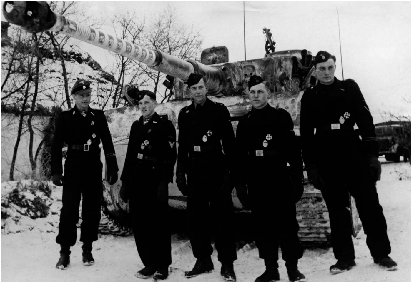
A Tiger I crew from the 502nd Heavy Tank Regiment dressed in the standard black armoured corps uniform. The factory-new tank is painted in standard dark yellow and is fitted with six smoke grenade dischargers on the turret. A further six are mounted on the top of the hull. (Panzerfoto)
