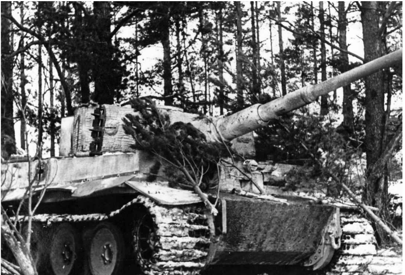
Two whitewashed mid-production Tiger I tanks carefully camouflaged at the edge of a wood, ready for immediate action. The near tank carries the tactical number 1 and is coated with Zimmerit, anti-magnetic paste. (Panzerfoto)
