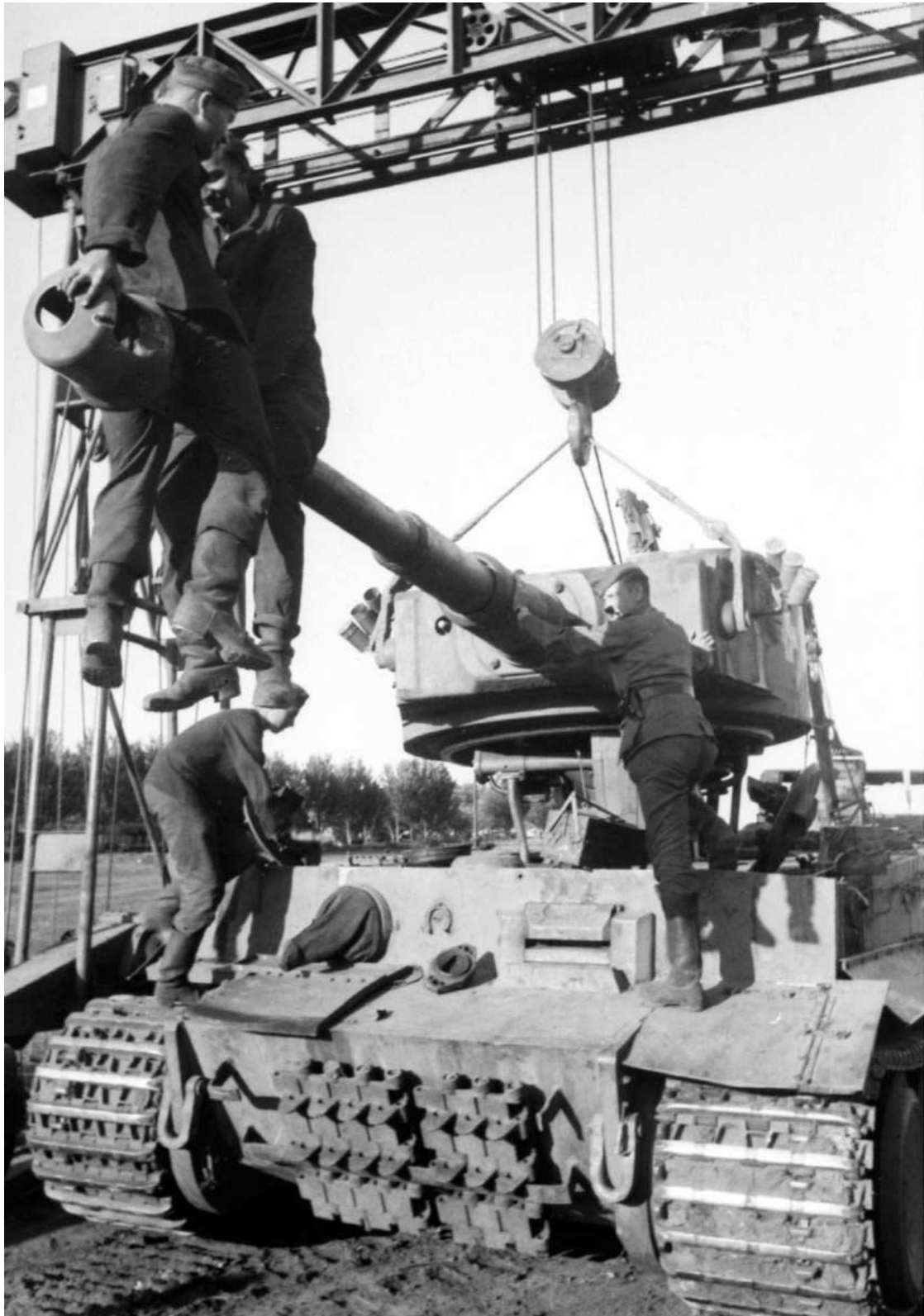
A Tiger I undergoes turret repair with the help of a crane, in the Soviet Union, summer 1943. (Bundesarchiv)
