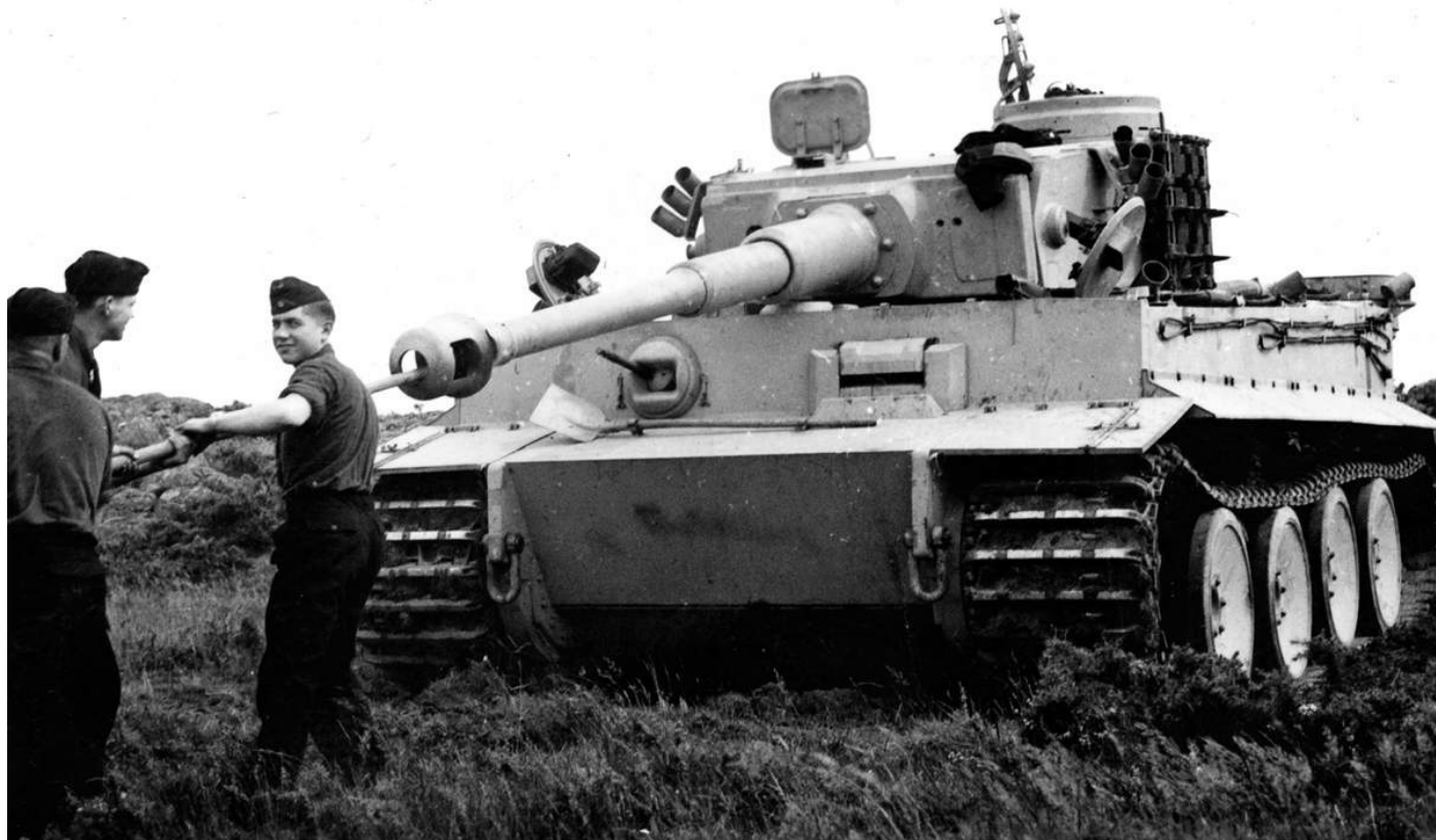
Cleaning the gun barrel required four men to push and pull the stiff brush through the bore in order to remove metal or powder residues from the rifling. (Panzerfoto)
