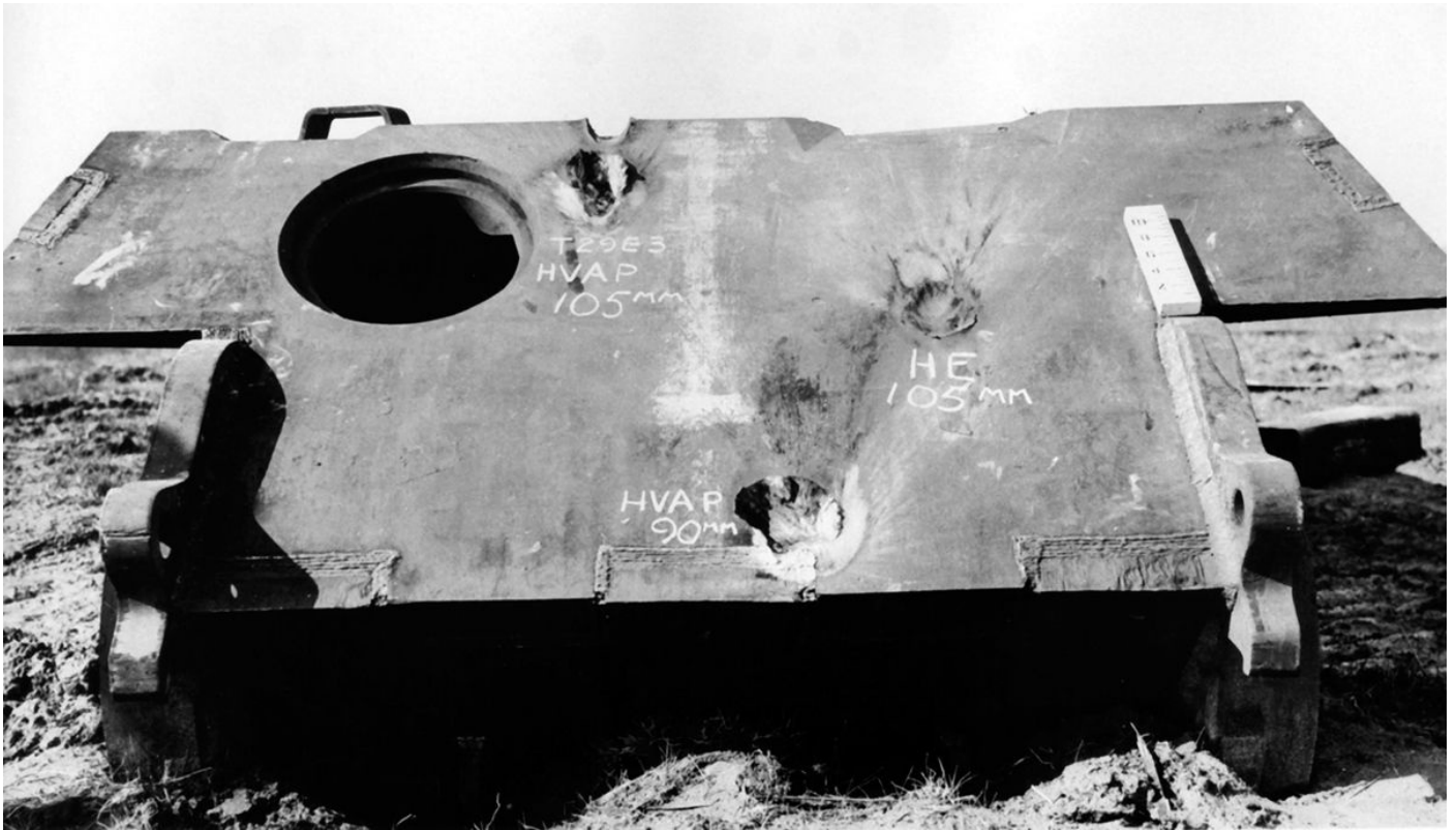
The thick armour plate of a Tiger II, used after the war for test firings by the US military. The 150mm armour has not been penetrated by HVAP shots from 90 and 105mm guns, which at that time were the most powerful US-manufactured anti-tank weapons in service. (NARA)
