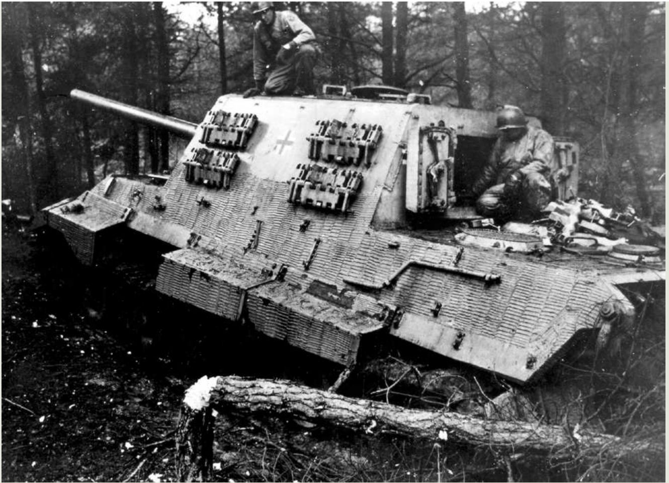
A Jagdtiger bogged down in soft ground, being inspected by US troops. (US Signal Corps)
