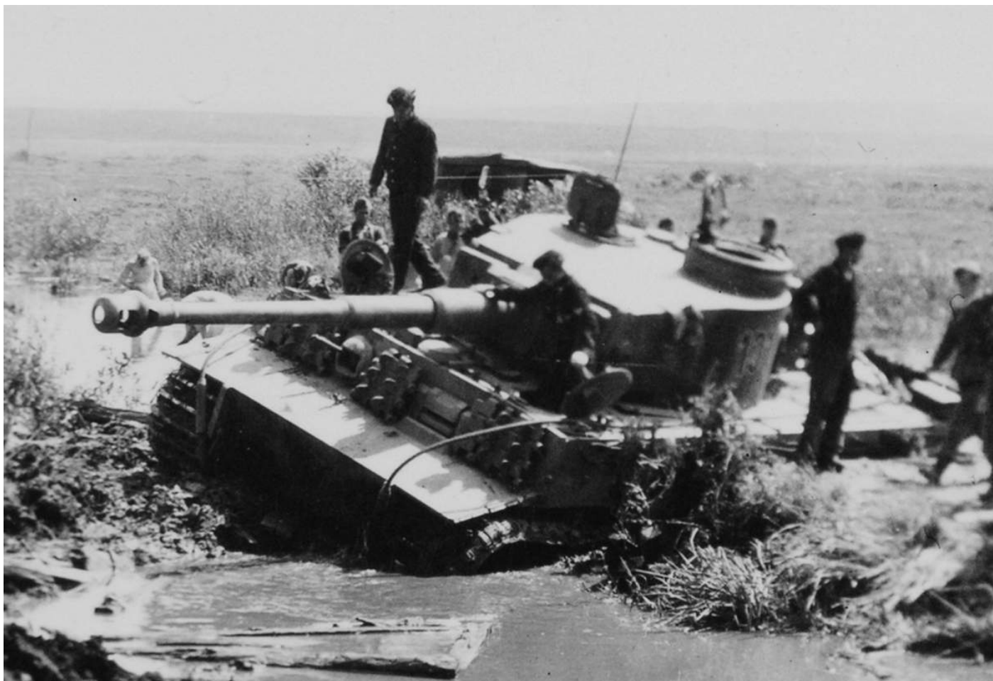
A Tiger I of the 503rd Heavy Panzer Regiment, bogged down in marshy terrain. If a vehicle became stuck like this, it would have to be recovered by several halftracks, and if recovery proved impossible, the crew would have to destroy the tank. (Panzerfoto)
