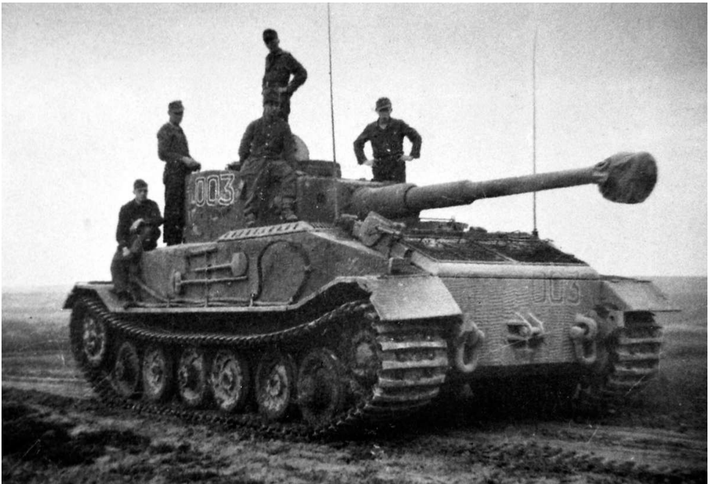
A Befehlstiger, tactical number 003, featuring the distinctive Porsche hull and the additional aerial for command radio equipment. The turret is turned toward the rear of the tank. (Panzerfoto)
