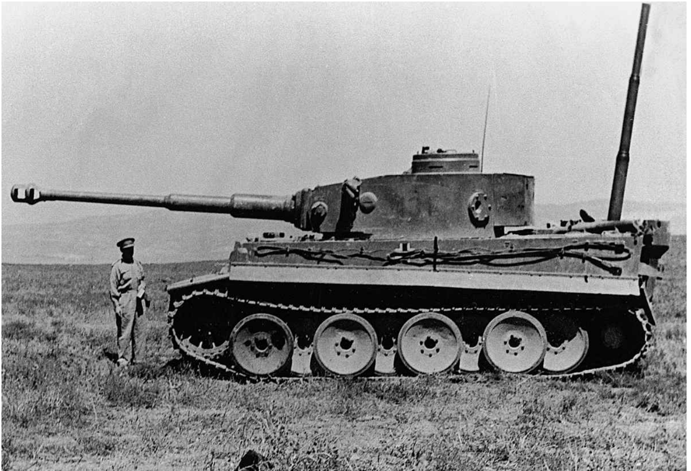
Taken in Tunisia in early 1943, this side view of an early Tiger shows it with its wading tube erected. Also visible is the drum-shaped original commander's turret cupola with its vision slits. (Tank Museum)
