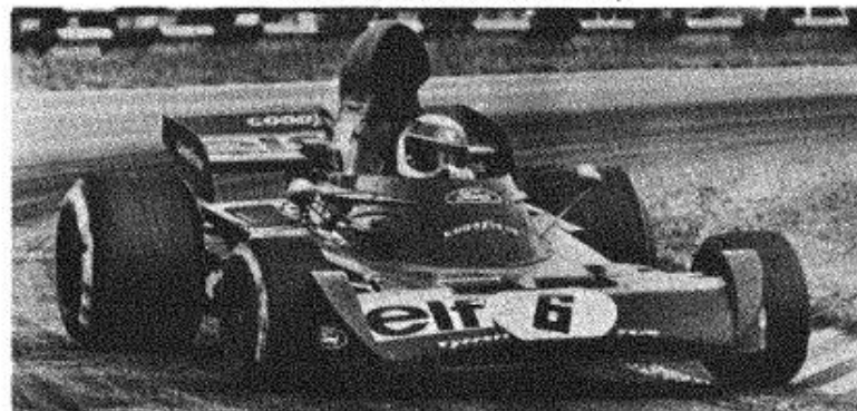
Ram-type overhead air intakes for the engine became common wear in 1971, and by the following season were being integrated with engine covers to smooth out the airflow to the rear wing. Jackie Stewart's Tyrrell is typical of that approach
