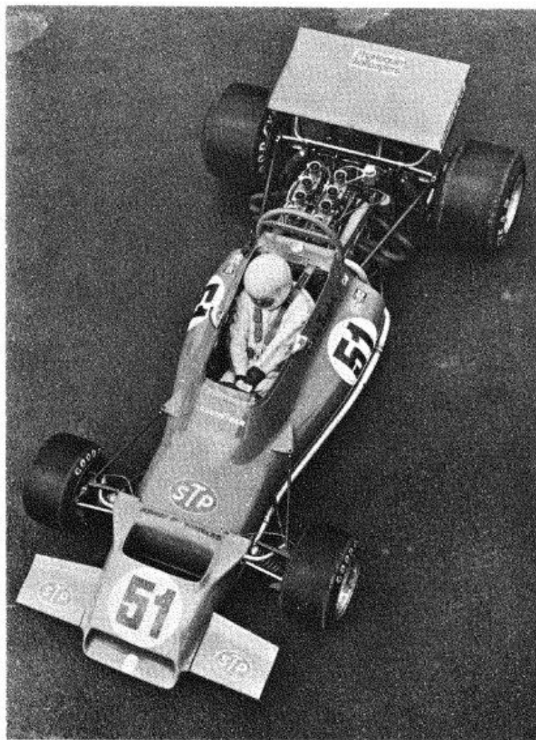
In laying down the guide-lines for the McRae Leda, Graham McRae specified a bulged mid-section for the monocoque, for good torsional stiffness and a low position of the fuel load. The upper panels were welded together, not riveted, to save weight
