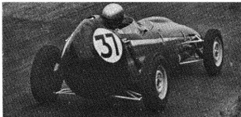
Strut-type rear suspension was a feature of the wedge-shape Terrier Mark 4, a Formula Junior car
