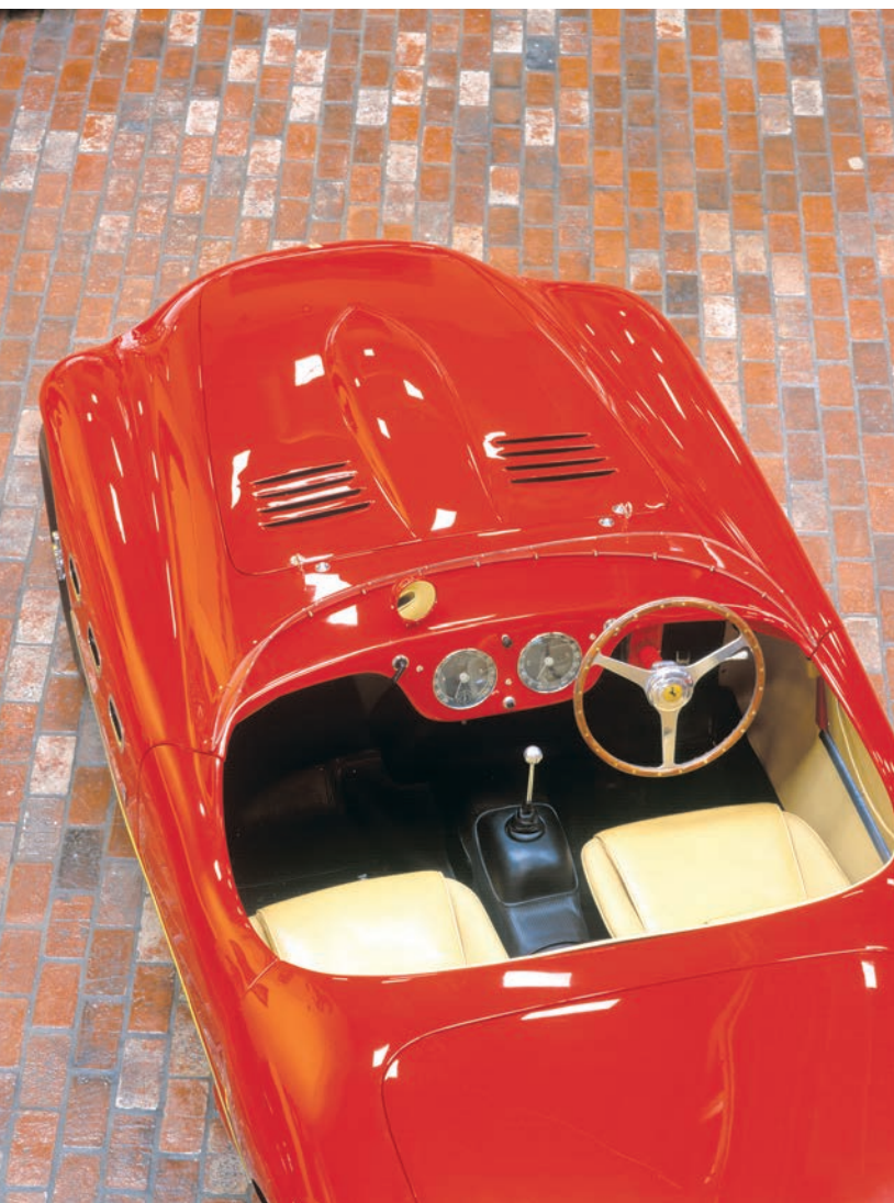
The cockpit of the 250 MM was just that, a place for the pilota , a traditional right-hand-drive racing configuration with two large combination gauges, bucket-type seats, and a large, wood-rimmed steering wheel. The 250 MM was equipped with a new four-speed all-synchromesh transmission.
