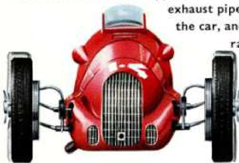
The Type 158B car (above and below, left) with which Emilio Villoresi won the 1938 Coppa Ciano at Leghorn. Note the exhaust pipe position beneath the car, and the shape of the radiator grille.
