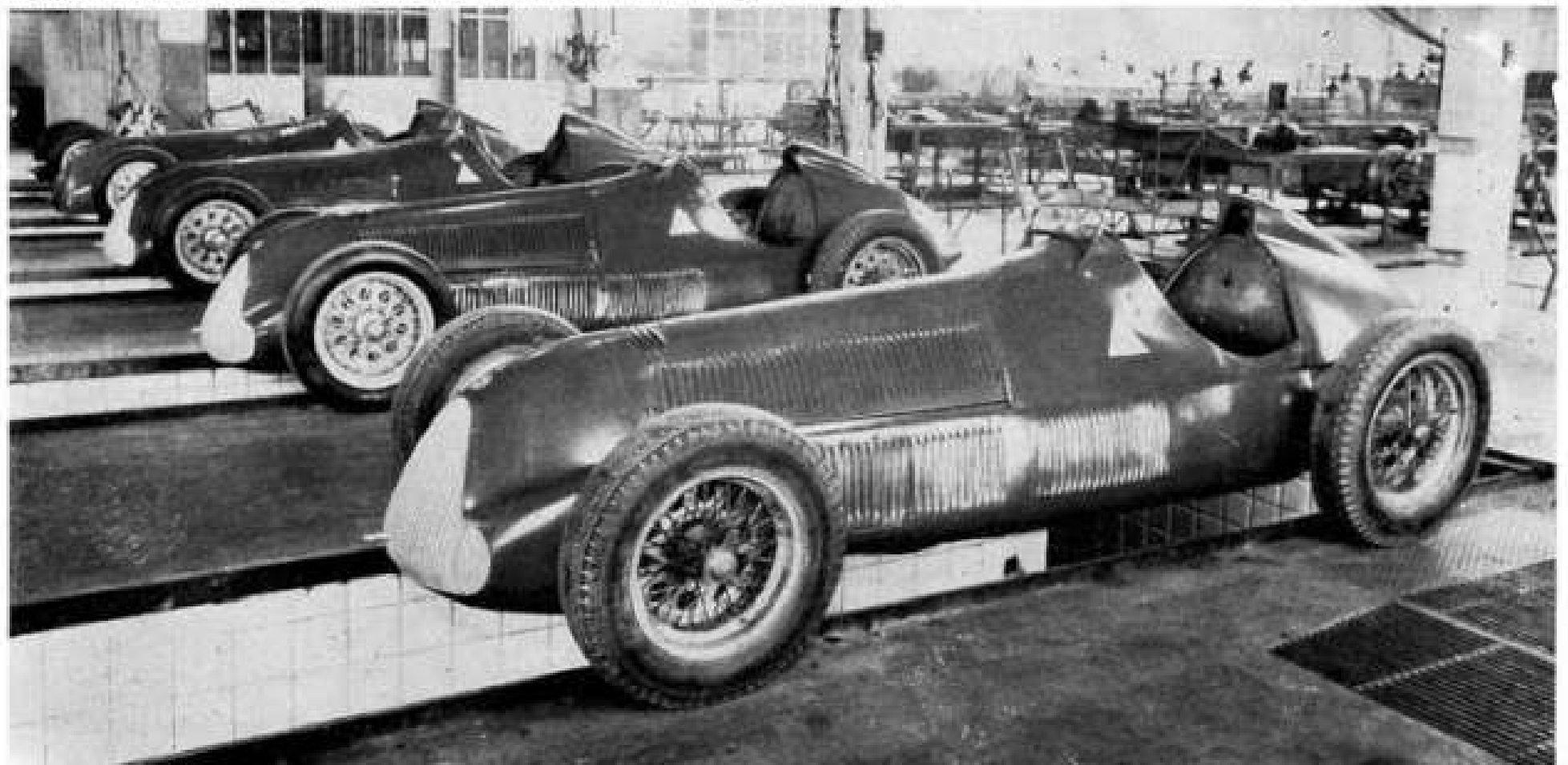
Gleaming new 158s (on 'slave' tyres) in the Alfa Corse shops early in 1940. These have the 'definitive' outline, most noticeably with the scuttle line extended to enclose the rear-view mirrors and a higher tail line. (Photo: Alfa Romeo S.A.)
