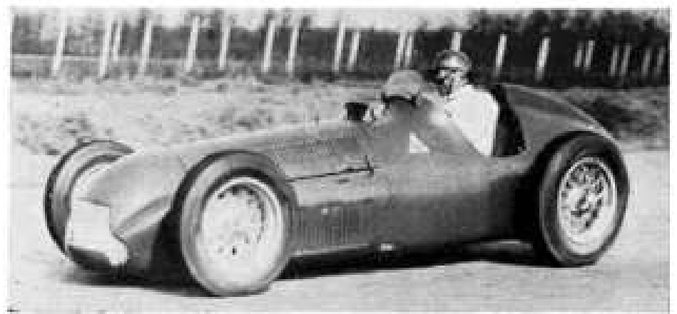
Battista Guidotti, who was the outstanding manager of the post-war Alfa team and could drive as well as some of the men employed in the équipe in that capacity, braking fiercely while testing a 158 in 1950. The grille is partly blanked with plates: these were used in cold weather to maintain optimum engine temperatures. (Photo: Alfa Romeo S.A.)
