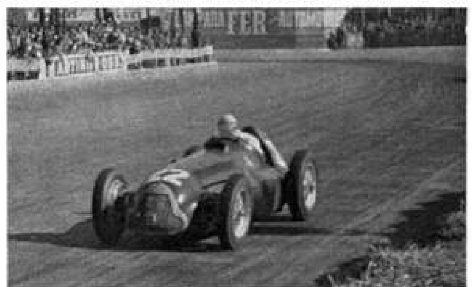
Left: That the 158/159 should have appeared slim in profile was a tribute to its fine lines for, as this shot of Fangio in the 1951 Italian Grand Prix shows, it was a bulky car. This example was a 'de Dion' 159, on which the twin exhausts were reintroduced. (Photo: Alfa Romeo S.A.) Right: Final race and final victory. Juan Manuel Fangio in the 1951 Spanish Grand Prix. (Photo: Cyril Posthumus Esq.)
