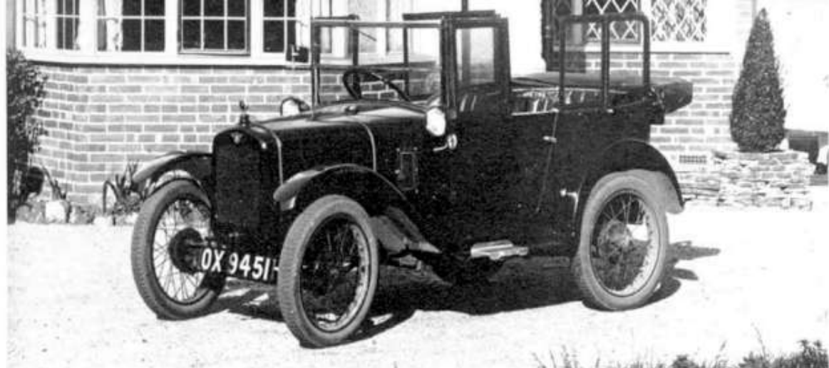
All-weather Tourer. An early modification to the original Chummy was the wider door with sloping rear edge. The rigid side-curtains were regarded as extremely weather-tight in 1927. (Photo: Austin Motor Co. Ltd.)
