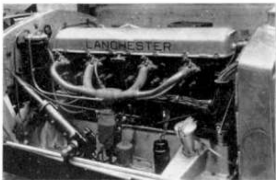
Off side of 'Forty' engine showing advanced design of induction manifold. (Photo: Montagu Motor Museum)
