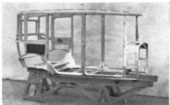
Lanchester body frame of cast aluminium and ash, 1922. Later examples had aluminium centre pillars and rear quarter-framing. (Photo: Mr George H. Lanchester)
