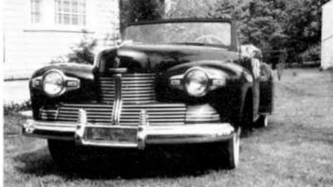
For 1942, Lincoln extensively revised the bodywork of the Continental, with a heavier horizontal-barred grille and bumpers, boxy fenders (wings) and squared-off hood (bonnet). Overall length was increased by 7-18 in. A block bored out to 2½ in. proved quite troublesome. (Photo: Charles L. Betts, Jr.)
