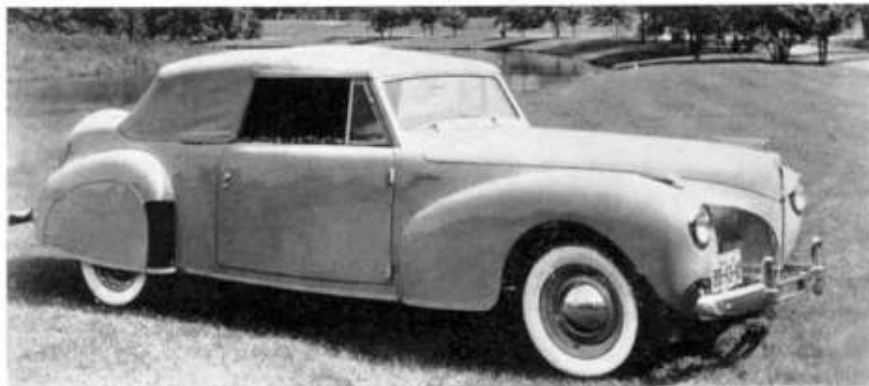
1941 Lincoln Continental Cabriolet; note the addition of Lincoln Continental script at the sides of the hood (bonnet), push-button door latches and Lincoln V-12 on the hubcaps. (Photo: Ford Archives)
