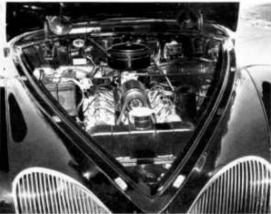
The Model H V-12 Lincoln Zephyr engine which powered the Continentals from first to last. The version shown is the 1941 292 cu. in. model which developed 120 b.h.p. at 3,500 r.p.m. It had polished aluminium cylinder heads and intake manifold, with chrome acorn nuts atop the head studs.
