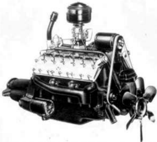
The Model H V-12 Lincoln Zephyr engine which powered the Continentals from first to last. The version shown is the 1941 292 cu. in. model which developed 120 b.h.p. at 3,500 r.p.m. It had polished aluminium cylinder heads and intake manifold, with chrome acorn nuts atop the head studs.
