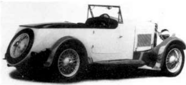
Two special bodies on the Mark II chassis. The two-seater features a large luggage boot and disappearing hood. The saloon was specially built for Gordon Crosby, the well-known motoring artist. Both cars are fitted with the cycle-type mudguards and 'aerofoil' running board which had suddenly become fashionable.
