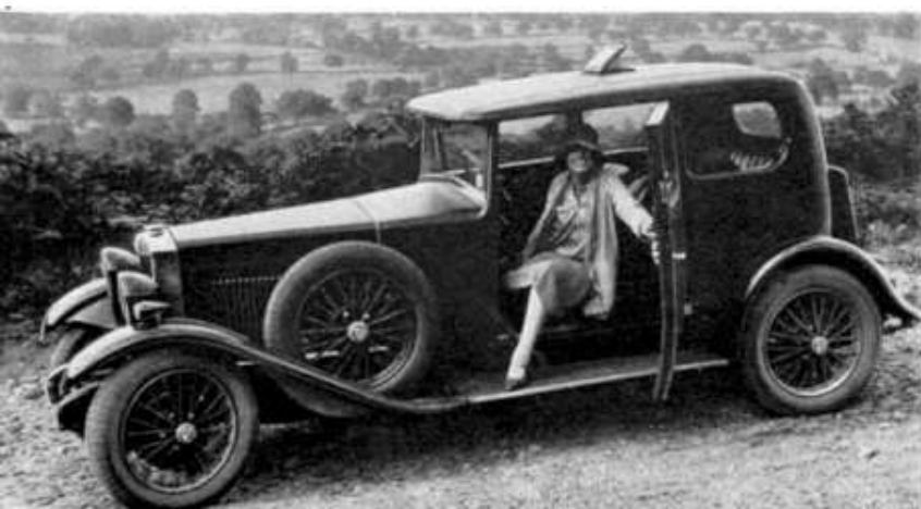
This prototype of the two-door Sportsman's Salonette, with five-stud wheels, was displayed on the M.G. stand at the 1928 Show and subsequently driven in the 1929 Monte Carlo Rally by Sir Francis Samuelson.
