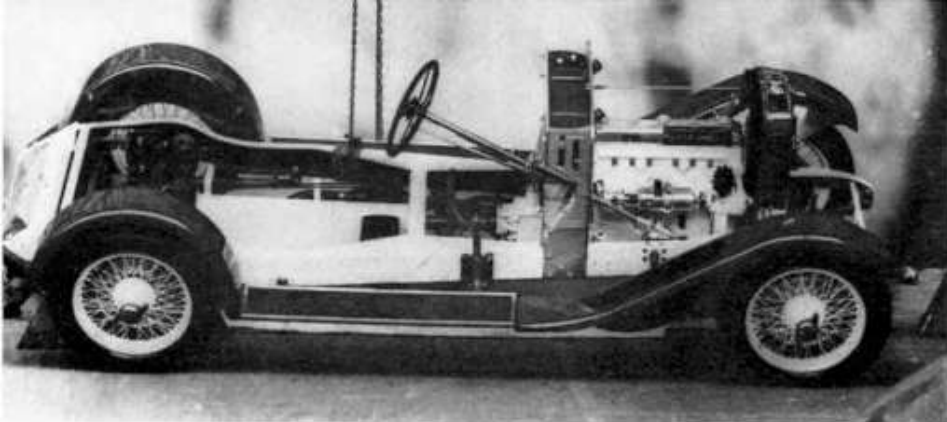
The sectioned Mark I chassis prepared for the 1928 Motor Show revealed many significant differences from the Morris-based prototype.
