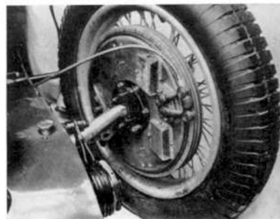
The twin-lever brakes fitted to the 1934 model 'K3' Magnette. (Photo: M.G. Car Co. Ltd.)
