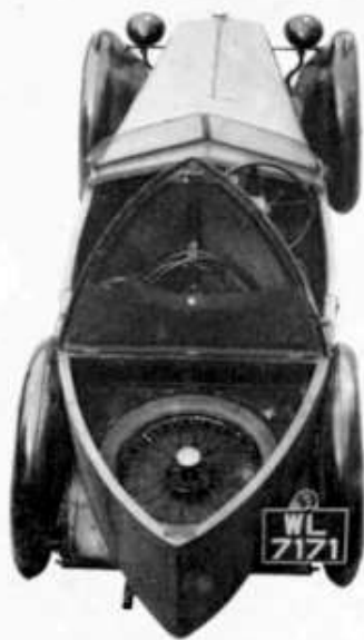
The hood stowed neatly in the boot lid, leaving a surprising amount of luggage space in the pointed tail of the Midget body. (Photo: M.G.)
