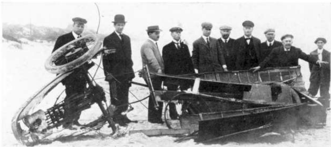
All that was left: the geared-up (11/13) final drive mechanism and the relatively tiny cylinders may be clearly seen. (Photo: Montagu Motor Museum)
