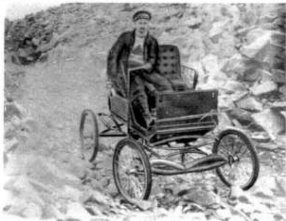
1901 Locomobile, with side-lever steering in place of the more usual bath-chair type of tiller. (Photo: Autocar)
