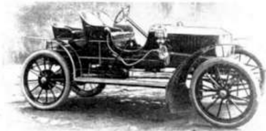
A 30 h.p. example of the 'Speedy Roadster' which was capable of reaching 75 m.p.h. in a brief spurt. (Photo: Autocar)
