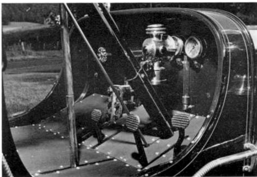
A good light for the boiler gauge-glass was essential for night driving: 1907 Model EX. (Photo: Charles L. Betts, Jr. Collection)
