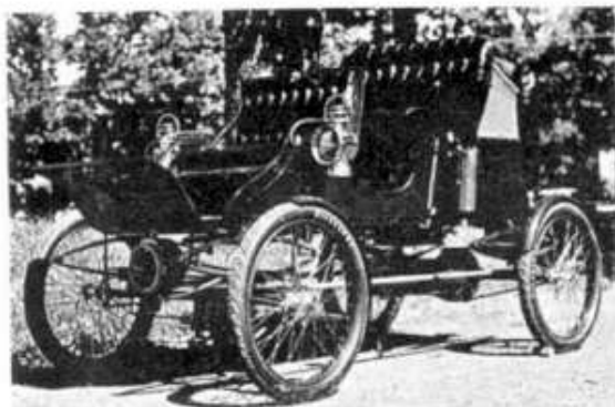
Intermediate type: a 1903 Stanley with the new arrangement of enclosed horizontal engine supported on the reach-bars, but still with rear-mounted boiler. The occasional seat in front could be folded away when not in use.
