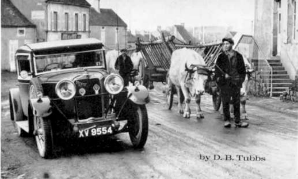
The 14/45 Talbot and its successors may be said to have been born and bred in the Alps by proxy, since their designer, Mr. Georges Roesch, was born in Switzerland and personally did much testing there. Here an early Weymann Sunshine Coupé poses beside some bullock carts after an Alpine foray. Note that the opening of the sliding sunroof extends down almost to the windscreen.
