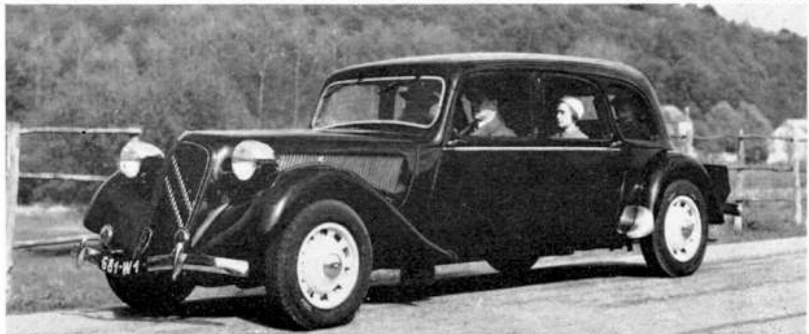
Bandit's Delight—or the 8/9-seater version of the Quinze Chevaux as it appeared in 1939. The painted radiator shell and model designation covering the starting-handle hole are distinguishing features of French-built cars. Also in evidence are the 'Pilote' wheels, while multiple bonnet louvres were to spread to the four-cylinder tractions after the war. (Photo: S. A. André Citroën)
