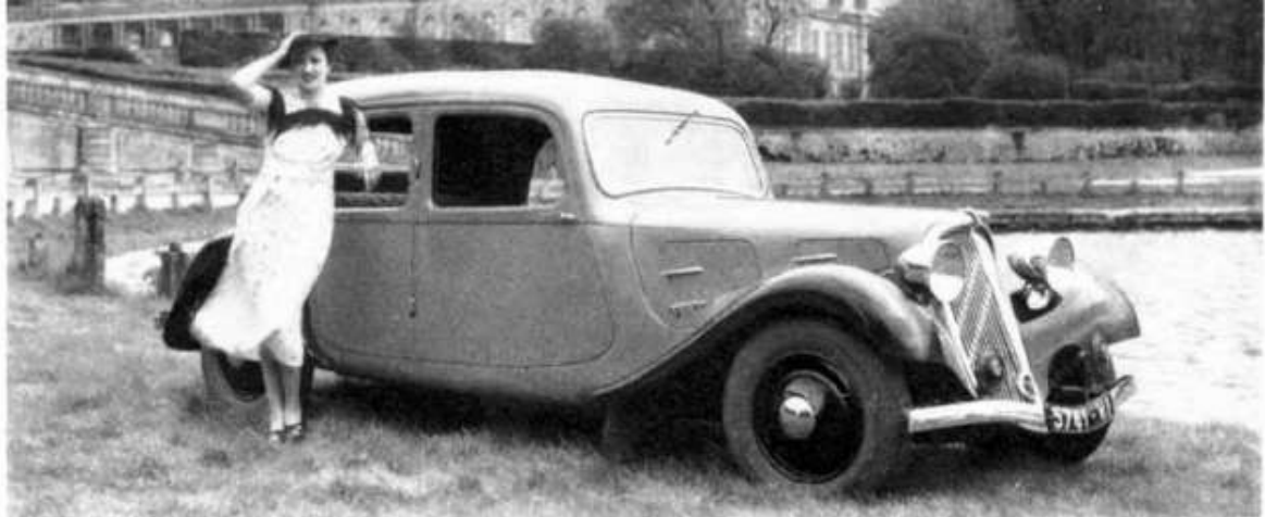
As it was in the Beginning: one of the first 7CVs poses for the public-relations camera. Exposed twin horns indicate 1934, while the single screenwiper and left-hand drive confirm the origins of this car as Paris rather than Slough.
