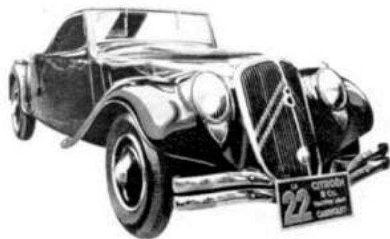
The Citroën That Never Was—the 3·8-litre V8 of 1934 coincided with a financial crisis, and reputedly only six were made. The complete car was recognisable by a stylised front end and recessed headlamps, while the engine (below) was in effect a 'double 11' giving 100 h.h.p. (Photos: S. A. André Citroën)
