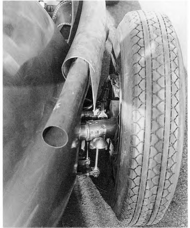
Detail photo of the right rear suspension and exhaust.
