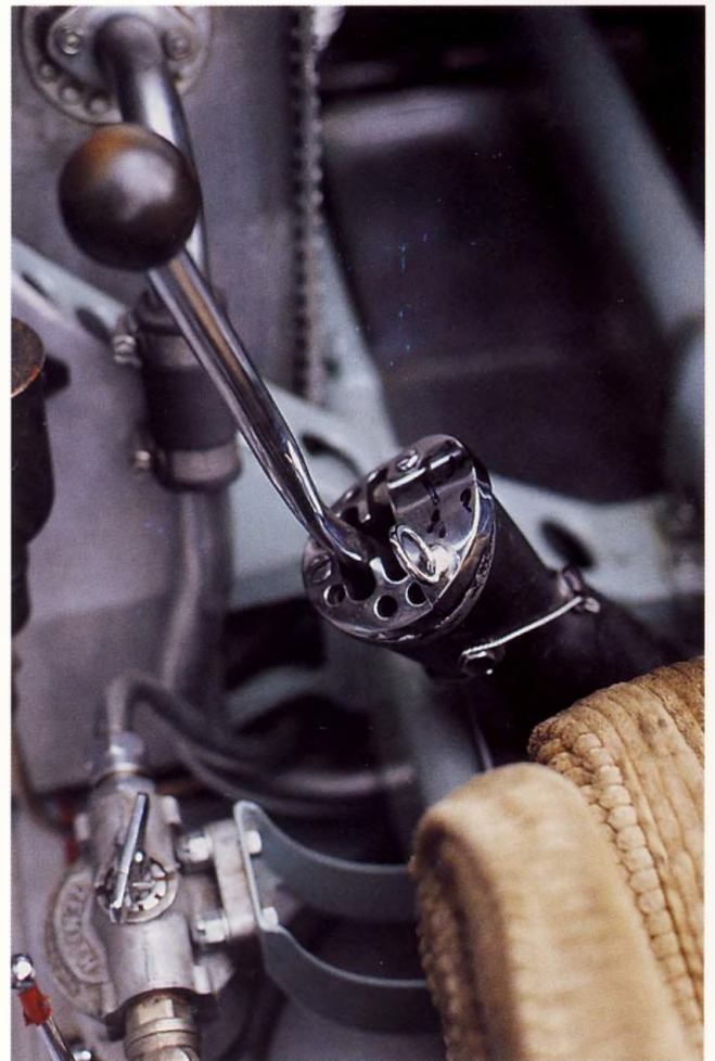
A close-up view of the gear lever, a straight-forward 4-speed mechanism, with a fuel tap down to the left. (Peter Collins)
