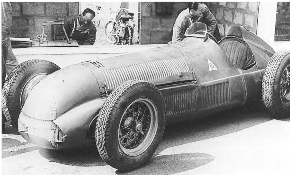
The 159 with the 'splash guards' added behind the front wheels. Sanesi's car is behind. Zanardi watches on the right.
