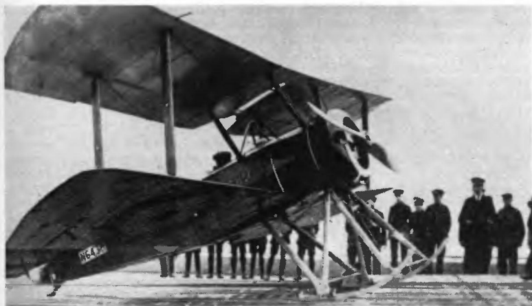
This familiar but historic picture shows a Beardmore-built Sopwith Pup undergoing trials of deck arrestor gear.
