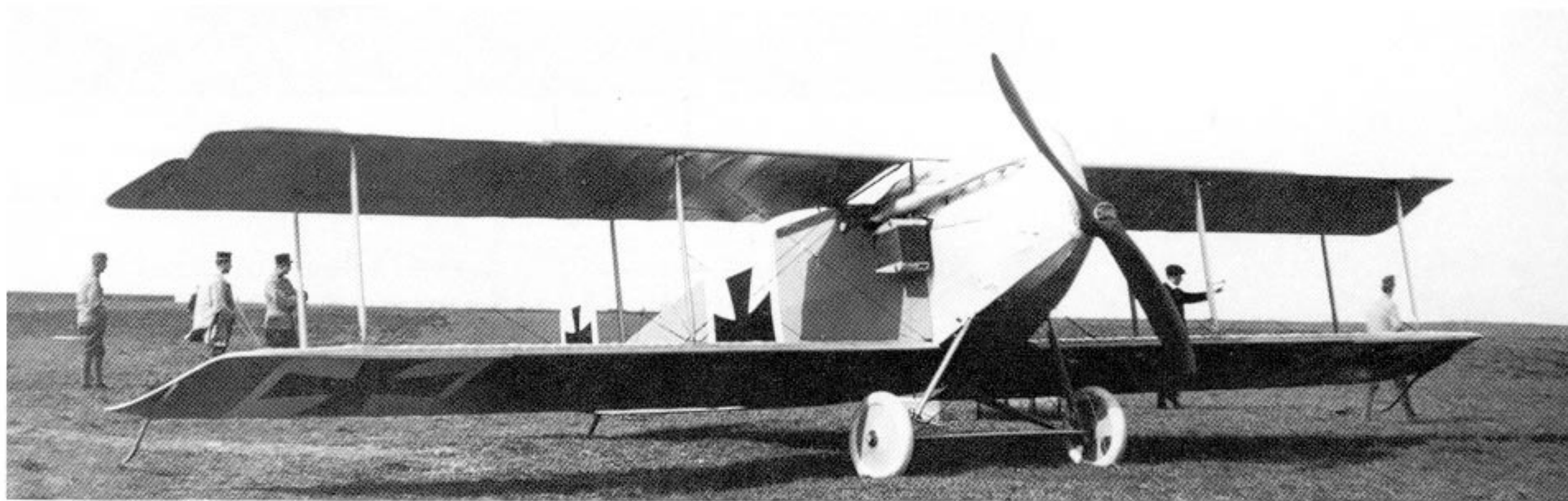
Right and below: The freshly-painted Fokker 03.91 (M 16) upon its arrival at the Aspern test center in April 1916. The wing-tip skids prevented the tips from touching, particularly on uneven or rough airfields. The military serial number has not yet been applied, nor does armament appear to have been installed.
