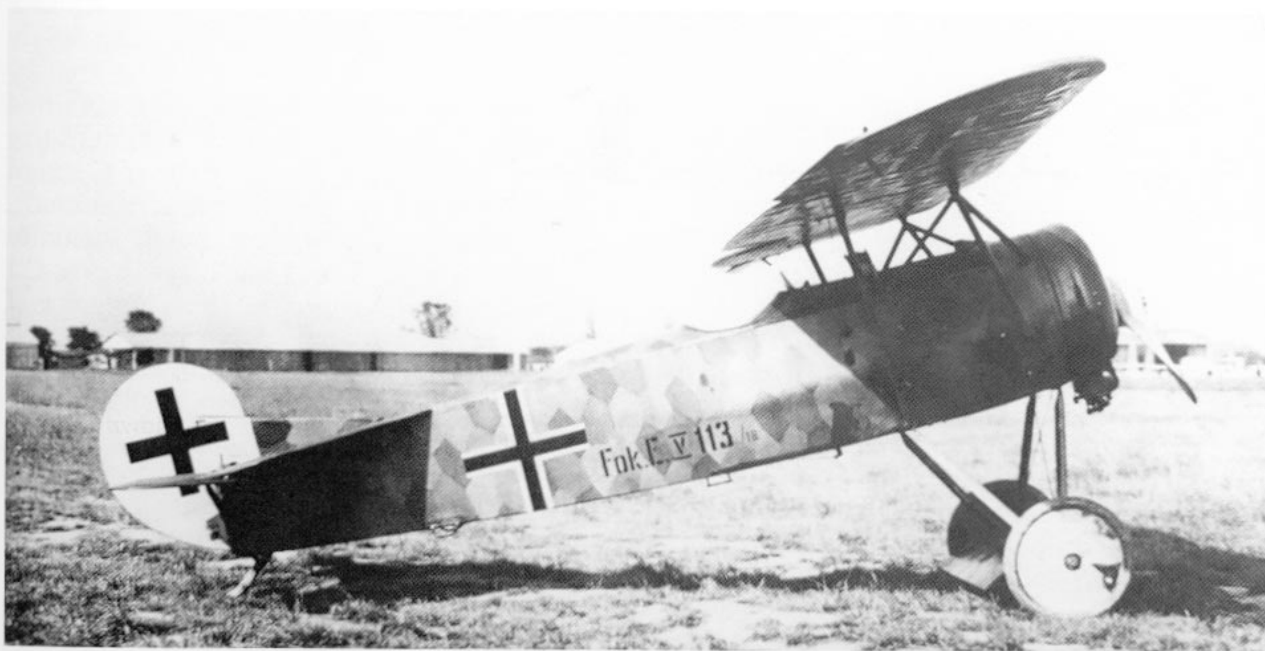
The unarmed Fokker E.V 113/18 on the Aspern airfield in July 1918. The cowling was bulged to accommodate the greater diameter of the 11-cylinder, Steyr-built Le Rhône rotary engine. Although the E.V was extensively flight tested, a LFT designation was not assigned.
