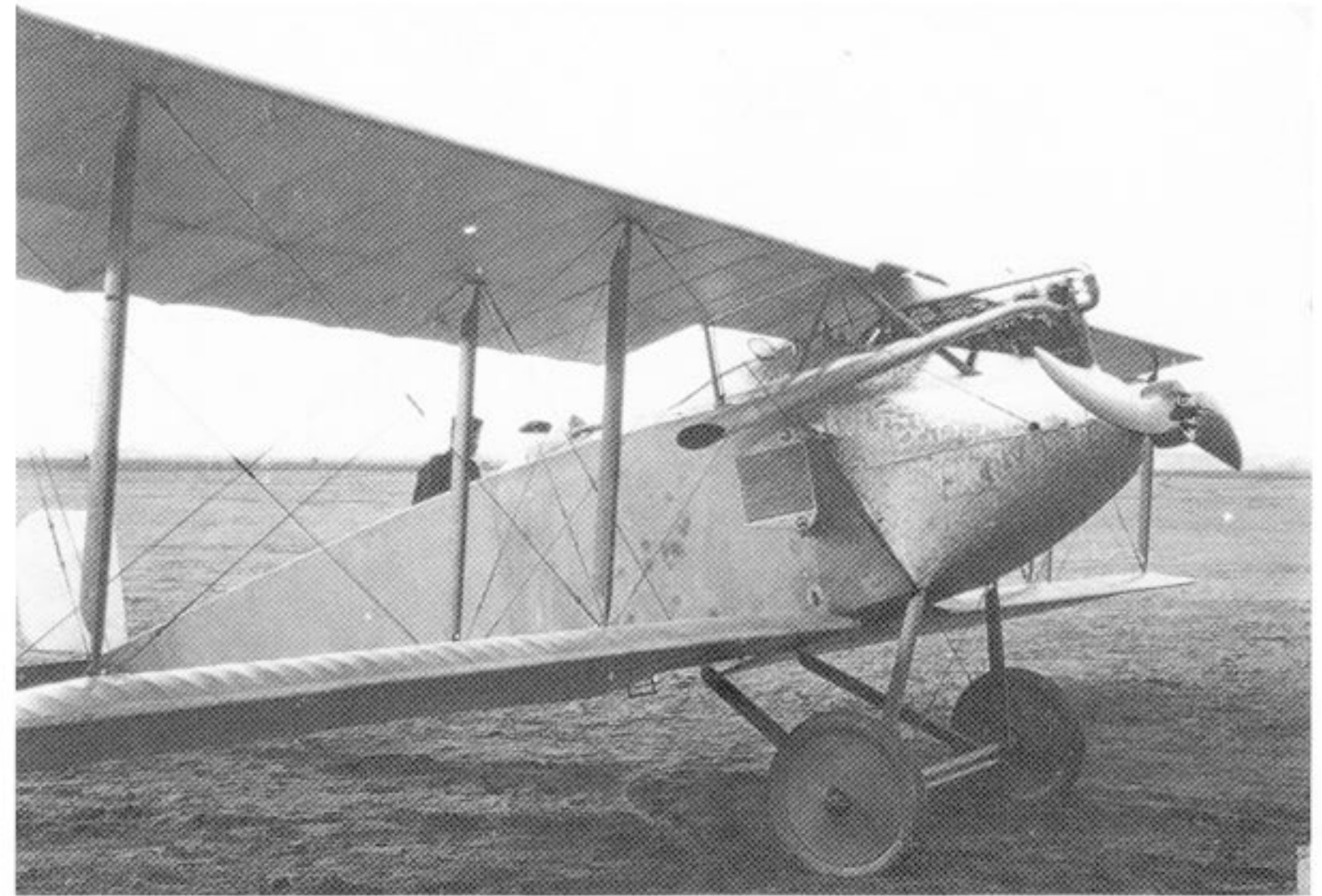
Above: The Fokker M 18 (w/n 501) prototype photographed at the German test center at Döberitz in the spring of 1916. It was powered by a 120 hp Mercedes engine and armed with one Spandau MG 08/15 machine gun.
