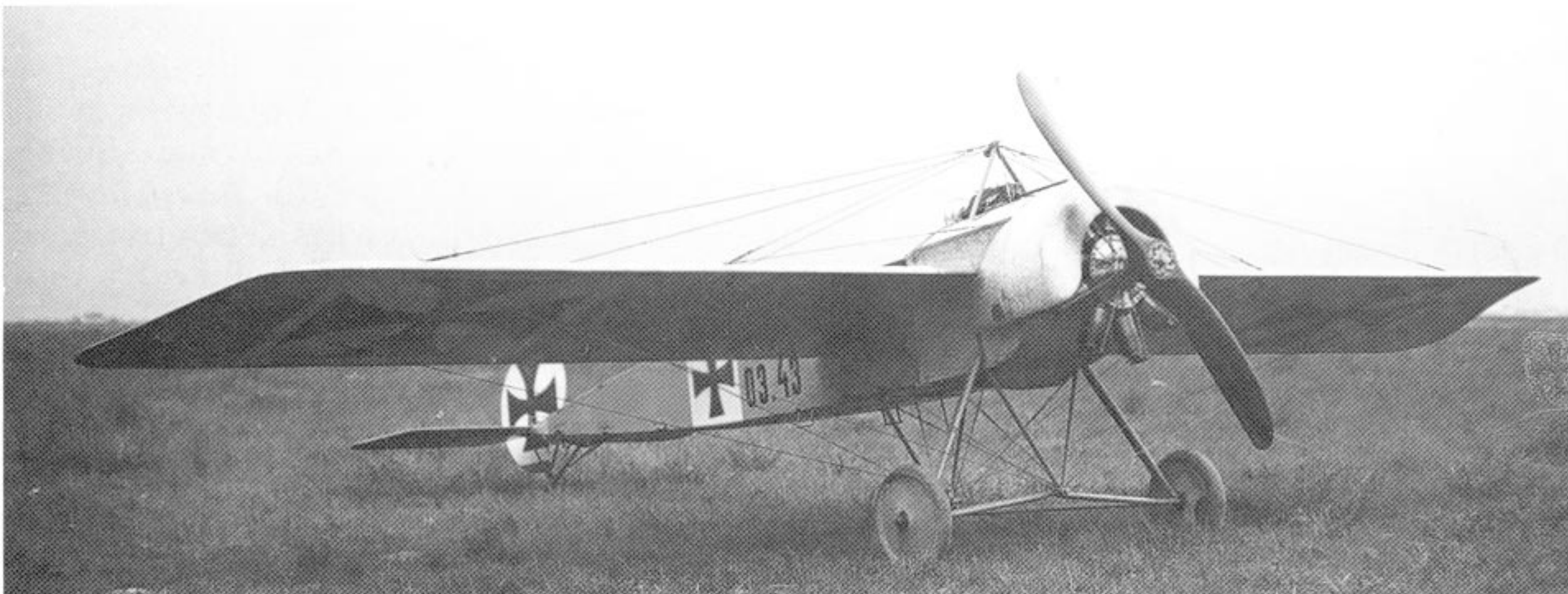
Fokker A.III 03.43 was flown by pilots of Flik 8 and 19 on the Isonzo Front in May 1916. This machine was one of the few armed with a synchronized Schwarzlose M 7/12 machine gun.
