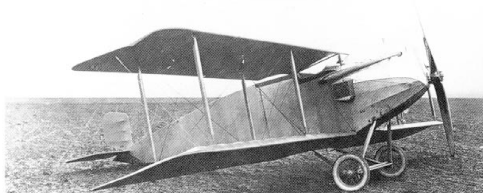
Above: The Daimler-engined Fokker M 16 (w/n 435) prototype photographed at Schwerin, probably in March 1916.
