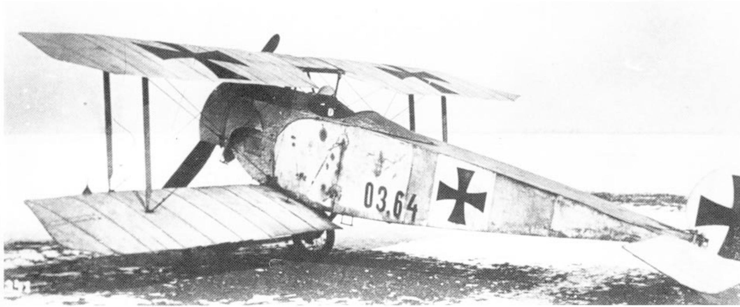
The castor oil in the exhaust fumes has stained the fabric of this Fokker B.II 03.64 trainer of Flek 6. The characteristic Fokker "button" rudder was standard on production machines.
