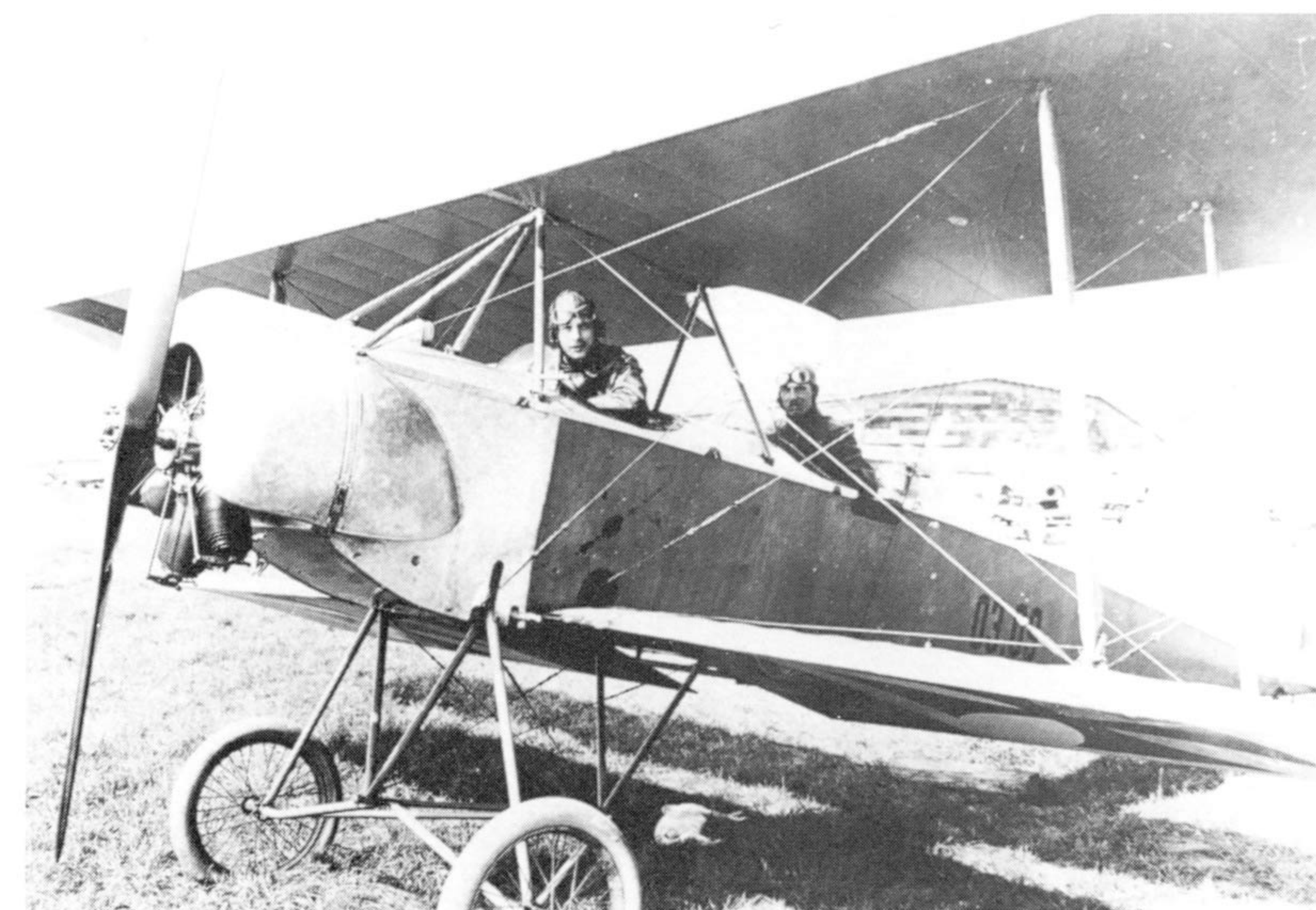
Affectionally dubbed Oelsardine (oil sardine) for the greasy rotary- engine exhaust which coated pilot and airframe, this Fokker B.I 03.09 (M 7) is shown here serving out its career as a secondary trainer with Flek 6.
