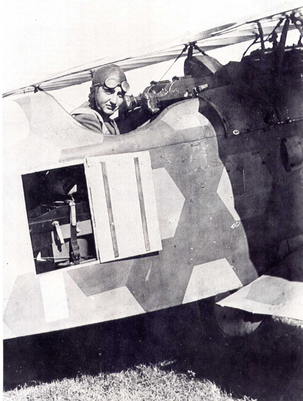
62. The open door shows the location of the remotely-controlled camera as installed in the Aviatik D.I photo-reconnaissance fighter. The guns have padded butts to protect the pilot. The pilot, Oblt. Ludwig Stilmungus , CO of Flik 40/P was killed in combat on August 12 1918.
