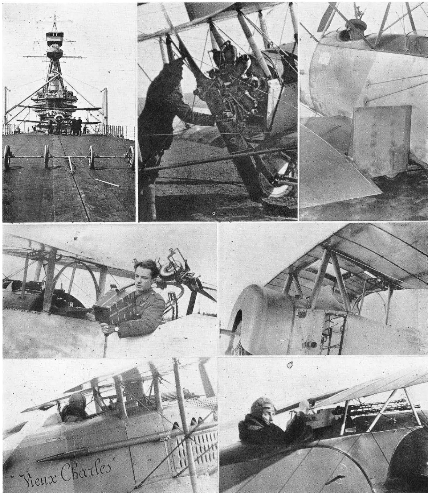
Top left: Sopwith Pup on an early aircraft carrier. Note tail-guide groove. In foreground is take-off trolley for floatplanes. Centre: Swinging the propeller of a D.H.2. Right: R.N.A.S. 1½ Strutter showing air-brake. Next: Two views of the Nieuport 12; on the left Lieutenant Tinne of 46 Squadron, R.F.C., with aerial camera. Lastly: Guynémer in his Spad S.7, and Leutnant Plüschow in Fokker D-II 2387/16.
