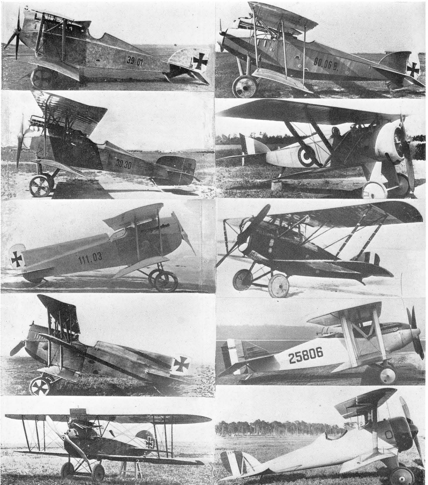
Left, top to bottom: Austrian-Aviatik D-II, 200 h.p. Austro-Daimler, 1918. Austrian-Aviatik D-III, 230 h.p. Hiero, 1918. Lohner D-type, 185 h.p. Austro-Daimler, 1917. Lohner Triplane, 185 h.p. Austro-Daimler, 1917. Phönix D-IIa, 230 h.p. Hiero, 1918. Right, top to bottom: Austrian W.K.F., D-I prototype, 230 h.p. Hiero, 1918. Italian Macchi M-14, 110 h.p. Le Rhône, 1918. Italian Pomilio Scout, 220 h.p. S.P.A., 1918. American Thomas-Morse MB-2 (2-seater), 400 h.p. Liberty, 1918, last, the American Heinrich Scout, 100 h.p. Gnôme of 1917.
