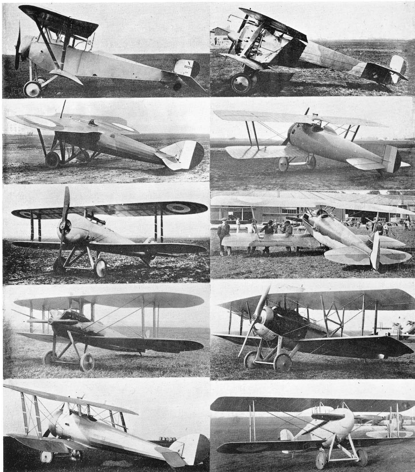
Left—Top to Bottom: Nieuport 20, 110 h.p. Le Rhône, 1916. Nieuport Monoplane, 170 h.p. Le Rhône, 1918. Nieuport Monocoque (28 variant), 170 h.p. Le Rhône, 1918. Nieuport 28/29, 275 h.p. Lorraine-Dietrich, 1917. Nieuport (28 variant), 200 h.p. Clerget, 1917. Right—Top to Bottom: R.E.P. C-1, 250 h.p. Salmson 9z, 1918. Spad 15, 170 h.p. Le Rhône or 160 h.p. Gnôme-Monosoupape, 1917. Spad 20 C-2, 300 h.p. Hispano-Suiza, 1918. Spad 22, 300 h.p. Hispano-Suiza, 1918. Wibault C-1, 220 h.p. Hispano-Suiza, 1918.
