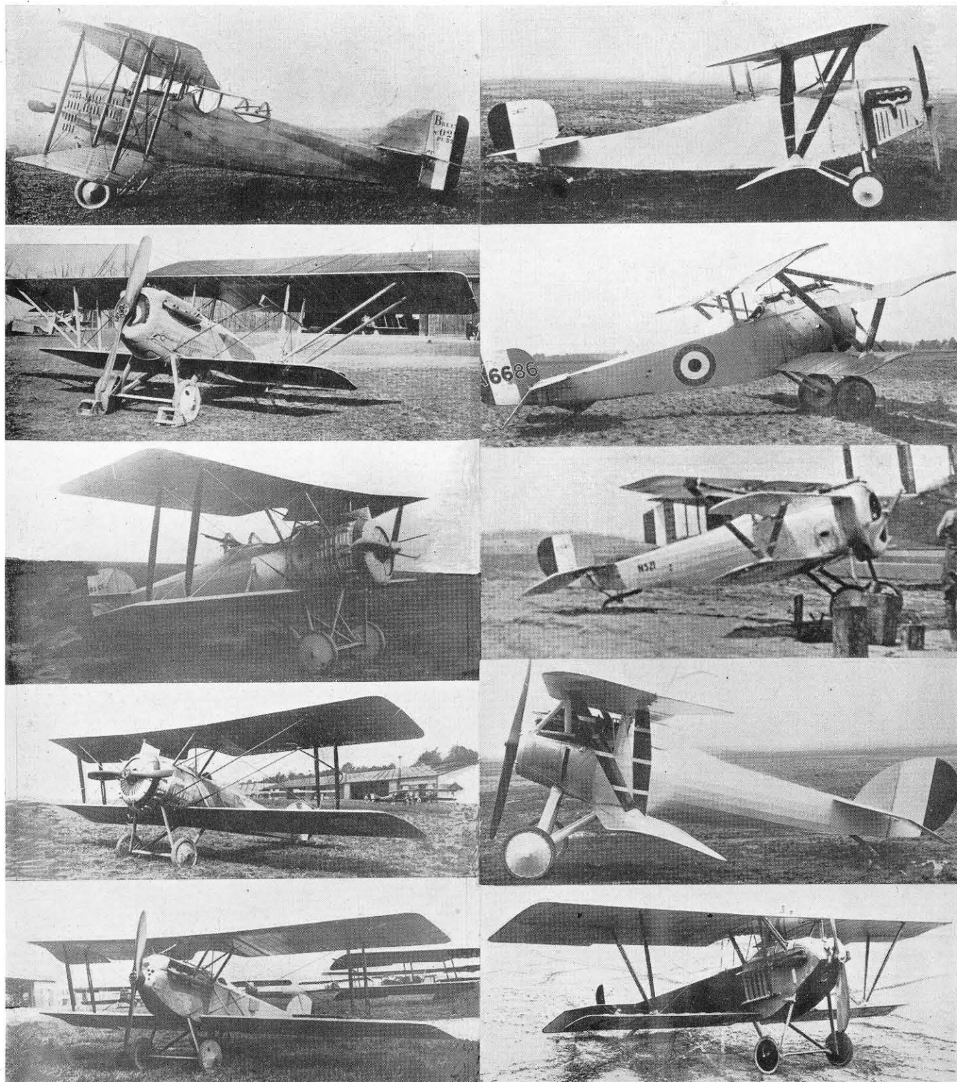
Top Left: All 1918, Breguet 17c2, 450 h.p. Renault. Next: De Marcay C.1, 300 h.p. Hispano-Suiza. Next: Hanriot HD-3c2, 260 h.p. Salmson. Next: Hanriot HD-9, AP-1, 260 h.p. Salmson, Escort fighter. Bottom: Hanriot HD-7c1, 300 h.p. Hispano-Suiza. Top Right: Nieuport Experimental two-seater, 180 h.p. Lorraine-Dietrich, 1915. Next: Nieuport Triplane, 110 h.p. Le Rhône, R.F.C., 1916. Next: Nieuport Triplane, 120 h.p. Le Rhône, R.N.A.S., 1916. Next: Nieuport, 150 h.p. Hispano-Suiza, 1917. Bottom: Nieuport 12, 150 h.p. Hispano-Suiza, 1917.
