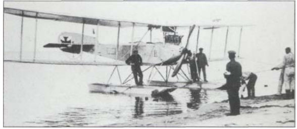
The 33B was an unarmed reconnaissance version powered by a 160hp Maybach, giving it a top level speed of 68mph at sea level. Only five of this variant were ever ordered. (Cowin Collection)
