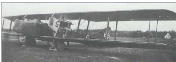
Although always overshadowed in the public eye by the Gotha name, the Friedrichshafen G III equipped three of the eight German bomber wings at the time of the Armistice. Larger and heavier than the contemporary Gotha G IV, the G III carried a far heavier bomb load and seemed far less susceptible to the landing gear failures that constantly beset the Gothas. With a 3-man crew, the G III was powered by two 260hp Mercedes D IVs and could carry up to 3,300 lb of bombs. Armed with two or three 7.92mm Parabellums, the G III had a top level speed of 87mph at 3,280 feet, along with a duration of 5 hours, implying a tactical radius of action, with full bomb load, of around 140 to 145 miles. Deployed initially in mid-1917, the G III and G IIIa went on to equip KG 1, KG 2 and KG 4 during 1917 and 1918. (Cowin Collection)
