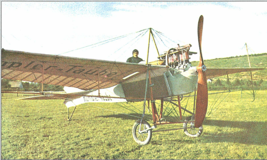
97). Not many Rumpler Taube monoplanes were fitted with an engine as powerful as this 120-hp Austro-Daimler. The extra-large laminar radiator on the fuselage sides reflects the engine power and the inefficiency of the radiator. The colour values of this 1911 aquatint postcard appear to be reasonably accurate.
