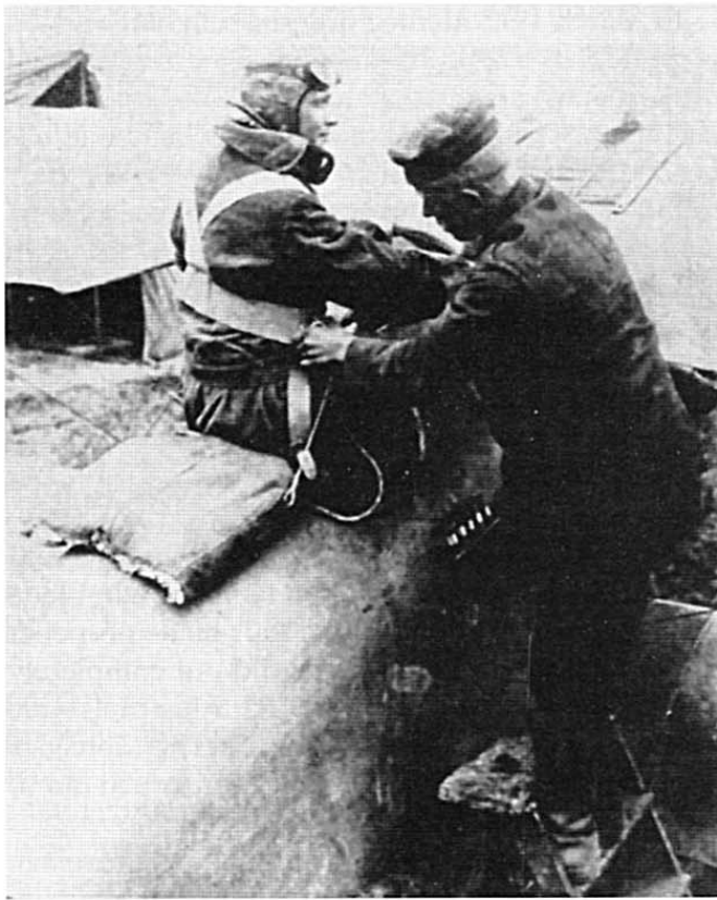
The Heinecke parachute seen here fitted to the fuselage of a D.III was pilot's last resort. On the side are flare gun rounds.
