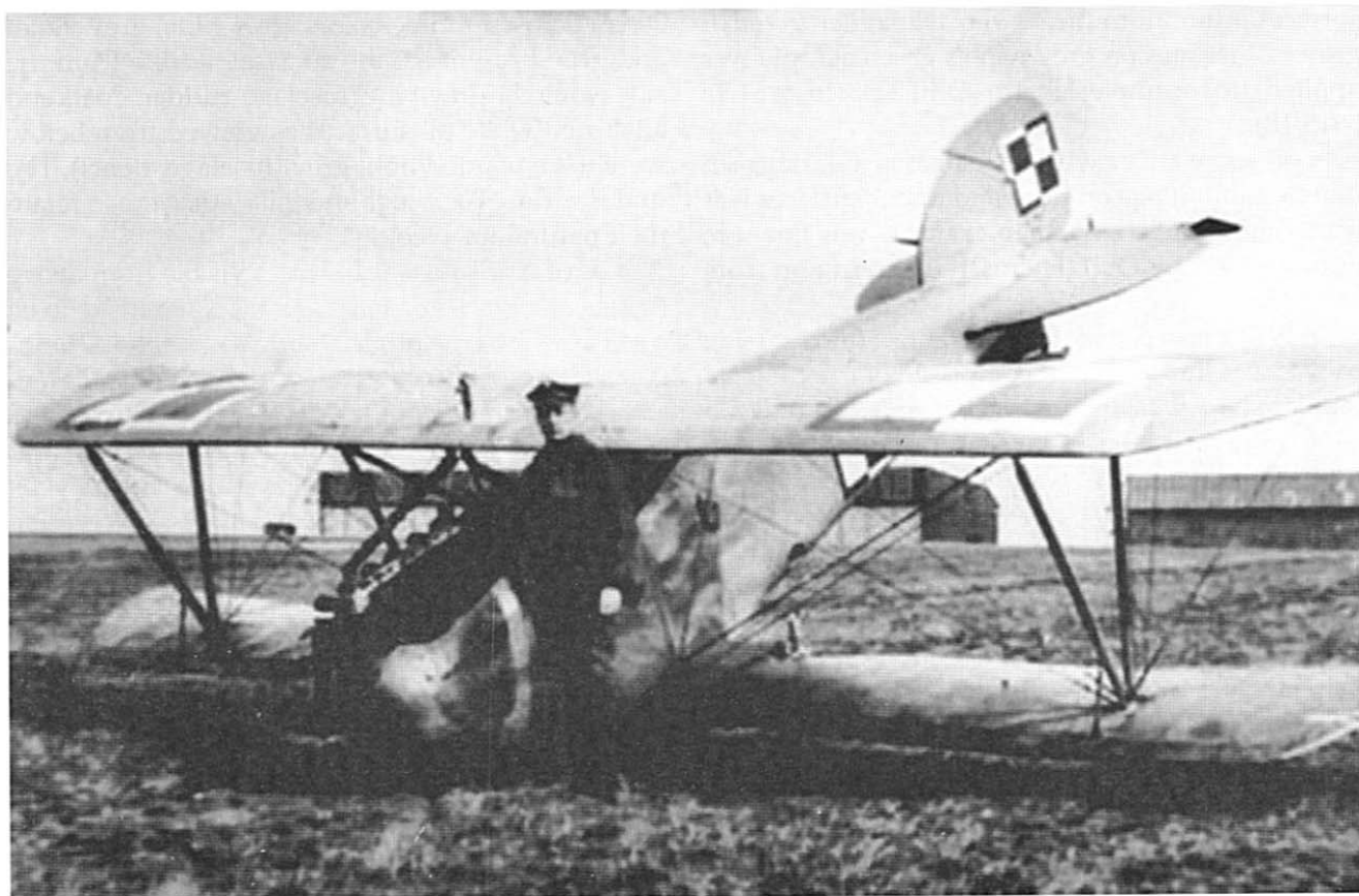
Plt. Lt. Doroszewski crashed an Albatros D.III (Oef) fitted with additional lower wings strengthening support taken after the Germans. It was camouflaged either in natural colors or light grey. Note Teves und Braun radiator installed on this plane and unusual form of aircraft number ALB. D.III 216 painted on the rudder.
