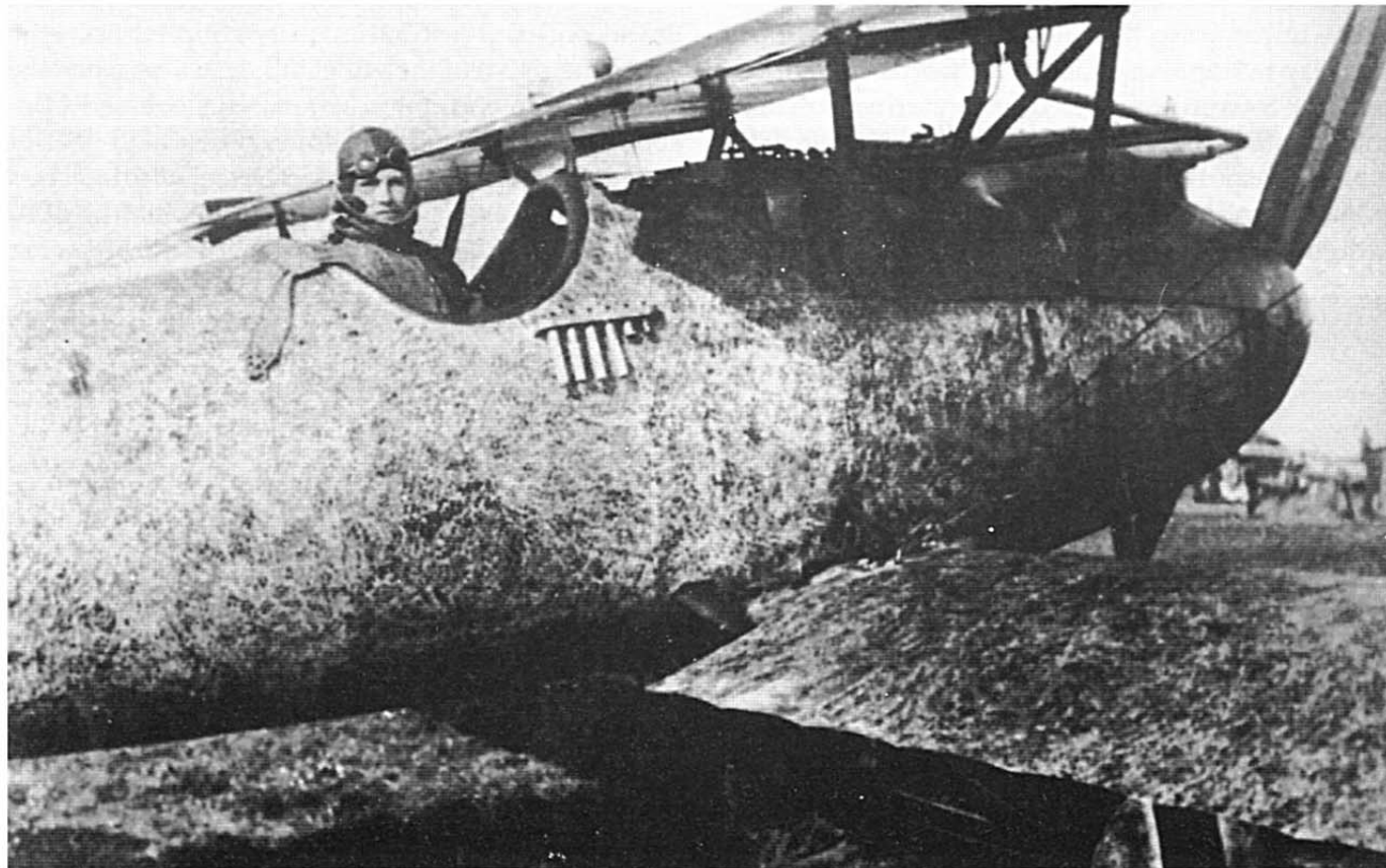
Lt. Ludwig Hanstein from Jasta 37 in the cockpit of Albatros D.V. His Albatros was overpainted in a silver grey finish, with dark green dapple camouflage. Under the cockpit there is a grip for flare pistol rounds.
