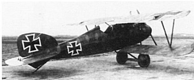
A prototype of the Albatros D.V completely covered in five-color lozenge camouflage. The rudder was taken from Albatros D.III.
