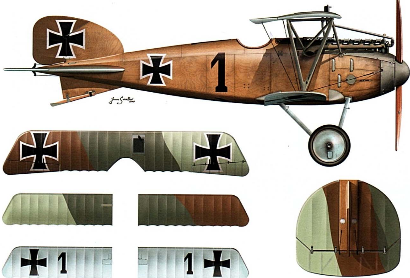
An Albatros D.III from Jasta 29. This aircraft was from the third and last production batch ordered in March 1917 and built at Johannistahl Albatros Factory. Upper surfaces of wings and tailplane were painted in three color terrain scheme. Note the usual German habit of repeating the aircraft number painted in black on both sides of fuselage and on the spine, probably painted on under surfaces of lower wings and fuselage.
