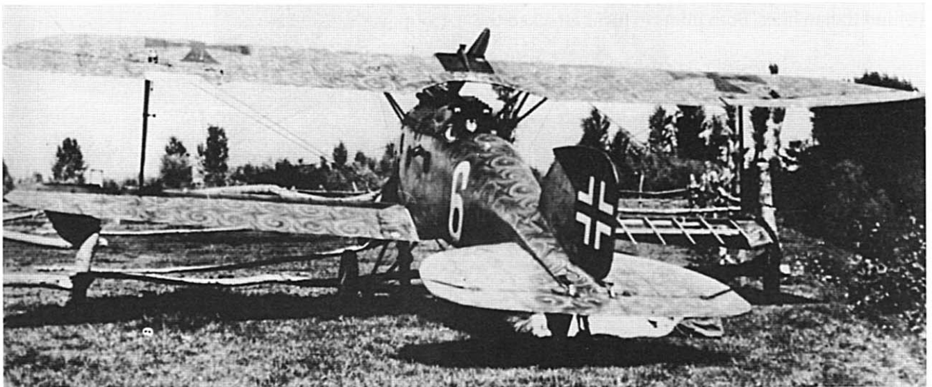
Albatros D.III (Oef) 253.64 that was flown by Stfw. Friedrich Hefty from Flik 42J. The plane had spiral-covered canvas skin and mixed markings combining old-fashioned and 1918 recognition marks. The picture was taken on Aug. 28, 1918 at Pinzano after an unfortunate landing when the right lower wing had been damaged in the process.
