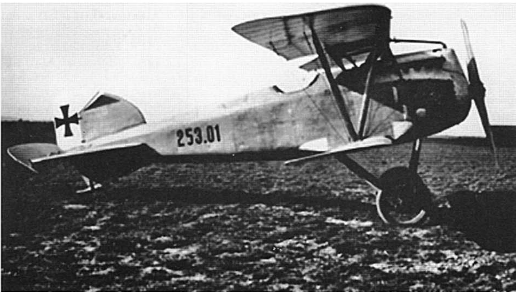
Albatros D.III (Oef) 253.01 was the first D.III (Oef) example to be fitted with the new 220 hp (161 kW) powerplant.
