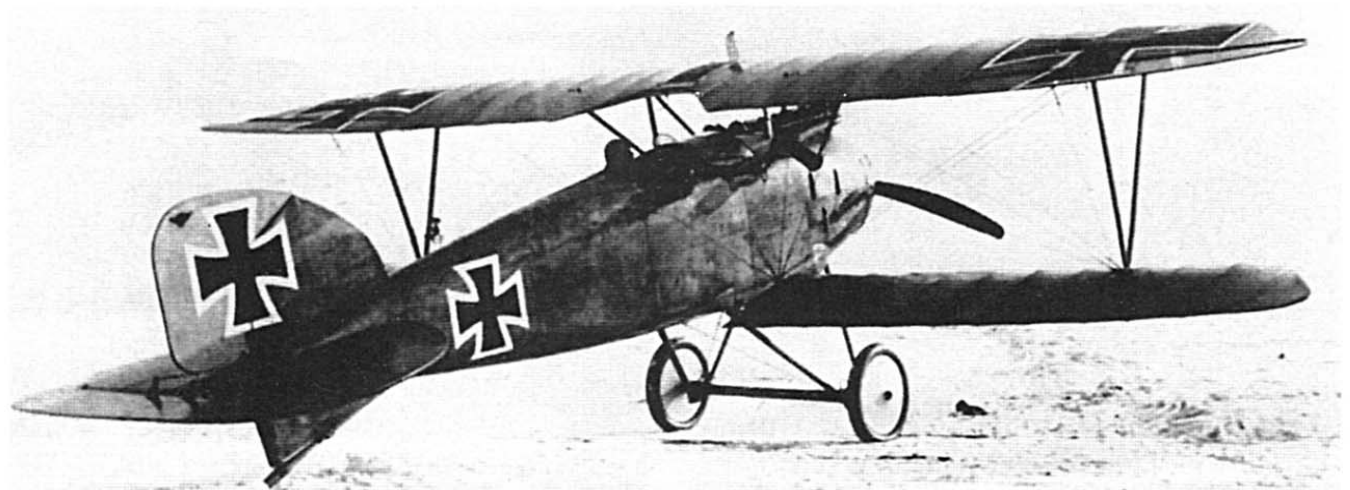
An early example of the Albatros D.III with a centrally mounted Teves und Braun radiator.
