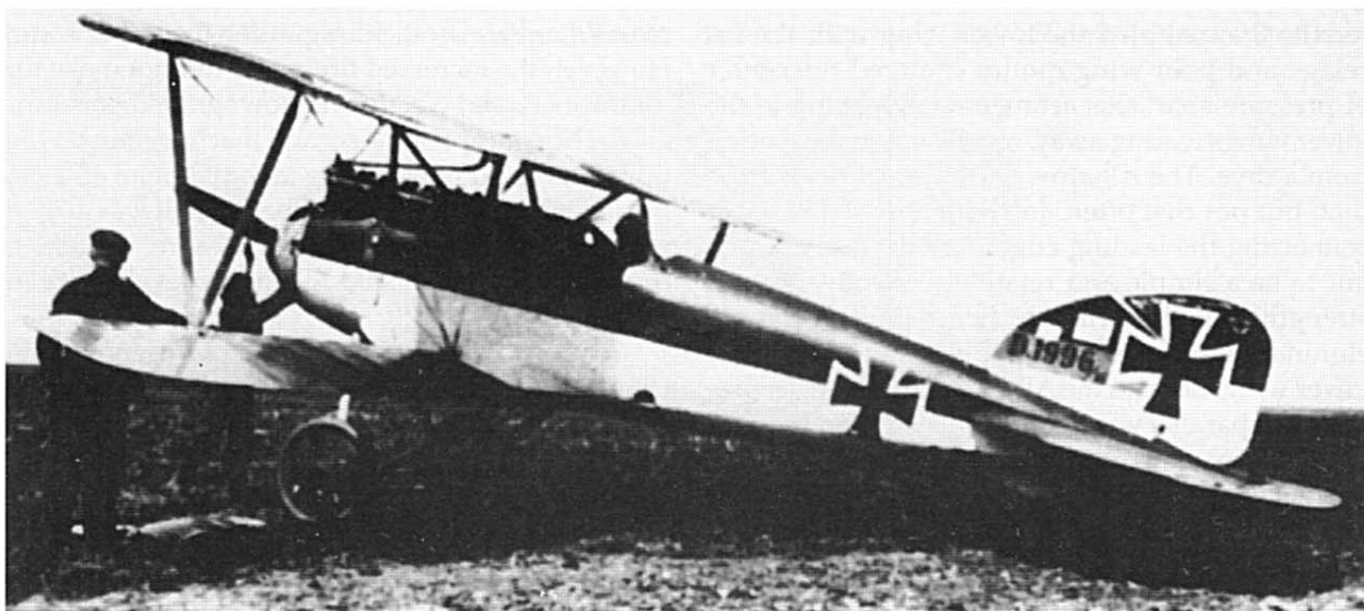
Lt. Rudolf Hohberg's Albatros D.III 1996/16 of Flieger Abteilung(A) 263 adapted to reconnaissance missions. The fuselage is painted in light blue and dark green, upper surfaces of wings and tailplane in three color Terrain Camouflage.
