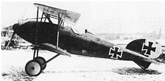
The Albatros D.IV prototype was fitted with a closely-cowled specially-g geared Mercedes engine.
