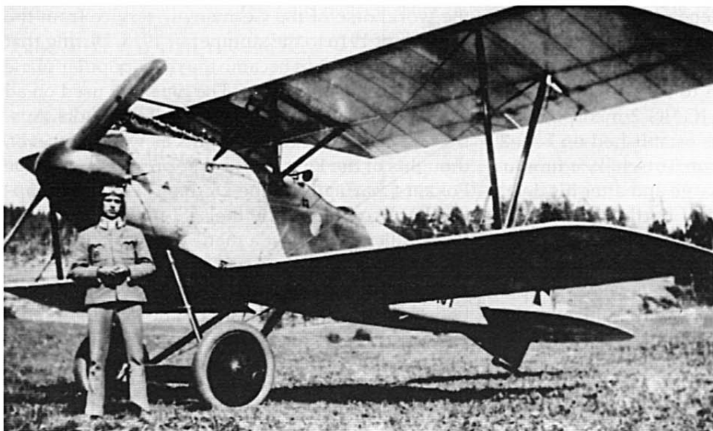
Albatros D.III(Oef) 53.37 from Flik 48. The red nose, wheels and struts constituted Flik 48's markings which shared the Perigine airfield with Stabsfeldw. Josef Kiss Flik 24. October 1917. This example received a refinement unusual for Austro-Hungarian-built Albatroses – a German strengthening of the lower wings by additional small struts. Next to the airplane is Stabsfeldwebel Josef Kiss, Austria-Hungary's fifth top scoring fighter pilot.
