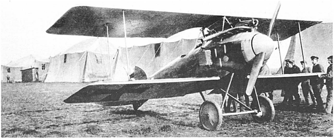
Albatros D.I 423/16 in plain varnish fuselage and fin (natural plywood color with a varnish finish).
