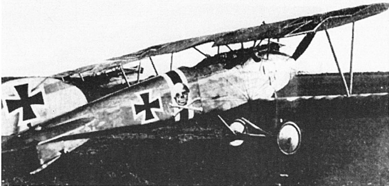
A later series example of the Albatros D.III with a Teves und Braun radiator offset to the left.
