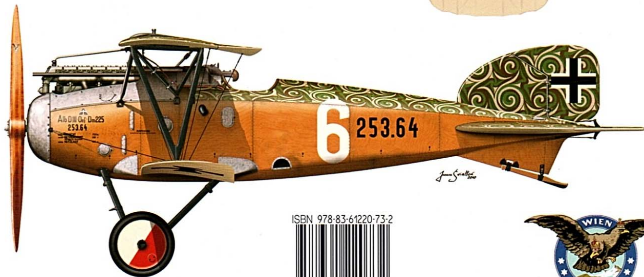
An Oefag build Albatros D.III 253.64 series from Flik 42J. This aircraft was flown by Kpr. Geza Keisz. Wings, tailplane and top decking was covered by printed whorled camouflage. Interesting combination of iron cross on the wings and straight cross on the tail. August 28, 1918. Note raised guns on this aircraft. The red-white wheel discs indicate Flik 42J aircrafts.
