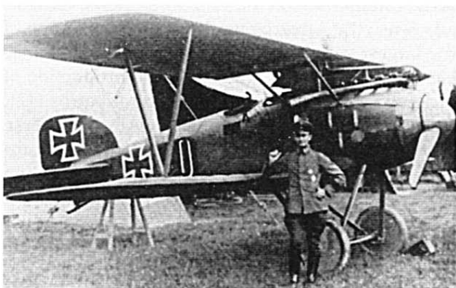
Lt. Reinhold Oertelt of Jasta 19 and his Albatros D.III 1997/16. The aircraft was from the first production batch. The brace on the cockpit holds a flare pistol. Below there is a container for flare cartridges.
