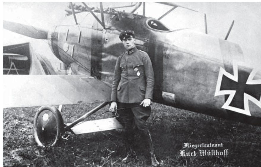
Jasta 4 pilot Leutnant Kurt Wüsthoff stands before his Albatros D.III(OAW), painted in Jasta 4 identifying black wound stripe. The various reflections of the high-gloss fuselage reveal the dents and wrinkles the birch skin accumulated over time. Note the axle fairing and round OAW valve access covers on the wheels.
