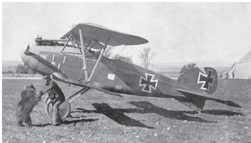
Albatros D.III(OAW) in Palestine. As the 600- and 750-series Johannisthal-built machines, the OAW Albatrosses had a rectangular footstep in the nose, ostensibly to assist ground access to the engine, although simple ladders were often used. Due to higher ambient air temperatures as compared with northern France, this D.III has two radiators.
