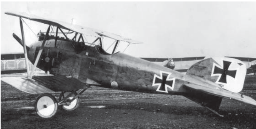
Unarmed Albatros D.III prototype at Johannisthal. Its sleek and ruggedly attractive lines belied structural problems with its new sesquiplane wing design, which featured the classic "V" interplane strut.
