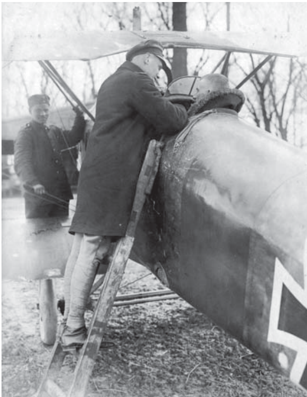
Lothar von Richthofen in the cockpit of a first production-batch D.III. Items of interest include apparent repair patches on the wings and fuselage; nonstandard windscreen; padding on the ladder; central radiator; and round footstep. Taken at Roucourt, c. late April, 1917.
