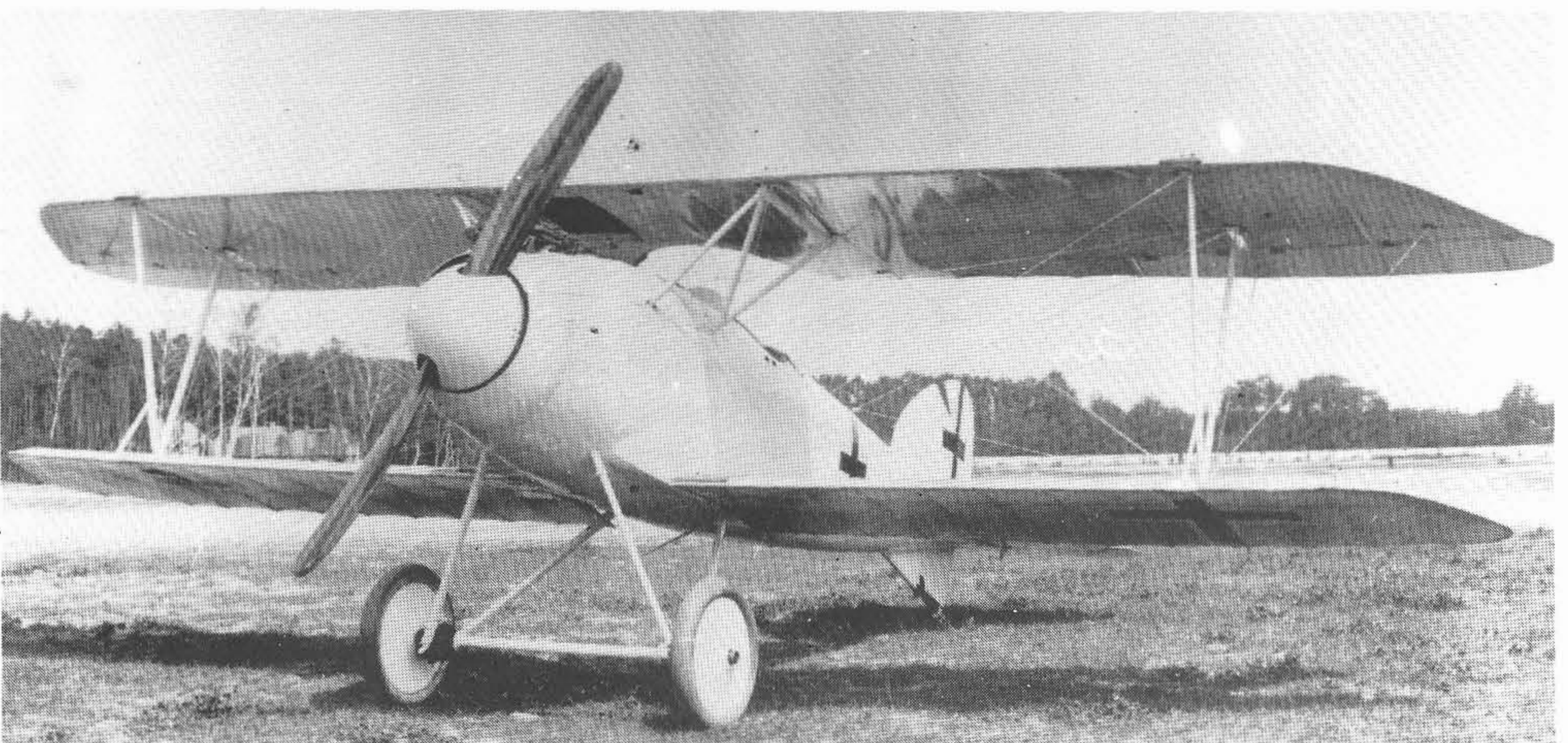
Below, D.III D.606/17 belonged to the Zentral Abnahme-Kommission , the organisation responsible for the production acceptance of German aeroplanes during the war. Those with an eye for detail may note the extra wing bracing cable from the lower end of the 'vee' strut to the penultimate upper wing rib and those distinctive auxiliary wing braces.
