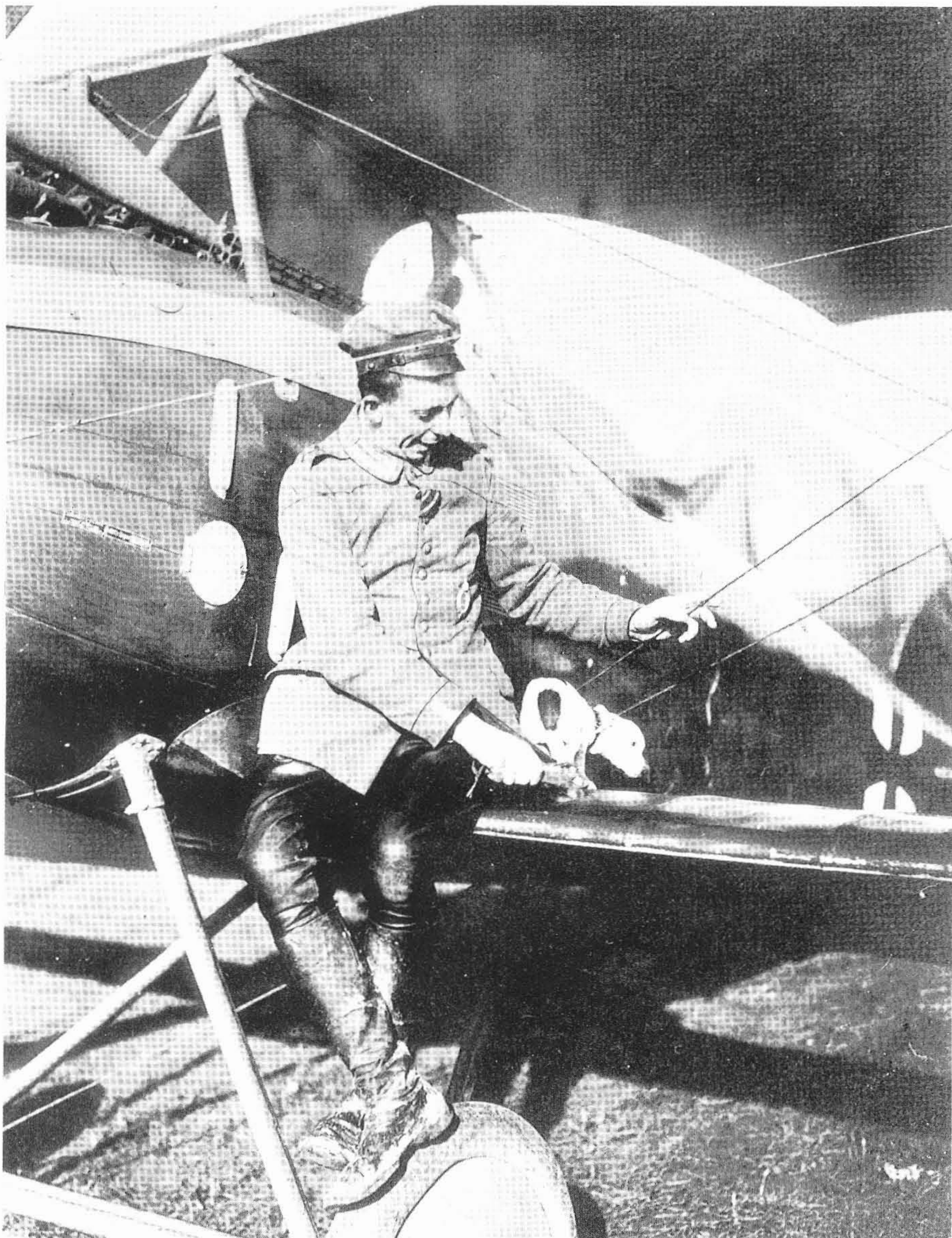
Vizfeldwebel Karl Holler of Jasta 6 gives a good impression of the size of this brand new Albatros D.I photographed at Ugny l'Equipée in August 1916. Modellers may note the method of fuselage ply covering, metal louvres, inspection panel, undercarriage and central cabane strut fixtures. The dark fuselage may indicate a red-stained finish and the wings bear evidence of camouflage painting – note style of insignia. (A E Ferko)
