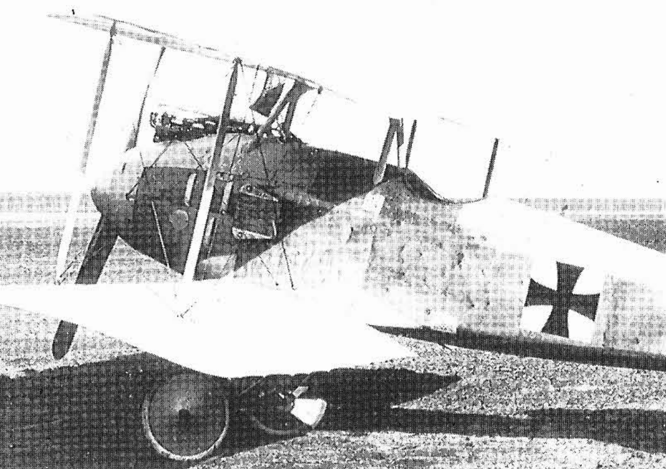
Below, prototype D.I in plain finish and non-standard exhaust at Johannisthal in early 1916.
