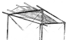
Rear fuselage detail showing the three-ply turtleback fairing supported on three wooden battens.
