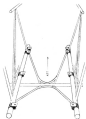
Engine bearers were formed of steel tubes, supported on a tubular structure welded integrally with fuselage and 'ventro-section' struts. Note the slight attachment lugs for the engine cranks.
