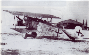
Below, appearing factory-fresh is this Fokker DVII (GAW) 9423/18 on a British aerodrome after the war. The painted camouflage on the cowling was seen on many GAW-built machines.
