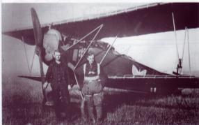
Centre and below, two views of Lieutenant Hans Jungwirth's Fokker D.VII (D.IV) 4484/18 of Jasta 76 at Bald airfield in 1918. Of interest are the pale rib tapes over the printed-fabric-covered wings and various stencil data on struts and lower wing ribs (centre photo). This aeroblane is depicted in colour on the rear cover. (The AE 150 Forke)
