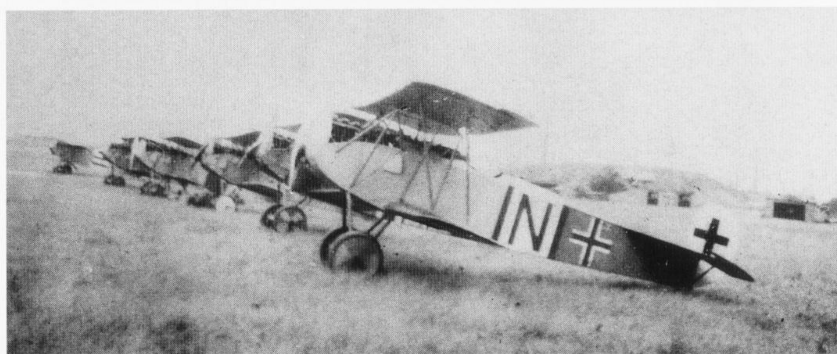
Right, not a very sharp picture, and the unit is unidentified, but these OAW D.VIIs in late markings all have their upper cowl panels removed to keep the ammunition cool in the hot summer weather. The wheels are quartered in photographically light and dark colours – green and mauve? (GVW via A Durkota)
