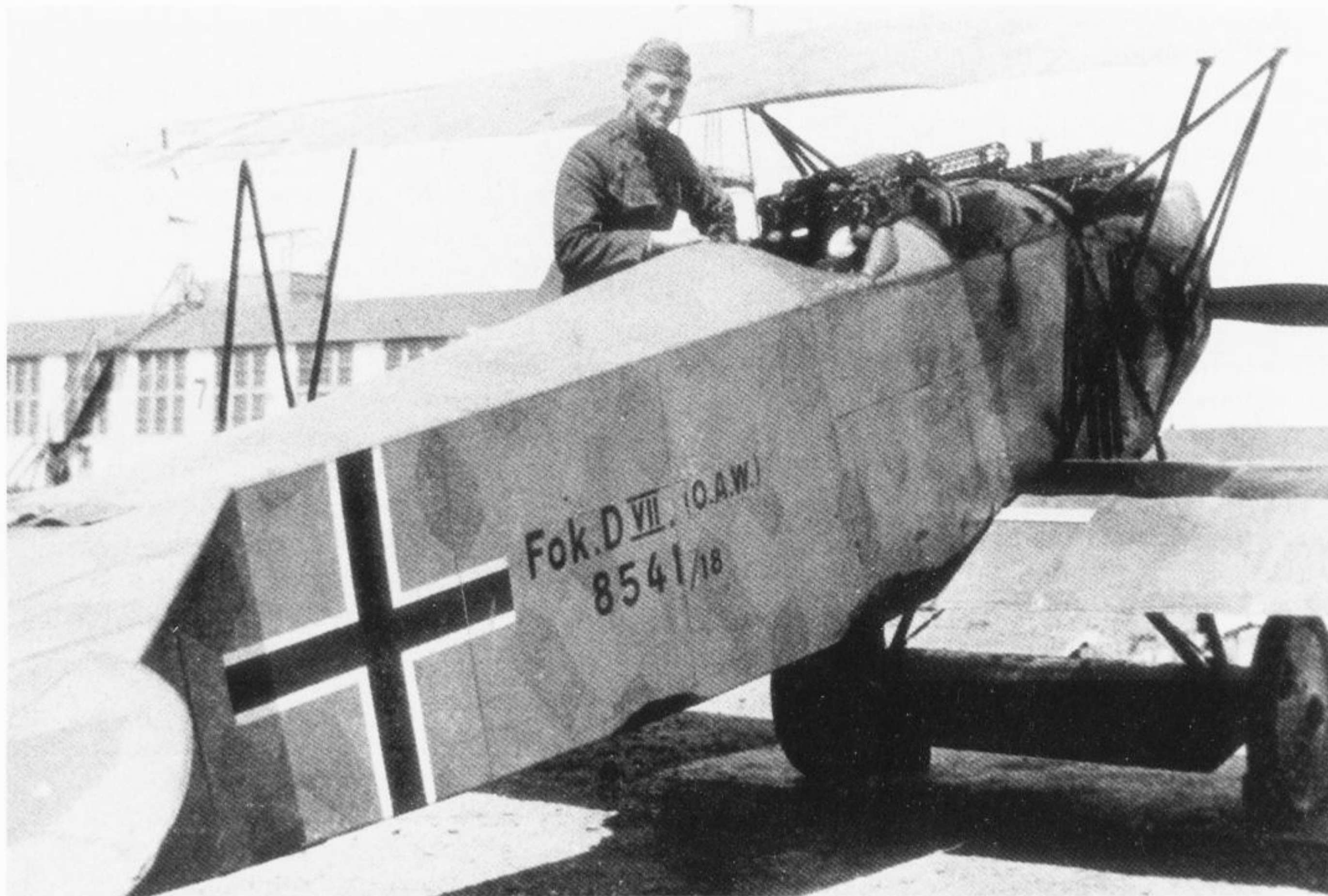
Left, the fuselage spacers and bracing wires of 8541/18 are clearly visible through the four-colour fabric. Samples at the RAF Museum still retain impressions of these wires; the fabric slackened when first doped and moulded itself to the wires, which left their mark when it dried and tightened. (GVW)
