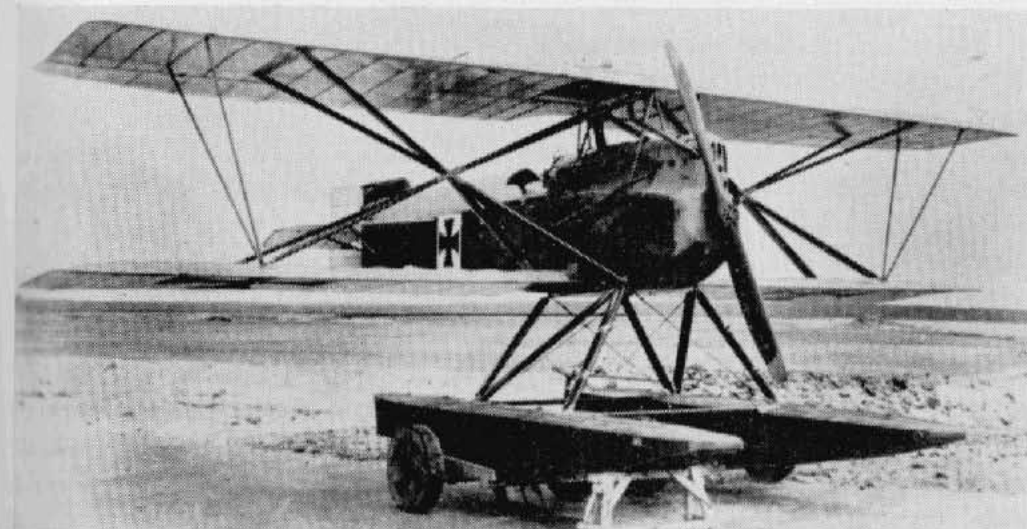
Brandenburg K.D.W. with 160 h.p. Maybach Mb III engine. (Photo: Imp. War Museum.)
