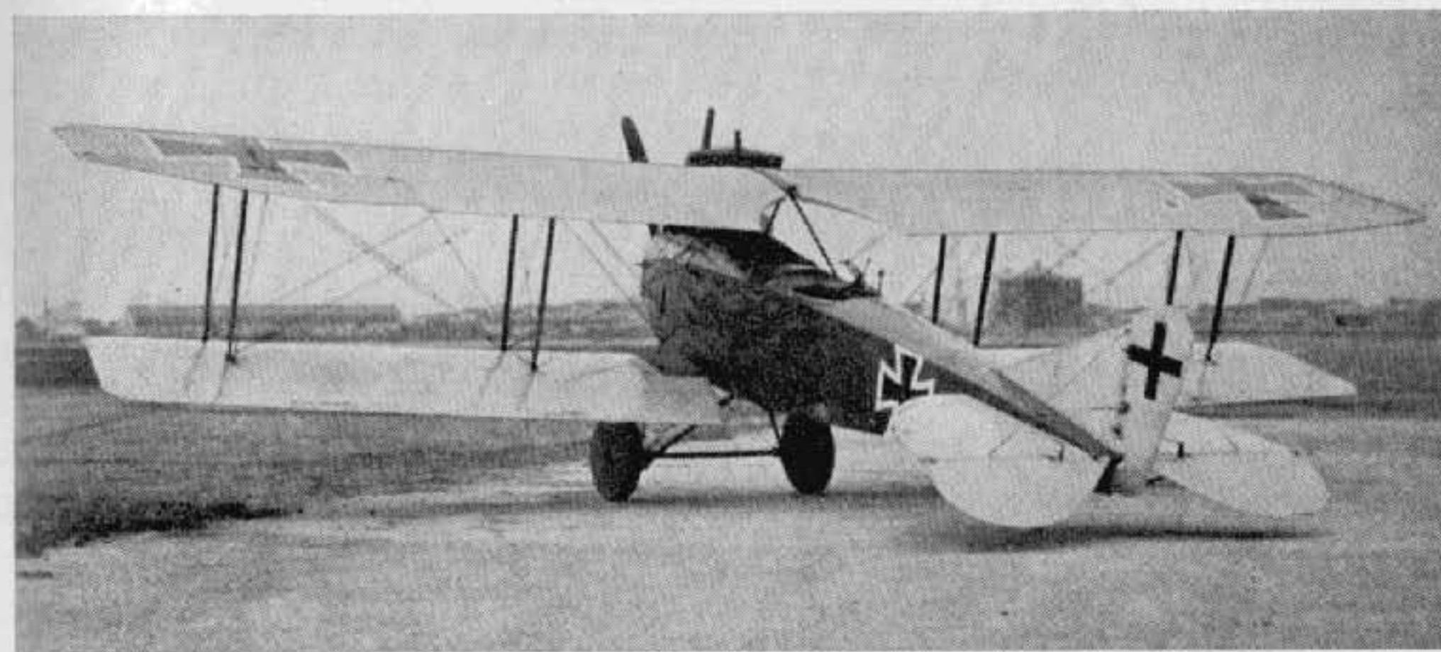
Albatros C III (licence-built by L.V.G., with further modified fin and rudder). (Photo: A. Imrie.)
