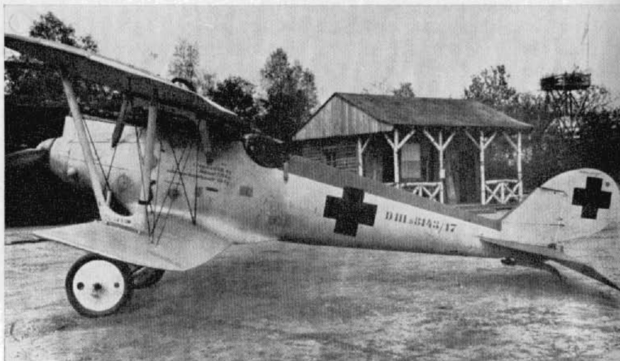
Pfalz D IIIa, with modified tailplane (serial 8143/17). (Photo: Egon Krueger.)
