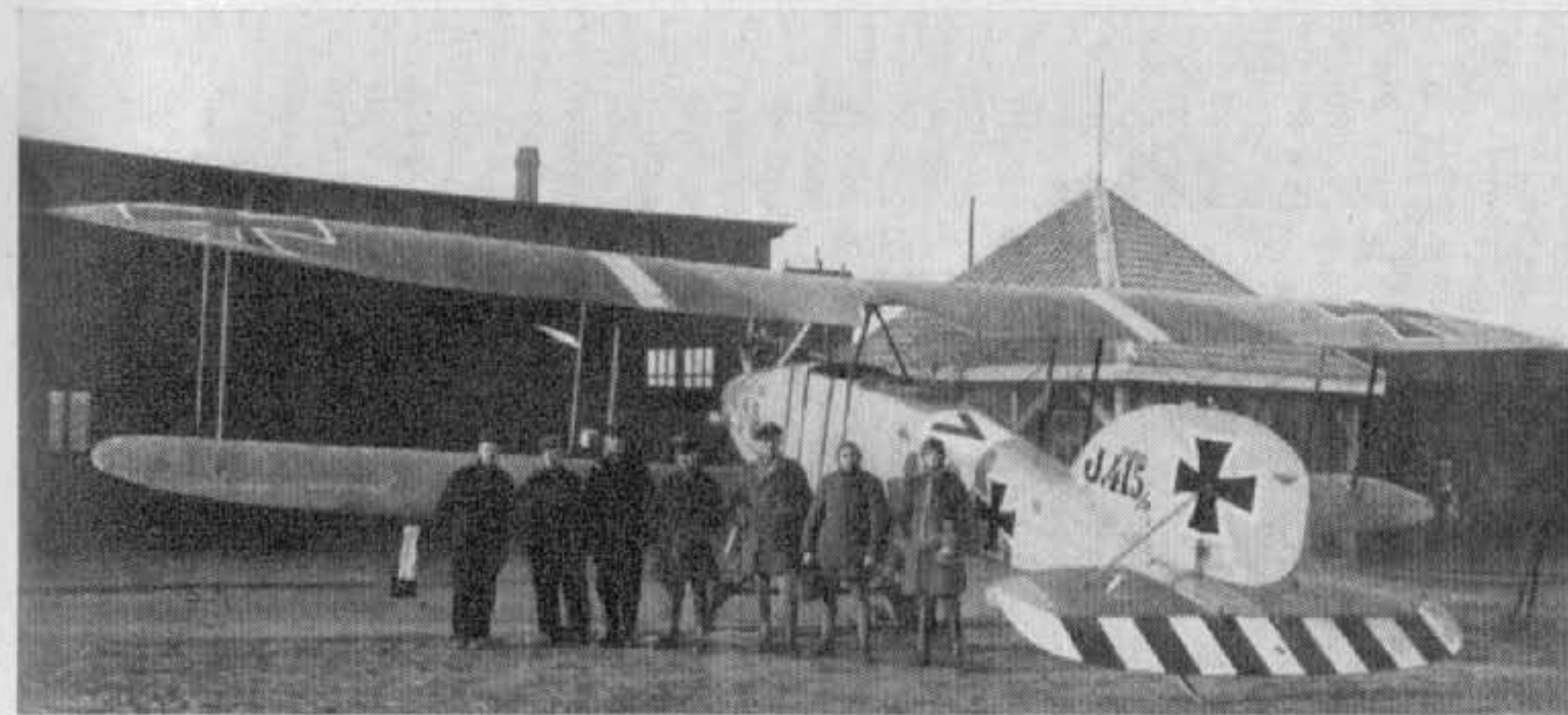
One of the specialised ground attack aircraft used in increasing numbers by the German Air Force from 1917 onwards—an Albatros J I (J 415/17). (Photo: A. Imrie.)
