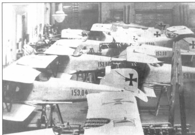
Almost finished... Note the differences between the suction piping of the 185hp engine of 53.60 and the 200hp engine of Albatroses series 153. 153.01 was fitted with the earlier exhaust collector, the same one as planes of series 53.
