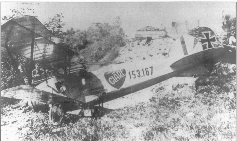
An escort plane of Flik 2D, Albatros D.III (Oef) 153.167 after an emergency landing at Belluno in May 1918. The camouflage of upper surfaces is quite distinct as well as the personal marking “CLÄRE” in a heart on the port and a quatrifoil on the starboard side of the fuselage.
