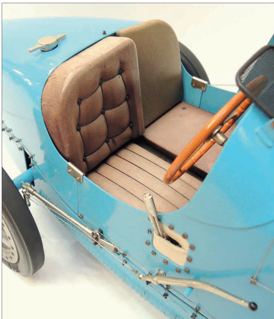
The driver's seat was padded for comfort, the riding mechanic's 'perch' was not – to save weight. Note the external gear lever and handbrake detailing.
