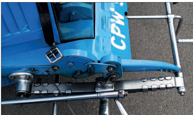
Above: Later cars with 330mm brake drums and extra (inverted) leaf spring (stiffener), had the leaf springs clipped at both ends, not just the front.
