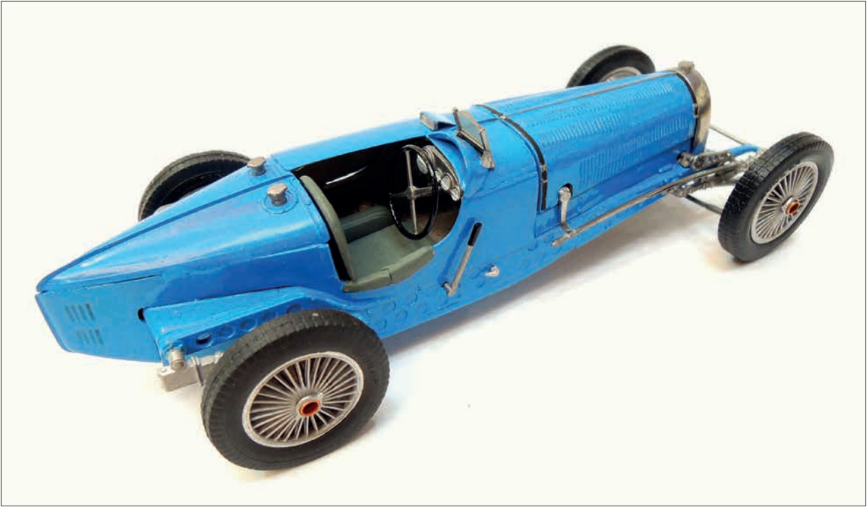
The Type 59 model (manufactured by Brumm) shows the longer, lower design and build of Jean Bugatti's later Grand Prix car. Note how the rear suspension is externally mounted – rather than internally enclosed on the Type 35 series. The 'spine' is also evident.
