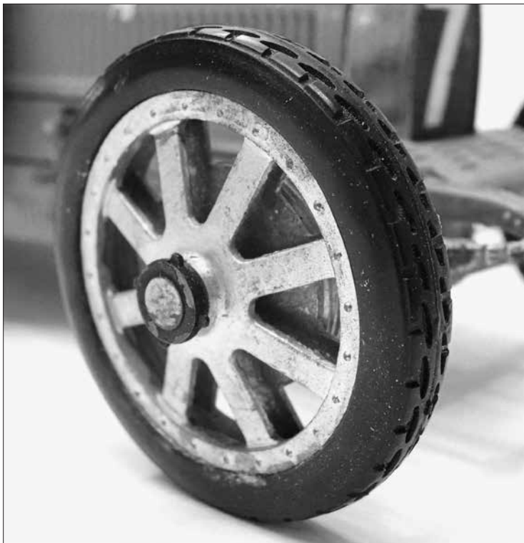
The essential cast alloy wheel with inset brake drum housing. Thirty-two or 24 screws on the rim according to date and specification.
