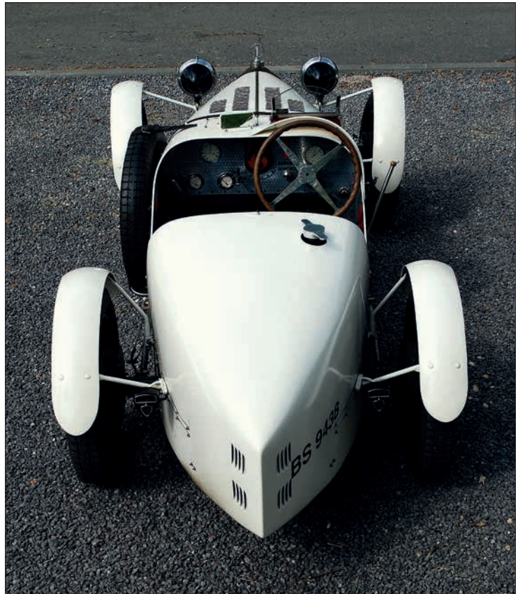
Pointed stern, mudguards (or wings) and rare white paint. Note the elliptical front-to-rear body planform.
