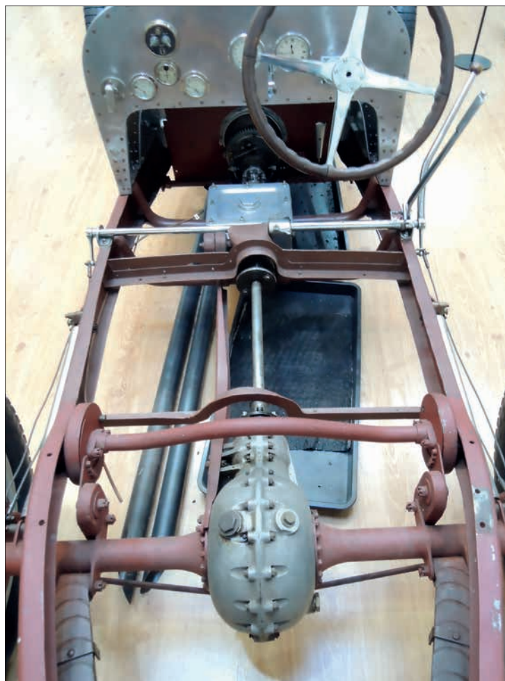
The Type 35 series chassis – thin where possible and thicker where required. Note differential casting and scuttle design.
