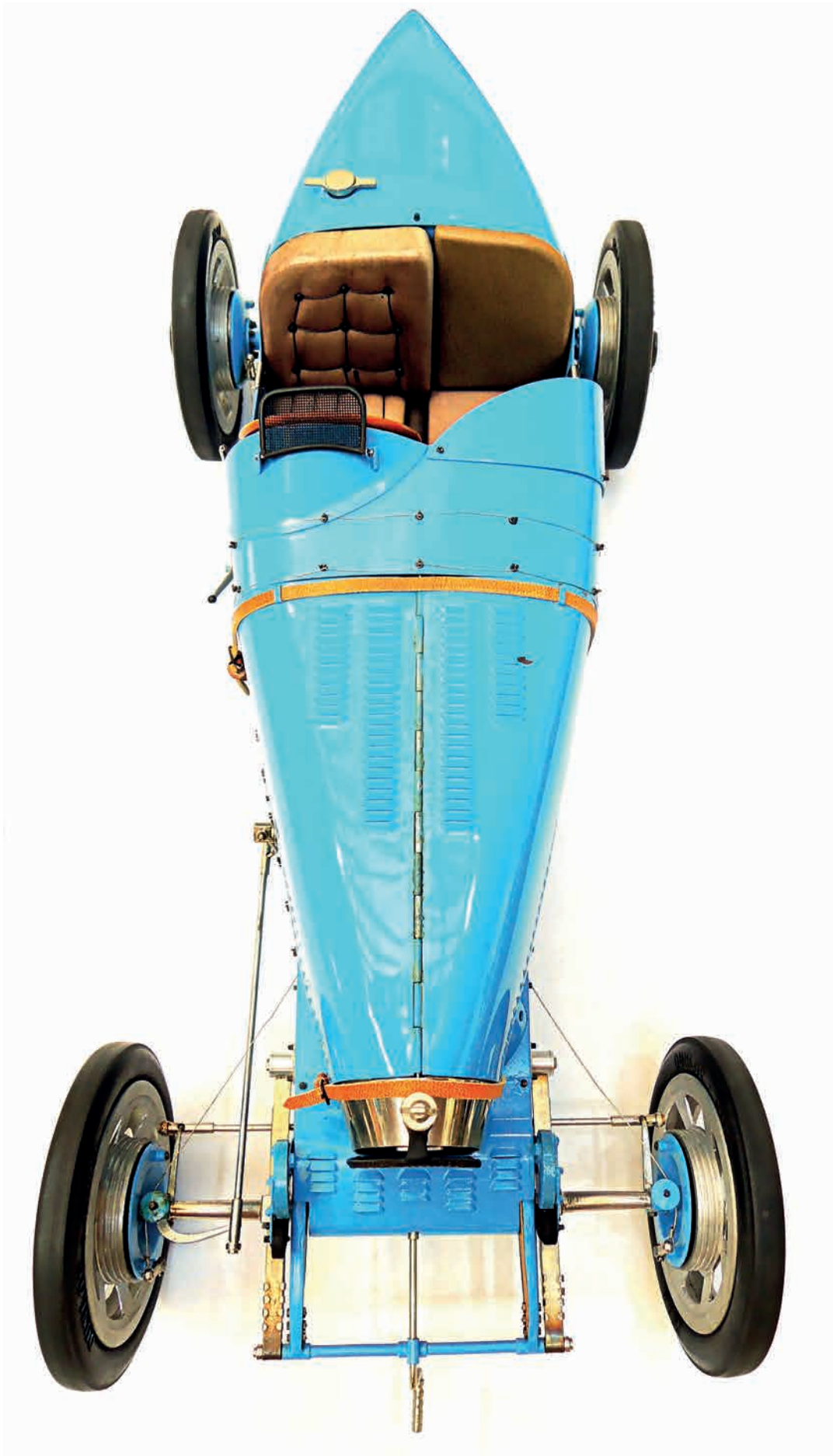
The genius of Ettore Bugatti's design is easily grasped in this view of the Type 35. Every line 'works' and blends into an elliptical whole. Note how the nose and the tail both narrow – to reduce aerodynamic drag. This is the 1/8 scale Art Auto Collection model at its detailed best.
