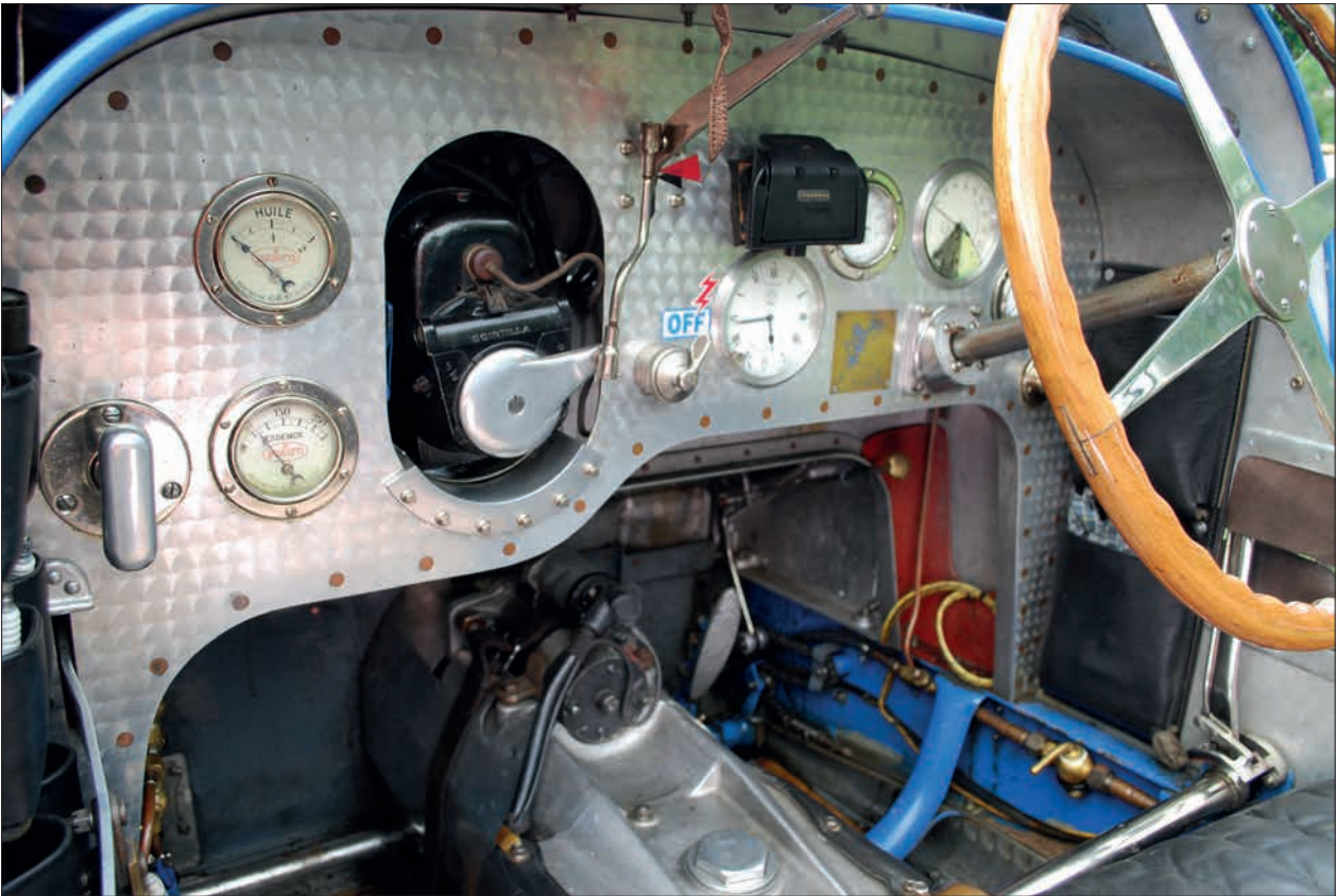
Dashboard design was not ignored by Bugatti, the Scintilla magneto and the walnut wood wheel being of note.
